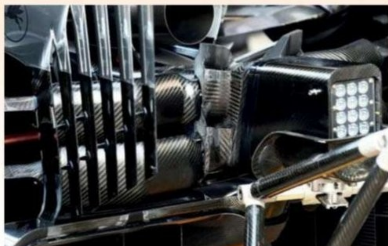
Clever interpretation of the rulebook has led to these 'mushroom' shrouds incorporated into the rear wishbones of the McLaren MP4-29. It's thought that they assist in managing airflow around the diffuser and compensate in part for the removal of the lower element of the rear wing mandated by the 2014 technical regulations
