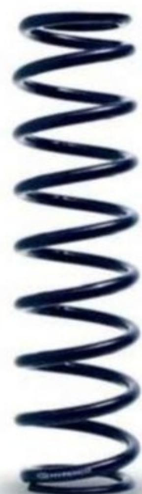
Hyperco's Optimum Body Diameter spring. See how the body diameter increases down the length of the spring, which optimises the applied stress and so the number of coils can be reduced; saving weight
