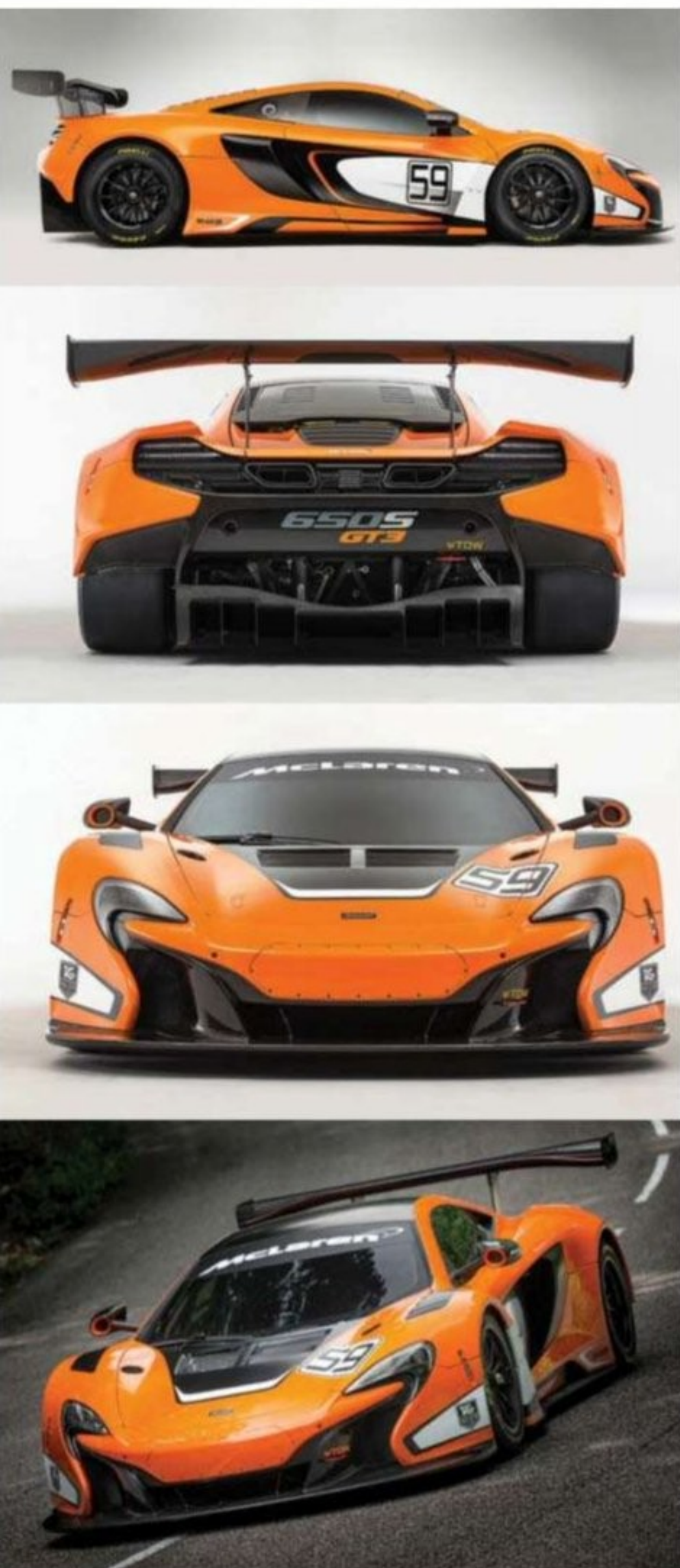
Every body panel is new, but improvements include maintenance accessibility as well as aero and cooling considerations. Cut away rear bumper replaces complex road car-derived design
