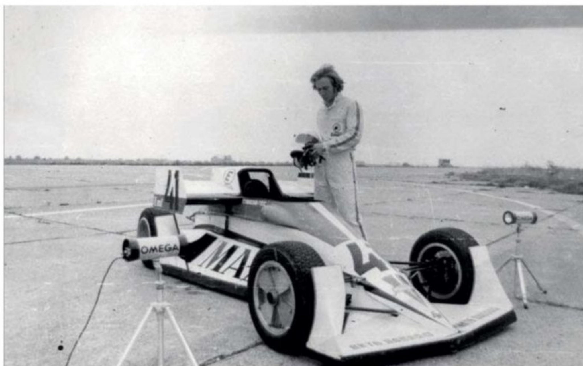
The MADI-Moskvitch had cable-linked suspension which interacted with resilient elements to control body roll
