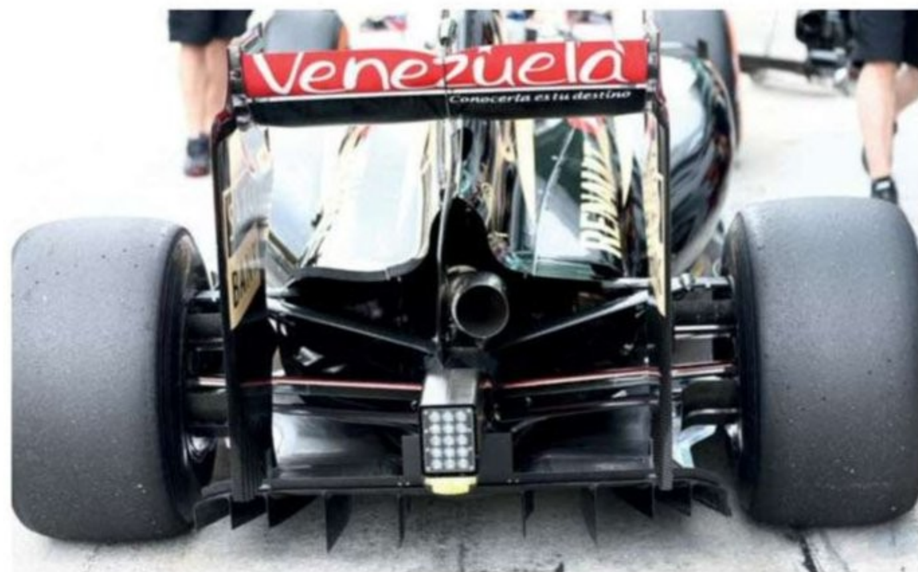
The slight assymetry of the wing strut and tailpipe arrangement is just as effective and lighter than other teams' more complex structures
