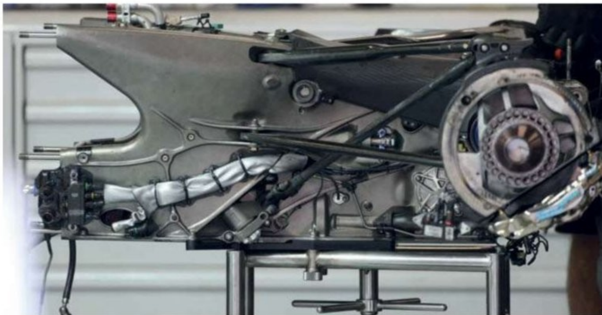
Above: Titanium-cased gearbox is unique to the E22. Full carbon fibre is a future option
