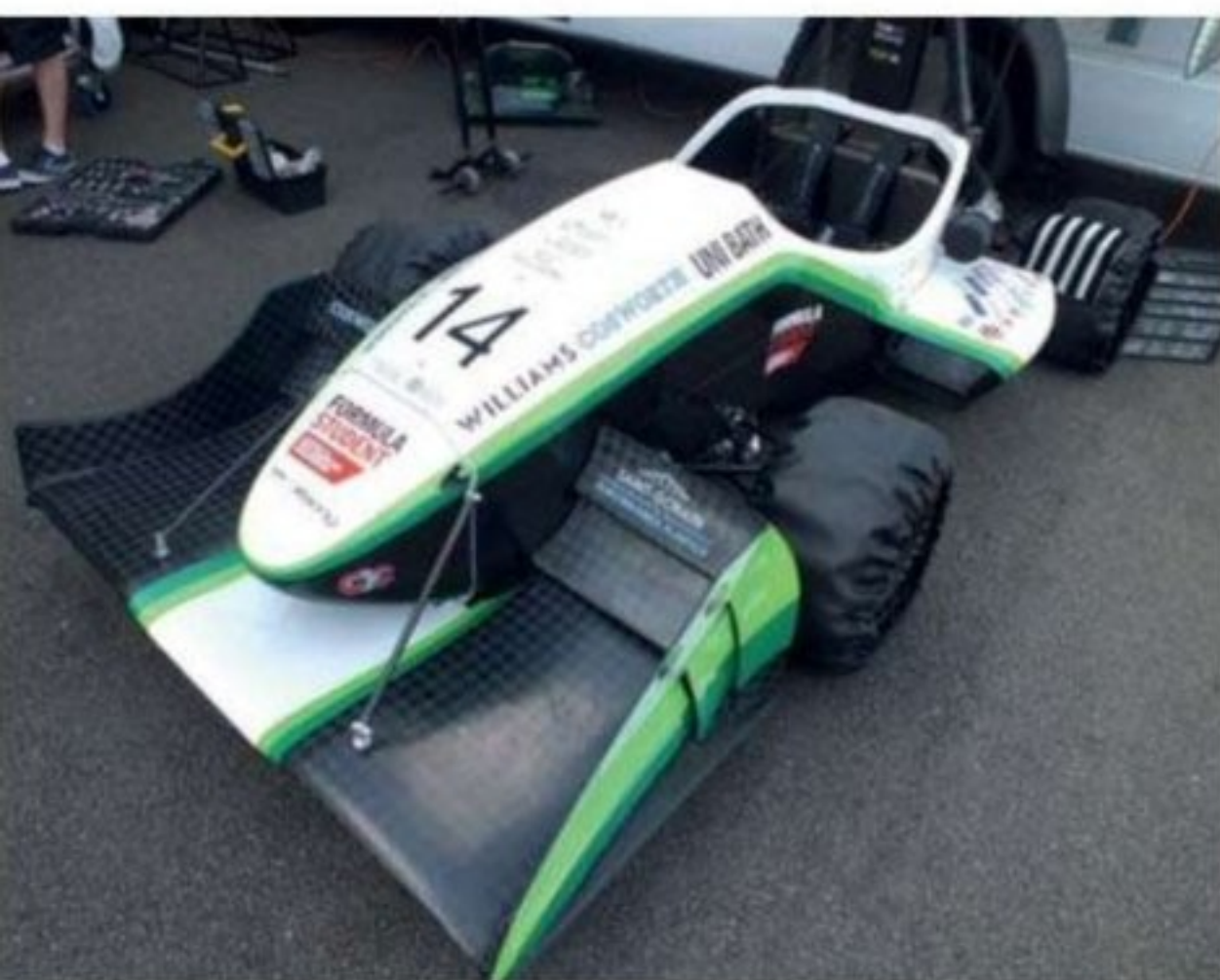
The University of Bath's entry featured an impressive front wing that uses vortex management to improve efficiency. Structure weighs only 3.5kg, but drag would be punitive at higher speeds
