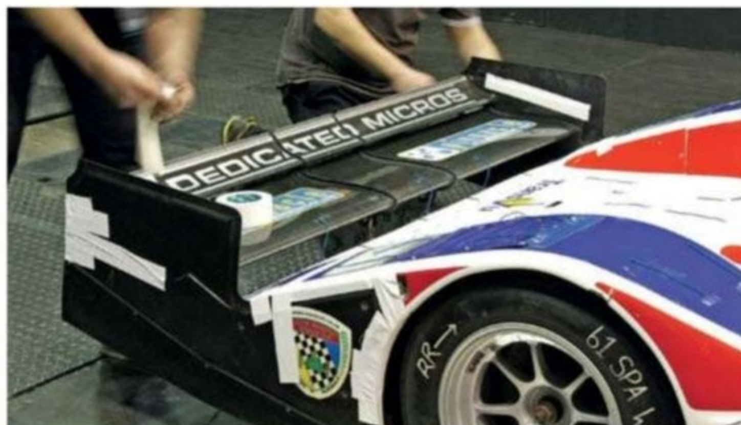
Picture 4: Lowering the wing to its normal position made a substantial difference to downforce and balance
