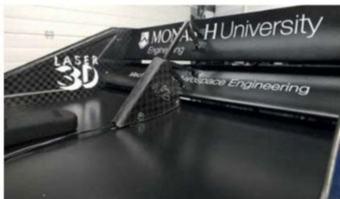
Monash University's entry featured DRS front and rear. The middle and top flaps on the rear wing open for straight line speed
