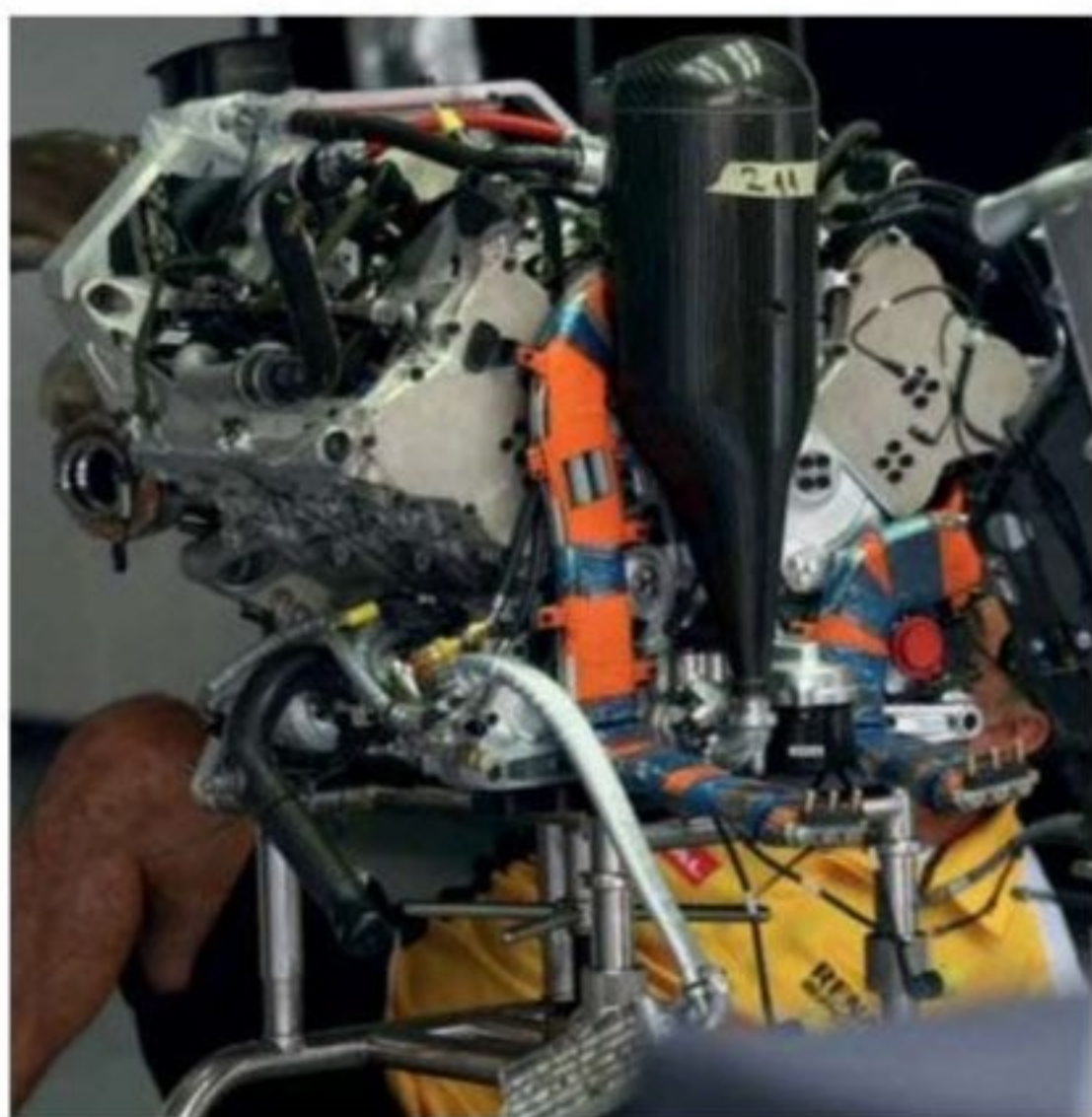
Reliability and power issues plagued the Renault V6 at the start of the season. Cooling problems are now mostly resolved
