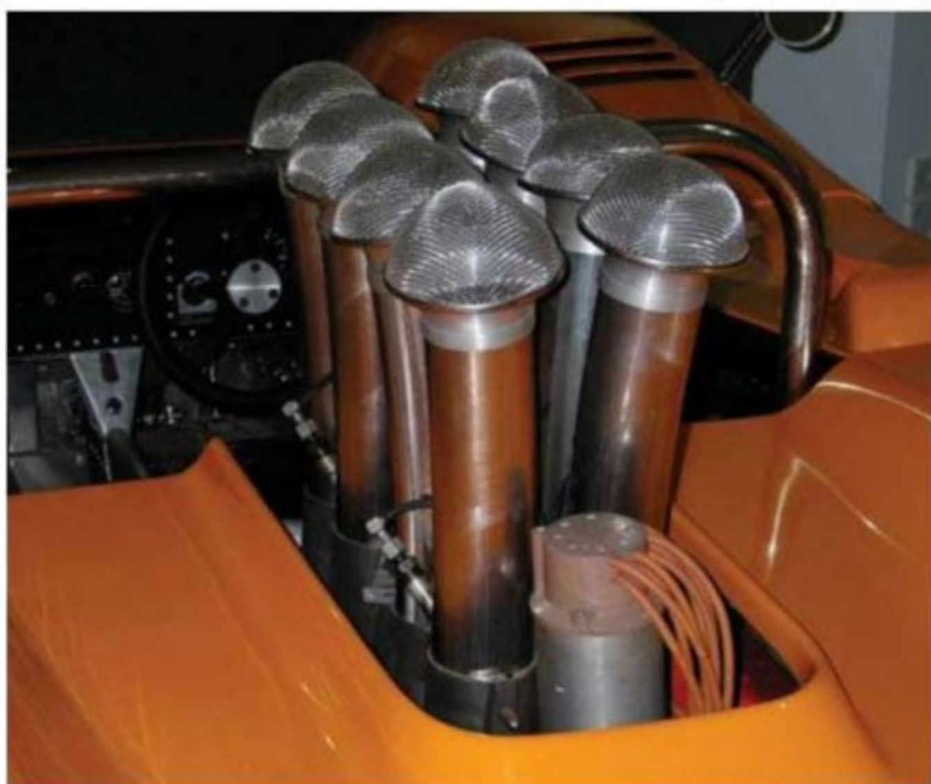
Tall stacks on the mechanical fuel injection. Magneto ignition
