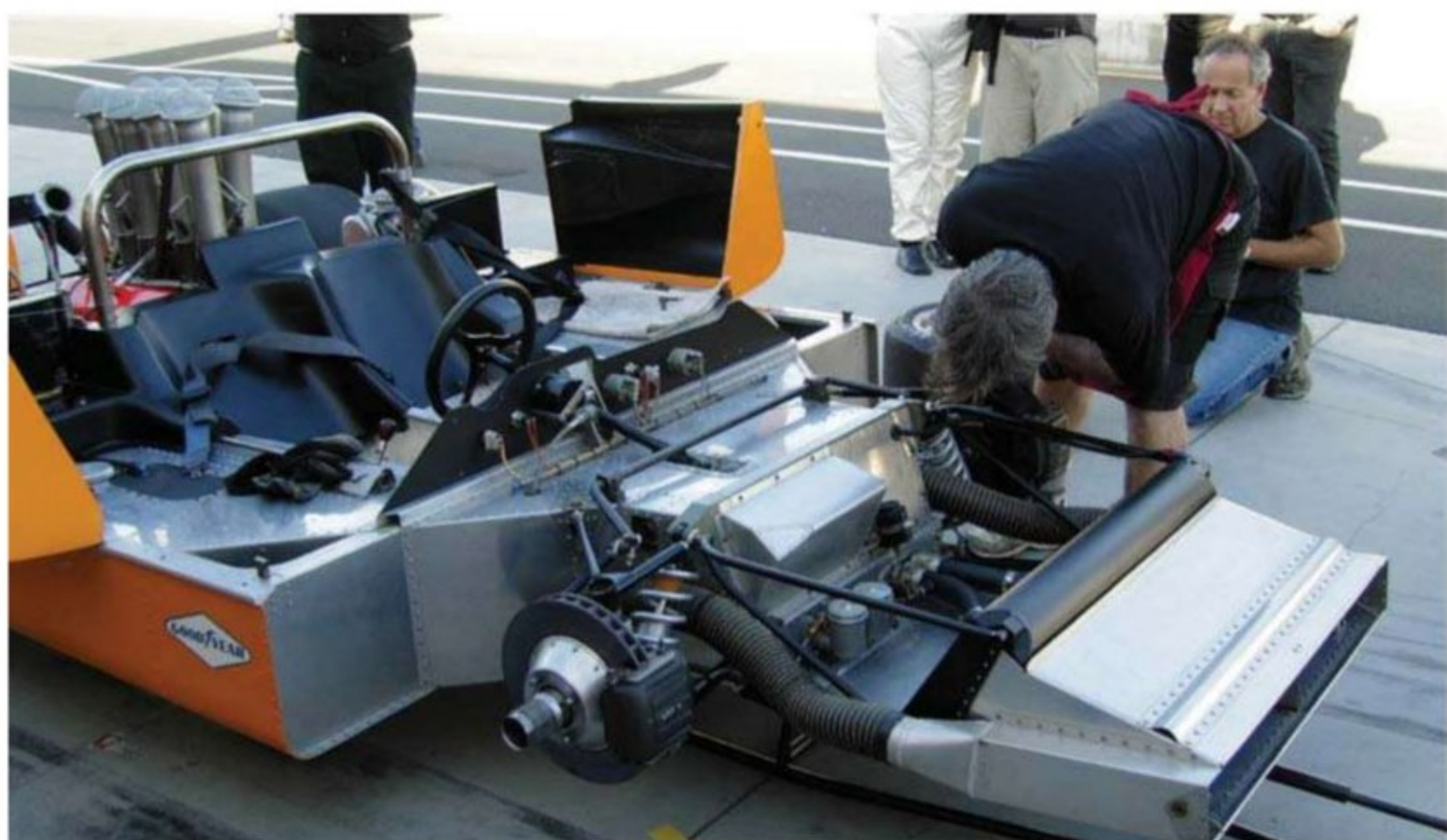
The Lockheed 11" ventilated discs were state of the art for the time
