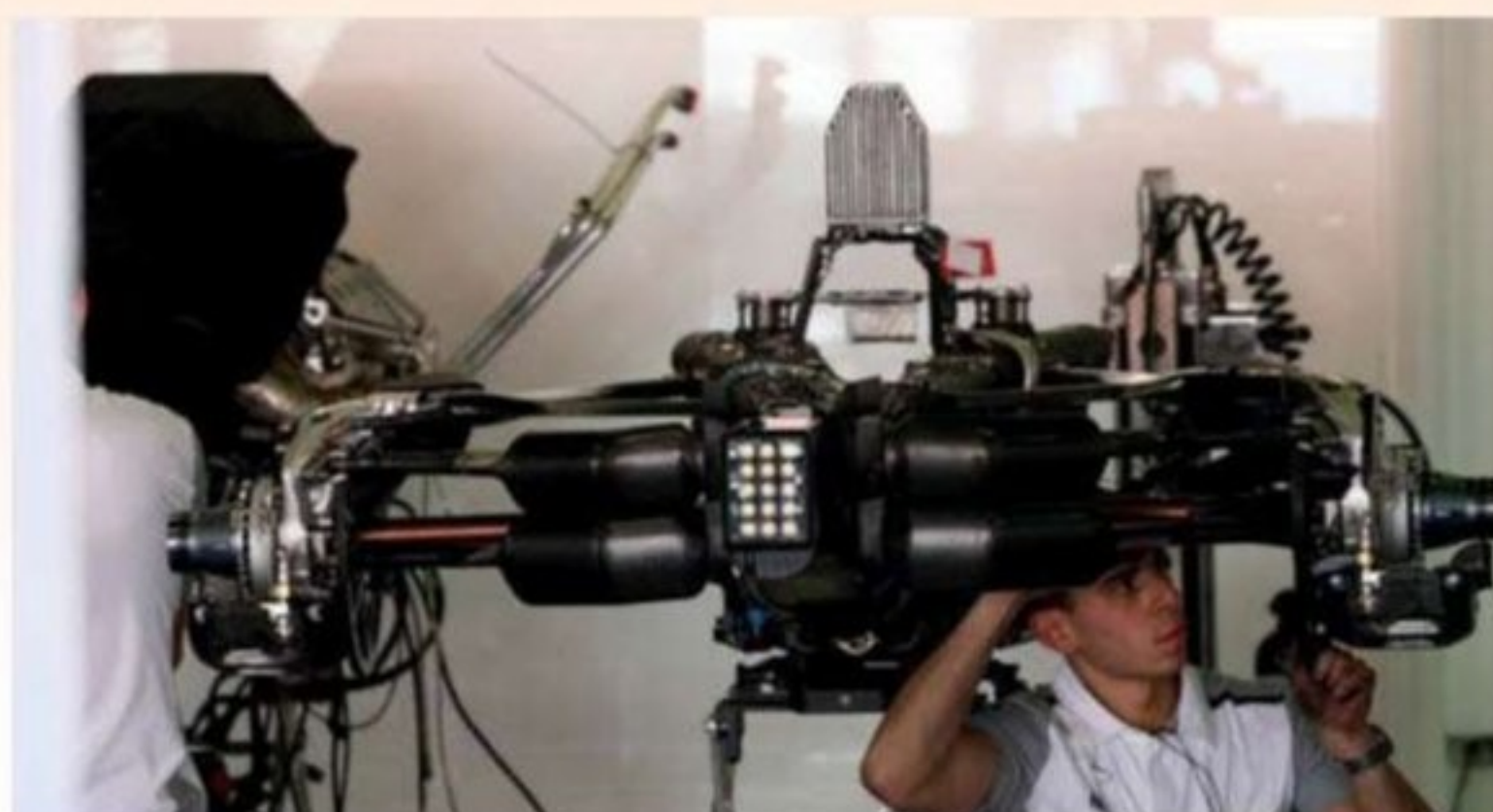
Clever interpretation of the rulebook has led to these 'mushroom' shrouds incorporated into the rear wishbones of the McLaren MP4-29. It's thought that they assist in managing airflow around the diffuser and compensate in part for the removal of the lower element of the rear wing mandated by the 2014 technical regulations
