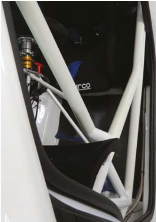
MINI design cues can be seen on the CAD tested and FIA-specification Golf roll cage
