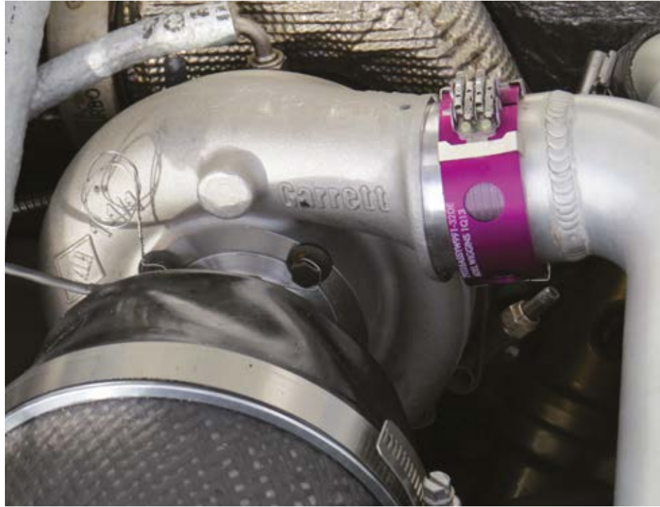
The Garrett turbocharger sits on top of the 16-valve engine – the specific turbocharger is designed to suit a 35mm restrictor, as per Chinese rally regulations
