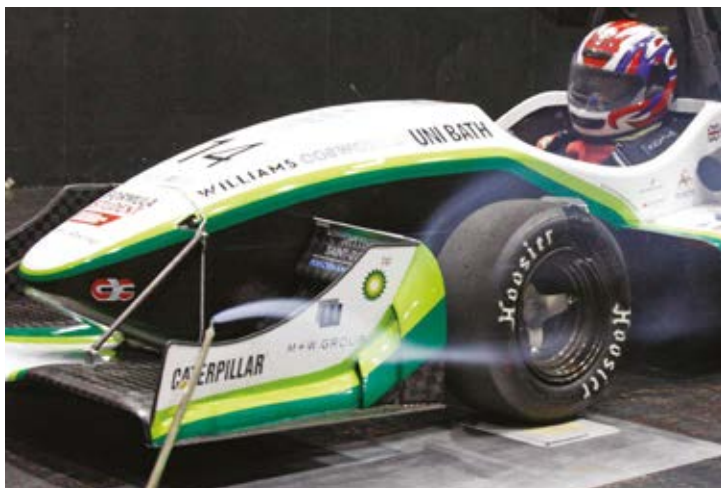
Figure 3: The upper surfaces of the front wing and end plate diverted air over and around the tyres
