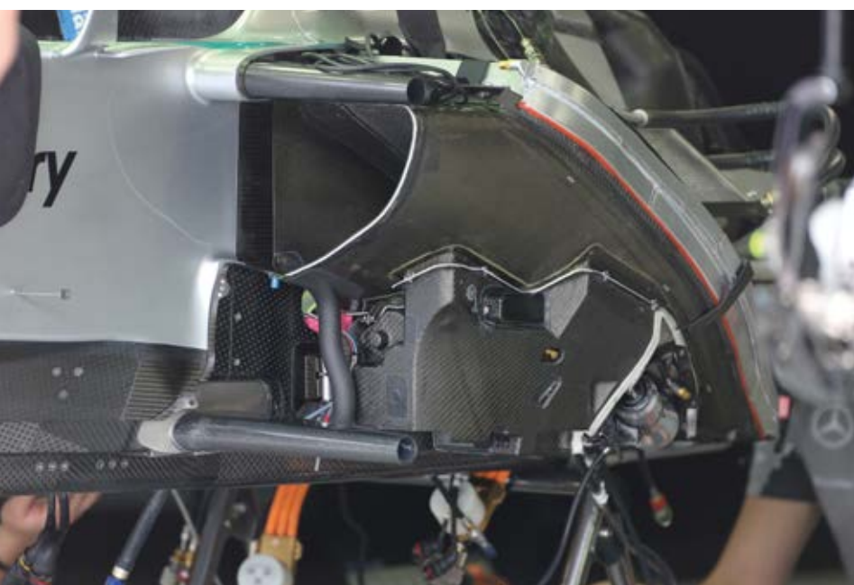
The space under the sidepod area of the car is exceptionally neat and tidy. Visible are the heat exchanger and the upper and lower side-impact structures, which are common to all 2014 F1 cars
