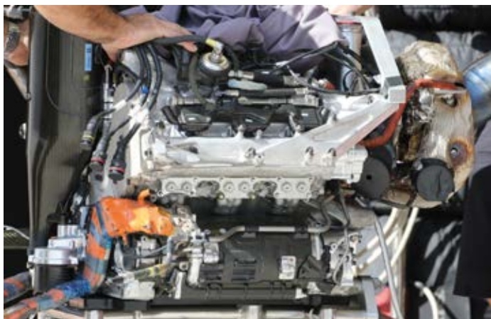
The Renault RS34 V6 engine showing clearly its turbocharger
