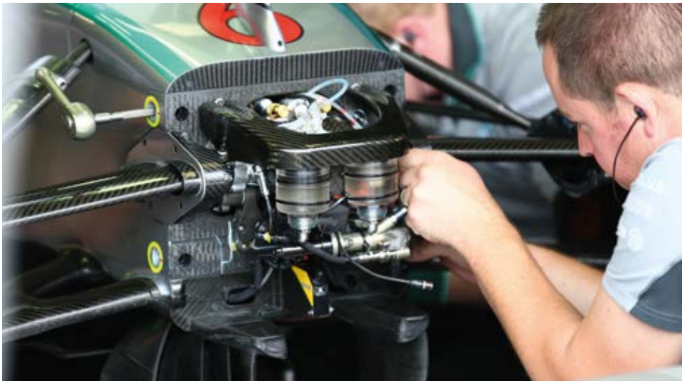
The front bulkhead, with master cylinders evident, shows typical clean Mercedes lines
