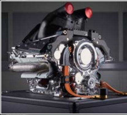
The Mercedes power unit is full of innovation including split turbo concept (above) and log-type exhausts
