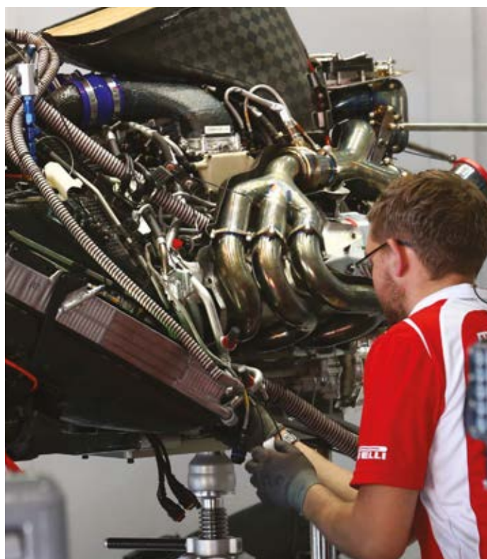
Ferrari-style exhausts as seen on the Marussia MR03. Note lack of thermal barrier
