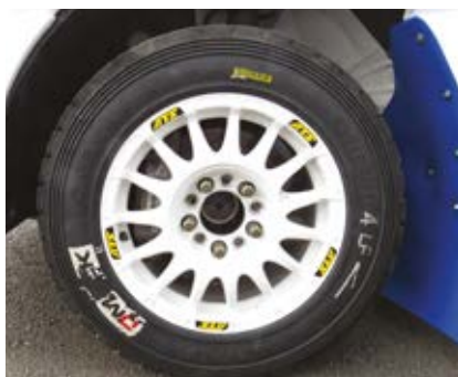
A Dmack tyre on an ATS wheel – the Golf's exterior panels are mainly Volkswagen steel, with flexible resin composite panelling used on the bumpers, front wings and lower rear wheel arch extensions
