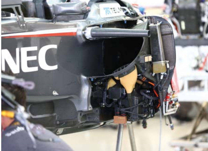
The Sauber sidepod with bodywork removed showing upper side impact structure – but with the lower removed. 'On the car side of things, we had a bad season'
