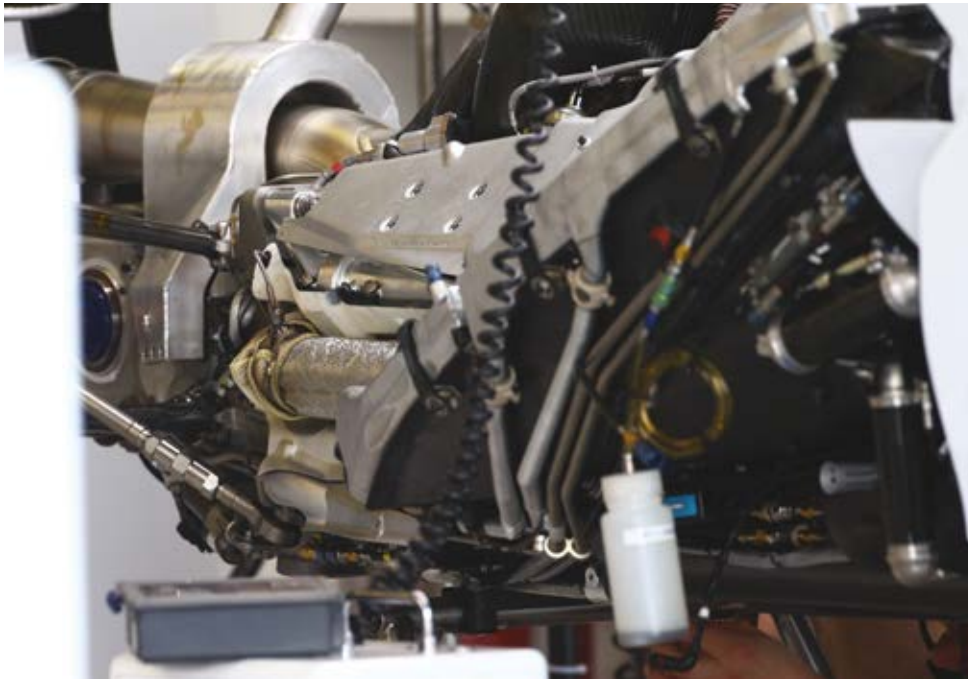
Mercedes HPP embedded staff into its customer teams to advise on installation of the power unit, and the results were quite varied, especially in terms of cooling as can be seen with the Williams solution (above) and the McLaren (below)
