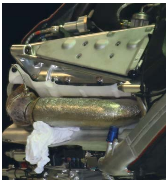
Mercedes Pu106A Hybrid engine showing log-type exhaust
