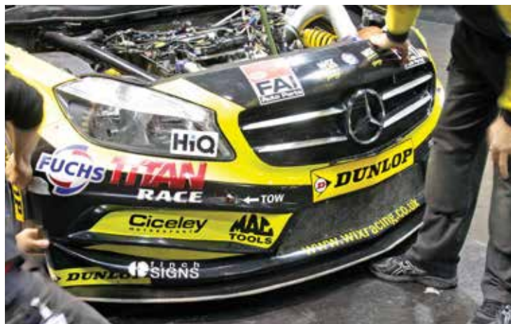
Figure 2: The baseline front bumper arrangement featured a recess directly above the splitter
