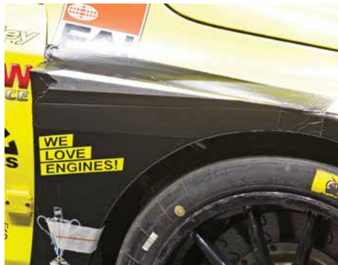
Figure 5: Levelling off the tops of the front wheel arches produced the expected result (it does happen sometimes!)
