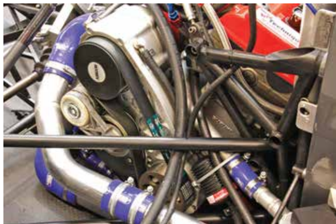
Figure 13: The compact Rotrex supercharger sits on the right side of the engine
