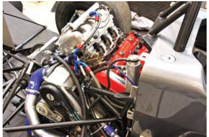
Figure 6: Tubular steel cradle and a machined billet alloy sump pan/floor panel support the Suzuki Hayabusa engine and transmission
