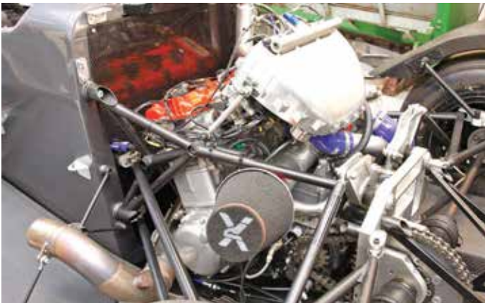
Figure 7: Tubular steel cradle and a machined billet alloy sump pan/floor panel support the Suzuki Hayabusa engine and transmission
