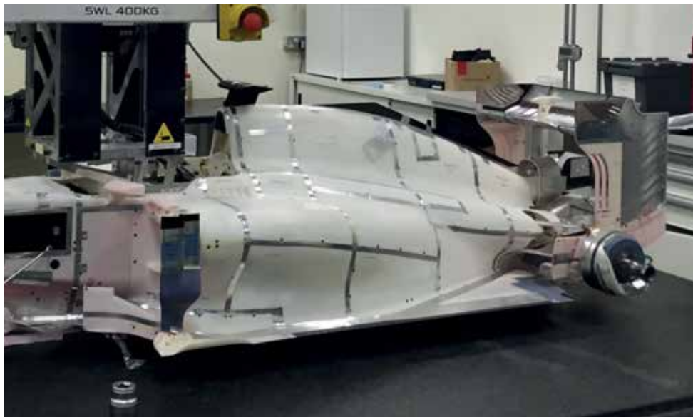
The Y-Lon rearing support and monkey wing seen on the model here is actually the same as MR03 as at this stage of testing. New designs of rear wing supports and monkey wings were designed and were due for testing
