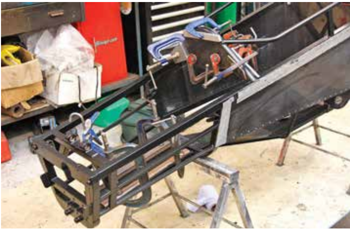
Figure 3: Hybrid chassis construction combines tubular steel spaceframe with composite sandwich panels and a monolithic carbon/epoxy 'wrap'
