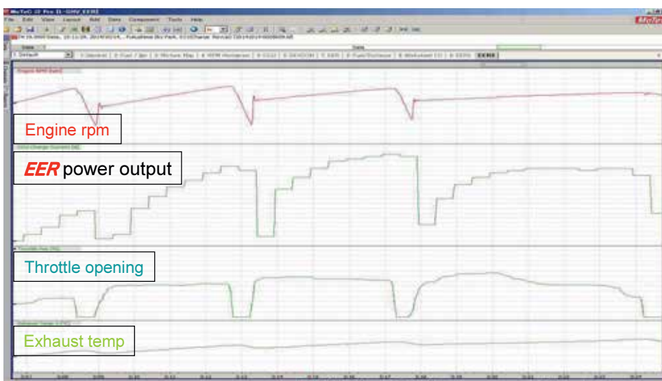
Figure 3: data from Fukushima airport shows the EER-Hybrid's power output and exhaust temperature
