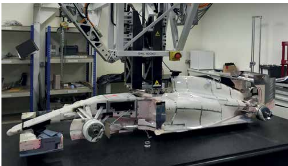
The wind tunnel model pictured here is in incomplete condition. While new front and rear wing endplates are evident, the model lacks some parts as it was in preparation to be shipped to McLaren’s wind tunnel before the team shut its doors
