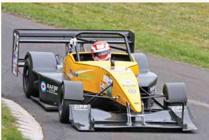
Figure 22: The Force LM continued the central seat trend but still met the old cockpit width rule
