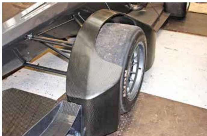
Figure 15: Wheel fairings – one of the features to provoked reaction at the unveiling of the Empire Evo...
