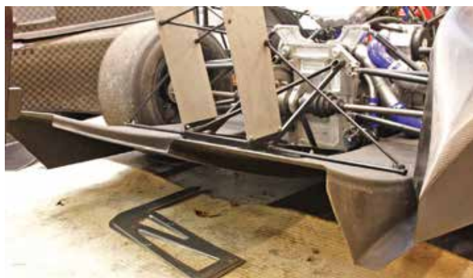
Figure 18: Voluminous diffuser – and entire underbody - is from the '00' series single seater racing car
