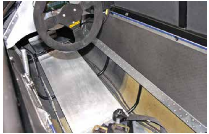
Figure 4: Carbon/honeycomb side panels and aluminium honeycomb floor panel are bonded and riveted to the spaceframe
