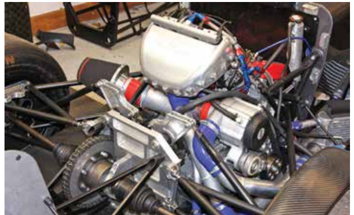
Figure 8: Machined billet rear bulkhead carries the rear suspension mounts and carries the final drive assembly
