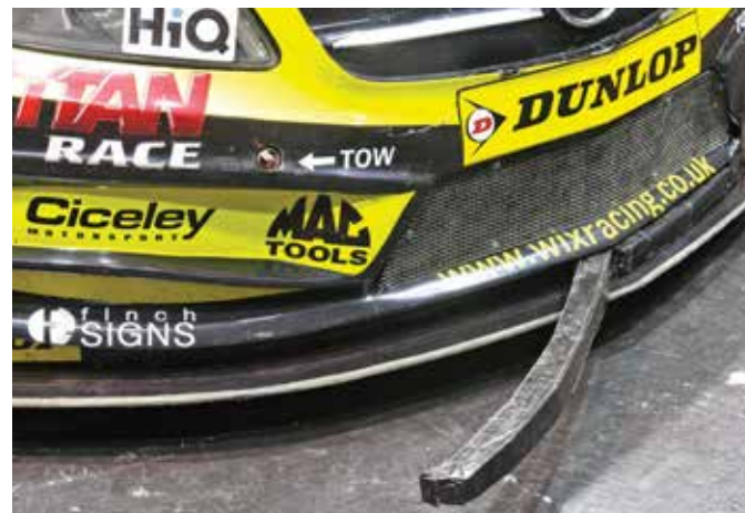
Figure 3: Filling in the recess above the splitter produced a clear result
