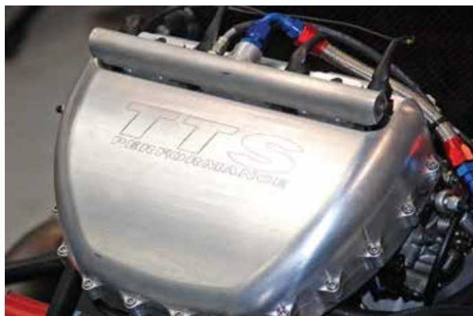
Figure 12: TTS Performance supplied the supercharger kit, which included a machined alloy plenum
