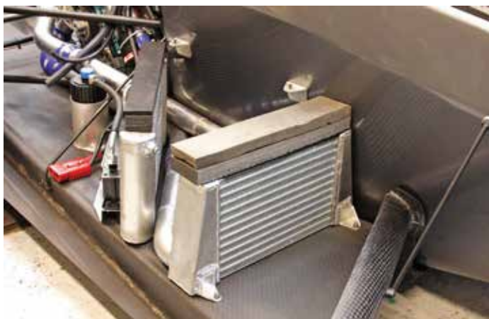
Figure 14: Intercooler, radiator and supercharger oil cooler sit line astern in the right sidepod
