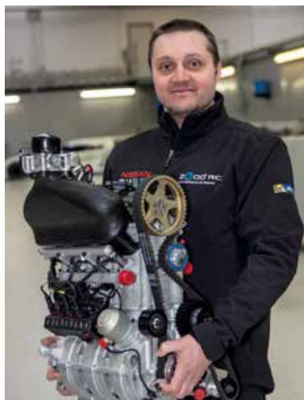
A reduction in minimum weight? For inspiration look at the Nissan Zeod project's three-cylinder ICE
