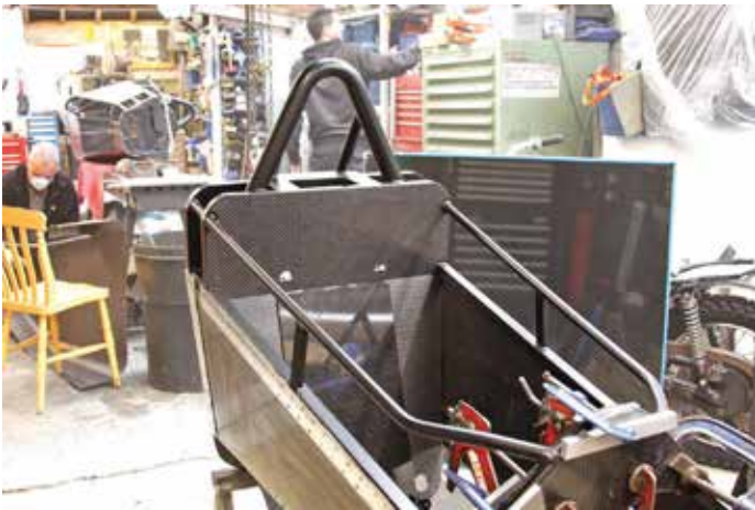
Figure 5: The pared-down cockpit setup on the workshop production line at Empire Racing Cars
