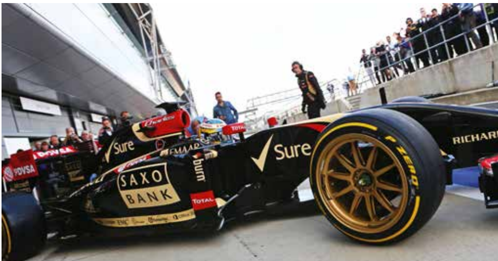
Larger wheels have the advantage of allowing larger brakes, but there are penalties if they go to extremes
