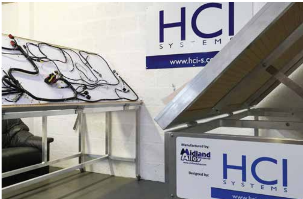
Figure 8: An example of an HCI formboard to help with assembling wiring harnesses
