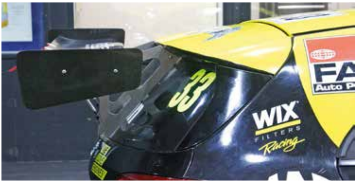
Photo 2: Lowering the roof spoiler very slightly had a tangible effect
