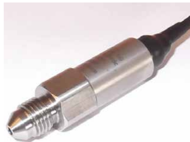
Figure 1: KA Sensors high temperature pressure sensor can operate effectively between -55degC and 150degC. The current demand for F1 is to increase this to above 200degC and although modern sensing technologies can cope, the electronics cannot
