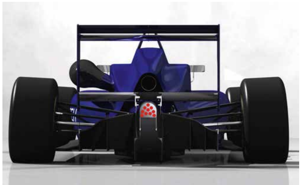
Centrally-mounted exhaust exit flies in the face of convention, but has upset the sports governing body in the process
