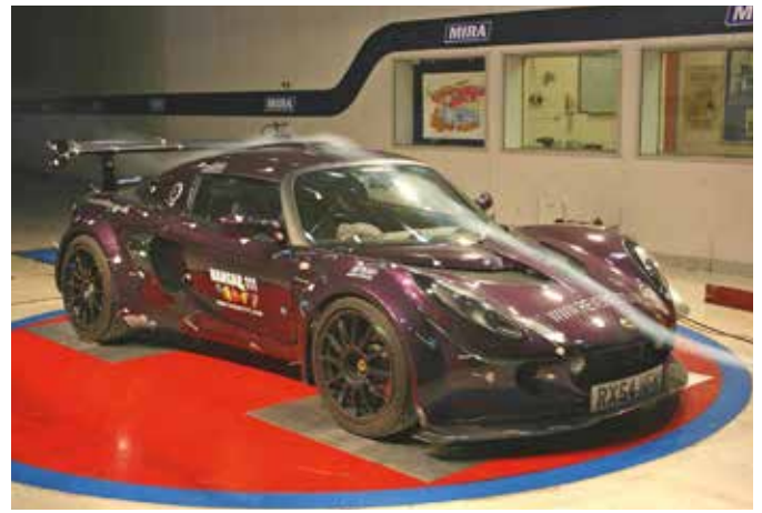
Picture 6: This motorsport-modified Lotus Exige produced comparable CD but greater CL from a more aggressive aerodynamic package
