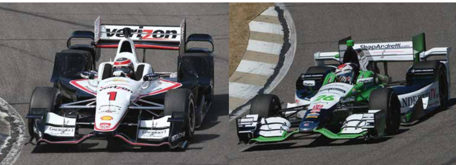
Comparison between the two aero kits demonstrates the different approaches. Chevrolet opted for a more traditional dual-element front wing while HPD went for multiple elements. The covers ahead of the rear wheels carry significance for the super speedway kits that were not yet released as Racecar Engineering went to press
