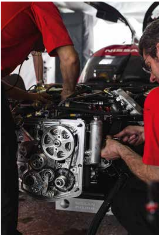
Engine is an even-firing, smooth-running, low vibration V6 and has been designed specifically to allow Nissan to compete at Le Mans
