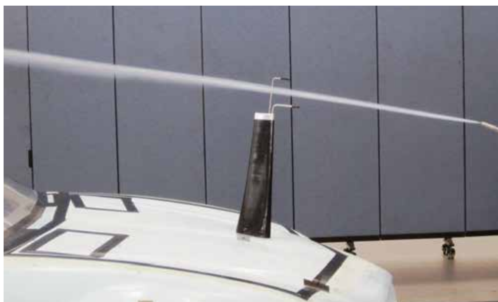
Figure 5: Final mounting position of the Pitot foil with smoke verification of the flow angle
