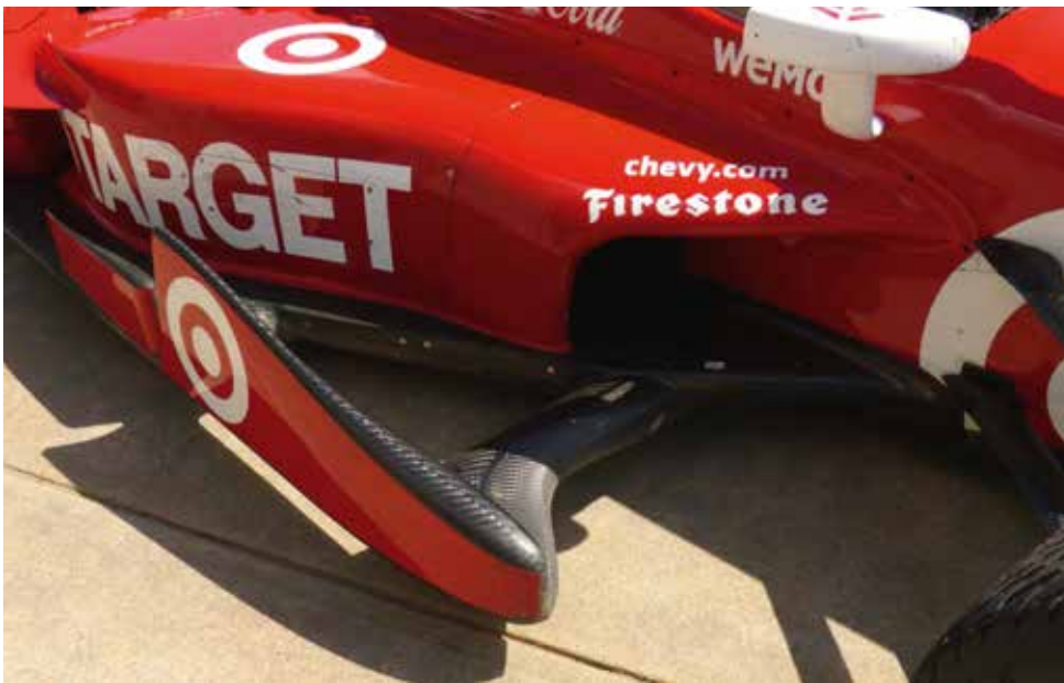
In a bid to improve stability should the nose rise, IndyCar worked with HPD and the solution was an underwing, and a cut out in the floor ahead of the sidepod. Initial instability was a concern, but teams worked on aero balance
