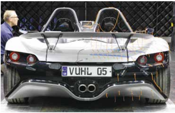
Picture 5: Twin short rear diffusers at the termination of the flat floor
