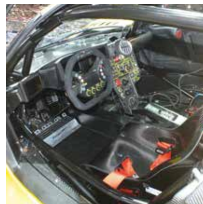
The SCG 003 promises to be a torque monster. Drive to the rear wheels is governed by a Hewland sequential transmission with paddle shift
