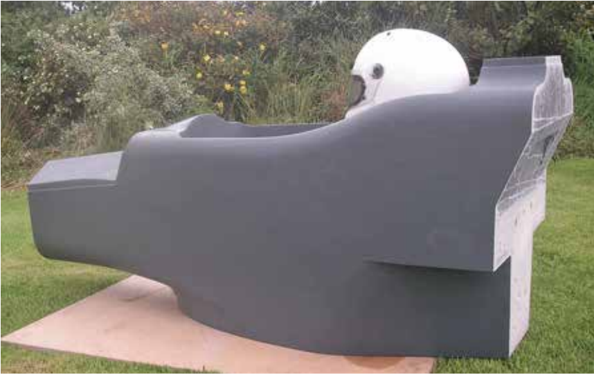
Picture 5: Chassis pattern made from epoxy tooling board and surface finished ready for mould manufacture
