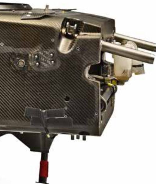
Picture 2: ‘Traditional’ twill weave carbon fabric can be seen in the wing elements of the Empire Wraith, with ‘trendy’ spread tow fabric featuring in the diffuser
