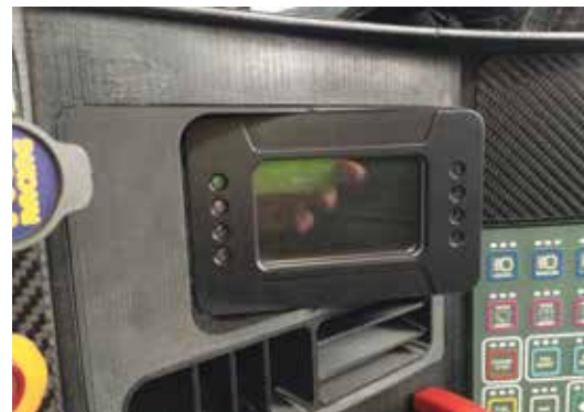
3D printed parts not only accelerated the manufacturing process but also improved reliability – during testing the parts successfully completed the equivalent mileage of two 24 hour Le Mans events
