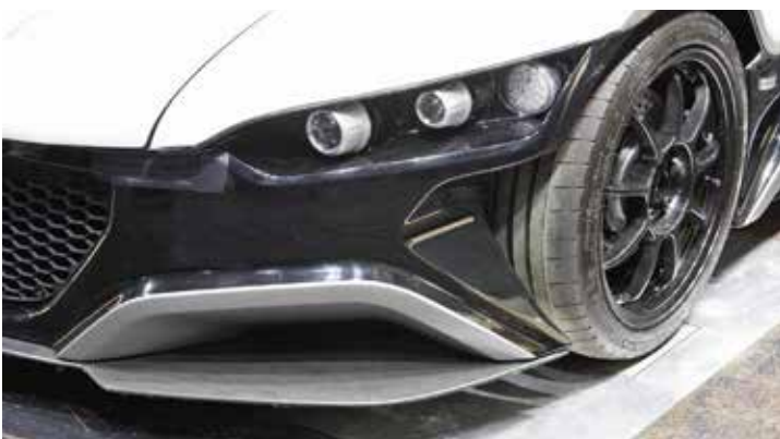
Picture 3: Front splitter and cutaway airdam in front of the front wheels
