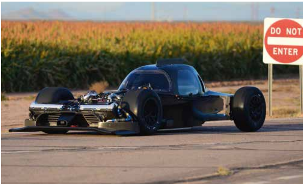
Top: The bottom half of carbon fibre tub has a distinct V shape to increase the volume of air passing through the car Above: The GT-R LM Nismo's engine is based on Cosworth's unraced direct injection 1.6-litre unit originally designed for F1
