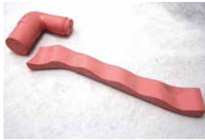
Picture 7: 'Aquacore' is a thermally stable, water soluble tooling medium
