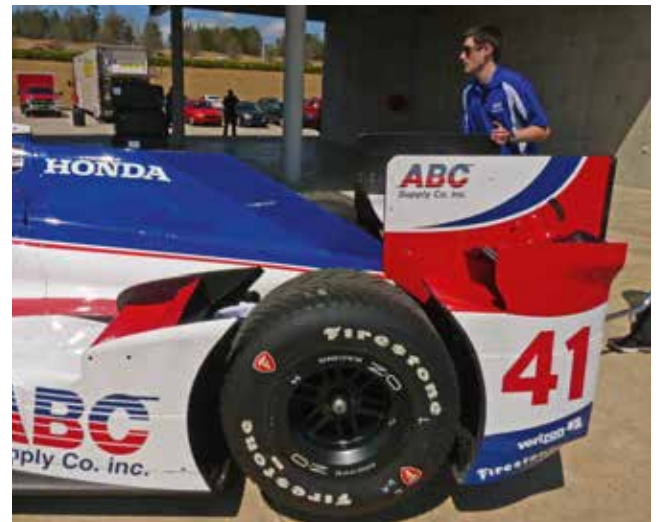
Chevrolet (left) went for cut openings in the rear wing in the example seen at the Barber Motorsport Park test in March, and a coke bottle shape around the radiator. Honda’s solution (right) shows a closed rear wing but the kit features more adjustable features than Chevrolet’s. It remains to be seen whether or not this will be an advantage.
