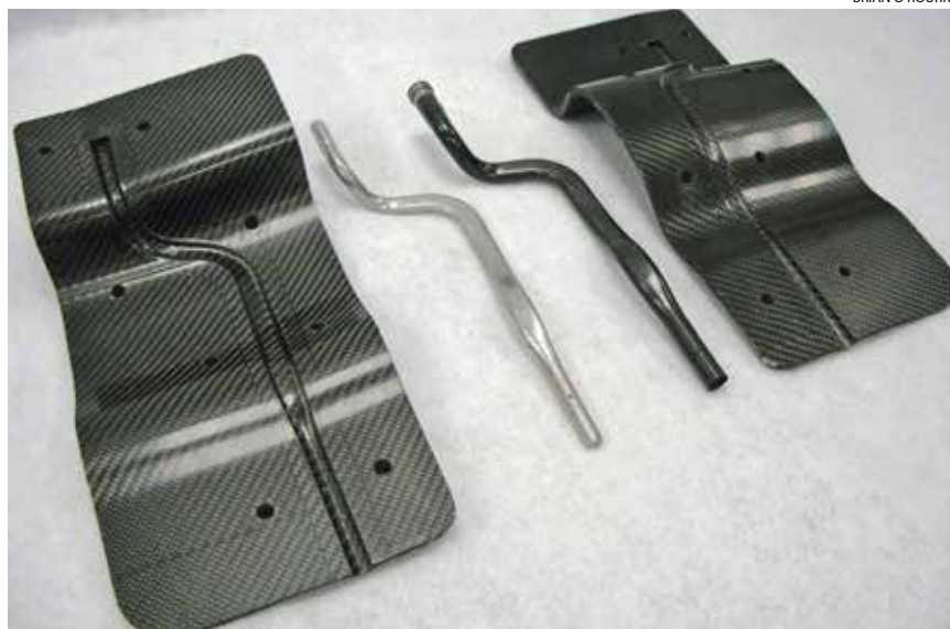
Picture 8: This small carbon pipe was made using carbon epoxy for the exterior tooling and a low-melting point alloy for the internal tooling
