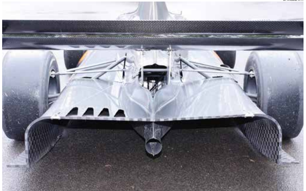
Picture 2: ‘Traditional’ twill weave carbon fabric can be seen in the wing elements of the Empire Wraith, with ‘trendy’ spread tow fabric featuring in the diffuser
