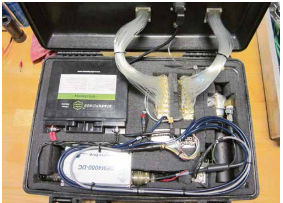
Figure 2: Scanivalve system in its enclosure
