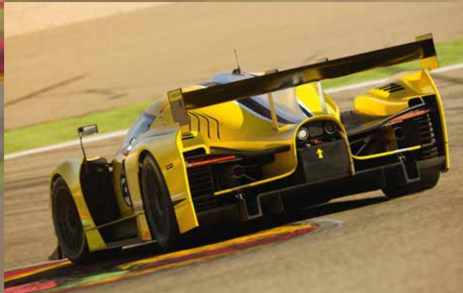
Glickenhaus says the SCG 003 will weigh 1350kg with a 49:51 weight distribution. it will be built around SCG's own carbon fibre monocoque
