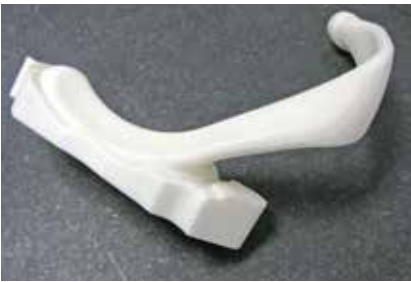
Picture 6: Additive Digital Manufacturing (ADM) is now used in many intricate tooling applications in F1. This one is soluble in high pH (alkaline) liquid
