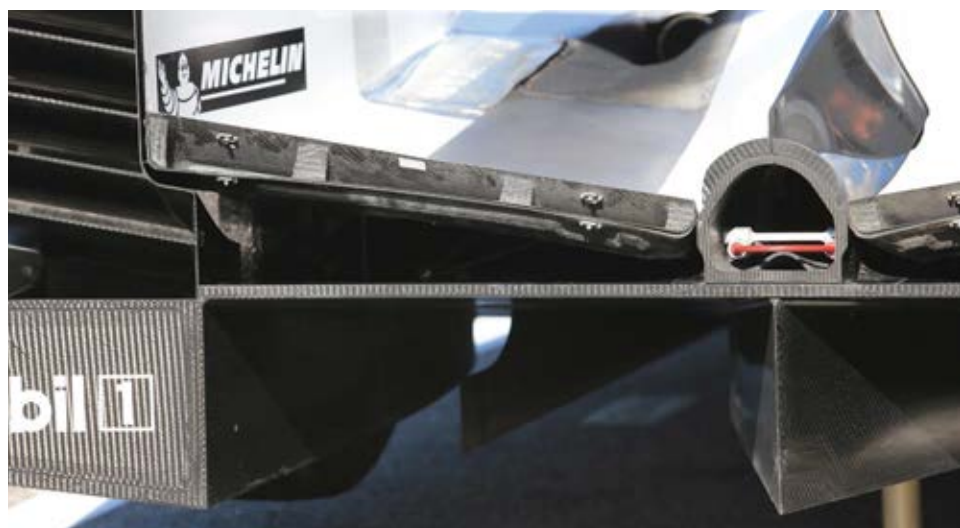
Porsche has tidied up the bodywork at the rear of the car. The underfloor features interesting aerodynamic devices that have helped to improve the airflow and make the car less peaky and easier to drive
