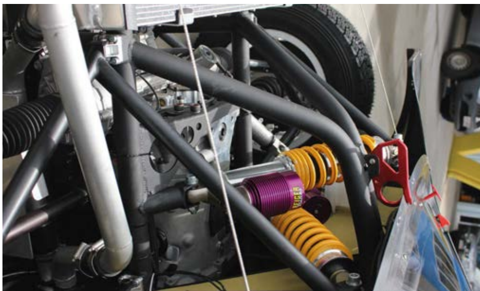
The suspension layout has been designed without pushrods – there’s no anti-dive or anti-squat front or rear
