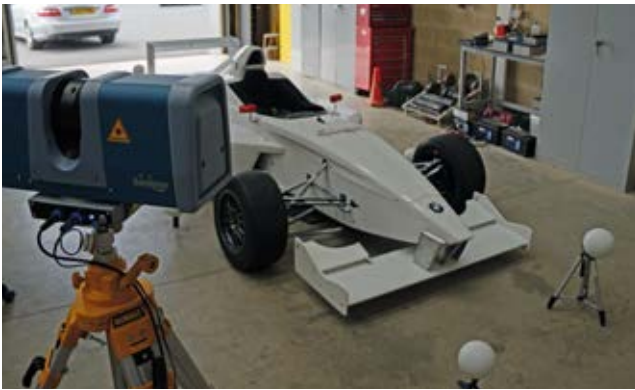
The scanner is mounted on a tripod so that each scan is 'global' – this improves accuracy when the multiple scans are brought together, rather than focusing on a small area
