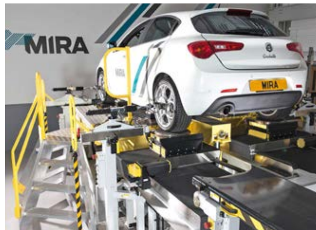
Chassis clamps fore and aft of the front and rear wheels, dynamic arms attached to the wheel hubs, and x-y tables under the tyres interface with the vehicle
