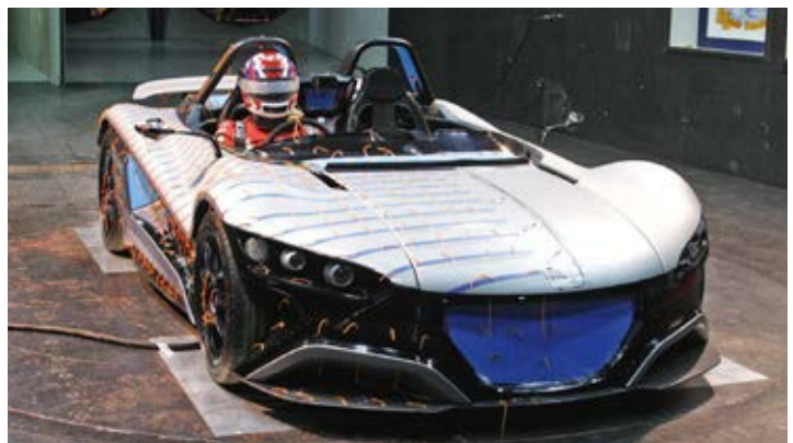
Picture 2: Inlets at the front, side, in the centre next to the driver and underneath at the rear were covered over (in blue for clarity)
