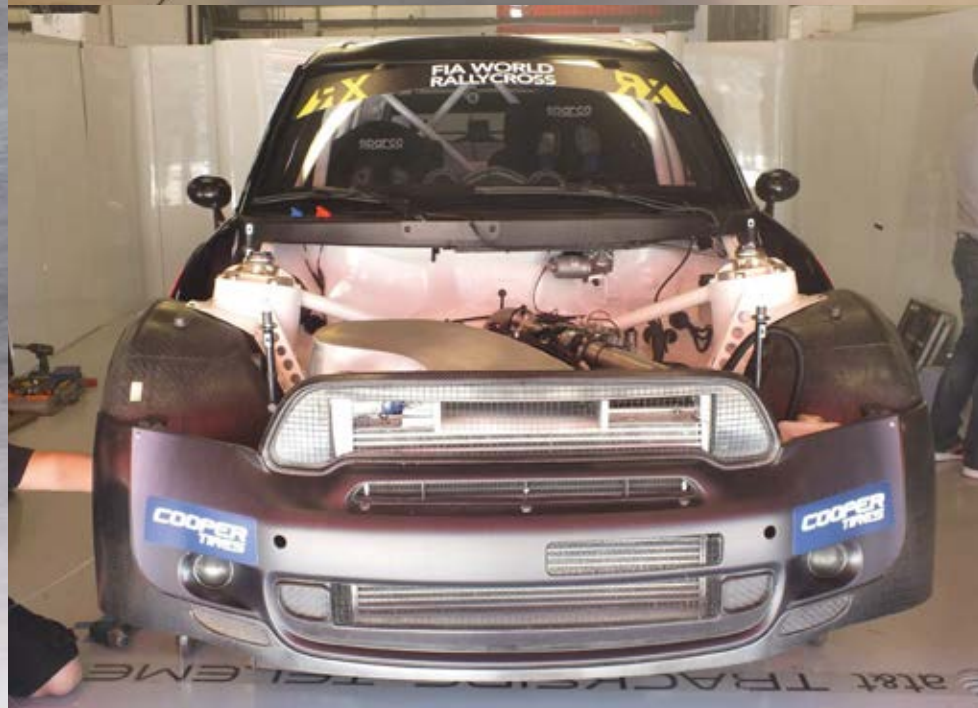
Top: The cooling fans can clearly be seen – these play a huge role in keeping performance consistent Above: Fans push air through the radiator and are constantly running for optimum results
