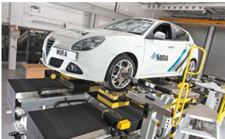
Chassis clamps fore and aft of the front and rear wheels, dynamic arms attached to the wheel hubs, and x-y tables under the tyres interface with the vehicle
