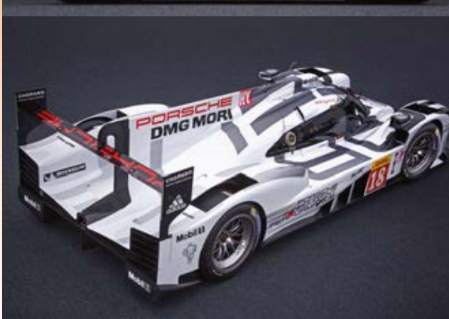
The two-litre V4 engine powers the rear axle with over 500bhp. When the driver recalls the stored energy from the battery, an extra 400bhp drives the front axle
