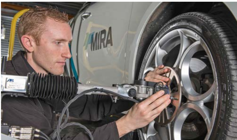
Fixing one of the dynamic arms to the wheel hub
