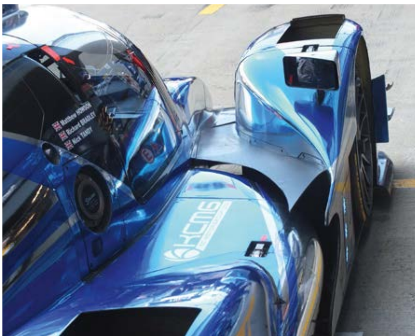
The ORECA 05 flies in the face of LMP2 convention and is 100mm narrower than the maximum width allowed
