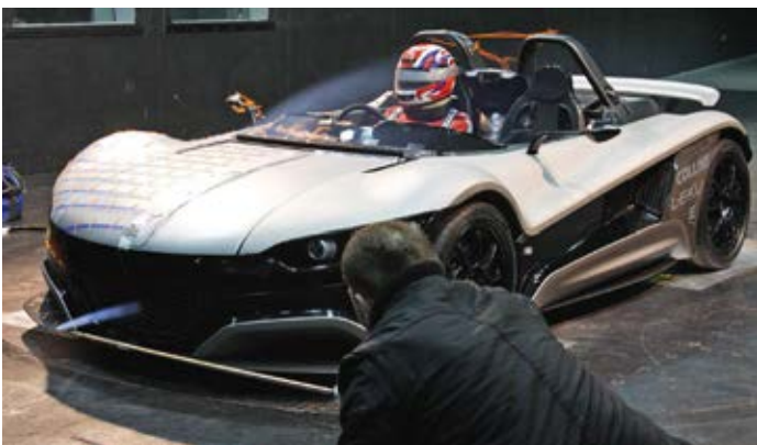
Picture 1: Cooling flows were examined on the VUHL 05 open two-seater sports car
