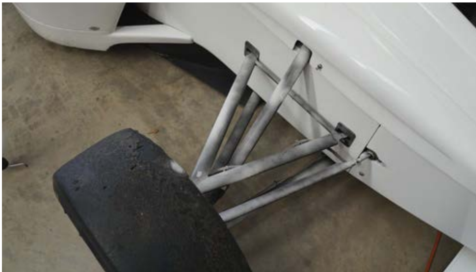
The black and shiny suspension arms need to be covered in a white chalk based powder spray to make the surface appear matt to ensure that the whole component can be seen by the scanner
