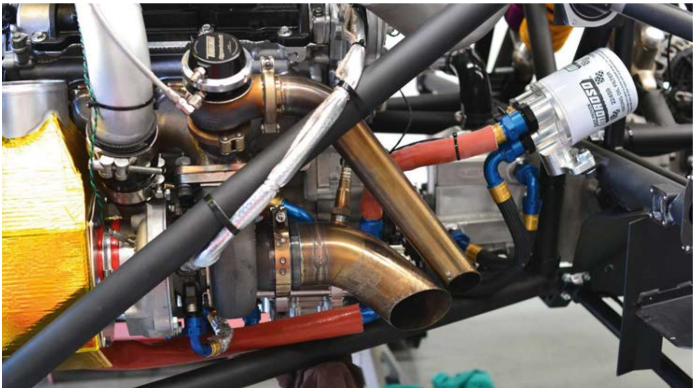
The exhaust exits blow directly into the diffuser tunnels in an attempt to further boost downforce
