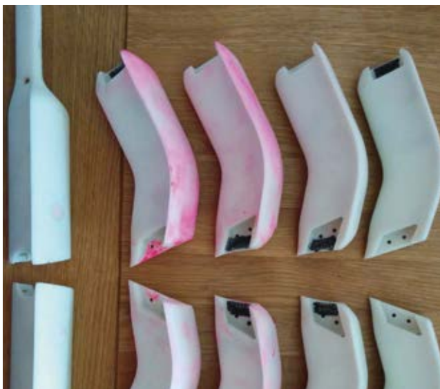
The rear wishbone from Marussia's MR03 uses a 'mushroom' suspension blocker
