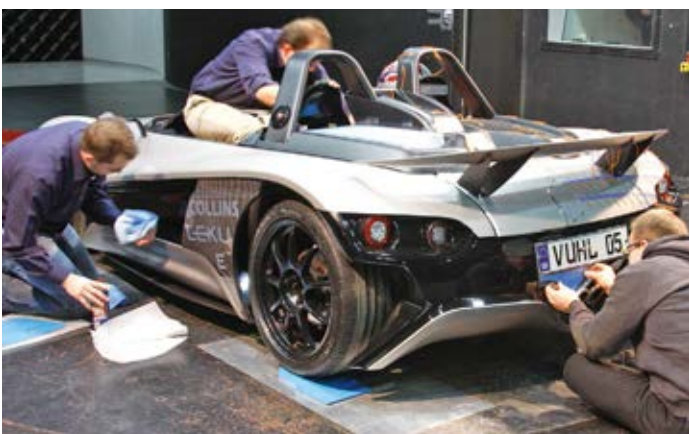
Picture 3: Outlets on the rear deck and in the rear panel were also covered over
