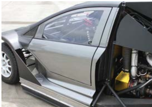
The 120mm rubber skirts run along the car's entire length and are an integral element of the aero package
