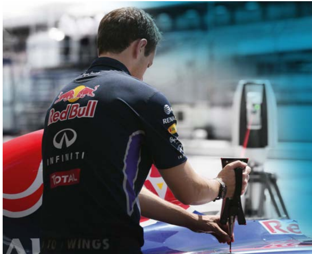
Measuring the engine cover using a Leica Absolute Tracker AT960
