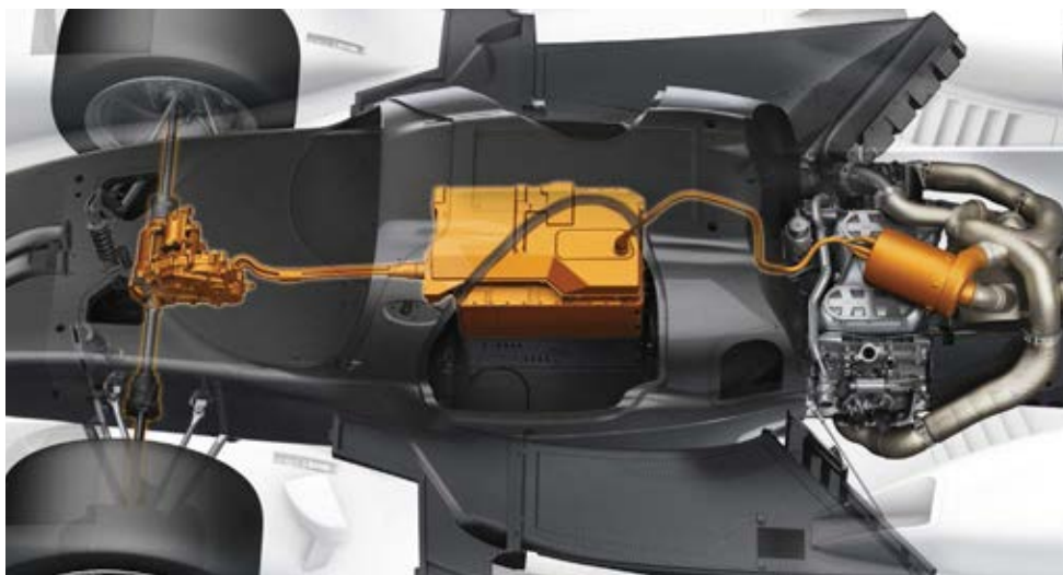
The battery system on the Porsche 919 uses cells developed by A123 Systems, who also supply a number of F1 teams
