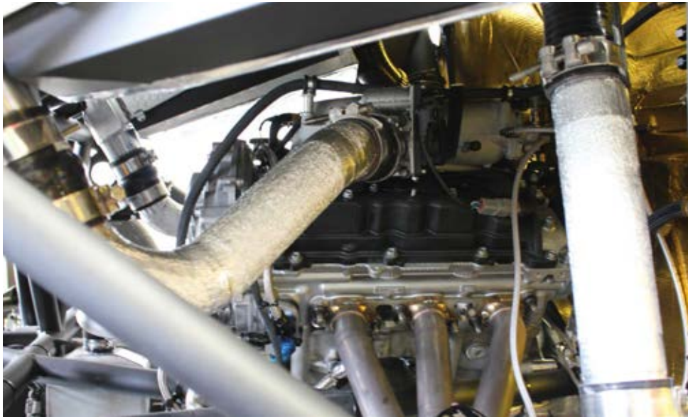
The amount of plumbing associated with the turbo, and the amount of heat the unit generates, left Cepnich surprised
