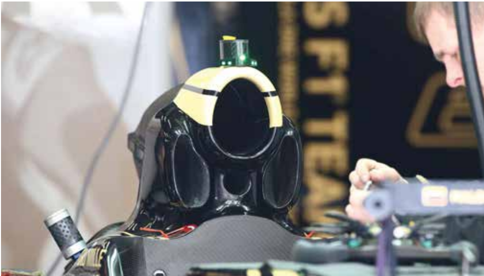
The E23's distinctive roll hoop inlets certainly catch the eye – the usual airbox intake is flanked by two additional inlets
