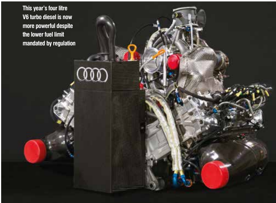
The carbon fibre gearbox dates back to 2013 but has been re-worked for 2015
