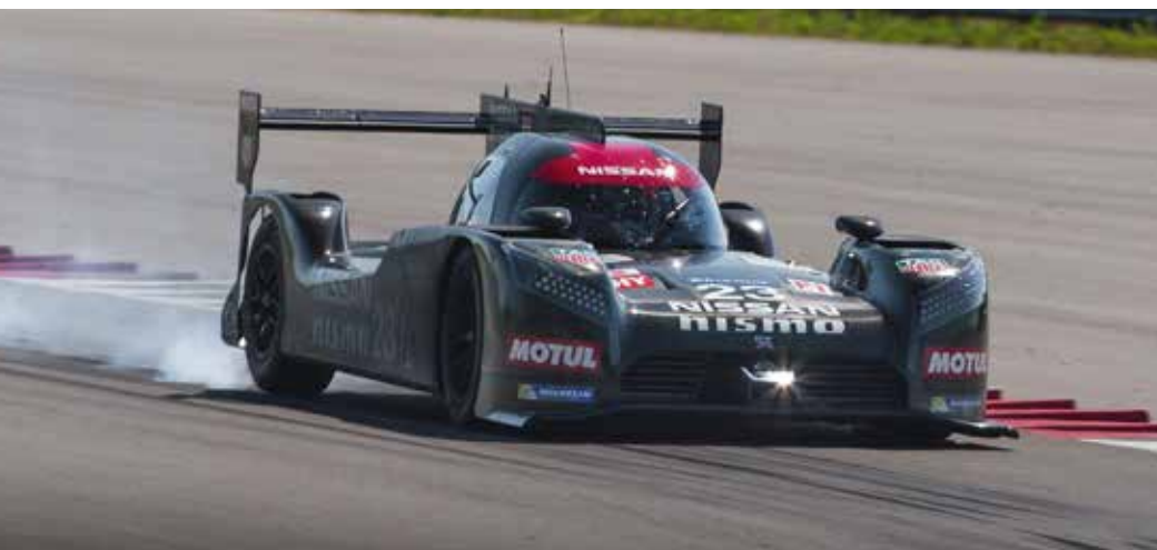
Being front wheel drive, the GT-R LM NISMO runs bigger tyres up front – 14 inch wide Michelins versus nine inch rears
