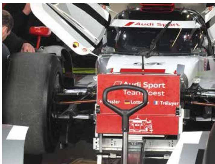
The front end of the R18 has been re-done this year, requiring a new crash test for the car. Front suspension is pushrod, also pictured here are the ERS driveshafts
