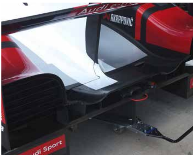
The rear of the R18 shows the impact of the rule change that stipulates that the engine cover and diffuser gap covers the crash structure
