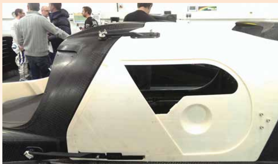
Above: The fully functional door constructed from the 3D printing processes
