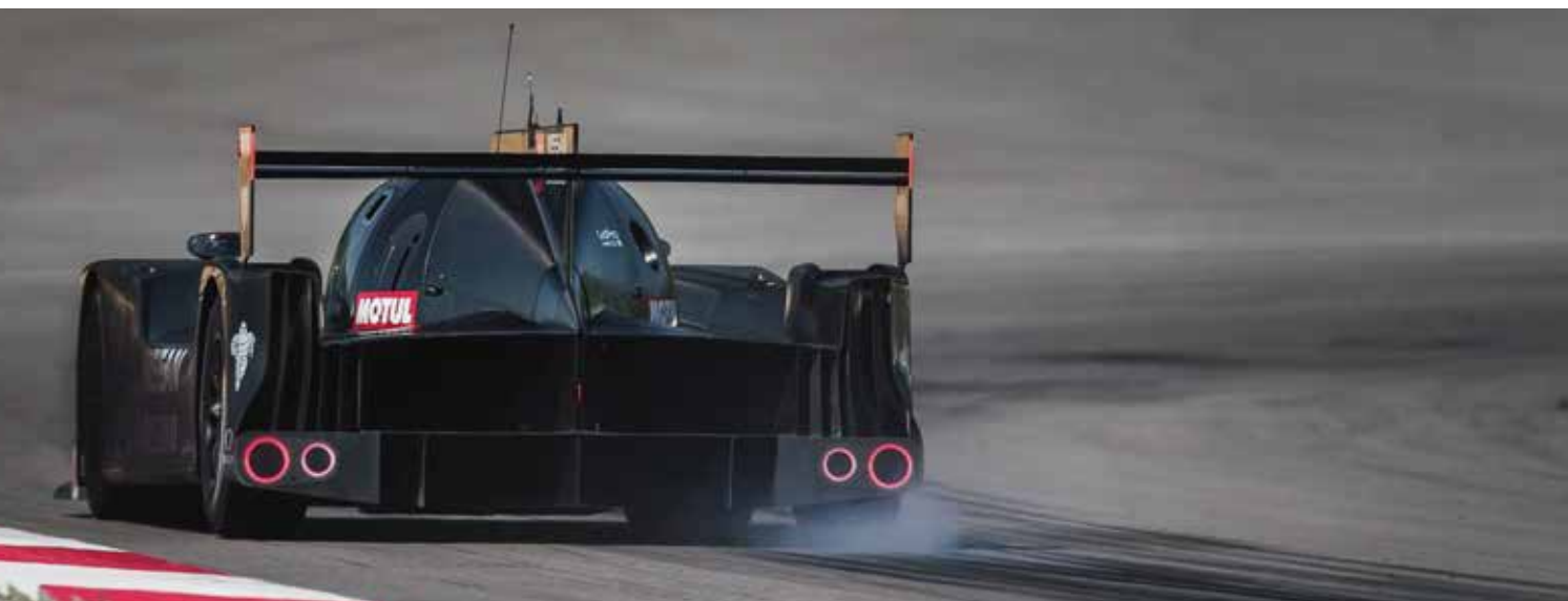
Lifting the inside rear has meant that the team has to watch out for flat-spotting the tyres. It's an unusual phenomenon in an unusual design concept
