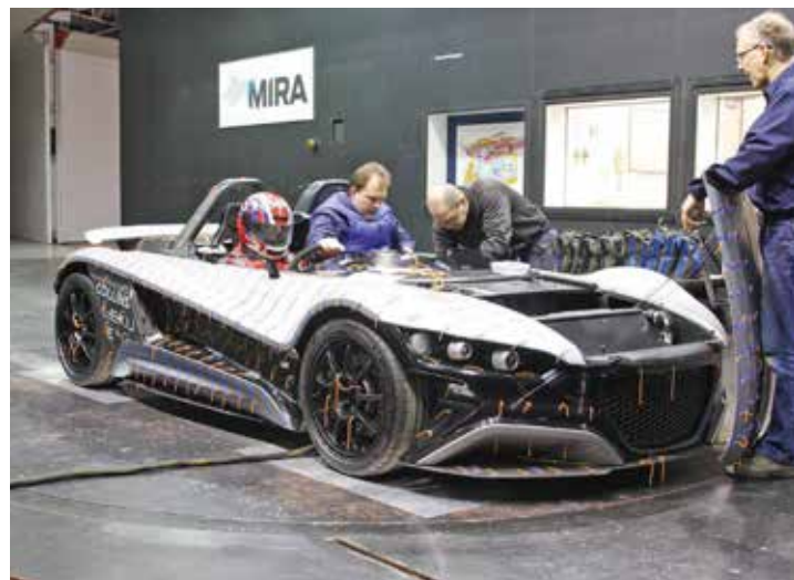
Picture 1: This month the VUHL 05 front end is modified, and surface pressures are measured via the loom of capillary tubing seen emerging from under the car
