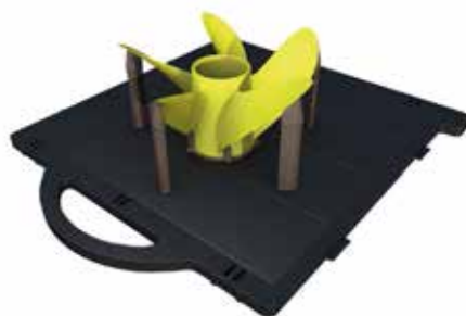
An example part showing the support material
