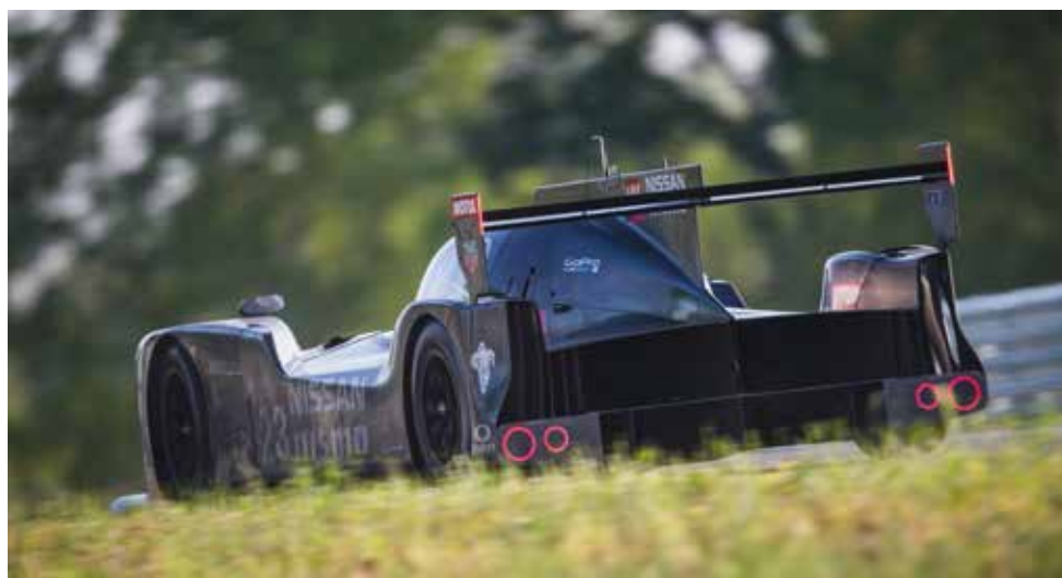
Nissan's GT-R LM NISMO features a weight distribution of at least 65 per cent front, and 35 per cent rear
