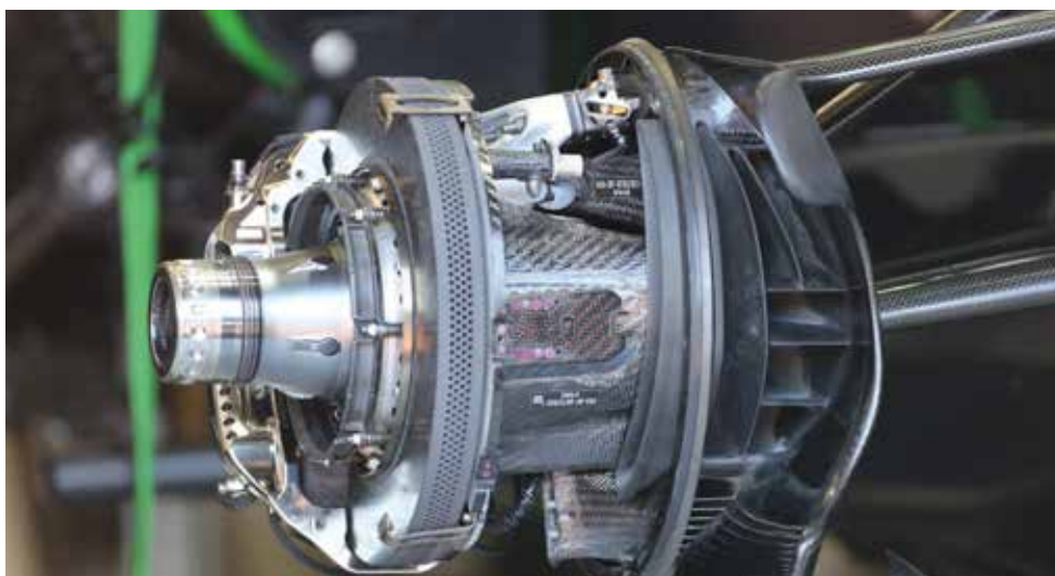
Front brake. McLaren is the only team on F1 grid to use Akebono callipers. Front axle is hollow to influence flow structures
