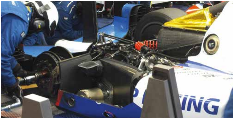
The Nissan 4.5-litre VKE-45 V8 sits in a monocoque of aluminium honeycomb with carbon fibre skins, built by ARS Tech
