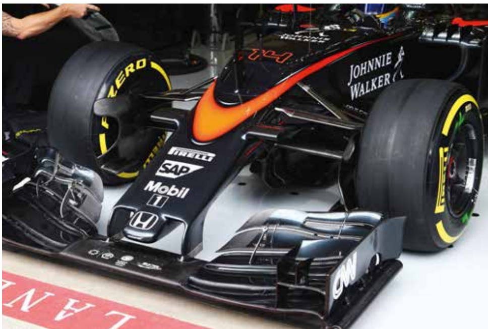
Changes in chassis regulations to banish ugly noses caused McLaren some packaging issues. Original Nose was long and wide and protruded from leading edge of front wing, but the team introduced this all-new nose for the Austrian Grand Prix
