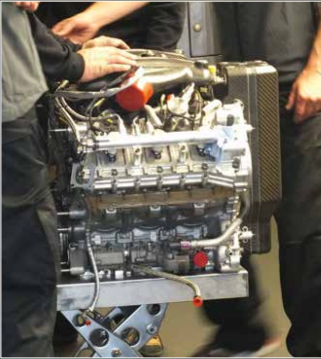
Main picture: The AER-engined Rebellion went well at Le Mans, winning LMP1 privateer class Left: Installing AER's turbocharged lump was the obvious solution once Toyota engine became unavailable at the end of 2014, but adapting it was not the work of a moment Above: Meeting the cooling demands of the new engine while not compromising the aero was a major challenge for the design team while the turbocharged engine also required a bigger inlet
