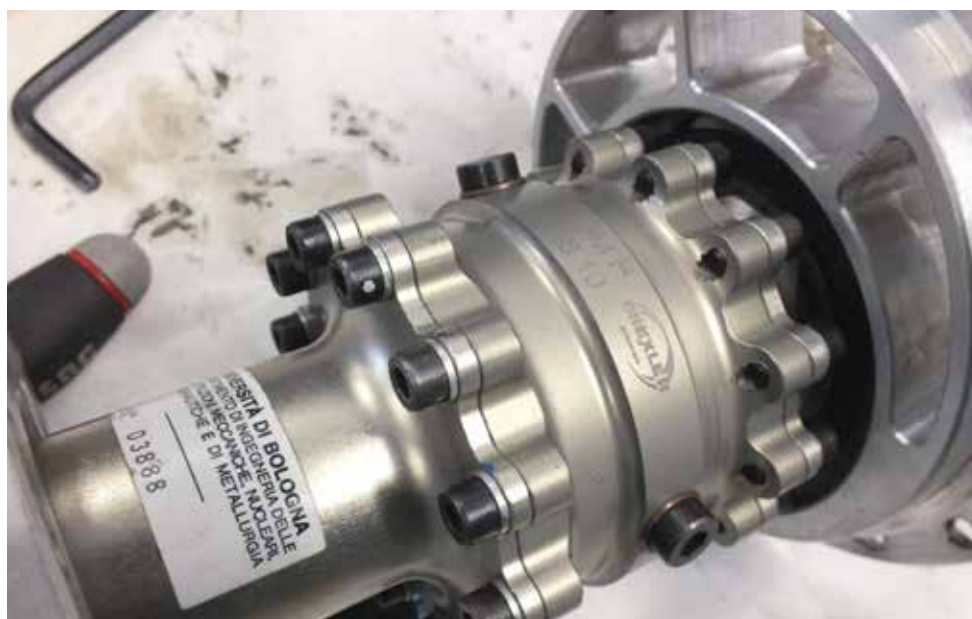
Drexler manufactures a clutch pack differential that comes preloaded; Charlotte FSAE team reduced preload by half
