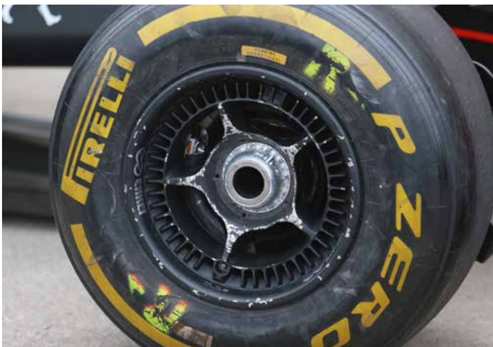
McLaren is one of a number of teams to do a lot of work on front wheel design in order to optimise flow around front of car
