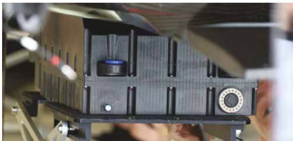
Above: The battery pack on the McLaren, with FIA seals, temperature strips and high-power connectors. This unit is mounted at the base of the MP4-30 chassis
