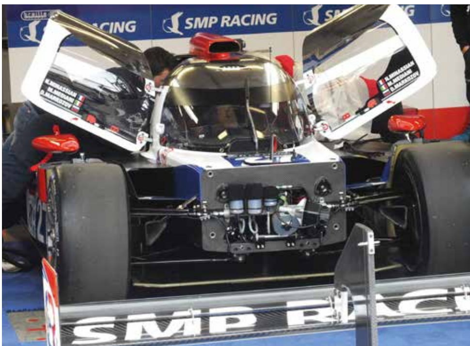
Car has been designed to lower the roof as much as possible within limits of the LMP2 regs with a steep, short windscreen
