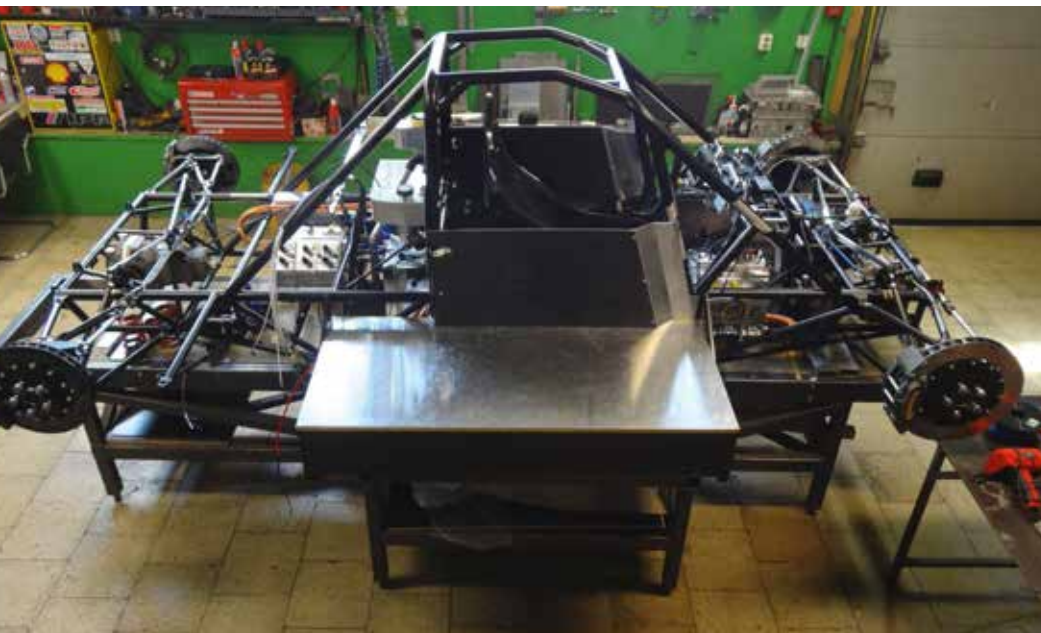
The battery packs sit either side of the driver between the front and rear wheels, saddlebag style, in these hermetically sealed and electrically isolated aluminium containers. The battery pack is capable of full discharge in eight minutes
