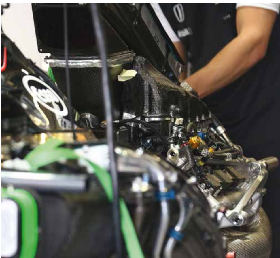
At the start of the 2015 season the RA615H featured a machined aluminium plenum, unique in Formula 1, but this was simply for reliability purposes and Honda has now reverted back to this composite plenum, as included in original design
