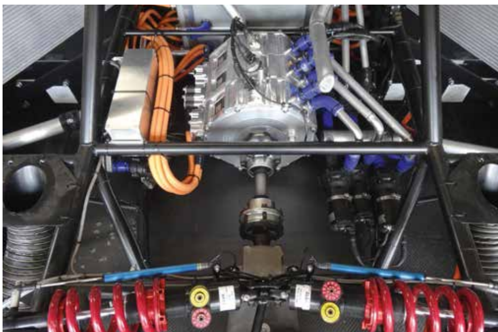
All four wheels are driven by six electric motors, the off-the-shelf YASA-400s triple-stacked in the car at the front and rear axles. The output from the motors is fed to the BBS wheels and R18 Hankook tyres via Sadev SP03 limited-slip differential
