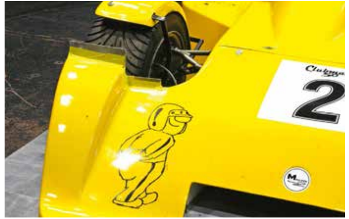
The inner and outer nose Gurneys on the Mk 18B, with the inner at 'low' height
