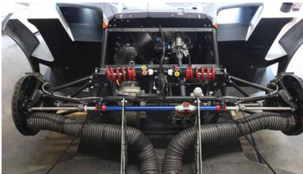
The suspension is double wishbone with pull-rods all-round. At the sharp end the eO PP03 features Sachs dampers, Eibach springs and electrically-assisted Woodward rack and pinion steering. Brakes are by AP Racing with vented steel discs
