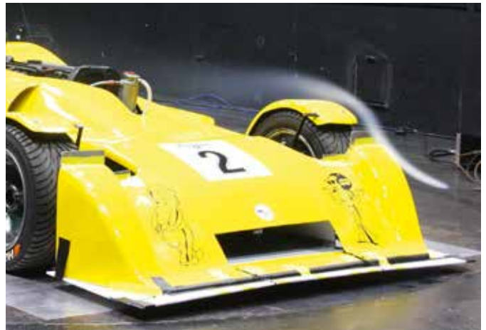
Outer nose Gurneys modified the flow over the front of the Mallock's 'mudguards'
