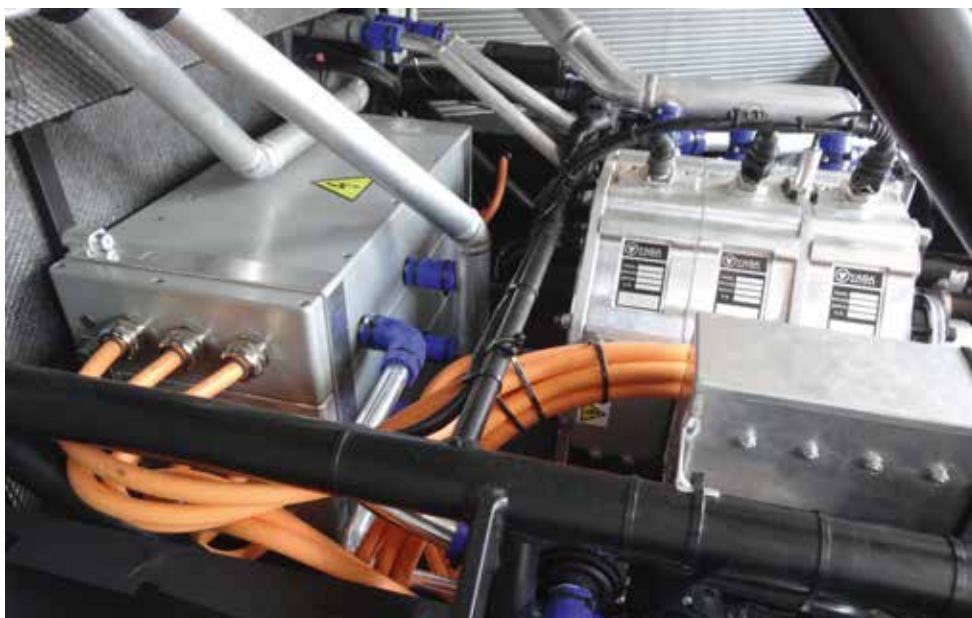
Cooling is a major concern and the Drive eO PP03 requires a flow rate of dielectric fluid of some 15 litres per second for each of its six electric motors. The tube-frame chassis is quite straightforward, and has been designed and built in Latvia
