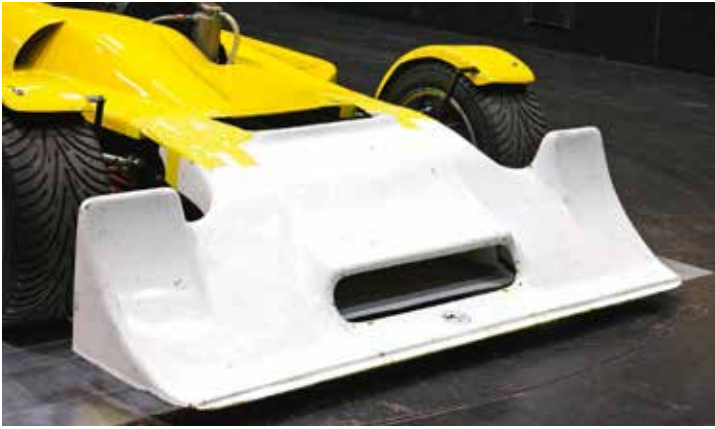
The Mk 18B sporting its high downforce nose with its sharp concave cross section
