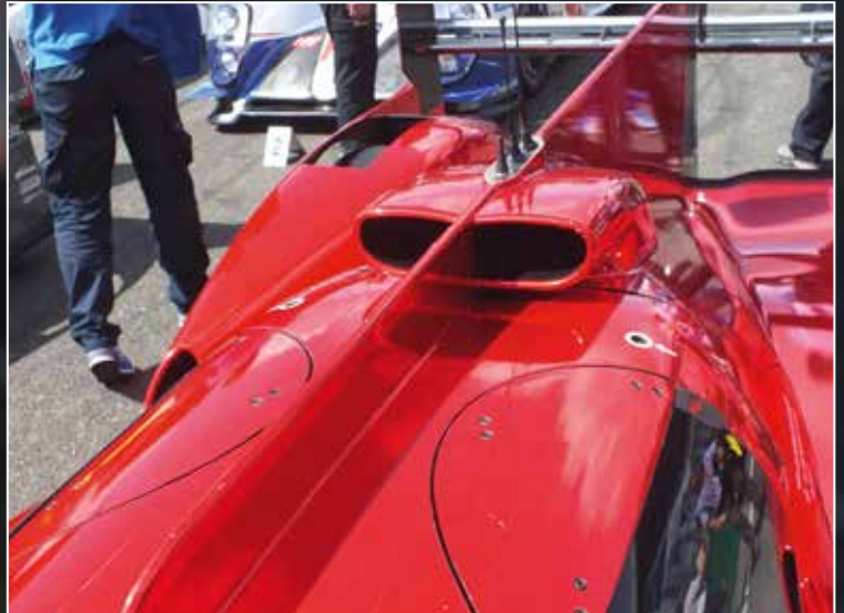
Main picture: The AER-engined Rebellion went well at Le Mans, winning LMP1 privateer class Left: Installing AER's turbocharged lump was the obvious solution once Toyota engine became unavailable at the end of 2014, but adapting it was not the work of a moment Above: Meeting the cooling demands of the new engine while not compromising the aero was a major challenge for the design team while the turbocharged engine also required a bigger inlet
