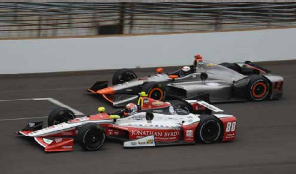
Chevrolet says that its original engine cover caused more of a yaw moment, adding front downforce, which in turn unloaded the tail and caused car to pivot into a faster spin, bringing the back around at very high speed
