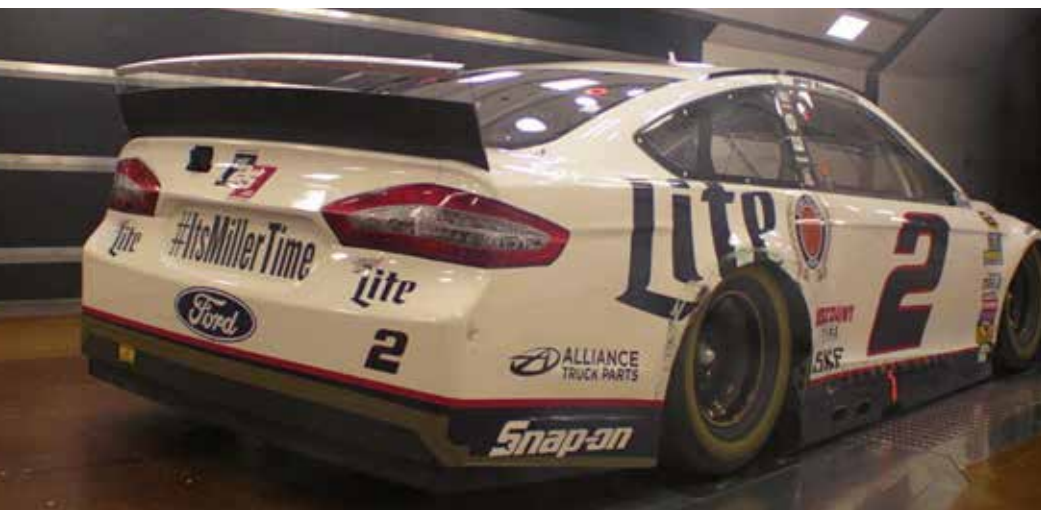
The Penske No.2 NASCAR Sprint Cup entry sporting the Indianapolis spec high drag package in the Aerodyn wind tunnel
