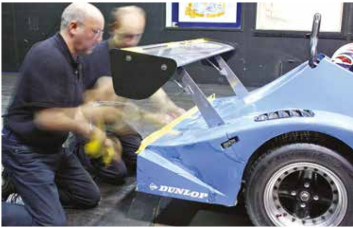
Rapid adjustments to the rear wing of the Mk 28/36 and the fitting of a 20mm-high Gurney to the trailing edge of the body balanced the 'current' spec Clubmans racer
