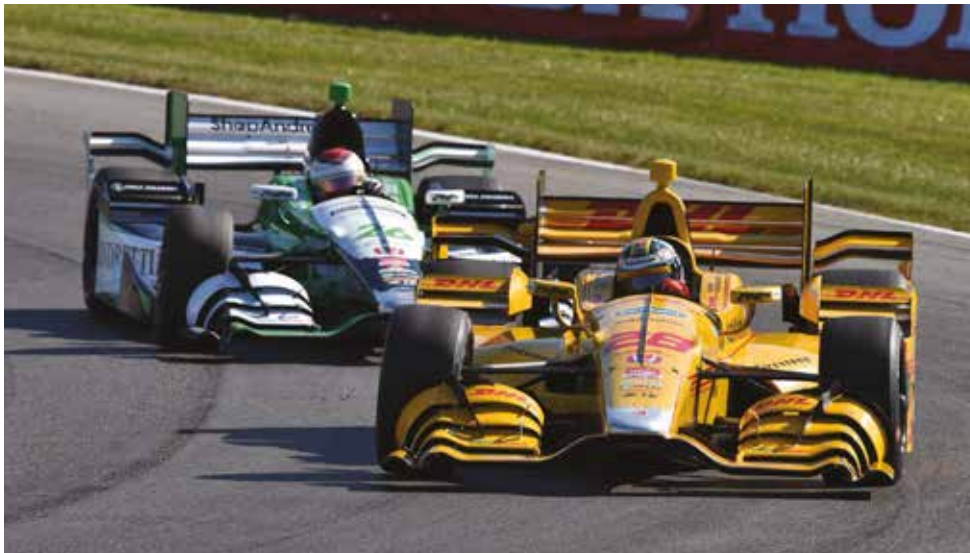
Honda road kit minus the front wing endplates. Honda believes it has been at a disadvantage this year and is looking to make improvements in more than the three stipulated modification boxes, and is especially keen to develop the front wing
