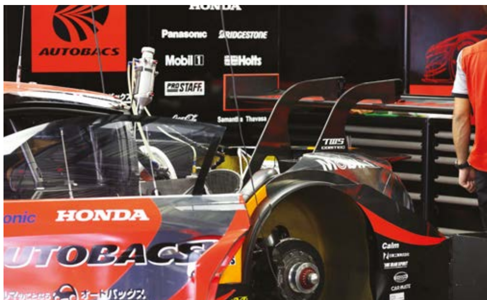
The rear wing on the Honda NSX is a spec part and is identical to that used in the DTM in 2013, although the Super GT cars do not use any form of DRS. At the sharp end the front spoiler is also a spec part, as is the car's underfloor and the diffuser
