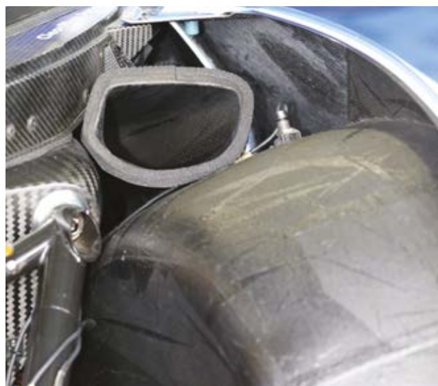
The monocoque of the Super GT Honda NSX had to be reshaped to avoid a clash with the steered front wheels – but as can be seen here it is still a very tight fit
