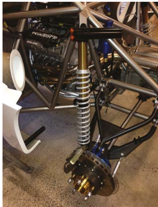
Kelsey is a great believer in plenty of suspension travel, a design philosophy he picked up on a visit to California to watch the Baja 1000. The brake system is from a stillborn Subaru World Rally car project
