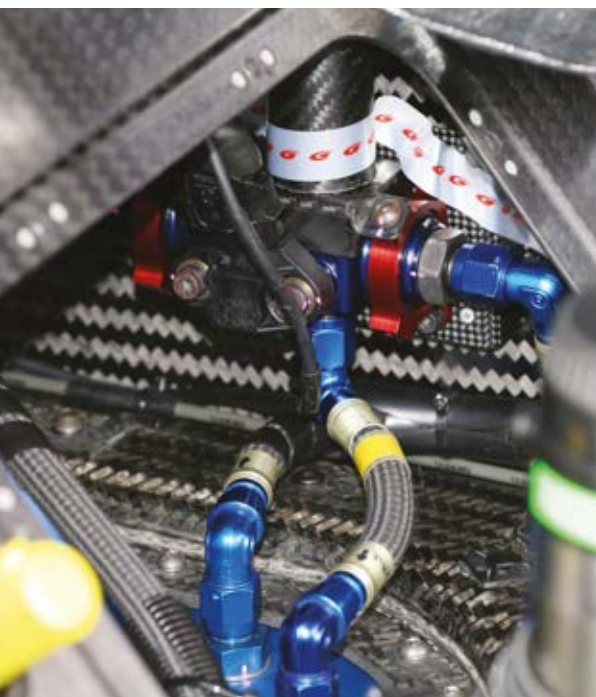
GT500 uses a Toyota-designed fuel flow restrictor which limits flow to 100kg/h. Super GT racecars are required to run on pump fuel
