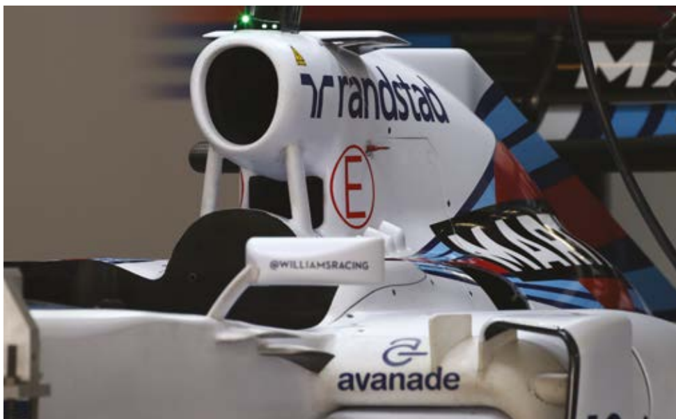
As with much of the car, the FW37's roll hoop concept is largely a carry over from the FW36, although the twin forward-support design dates back to the FW35 despite the change from Renault V8 to Mercedes V6 that has taken place since
