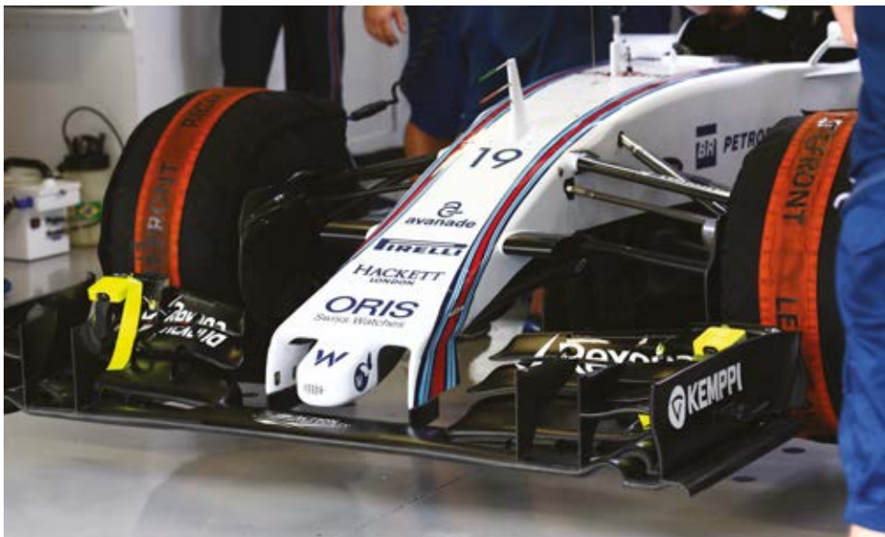
Williams opted for a so-called 'short nose' for the FW37, where the leading edge of the nose structure sits very close to the trailing edge of the centre section of the front wing; this resulted in a small shift of the aero balance to the rear of the car
