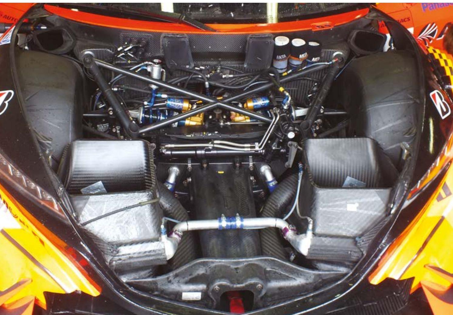
Under the front bodywork of the NSX; showing the front impact structure, suspension, front subframe and the location of the front water coolers. But no engine, as that's in the middle
