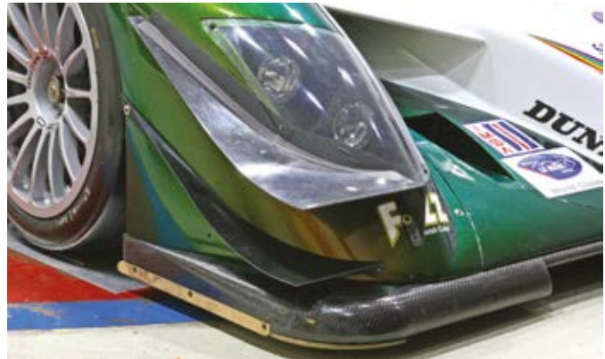
The Radical SR10 LMP1 racecar, as featured in Aerobytes back in 2008, had steeper dive planes and responded differently when an upper pair was added
