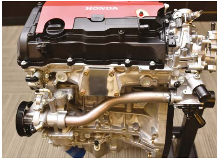
US Formula 4 will be powered by the Honda K20 C1 2.0-litre engine which will give around 160bhp, the maximum power mandated by the FIA. Crawford has previously worked with Honda with its Formula Lites car
