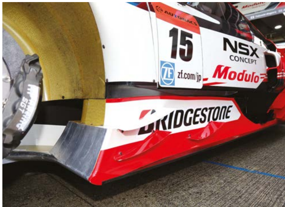
There's a free area for turning vanes and other devices on the side of the GT500 cars, in common with DTM. The DTM cars actually produce more downforce, but Japanese cousins have more grip thanks to free tyres
