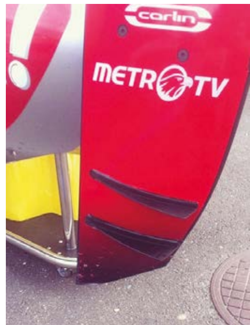
Carlin and Prema Powerteam arrived at the Red Bull Ring round with what might be best described as a pair of diveplanes on the lower reaches of their barge boards. Carlin says they do little other than providing a small improvement in balance
