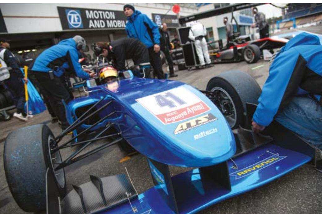
The bodywork along the top of the F24 appears rather boxy but this is part of a ‘keep it simple’ approach, the team says. ArtLine is planning on linking up with a Russian composite manufacturer to make its own monocoque and body parts
