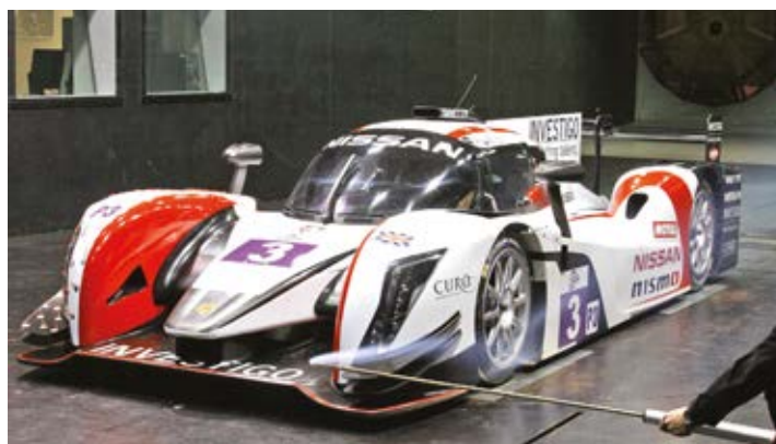
Here the smoke in the dive plane wake can be seen outboard of the upper wheel arch
