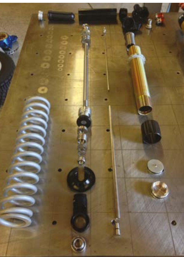
Because of the costs involved with high-end rally shocks Kelsey decided to design and build his own dampers. To protect the IP in the shocks he made sure parts were machined by different companies while also making some bits himself on his lathe
