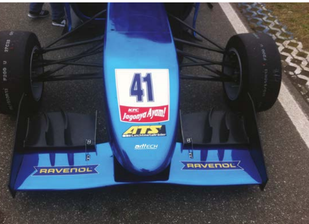
The ArtTech F24 F3 car has a distinctly stubby nose, below which two vertical flaps on the front wing direct air under the floor to the diffuser. The team behind the new car was keen to stress that it is still in the early stages of its development
