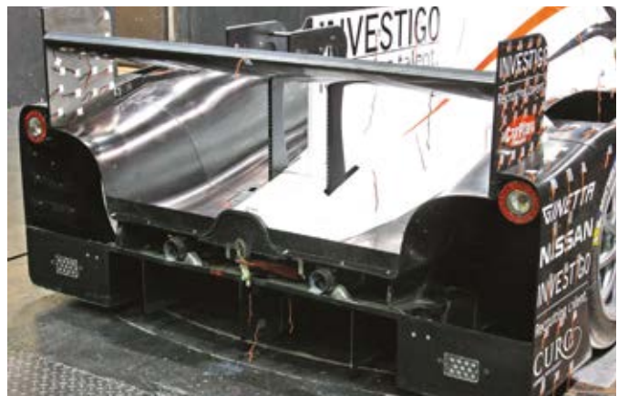
Removing the elements inside rear wheel arch rear openings – to study the impact of an incoming regulation change – had a small yet doubly surprising effect
