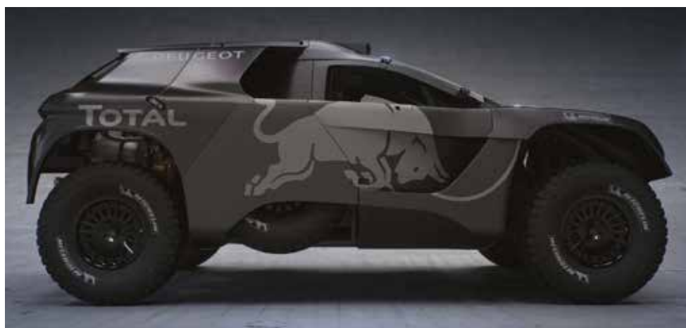
Front and rear overhangs were reduced even further but the main difference between the DKR16 and its predecessor is that it is wider and longer with a lower centre of gravity. The roof-mounted air-intake has been the subject of aero development
