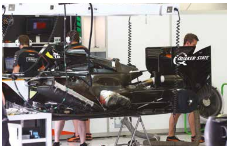
The back end of the car stripped down to its bones with heat shields and some underbody parts remaining in place. Also visible is the exhaust manifold and the left side main heat exchanger
