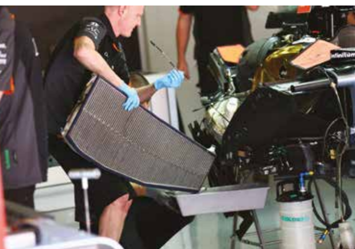
One of the changes on the B spec car was a new cooling system – as is the case with all modern Formula 1 cars the radiator is sculpted to fit tight sidepod space
