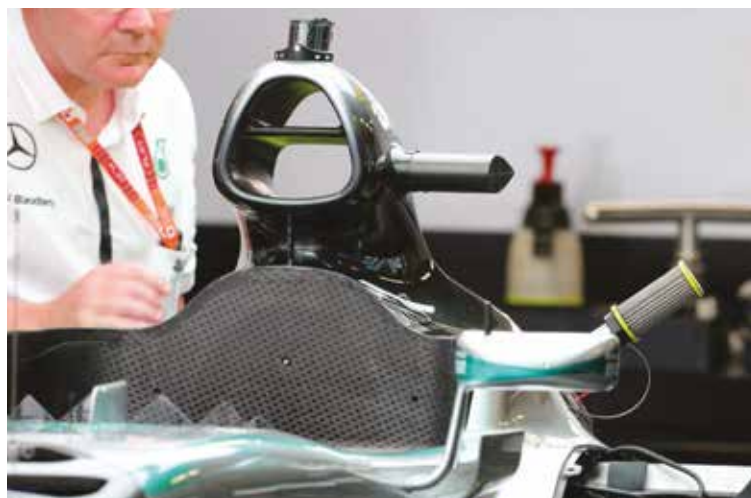
The twin forward roll hoop supports of last year's car have been replaced with an extremely thin single support under the centre of the roll hoop while the cooling duct is no longer there
