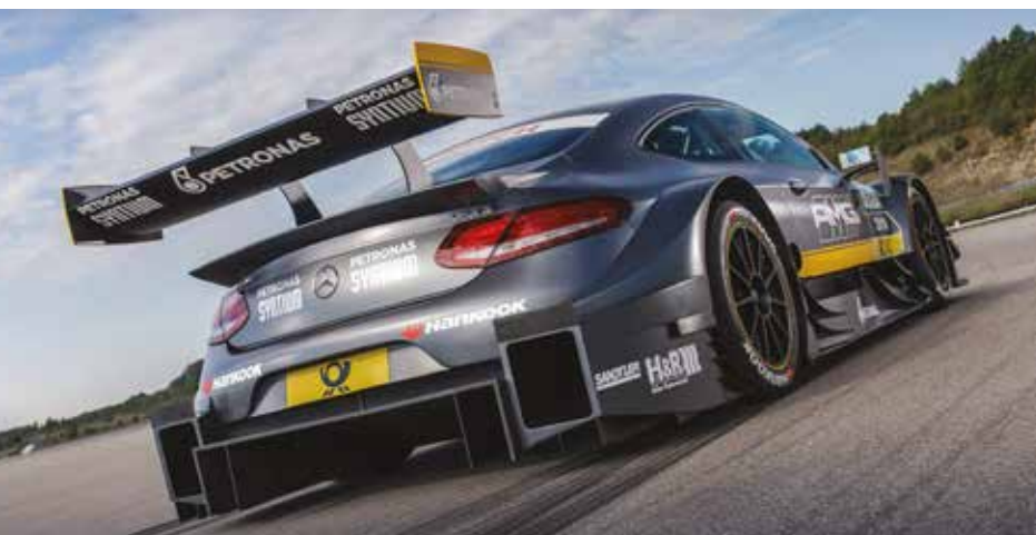
The new C63 has had a number of aero nips and tucks including a modified front and rear diffuser, while the DRS-fitted rear wing is basically a DTM controlled item which is also used by rivals Audi and BMW
