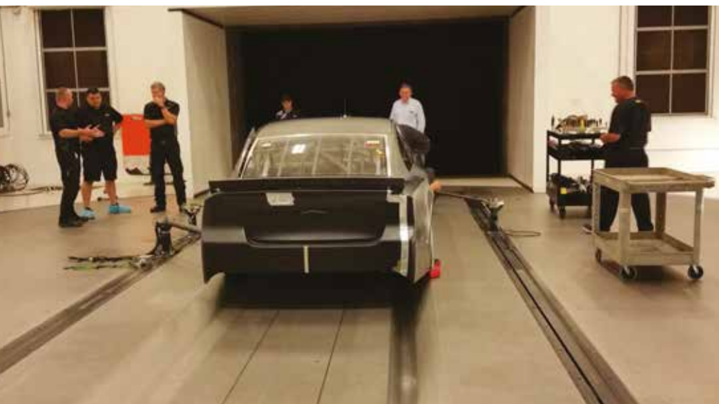
The symmetric spoiler and quarter panel. Lack of tail offset substantially decreases yaw moment and overall sideforce
