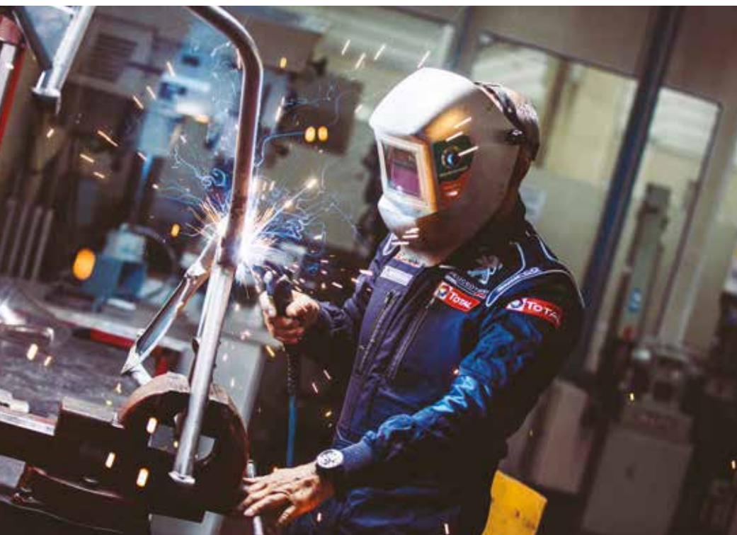
Modifying tubular chassis was a relatively simple affair as it is easier than working on carbon, but a redesign was required nonetheless. The car is also lighter than 2015 version as the team made use of lessons learnt to redesign some parts
