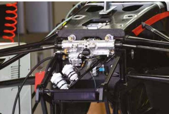
Front bulkhead showing steering rack and inboard suspension pickups. Unusually the torsion bars are mounted vertically on top of the chassis behind third element
