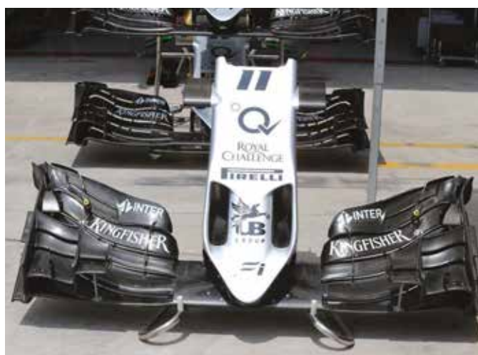
The VJM08B's striking nose: the vents are deemed legal as they are not see-through because of the fitting of a pair of spoon-shaped underbody panels inside the holes
