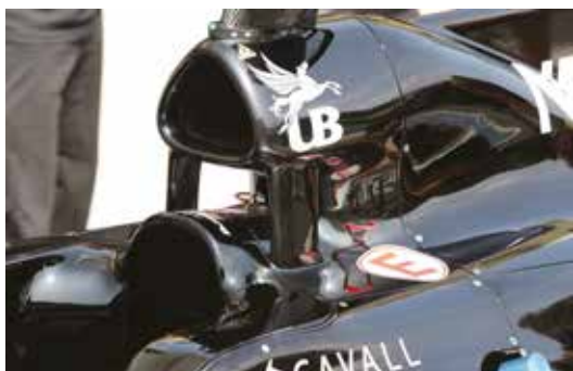
For its roll hoop the Force India VJM08B uses a twin forward support philosophy in common with many cars on the F1 grid
