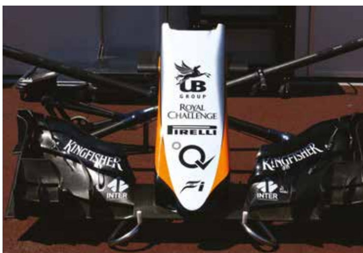
The more conventional nose with which Force India started the season. It had hoped to change to a short nose but the chassis architecture at the front prohibited this modification
