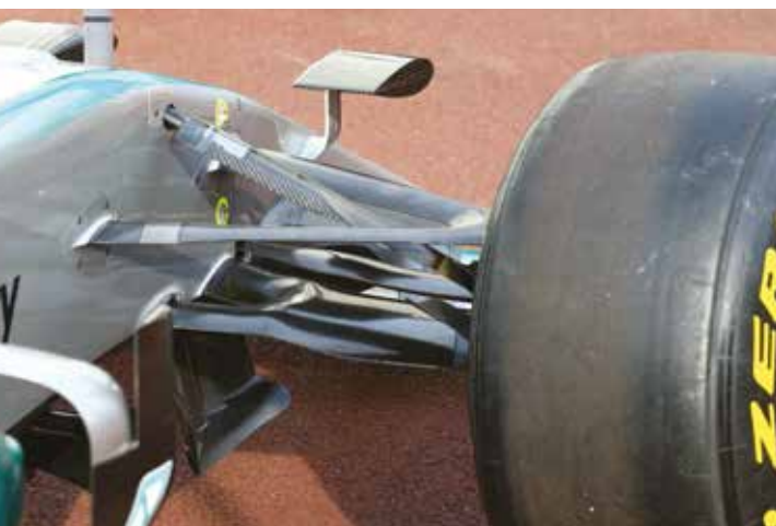
Front lower wishbone was a massive structural challenge as the team had to make it take the loads while delivering what the aerodynamicists demanded
