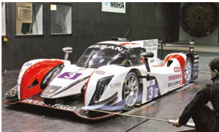
The car's dive planes affected its response to changes in yaw angle in some very interesting ways – the Ginetta was tested with and without the dive planes in place
