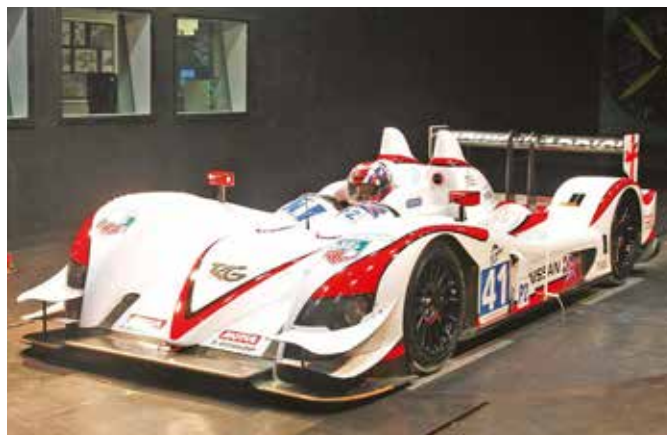
The Greaves Motorsport Zytek LMP2 had a broadly similar front end to the Ginetta (twin dive planes and similar front splitter) and responded like the LMP3 in yaw
