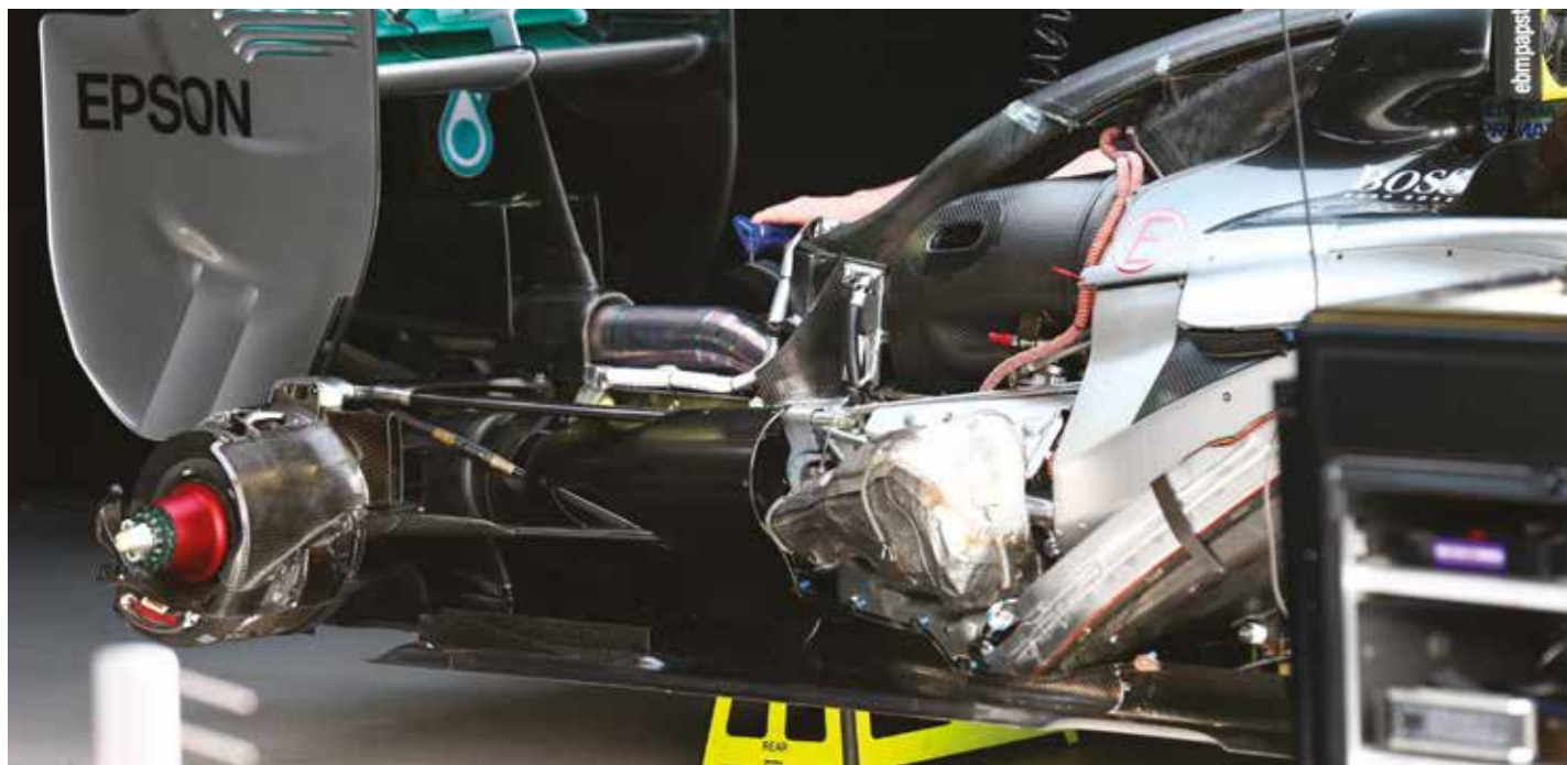
The rear end of the W06, with the bodywork removed showing the larger plenum and new exhaust design – for more on Mercedes' all-conquering power unit turn to page 18 of this issue. This picture is also a great illustration of the sort of complex packaging that's a major part of a successful F1 racecar
