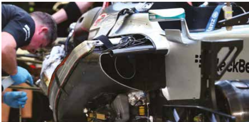
A view of one of the sidepod areas on the car. The cooling ducts are very similar in size to the W05 but the coolers and the ducting are more efficient. Cooling has been a challenge with the new power units since 2014
