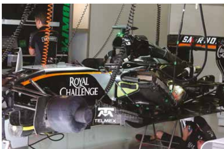
Force India produced a light weight and heavy weight chassis for its drivers in 2015; the lighter to compensate for Hulkenberg's greater weight. Next year both drivers will use lighter chassis
