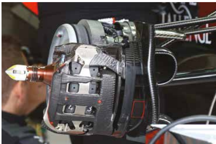
The brakes on the VJM08 prior to modification. At the Spanish GP Force India introduced a minor change by moving brake calipers from ahead of the front axle to behind it (see right)
