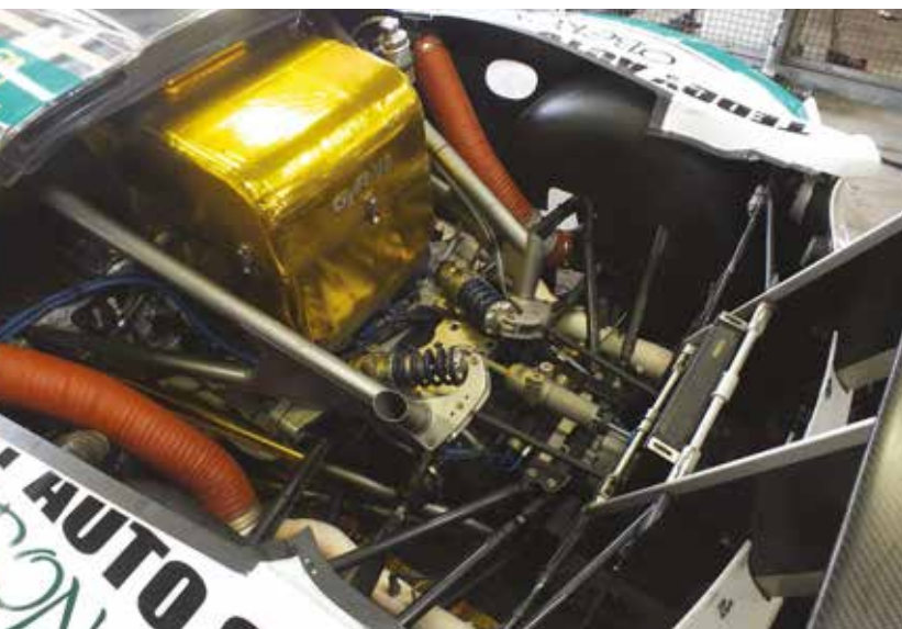
Somewhere in there is a Nissan VK45DE V8 – the engine also found in most LMP2 racecars. The rear suspension is carried partly on the transmission casing and partly on the bellhousing
