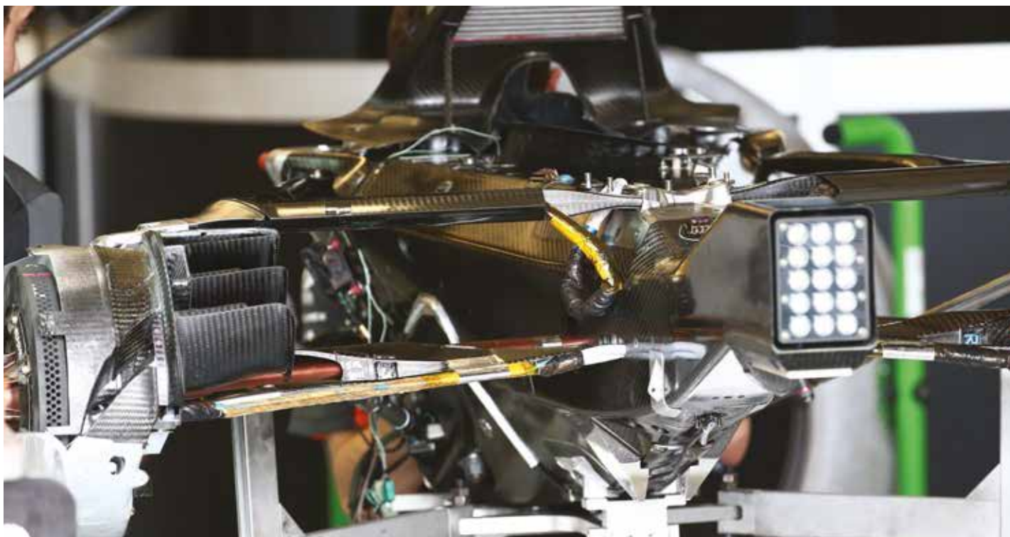
Mercedes twin-skin hybrid transmission and the rear suspension driveshaft passes through the lower wishbone. The use of the Mercedes 'box does bring some design constraints
