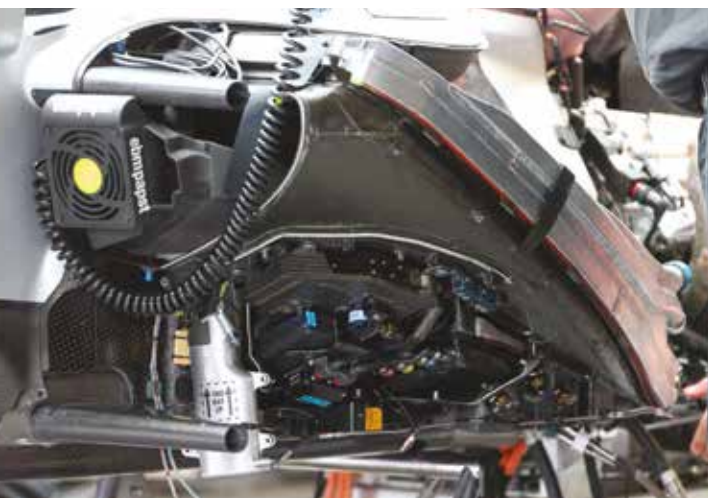
Sidepod area with bodywork removed. Side impact structures are visible; it's not as neat as it was in the W05 in this area but loss of FRIC freed up some space
