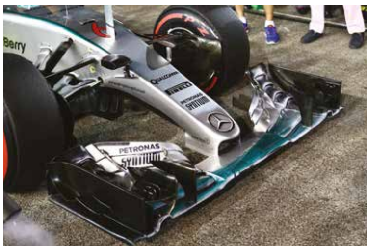
The biggest F1 rule change from 2014 to 2015 was to the nose of the cars but Mercedes did not have to change much in this area and the nose is similar to that seen on last year's W05
