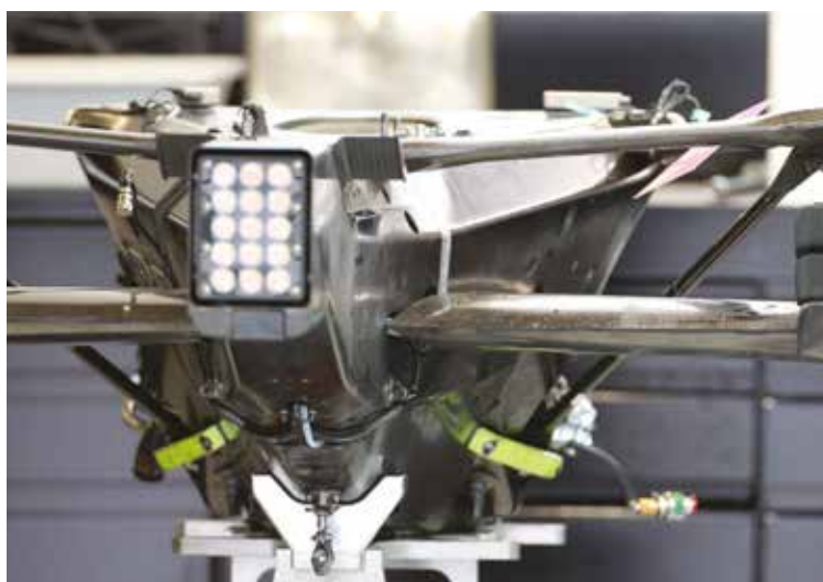
A closer look at the composite/titanium hybrid gearbox casing. The driveshaft passes through the rear leg of the lower wishbones which pick up on the composite casing of the transmission
