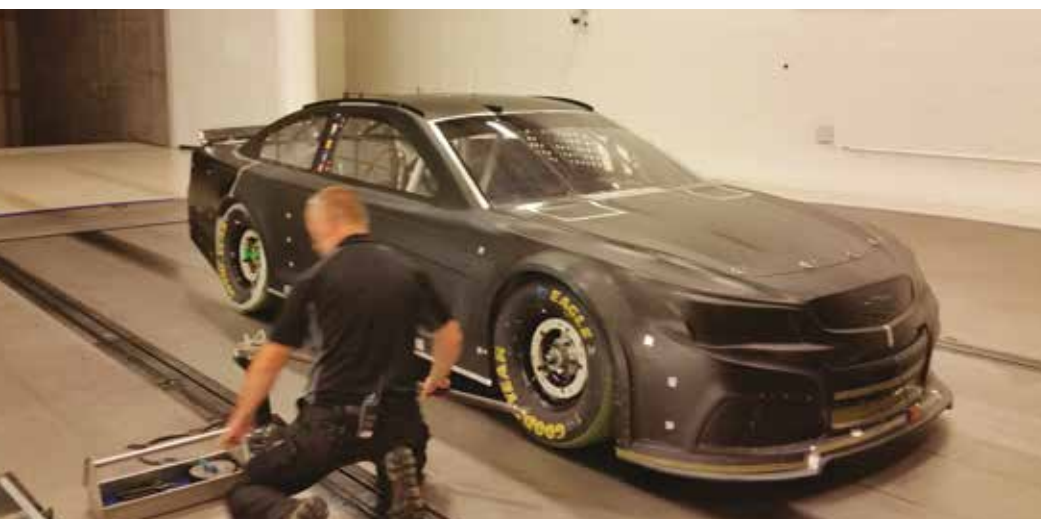
X-3 test car at the Windshear wind tunnel. The car was developed by NASCAR in conjunction with Richard Childress Racing
