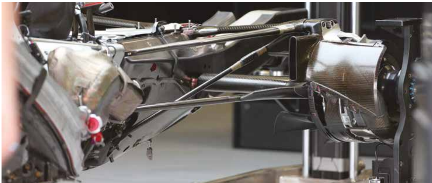
Mercedes uses a twin skinned transmission casing with a structural composite outer section and a titanium inner – the latter is just visible here at the front of the carbon case
