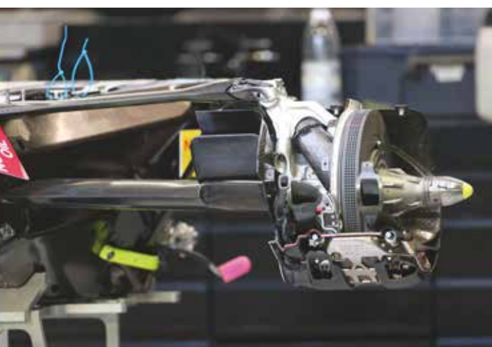
The rear brake assembly and upright: the uprights actually receive a great deal of attention in modern Formula 1 and are machined from a solid aluminium billet
