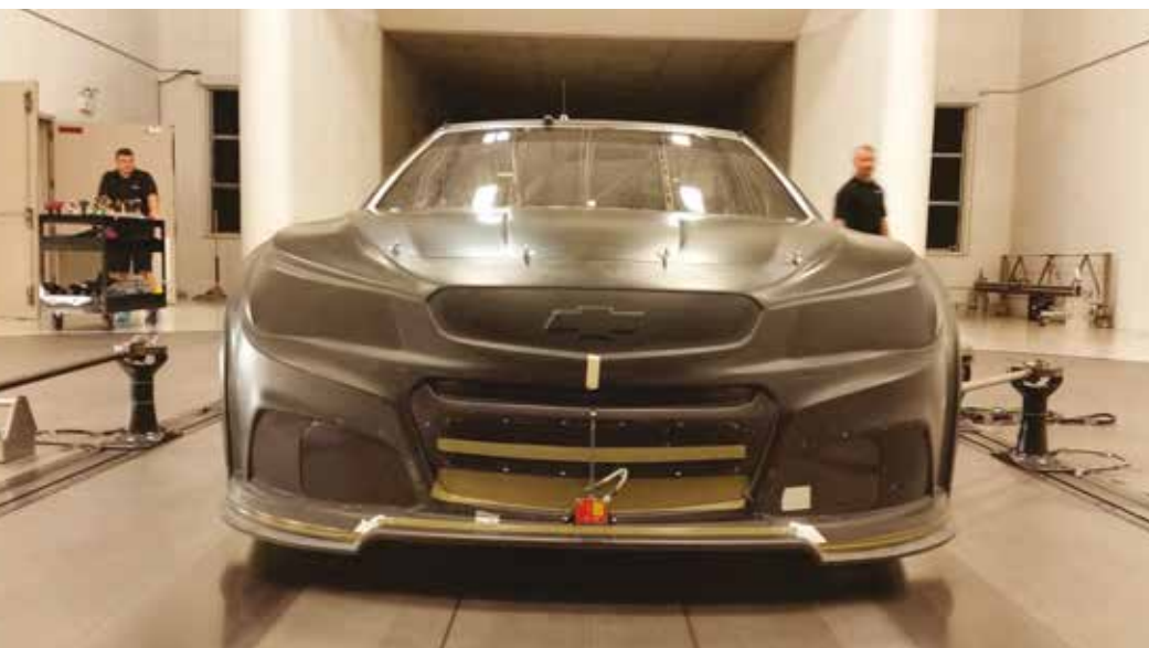
The X-3 features a raised splitter centre section to reduce ride height sensitivity, while it's also fitted with shorter side skirts
