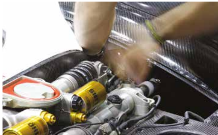
Dropping front ride height on suspension pushrods resulted in an increase in downforce
