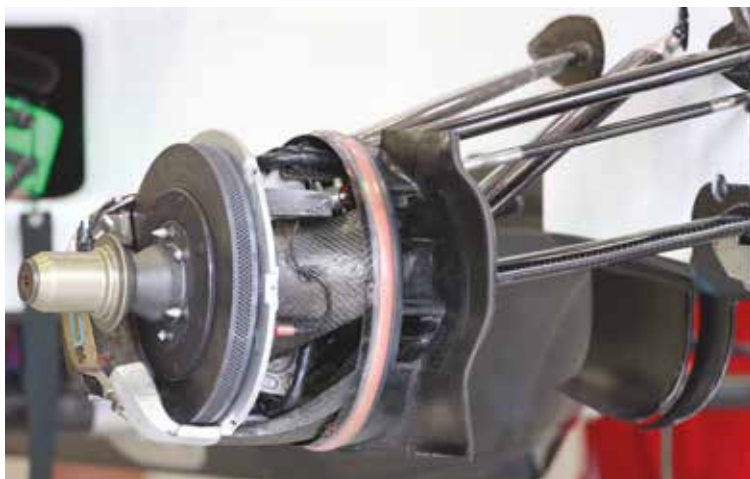
The brake ducts received an upgrade during the 2015 season. Some of the MR03B's improved performance was down to the relatively inexperienced drivers getting up to speed with the car
