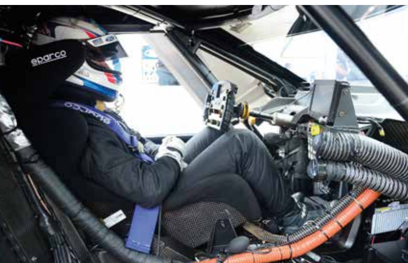
New cockpit rules see the drivers sitting in seats of a higher safety standard while nets must be fitted to windows. Steering column position is free and cabin temp must not exceed 32degC
