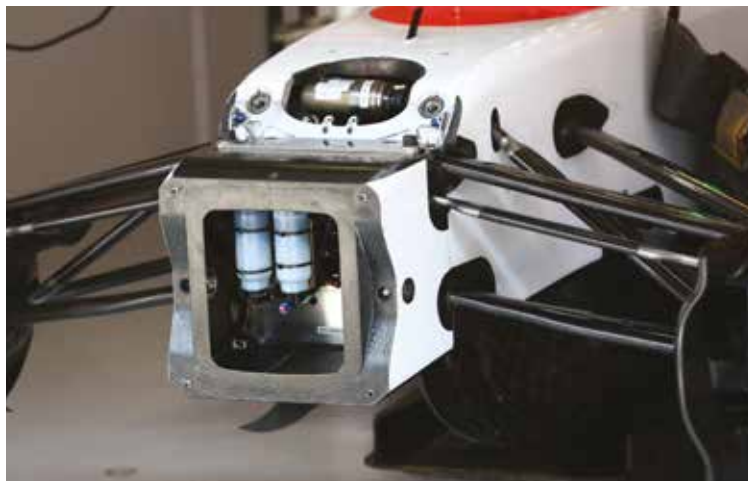
Front suspension is decoupled roll and receive spring system, to enable the team to individually tune and adjust damping. It also features inboard torsion bars
