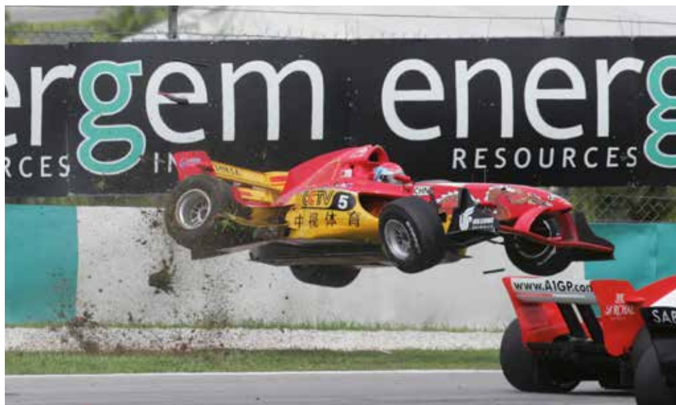
When a chassis lands floor-first after an airborne accident the forces are unusual and they can lead to serious injuries
