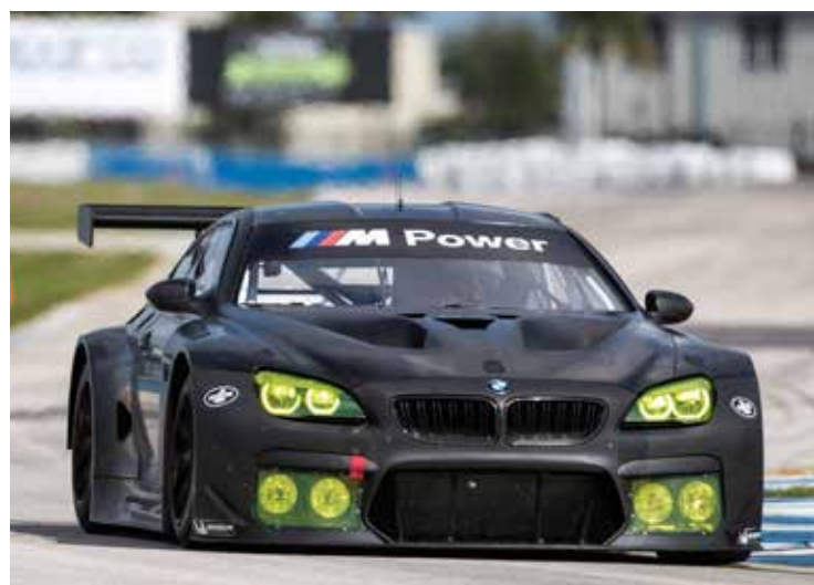
The BMW M6 GTE car was built using the company's Z4-replacing GT3 version as a basis, and it makes good use of the aerodynamic freedoms offered in the new GTE regulations
