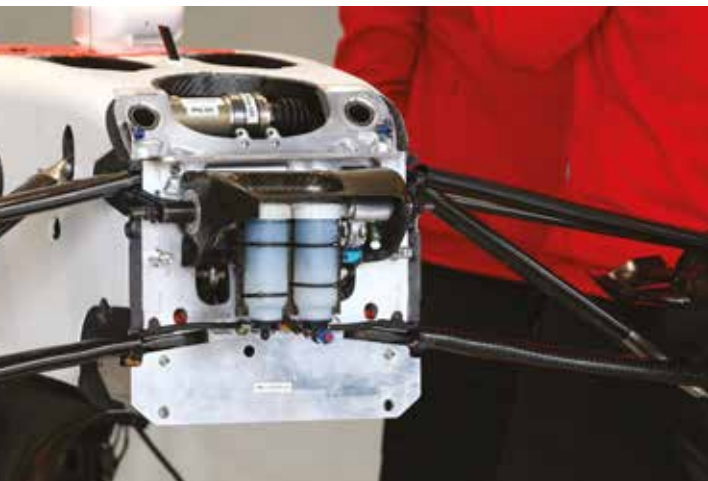
Manor aims to carry the metal bulkhead over into the 2016 racecar – this was actually a feature that was copied by the Red Bull team last season
