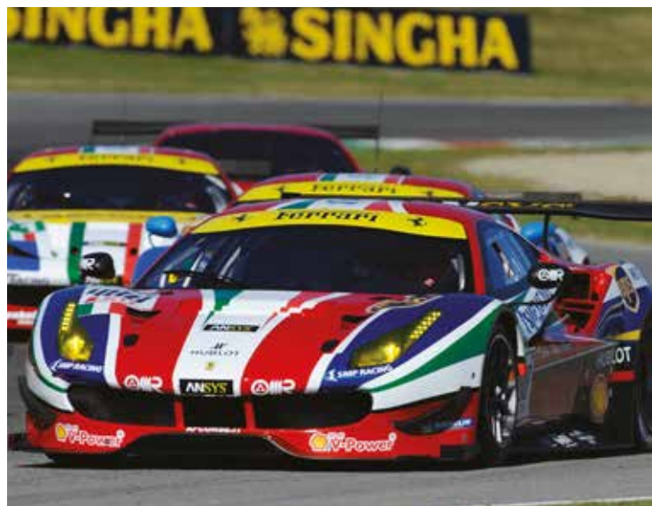
Ferrari has perhaps adopted the most extreme solution up front with a large splitter featuring a raised centre section and a Le Mans Prototype style cut-out and turning vane
