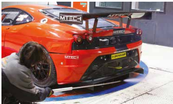
Flow from F430's central diffuser was orderly – but not so from the outer diffuser (below)
