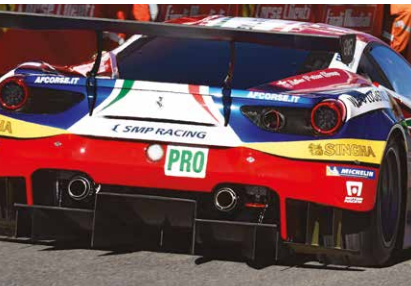
Ferrari's 488 GTE. The defining feature of the 2016 rules is the huge rear diffuser. The design of the diffusers is free but they must sit within the measurement area defined in the regulations
