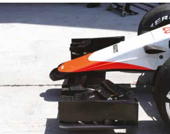
The 'B' version of the Manor MR03 had to have a brand new nose and various modifications to the monocoque to help it comply with the 2015 regulations
