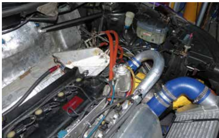
Citroën CTCC engine: the powerplants are based on 2-litre turbocharged units using the production block and head, but engine development is relatively free
