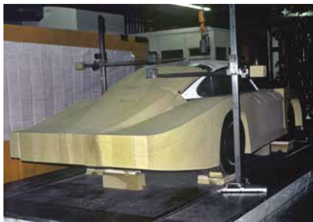
Shaping the very slick body buck for the 935/78 Group 5 racecar on an older model 935 – slippery aero was a must for the Mulsanne Straight at Le Mans
