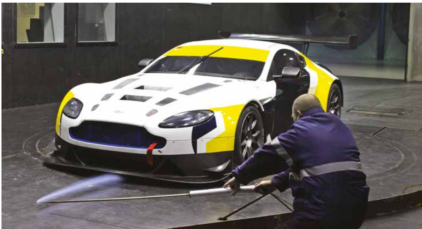
Note the smoke plume dipping under the Aston Martin's splitter, the underside of which is shaped into a cambered diffuser section across the central three quarters of its width
