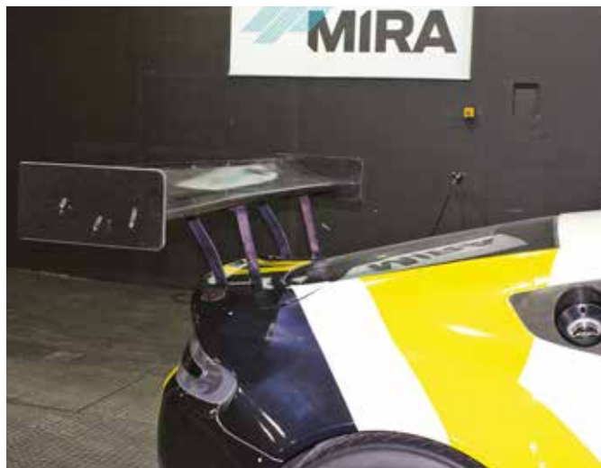
The rear wing is slightly twisted across its span which is a feature of Aston Martin GTs
