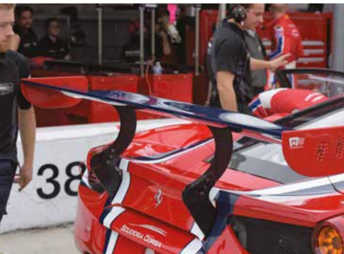
Ferrari's aerodynamic philosophy with its new 488 GTB racer is radical and centred on downforce. Its aggressive rear wing is part of a sophisticated package
