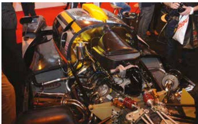
The Ginetta G57 is powered by a 6.2-litre Chevrolet engine giving 580bhp – the company claims it will be three seconds faster than an LMP2 around Silverstone
