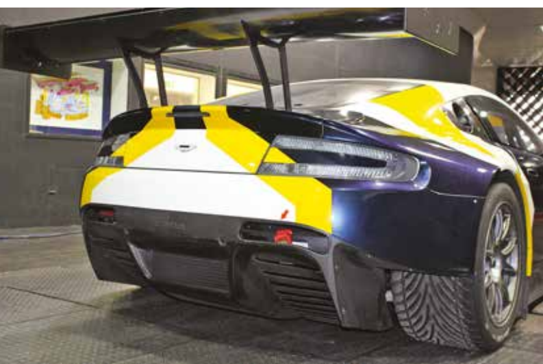
The lower rear section featured slotted pieces – the Aston does not have a flat floor panel
