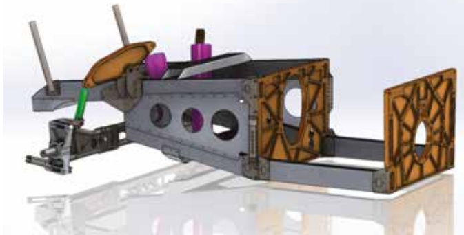
Hartley has fabricated an aluminium glu-lam monocoque box section in front of the engine which holds the front suspension and houses oil reservoirs for the dry sump
