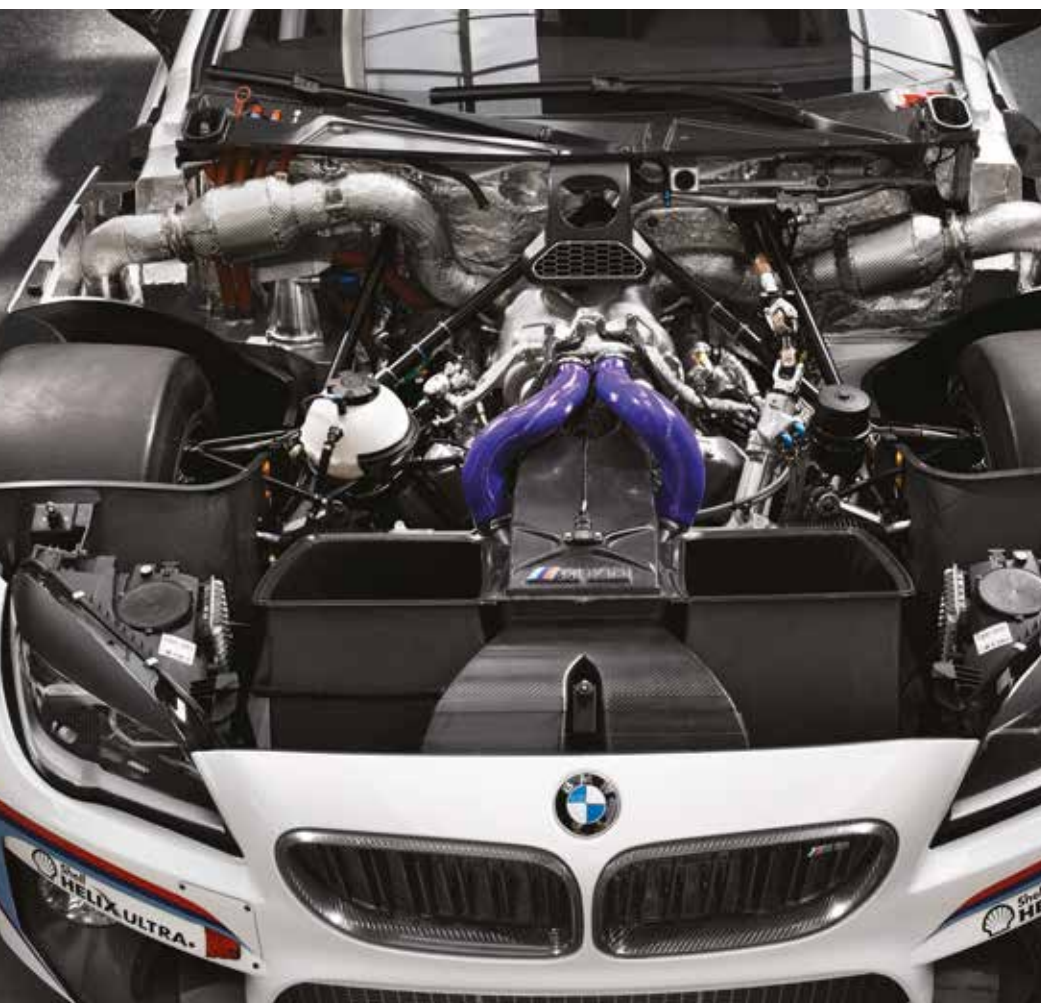
M6 engine produces 600bhp in road-going trim, which is a great base for this GT3 power unit. The turbo engine was suitable for both GT categories with minor modifications to allow the car to fit into the FIA performance windows
