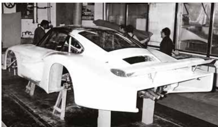
Porsche 935/78 undergoing its build process. Black roof and A- and B-pillars of the road car can be seen; the original body parts remaining once the 911 was transformed into a racecar
