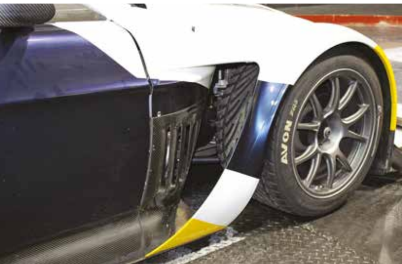
The front wheel arches feature large rear-facing vents to aid the exit of air from the arch
