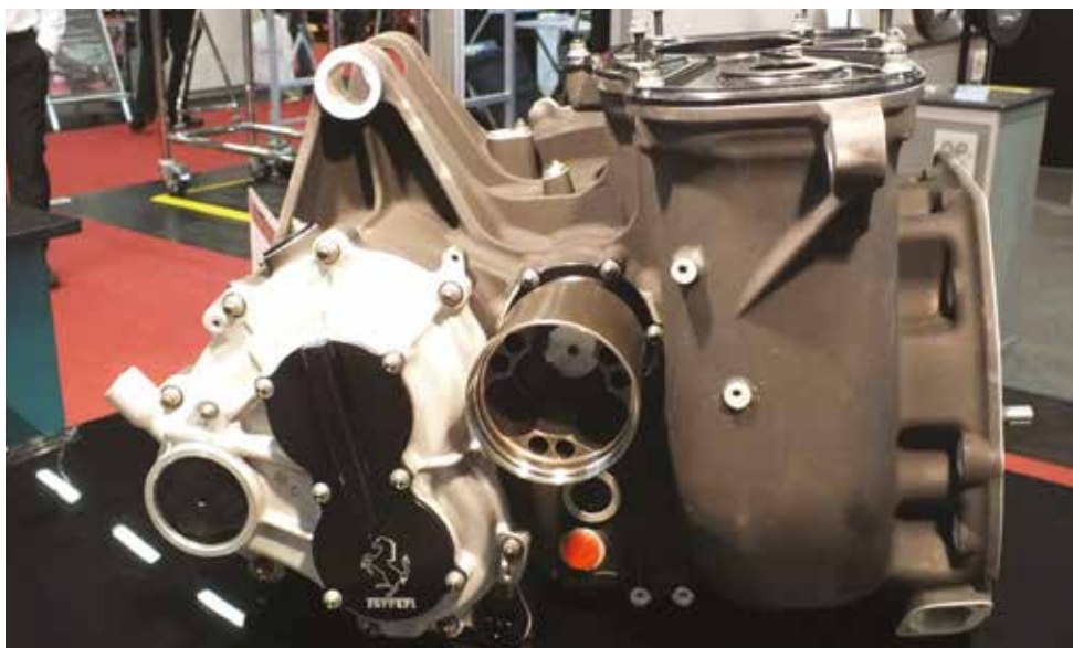
Ferrari has switched to this Xtrac transverse gearbox in order to allow the rear diffuser to rise further forward in the 488 than it did in its 458 predecessor. Meanwhile, the gearshift mechanism for the car has switched from Hewland to Megaline
