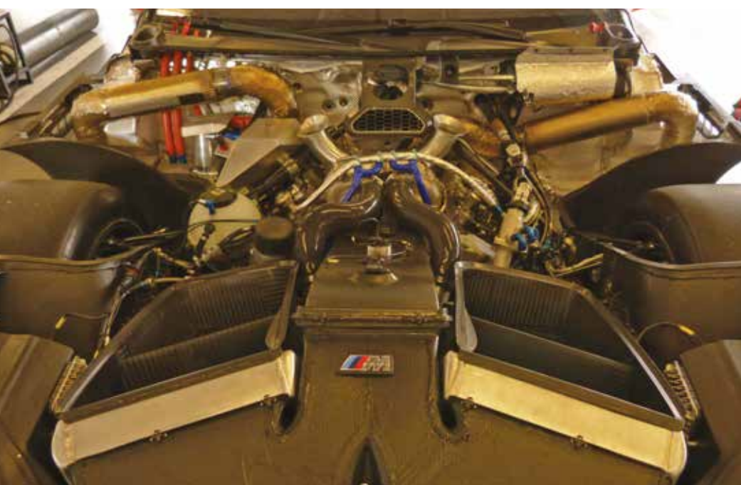
Switching to a dry sump has freed up space underneath the power unit and so the engine has been dropped in the chassis. The V8 engine suffered from overheating early in its development so it was tested in colder climes to begin with
