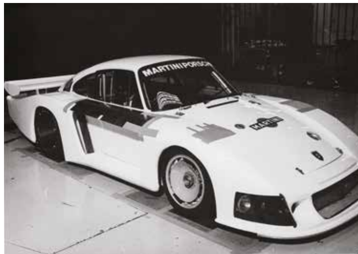
Porsche decided to switch from the wide and low rear wing (above) to a narrow, high wing (below) at the same time as the controversial door design was changed
