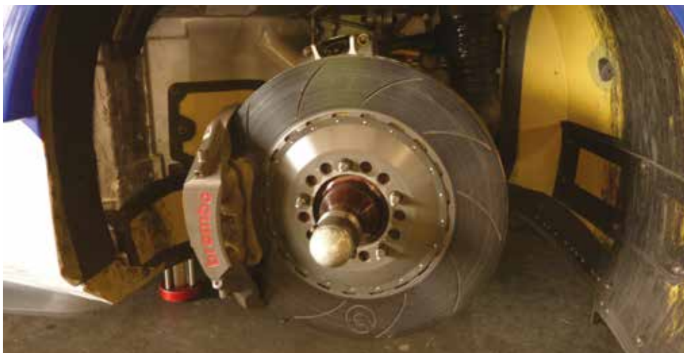
There has been much work on the braking system, partly aimed at easing the car's balance shift during weight transfer in the braking zone. The uprights are not hand crafted, as they were on the 458, to keep the costs down for GT3 customers
