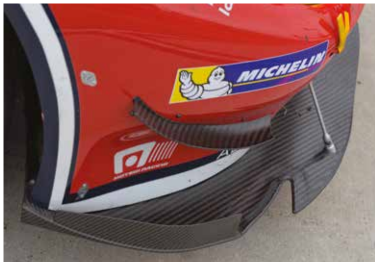
A new regulation allows the front splitter and the rear diffuser to protrude further than the edge of the car's bodywork, which could make these complex parts susceptible to crash damage
