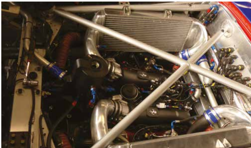
The engine in the GTLM version of the 488. The 3.9-litre turbocharged unit comes with a weight penalty. Due to the weight of the turbocharging system, the car has had to go on to something of a diet to hit the minimum weight
