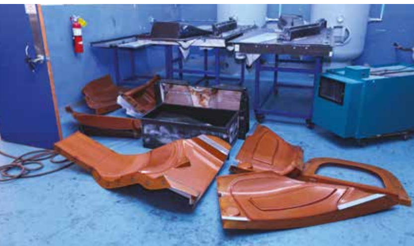
Doors, splitter and roof are made from pre-impregnated fibreglass cloth which is vacuum-bagged to remove air from the laminate and then heated in an autoclave at Elan's factory
