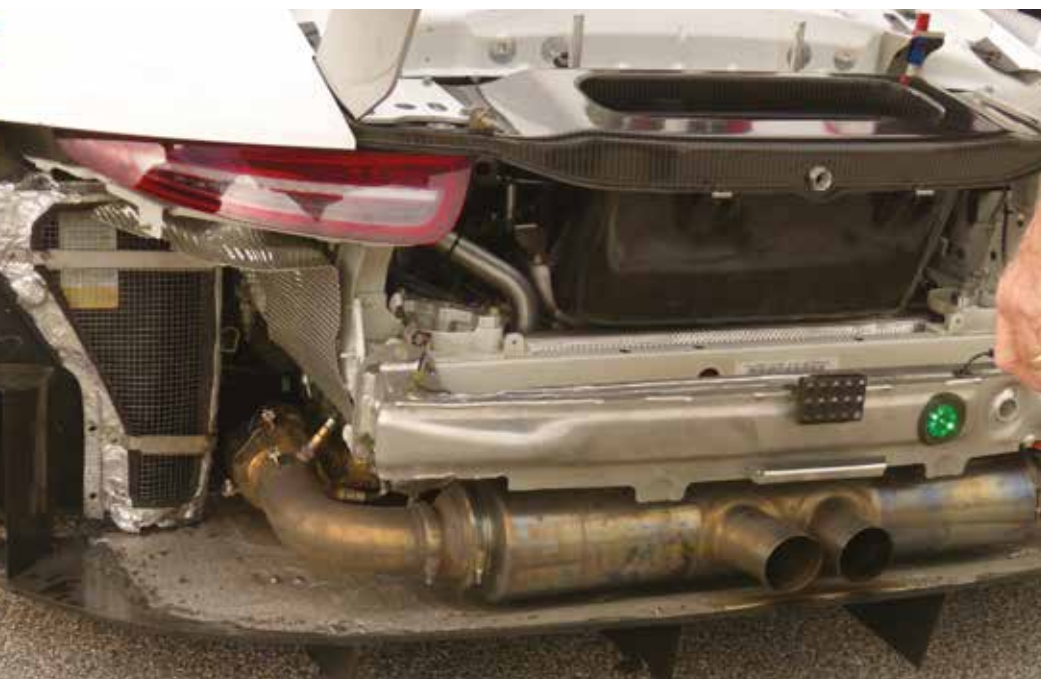
The sting in the tail: Porsche deliberated over whether it should use a turbocharged engine but in the end opted for the familiar 6-cylinder boxer in the GT3. The positioning of the engine means the diffuser cannot be lifted to a higher position
