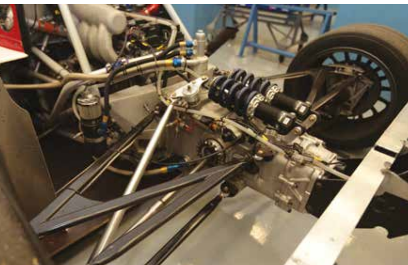
Suspension philosophy is all about saving costs: the rear uprights are the same as the front, for instance, and corners can be swapped. But dampers are top quality and relatively expensive
