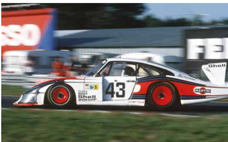
Just half the door was covered in compromise version of Moby Dick. When the FIA decided to reverse its decision to ban fully covered doors Singer opted to stick with this solution anyway
