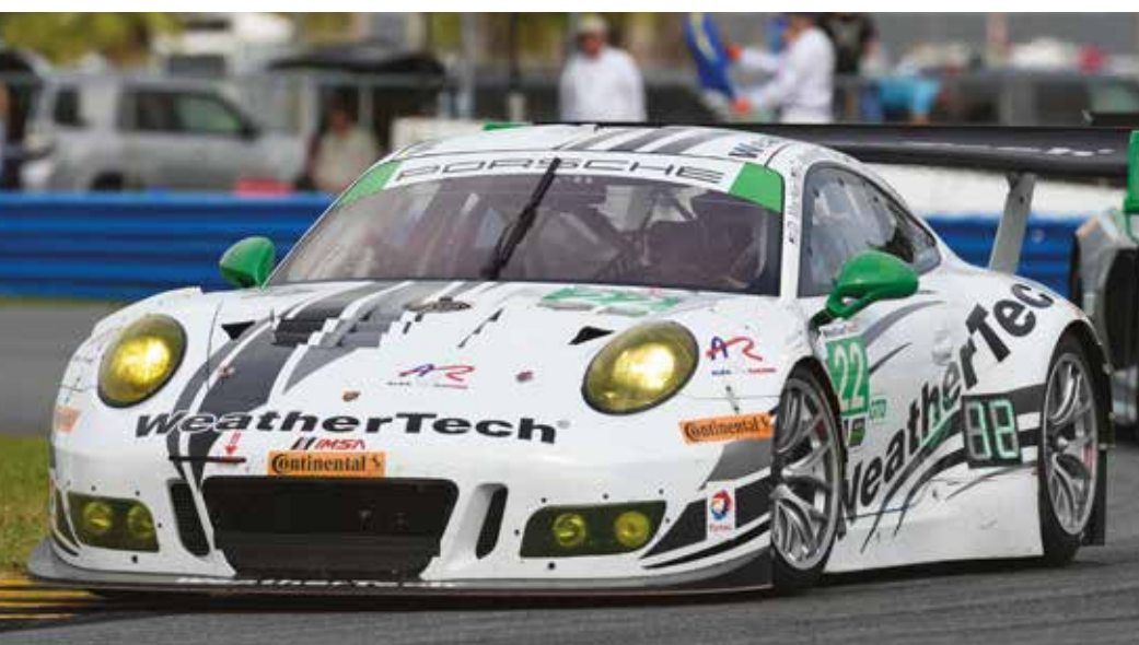
The GT3 R is an aerodynamically uncluttered car and Porsche believes that this is the essence of customer racing, feeling that over-developed aero can drive up the costs. Porsche has worked hard to reduce weight, with plenty of carbon body parts
