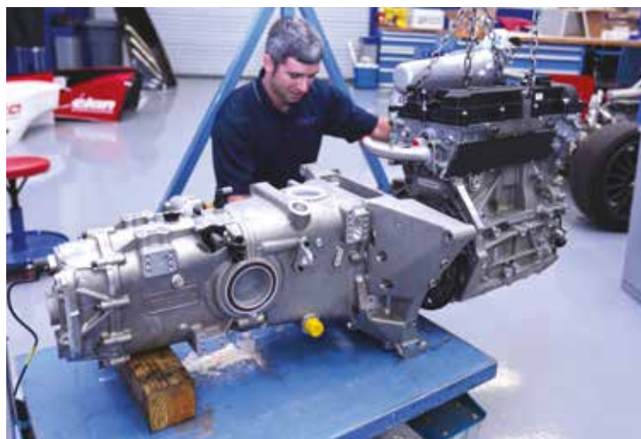
The Sadev 6-speed Formula 3-spec sequential gearbox is mated to a Mazda 2.0-litre MZR powerplant, which produces close to 200bhp and 145lb.ft of torque
