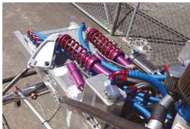
Hartley rebuilds and modifies its own shock absorbers, which is also a big part of its regular business. There's a shock dyno to calibrate damper performance
