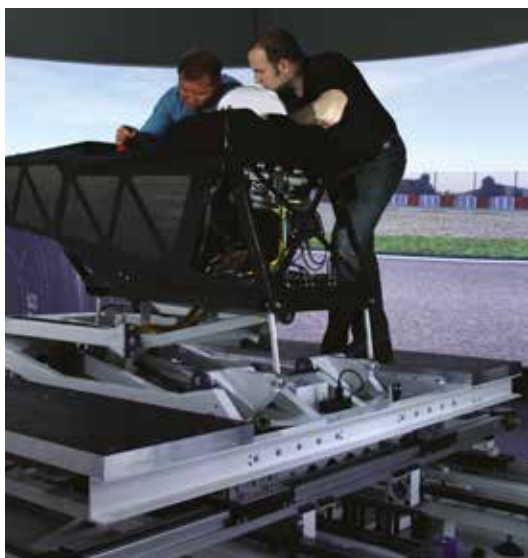
The platform is designed to be inherently stiff while it also has a very low centre of gravity, which reduces the bending moments
