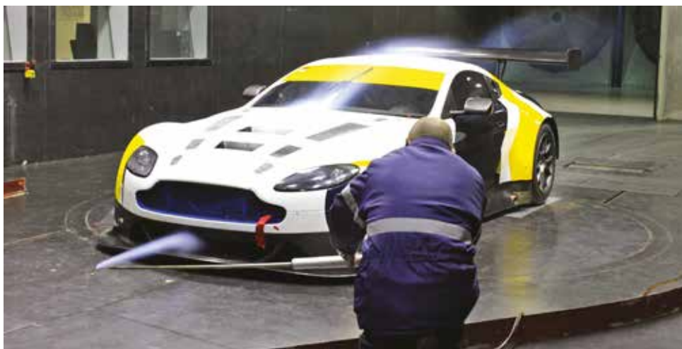
The front, lower aperture fed the rear bonnet duct. The smoke plume was a great way to show the different airflow routes
