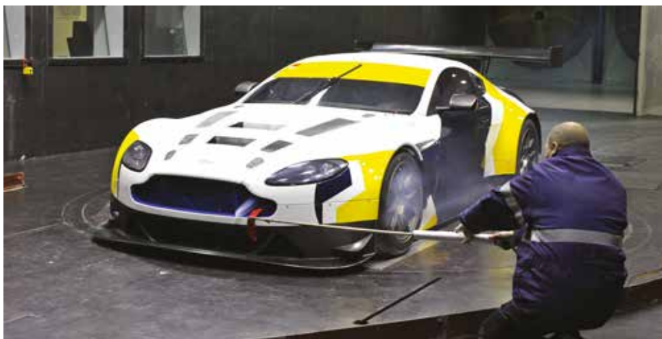
The outer, upper aperture fed the brake cooling ducts. The Aston features beautifully crafted, fully ducted, cooling systems
