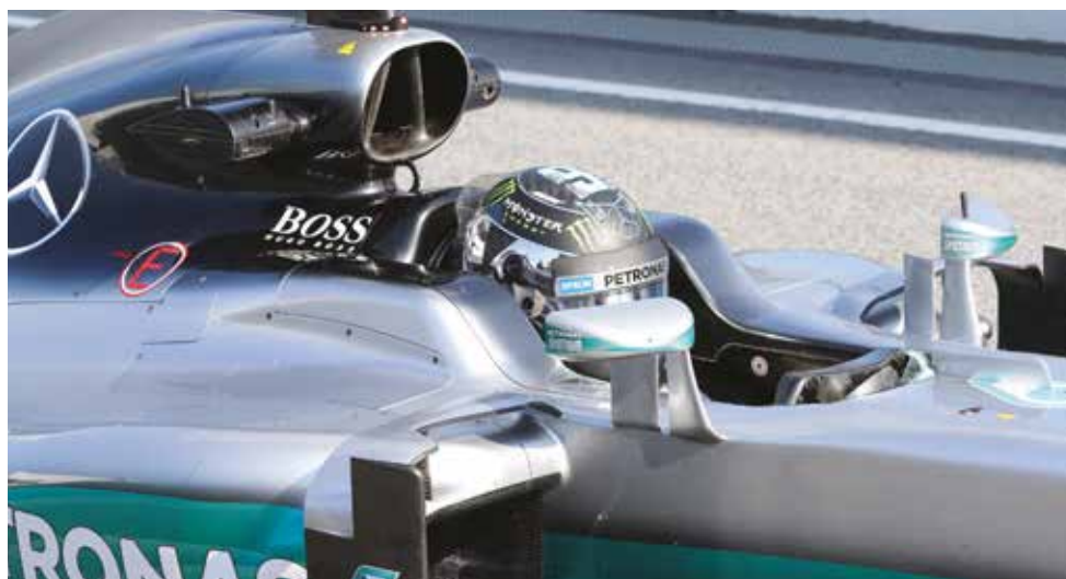
Higher cockpit sides are the main regulation change this year. These now have to pass a much tougher crash test of 50kN
