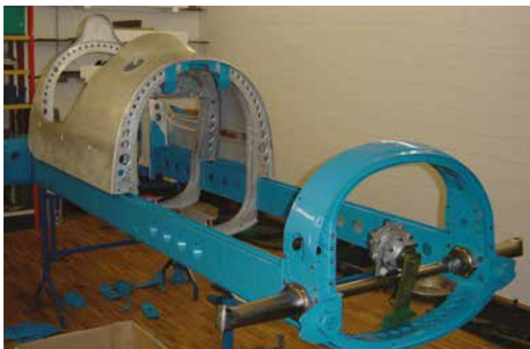
The chassis features two tall side sections plus three oval cross members to give it strength. There's an echo of 1930s aeronautical design thinking, unsurprising given the company's roots
