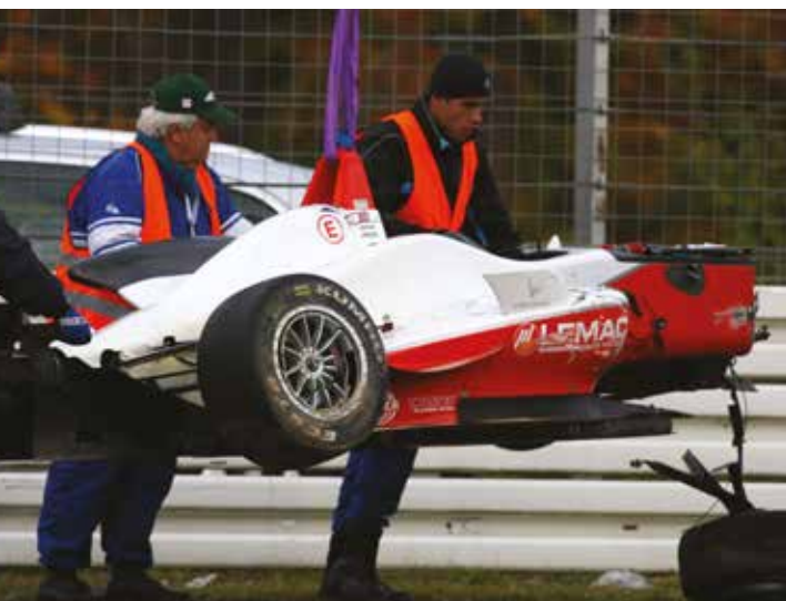
Most damage to a tub is clearly visible and the teams learn where that damage is more likely to occur. Sometimes they will also make use of ultrasonic testing
