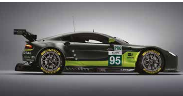
The huge diffuser is the most obvious change to the Vantage GTE, this to claw back downforce after a concerted effort to reduce drag; but it does sit in a highly vulnerable position
