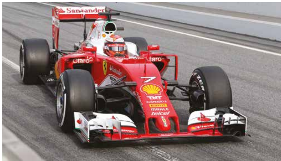
Ferrari has abandoned pullrod front suspension and has returned to a pushrod layout. Also note new short and narrow nose
