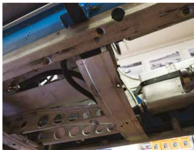
The underside of the frame showing drilled sections, which were an attempt to cut down weight. The car also features a full-length belly pan to help reduce drag
