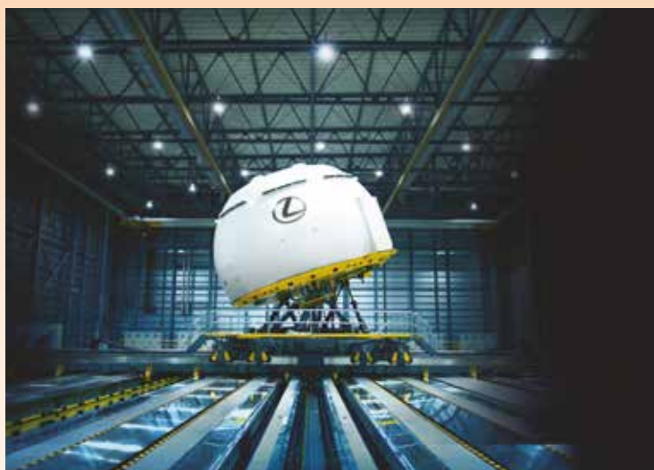
Human Factors DIL simulators are typically operated by road car manufacturers and they are designed to closely simulate actual road driving conditions. This one belongs to Lexus
