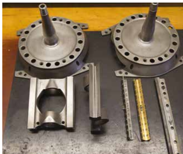
The original components of the CTA Arsenal's front sliding block suspension – these caused problems when the car made its woeful historic racing debut
