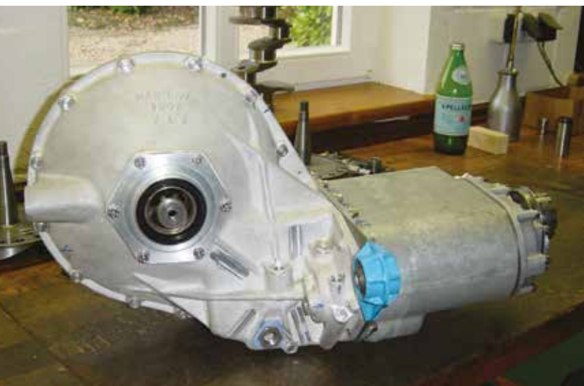
The car's gearbox and final drive unit. The transmission needed to be sturdy to handle the 330bhp produced by the Arsenal's hugely impressive 1500cc supercharged powerplant
