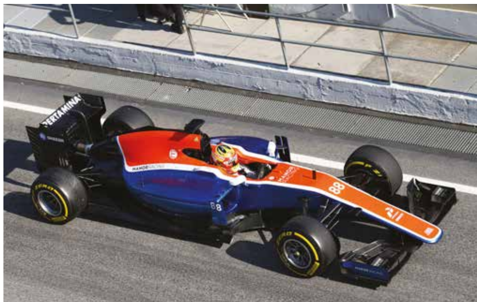
The Manor MRT05 is the team's first new car for two years. It has almost nothing in common with the 2014 MR03, but does share a lot with the stillborn MNR1. This year the team has also switched to a Mercedes engine and Williams transmission
