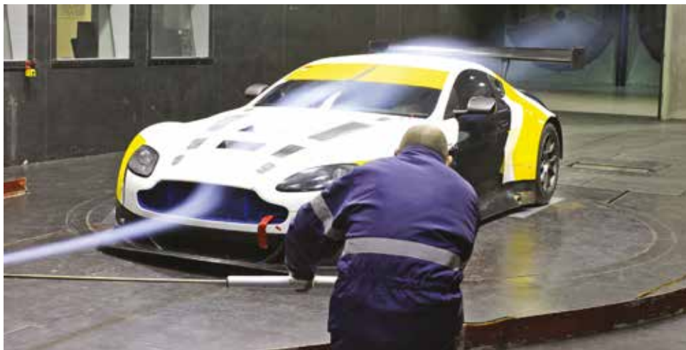
The Aston Martin in the wind tunnel. Here the front upper aperture can be seen feeding the forward exit duct in the bonnet
