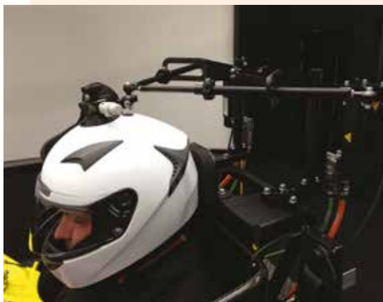
Ansible Motion's Helmet Loading System is just one way the company is enhancing the experience for simulator drivers
