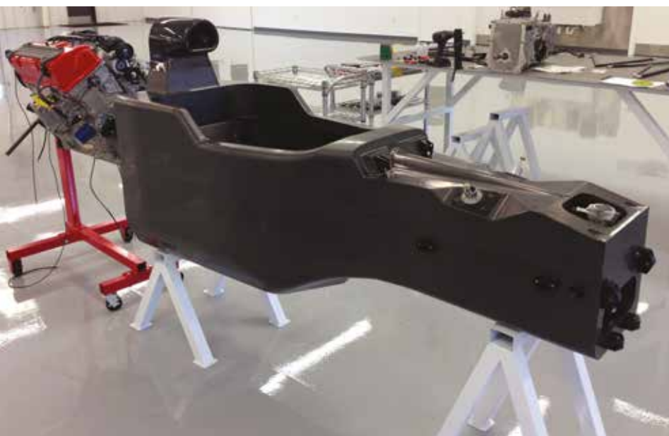
Modern carbon composite monocoques are extremely tough while the teams tend to send them back to the manufacturer for examination at regular intervals; but there is currently no regulation to ensure this happens
