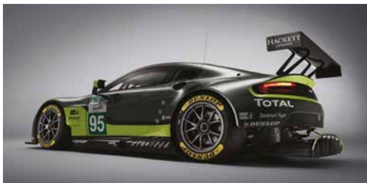
The huge diffuser is the most obvious change to the Vantage GTE, this to claw back downforce after a concerted effort to reduce drag; but it does sit in a highly vulnerable position
