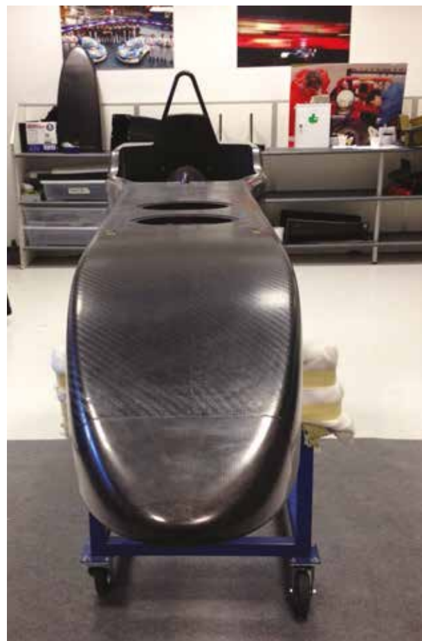
Carbon tubs have an internal and external skin of carbon fibre and a core constructed of Kevlar or an aluminium honeycomb
