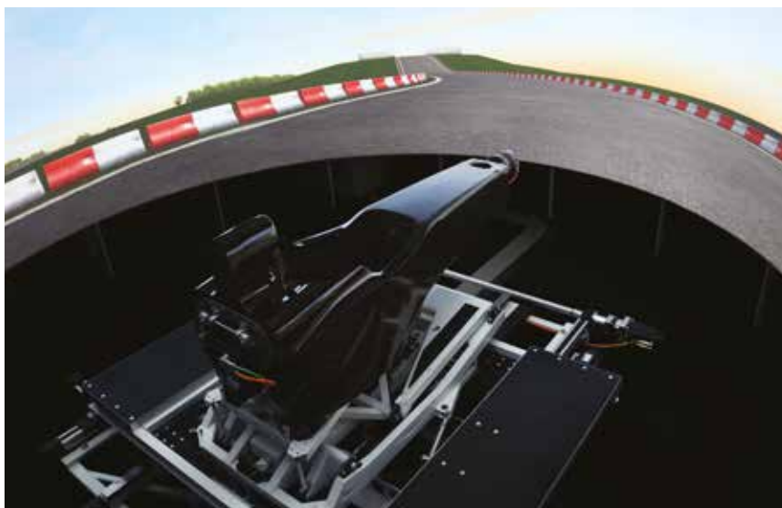
The cockpit the race driver will sit in needs to feel as real as possible. Typically Formula 1 teams will fit a monocoque to the simulator. For extra realism there will be torque force on steering wheel and seat belts
