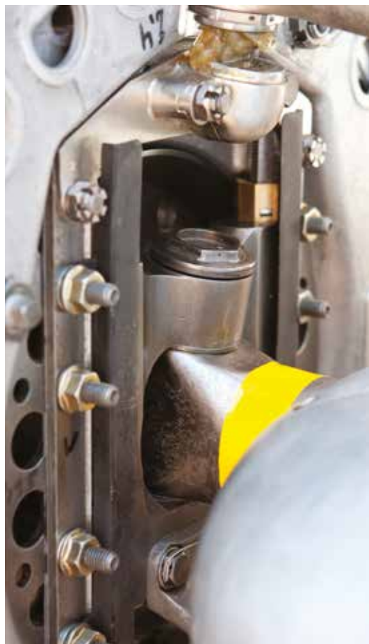
The original front sliding block suspension (above) as installed on the car when it run in 2010 Monaco Historic GP practice (below)
