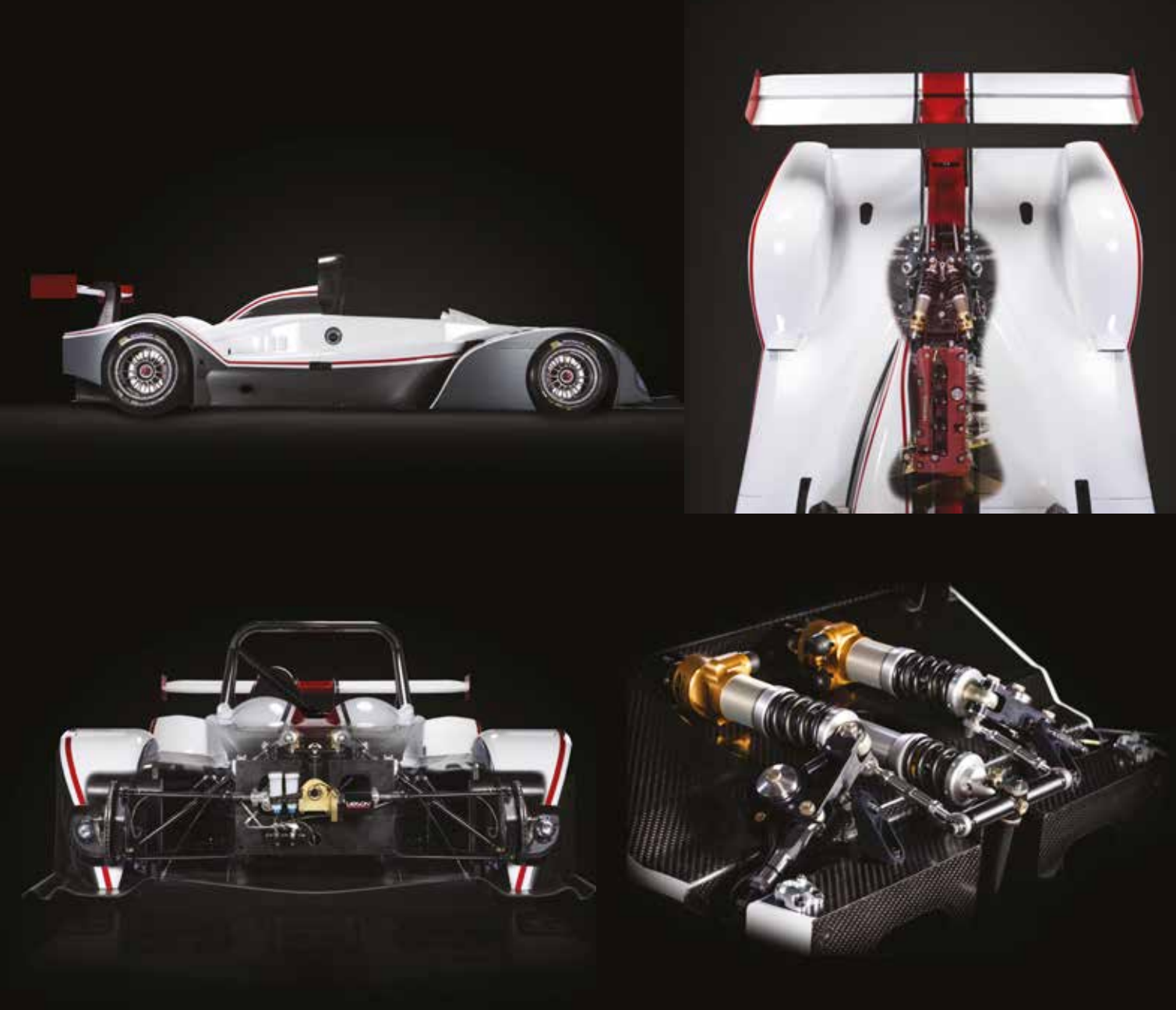
Top left and above left: The GH-20 is a full carbon monocoque – with carbon bodywork in V de V trim. Top right: The car is powered by a 2-litre Honda K20 engine. This dry sumped unit produces 255bhp and revs to 8200rpm, which is the maximum revs in V de V. Above right: Because of its high downforce levels the car uses a clever third element front suspension system which is adjustable by using spring stiffness and single way damping but also with the use of an ‘engagement gap’. Dampers are Ohlins TTX40 4-way adjustable
