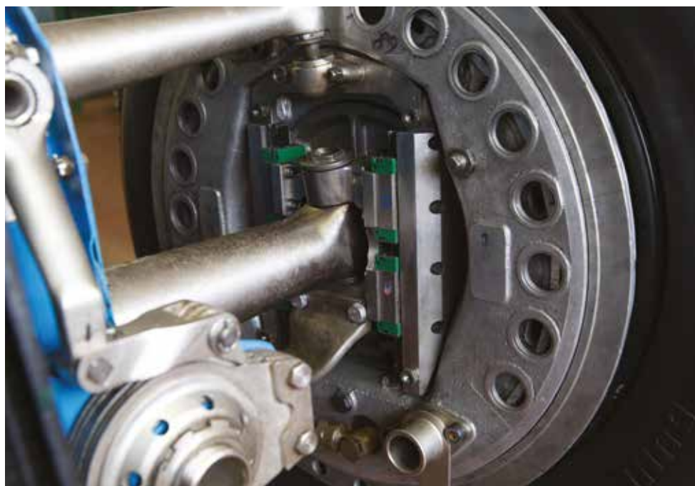
The modified front sliding blocks that are now fitted to the Arsenal. The blocks on the uprights fit in to slots on the back of the drum brakes, which allow the wheels to move up and down independently. It's a smart idea but it didn't quite work out
