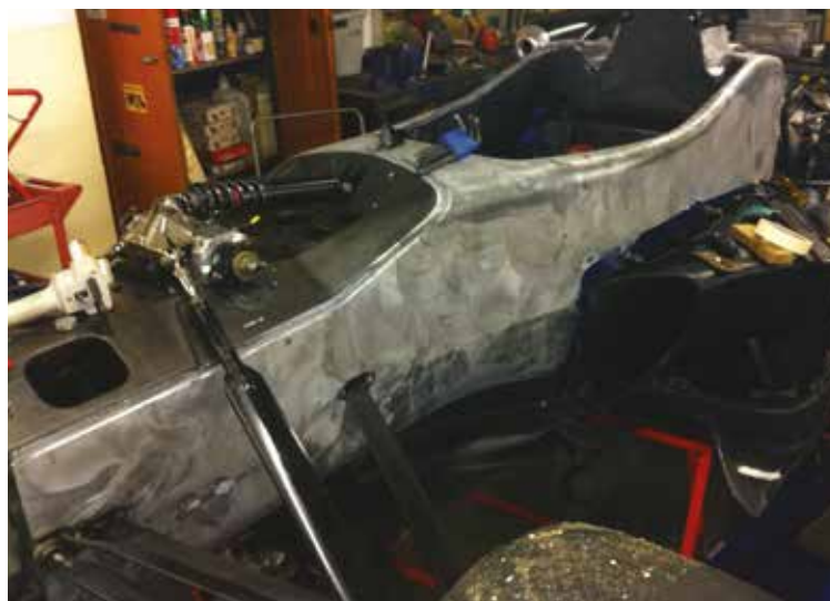
This old tub has seen better days but it might still be in great shape. Dallara checked one well-used 20-year-old chassis and found it was fine. Picture credit: Tristan Cliffe/Dallara F398.com
