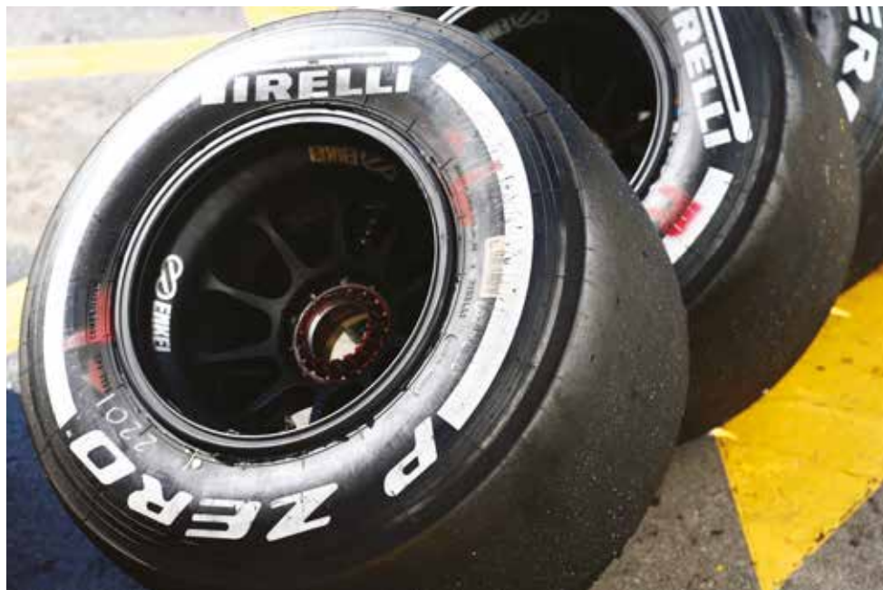
Pirelli has brought out a new type of tyre for Formula 1 in 2016. The new concept features a thin operational layer and a lower-grip base level beneath it. It forces teams to pit before wear reaches a critical level, as it did a couple of times in 2015
