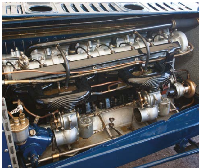
The 1919 Ballot (above) with the Ernest Henry designed twin-cam straight engine (above right). In many ways this was the forerunner of the legendary Offenhauser Indy engine
