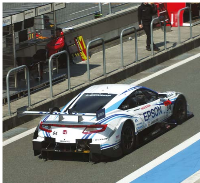
The Honda NSX Concept GT is the only mid-engined GT500 car. Up until this season it packed a hybrid but this has been discarded because of supply issues
