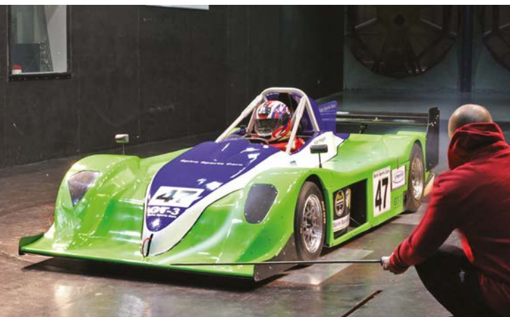
Bikeports car is much more advanced aerodynamically, with pronounced forward body concavity, splitter with diffuser, rear wing and rear diffuser. Single seat chassis also allowed
