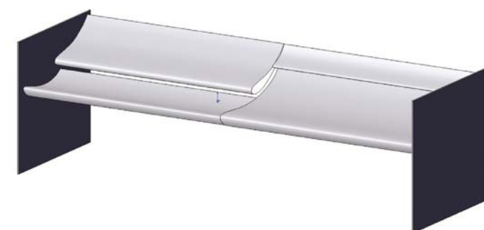
CAD 5: Maximum and minimum main element to flap chord ratios
