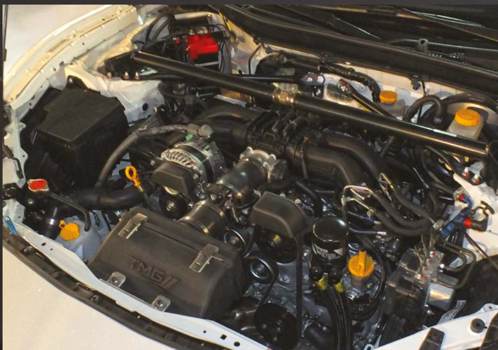
The Subaru-derived boxer engine is close to production specification for reasons of reliability and cost-effectiveness. TMG has kept an eye on costs at every stage of the GT86 CS-Cup's development, mindful of its amateur racer customer base
