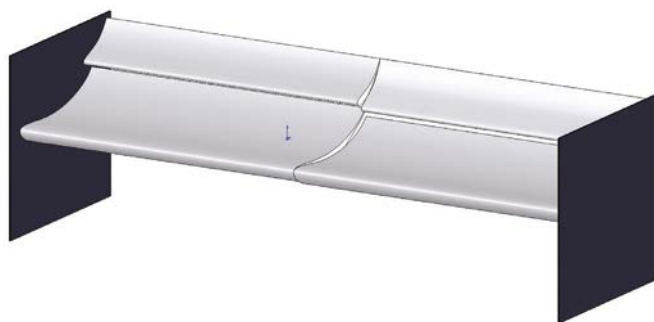
CAD 4: Minimum and maximum flap delta angles at the same overall angle
