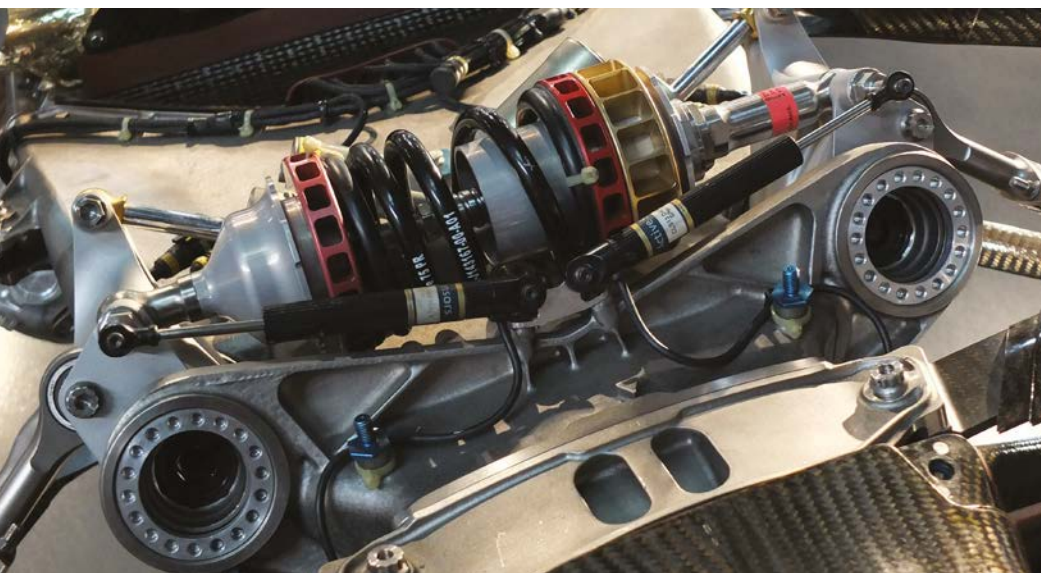
The TS050's rear suspension is based on the concept used on Toyota's Formula 1 car (pictured above). TMG would not be drawn on details but in essence the car's suspension is a double wishbone front and rear, pushrod system, with torsion bars
