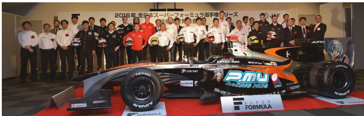
The Dallara SF14 is built to 2010 F1 safety standards and this year it goes into its third season as Super Formula chassis. The series says it will not replace the car until at least 2019
