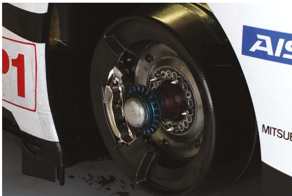
Toyota was the first of the P1 manufacturers to introduce a complete brake-by-wire system to handle the difference between those braking events that included the regeneration of the hybrid system and those that did not. Calipers are from Akebono
