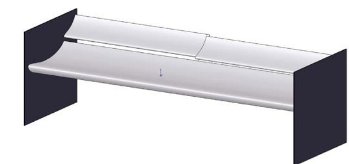
CAD 6: Slot gap variations; at the same vertical gap with the wing in isolation. The 20mm difference in horizontal overlap in this image significantly affected the results
