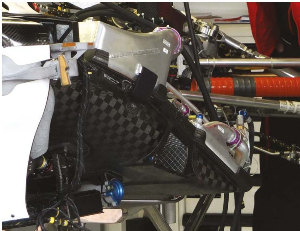
The sidepod of the TS050 contains the charge air cooler and the oil and water radiators arranged in a conventional single seater style. The packaging was a headache for TMG thanks to the late decision to switch to a turbo 2.4-litre V6 powerplant
