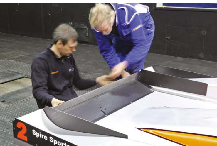
Tim Gray (left) and Paul Nightingale blur into action to fit a 60mm rear deck Gurney to the Spire GT-3 RGB car. This device added significant rear downforce
