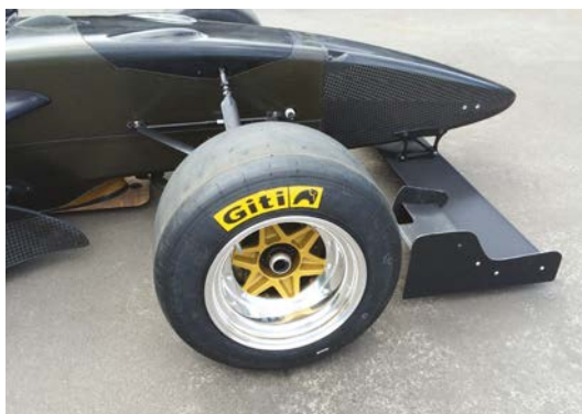
The aerodynamic capability of the modern Swift chassis has been reduced by cutting the front wing down to size, though the rear wing has not been altered. Singapore-based GiTi provides rubber
