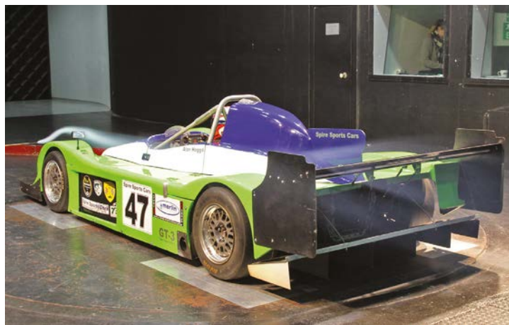
Bikeports car is much more advanced aerodynamically, with pronounced forward body concavity, splitter with diffuser, rear wing and rear diffuser. Single seat chassis also allowed
