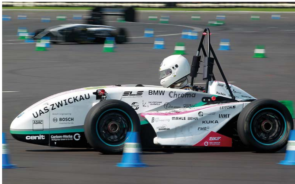
Making the track narrower at the rear than at the front is a common design feature of Formula Student cars, mainly because this helps the driver to negotiate the often tight courses without knocking over too many plastic bollards
