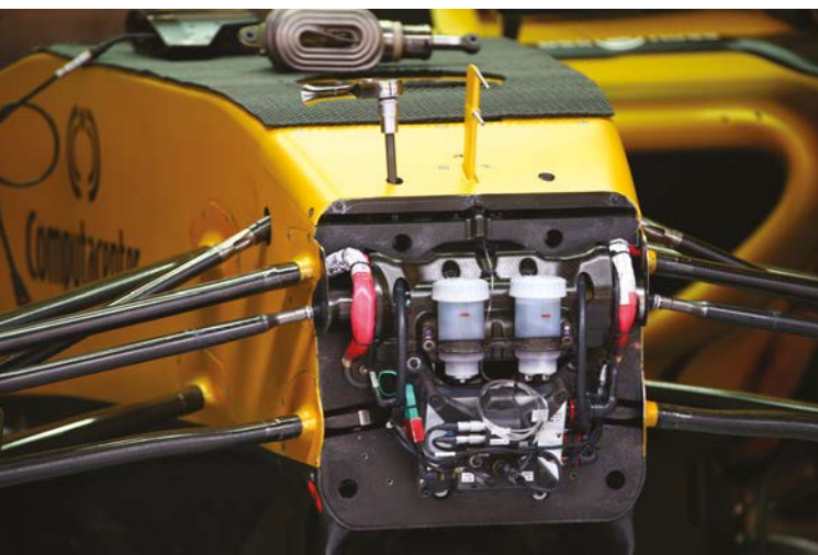
Front bulkhead. One of the big worries for Renault at the first test this year was that it simply did not know the exact weight of the car or just how that weight was distributed
