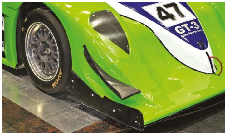
These dive planes produced an increase in downforce at the front and a loss at the rear
