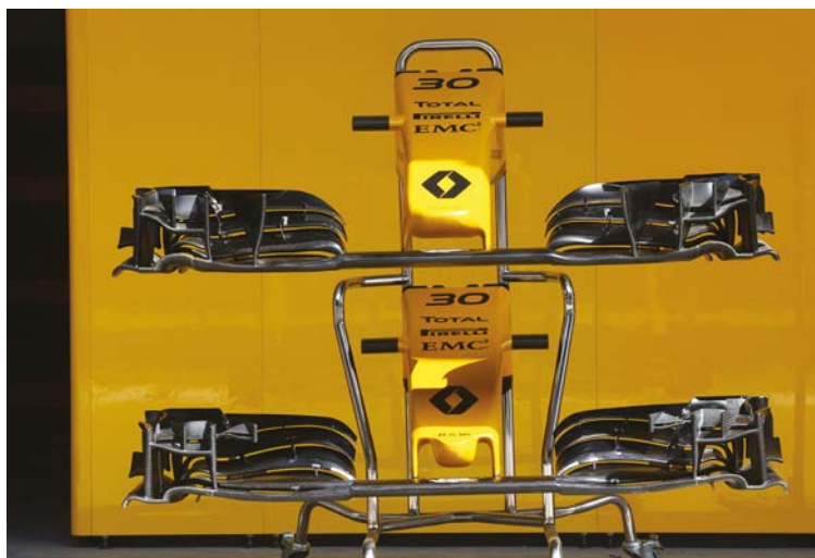
The Renault's launch spec nose is shown here above the RS16's new nose. The first of the two noses was very similar to that used on the Enstone team's 2015 racecar, the Lotus E23
