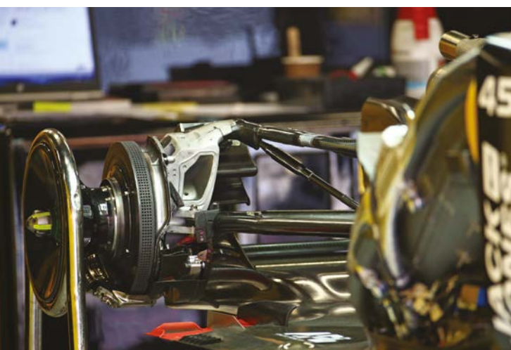
Rear brake and aluminium upright. Like all F1 cars the RS16 uses pull rods at the rear. Enstone was hit hard by the banning of interconnected technology in 2014
