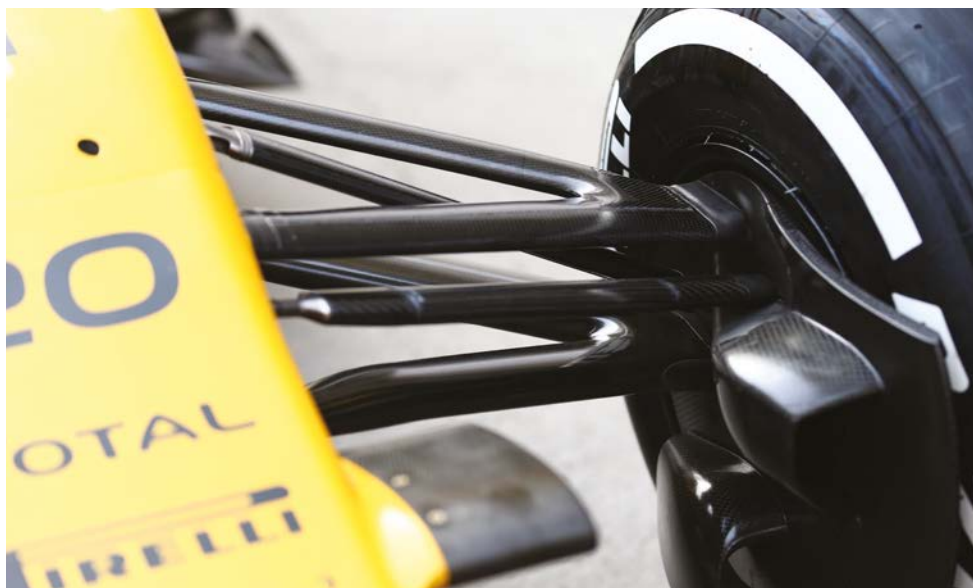
The RS16 does not have a blended lower wishbone on the front of the car, while the team has so far resisted the temptation to go with a narrow span wishbone, which some cars are running this season, though this approach is now being considered
