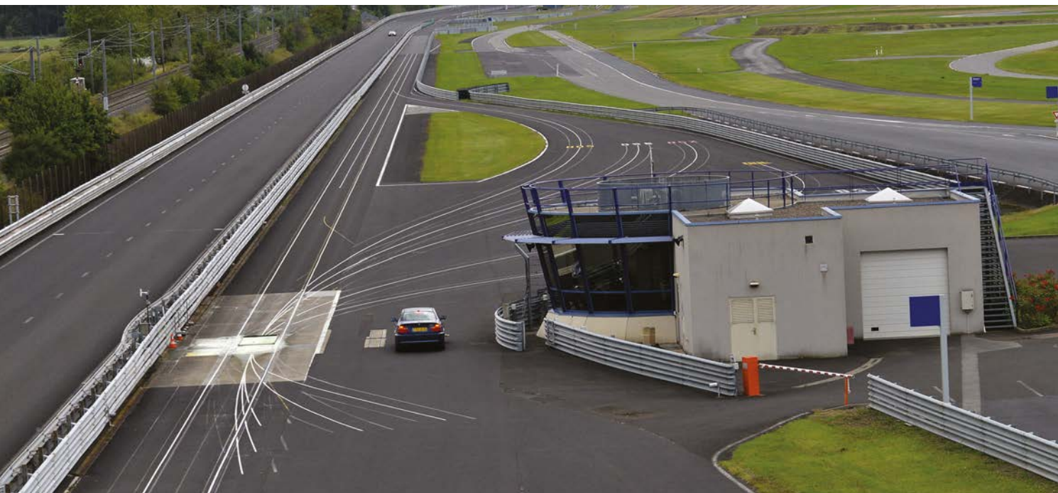
The FIA checks that GTE cars from the manufacturers fit within the performance boxes for power, drag and downforce – the latter is tested on this clever downforce plate at Ladoux
