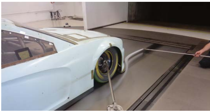
Xfinity cars have highly flared wheel openings. Note the flow of the smoke over the flare
