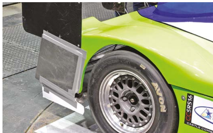
The rear infill panels produced a surprising drag reduction on the Bikesports racecar
