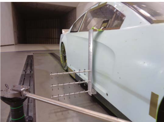
A 42 probe door-mounted Kiel testing array was fashioned for each side of the racecar
