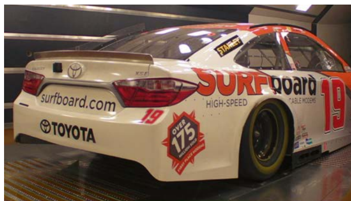
The Michigan/Kentucky development spoiler has been reduced in both width and height
