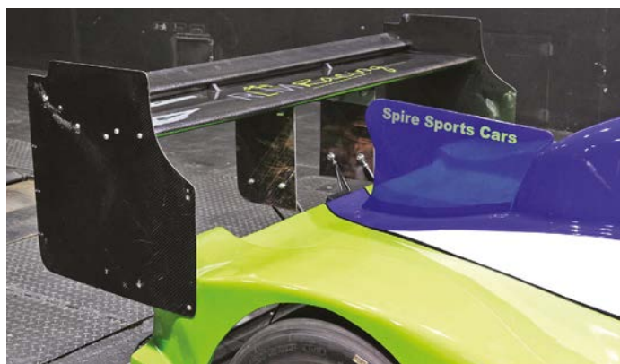
To begin with the rear wing was raised by 200mm to explore higher downforce potential
