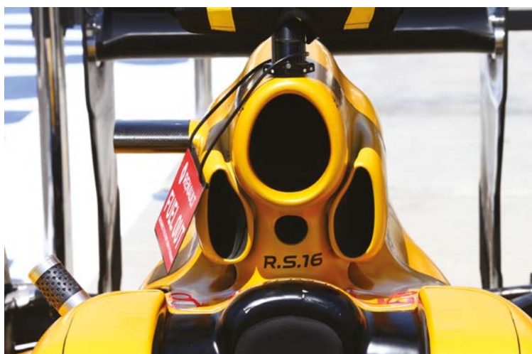
The roll hoop with cooling inlet 'ears'. Renault has leaned on many of the cooling lessons learnt in 2014, when the Lotus ran the then new Renault turbo engine. It now uses air-to-air coolers
