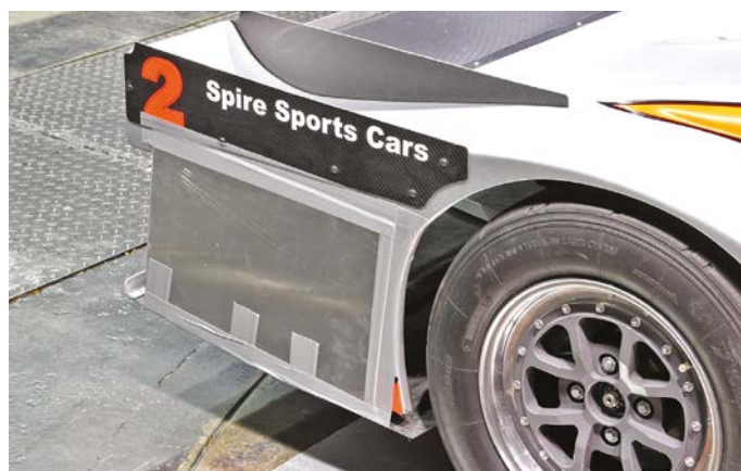
RGB infill panels produced a larger downforce change compared to the Bikesports car
