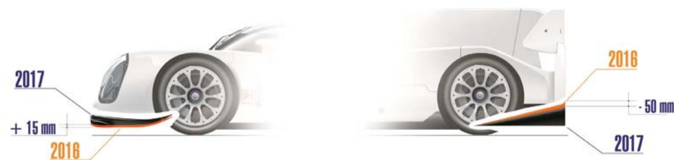
The height of the front splitter will be increased by 15mm on LMP1-H cars while the rear diffuser will be reduced by 50mm
