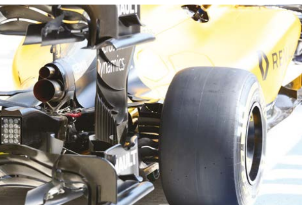
Tail pipe layout with wing pylon support above. The RS16 has just the single wastegate exit pipe, which is largely a packaging solution, while all the other cars in the F1 field use a twin exit
