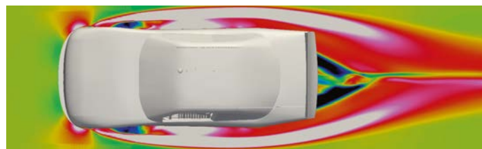
Figure 5: A CFD comparison of a flared fender opening with a smooth fender opening
