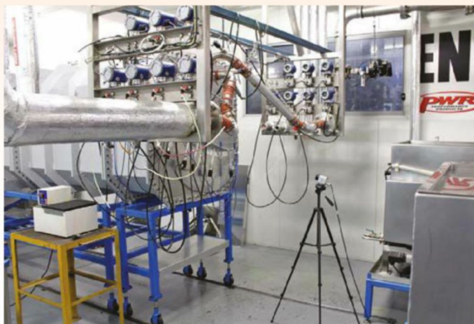
Charge cooler connected to the charge air feed. Temp and pressure sensors monitor conditions; thermal imaging cameras monitor upwind and downwind faces of cooler
