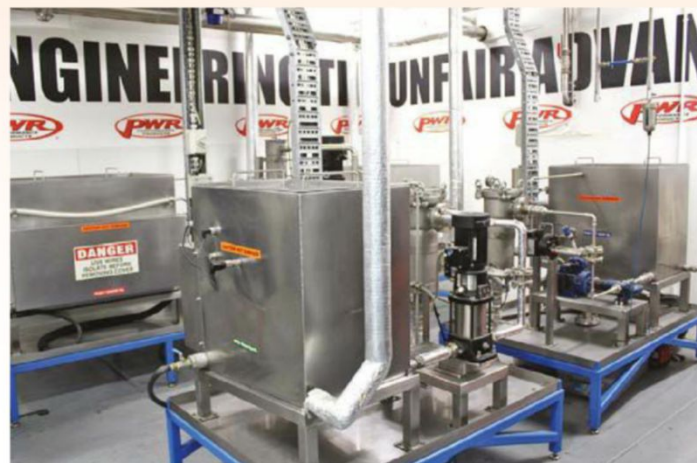
Two heated water circuits plus two heated oil circuits and a single heated charge air circuit are available. It is also possible to test multiple cooling components together
