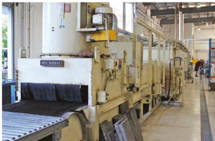
Brazing is a multi-stage process in the CAB. Cores are cleaned and flux-coated first
