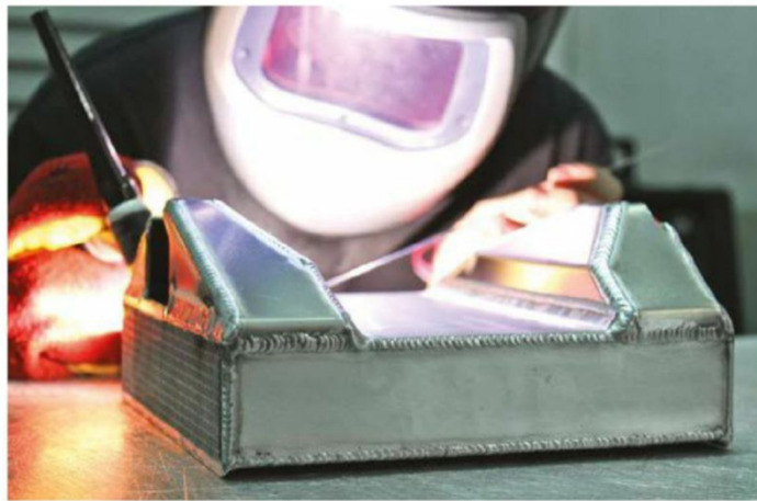
Tank with its integral connections is welded to a core to become the finished product
