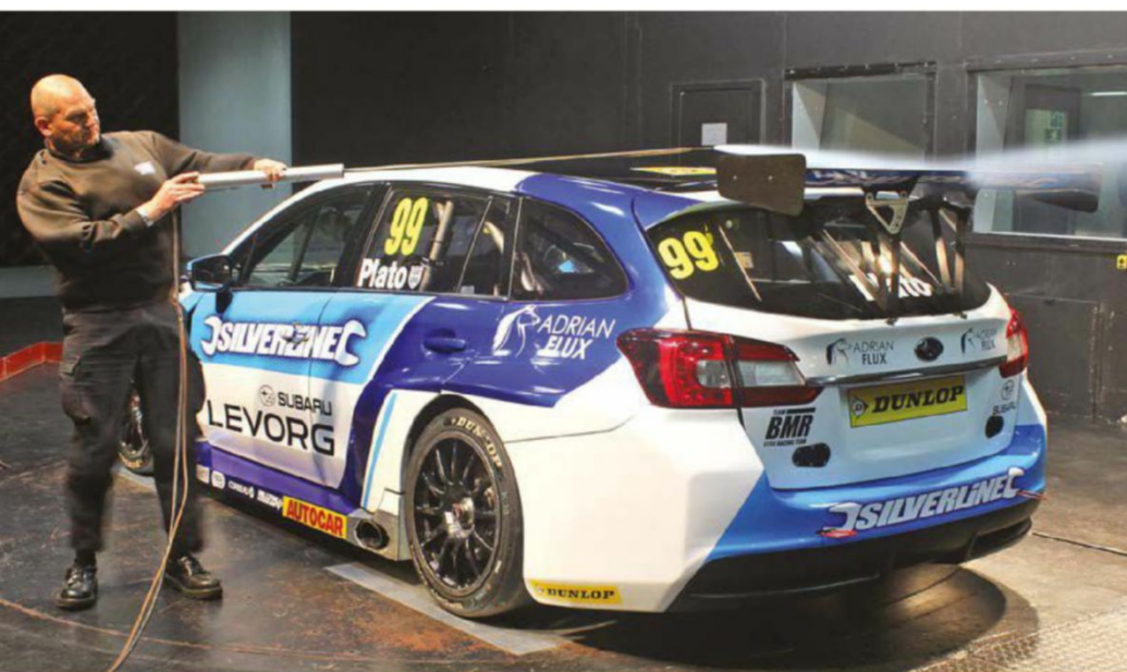
The British Touring Car Championship rear wings are fitted in specified locations designed to put a limit on the maximum downforce working on the rear axle. Rwd cars, like the Levorg, received a slight benefit in this area in the middle of 2013
