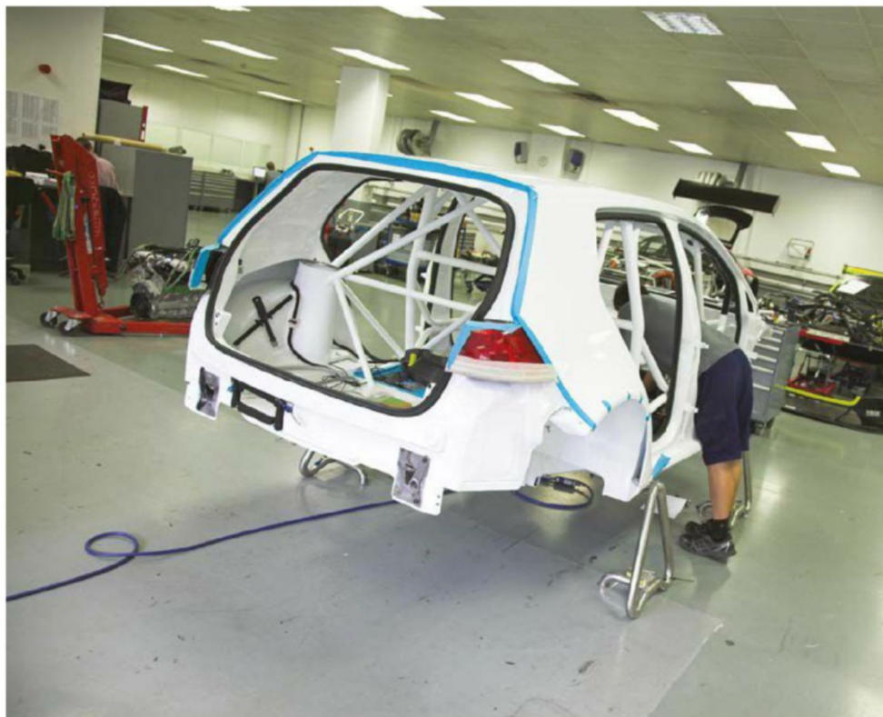
Having access to 3D geometric data of the roll cage, accurate to fractions of a millimetre, is essential to the build process
