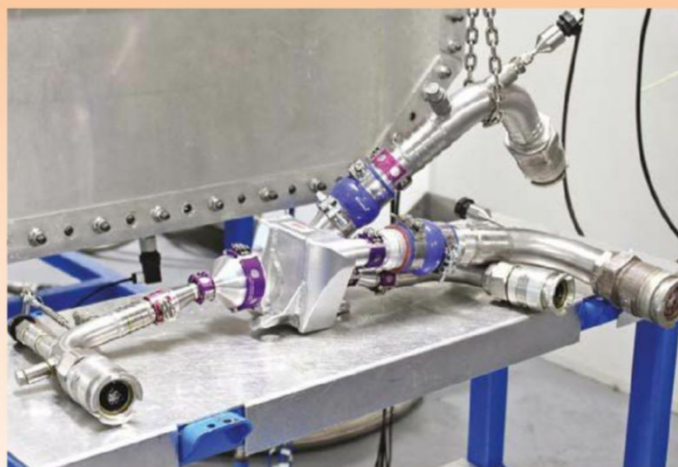
The oil/water heat exchanger being connected to oil and water supplies prior to its test
