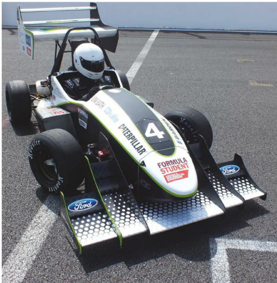
The Bath car has been designed to run with either unsprung aero or sprung aero; the latter shown here at Silverstone. Major aero elements are the big wings fore and aft plus a neat rear diffuser. There's a tube chassis at the rear, a tub at the front
