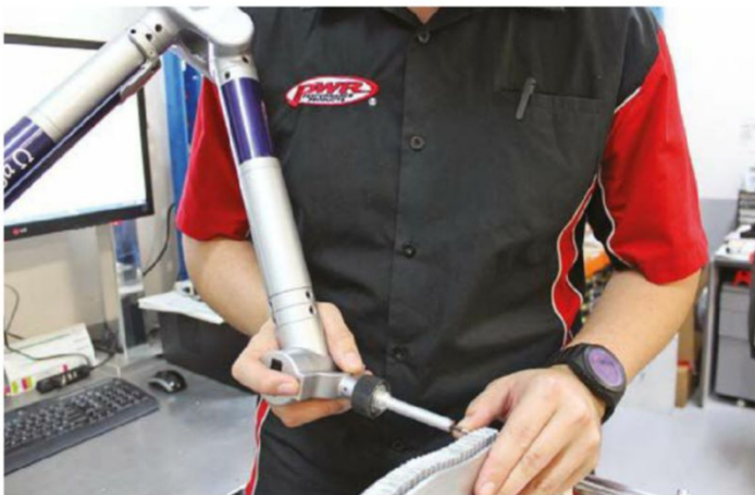
Quality assurance makes use of mechanical and laser coordinate measuring machines
