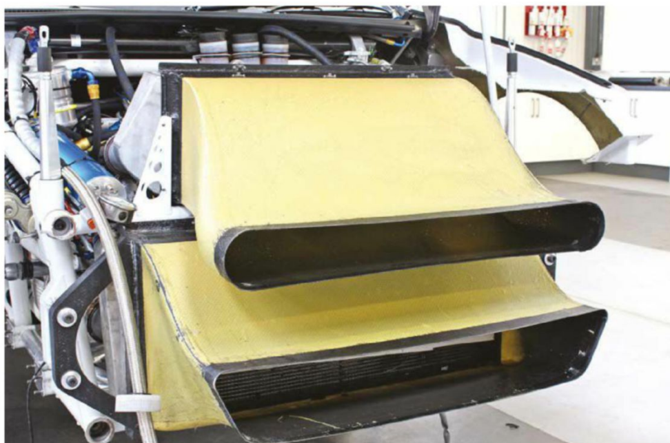
Boundary conditions to model cooling requirements might include vehicle speed and duct expansion ratio. British Touring Car Championship cars use PWR intercoolers – this is the Subaru Levorg's radiator and intercooler inlet duct installation
