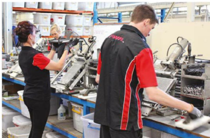
Stacking of fins, tubes and side plates to build up oil cooler cores prior to brazing
