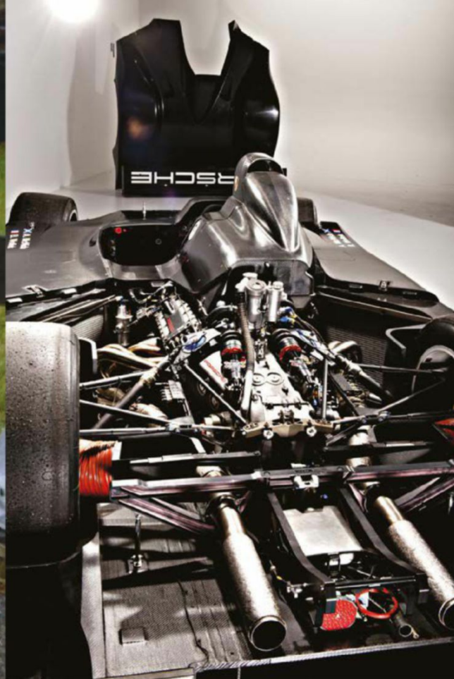
A version of the V10 engine was later used in the Carrera GT. Porsche's existing race engine, the flat six that had seen service in its GT1 98, was thought to be too heavy for this application
