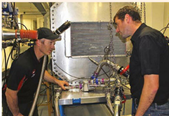
JC (left) and senior engineer Andi Scott confer on the heat exchanger test; note that the water radiator is connected to the wind tunnel outlet to control the water temperature
