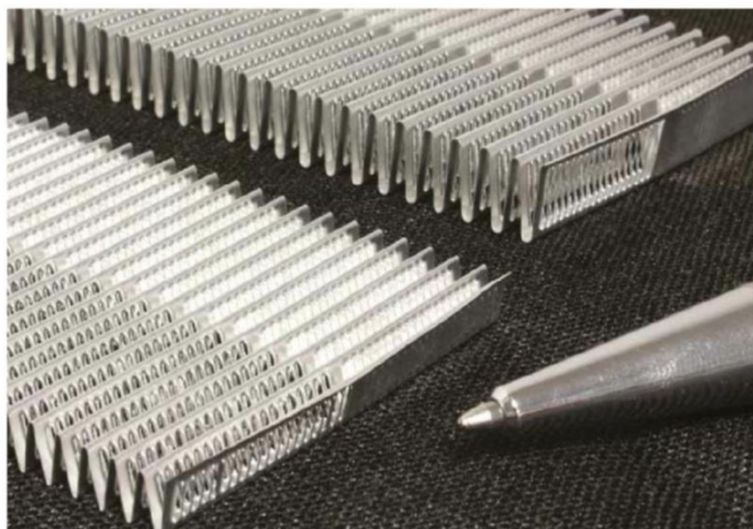
Two examples from the very wide variety of different fin strip sizes and configurations
