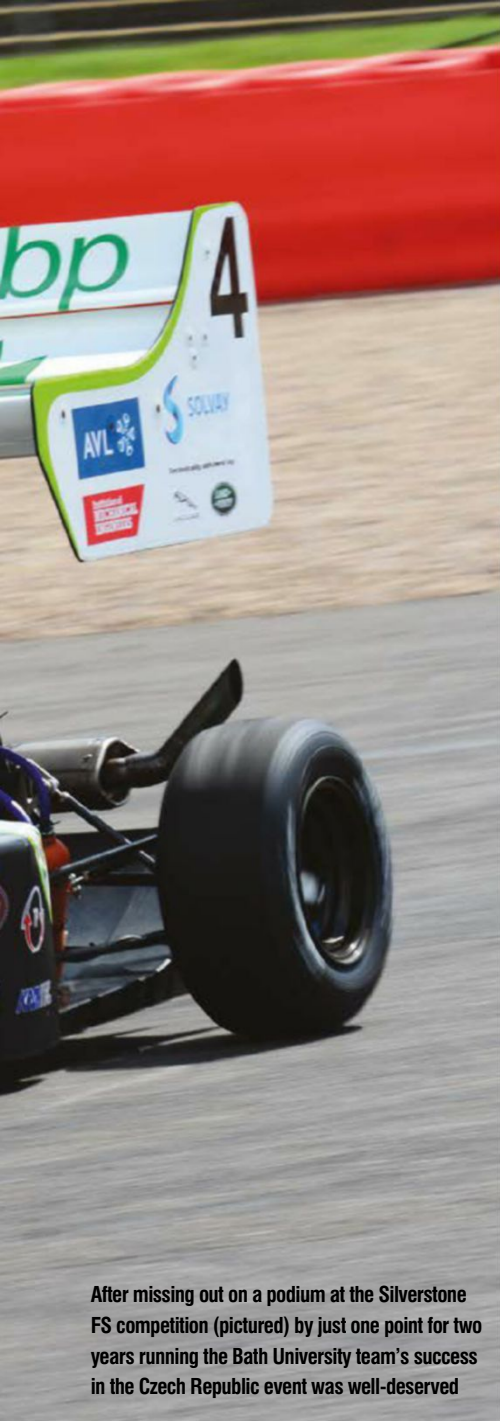
The Bath car has been designed to run with either unsprung aero or sprung aero; the latter shown here at Silverstone. Major aero elements are the big wings fore and aft plus a neat rear diffuser. There's a tube chassis at the rear, a tub at the front
