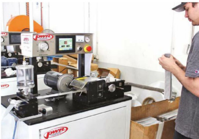
Aluminium strip is converted to concertinaed fin strips on this piece of machinery
