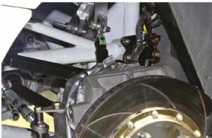
Ride adjusted via push rods (top centre) with nuts pre-slackened for rapid adjustments
