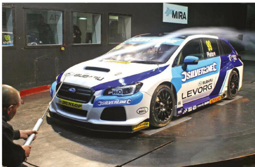
Team BMR's Subaru Levorg. The racecar's designer says drag is the most important aerodynamic parameter in the BTCC
