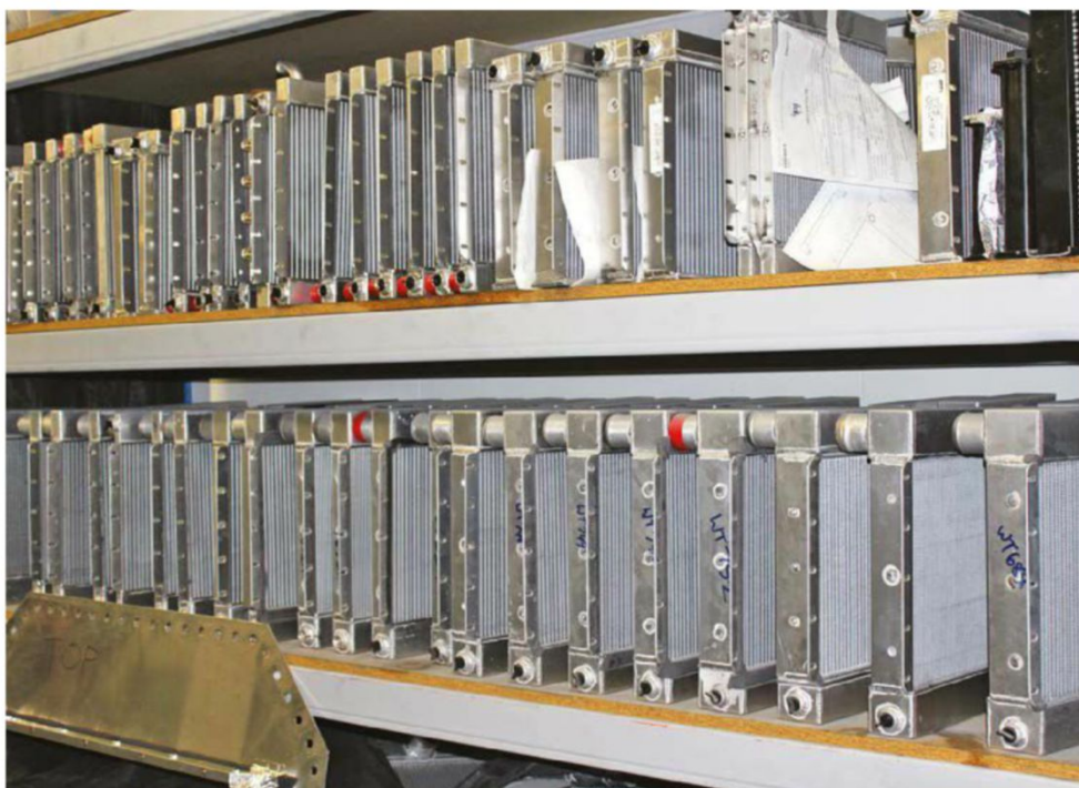
A small part of PWR's library of samples for all cooler types. This contains hundreds of different cooler core configurations
