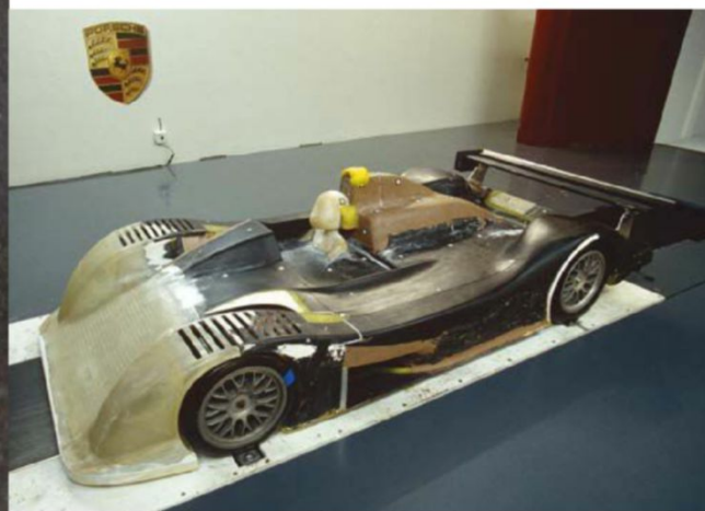
The aerodynamics were developed by Norbert Singer with 1:3 models in the rolling road model wind tunnel at Weissach. It was old tech but Singer knew it well and could get useful data from it
