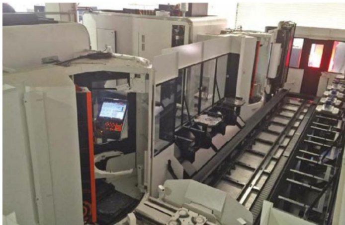
The company's new multi-pallet 5-axis machining centres have increased capacity
