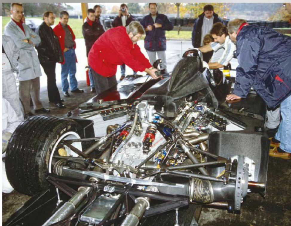
The suspension was conventional at the rear with double wishbones and pushrod operated spring/damper units horizontally arranged on top of the gearbox. The front was the same but with the spring/dampers located vertically in the bulkhead
