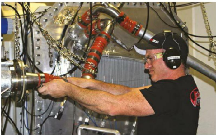
Julian Conlan (JC) completing the installation of a charge cooler which is to be tested
