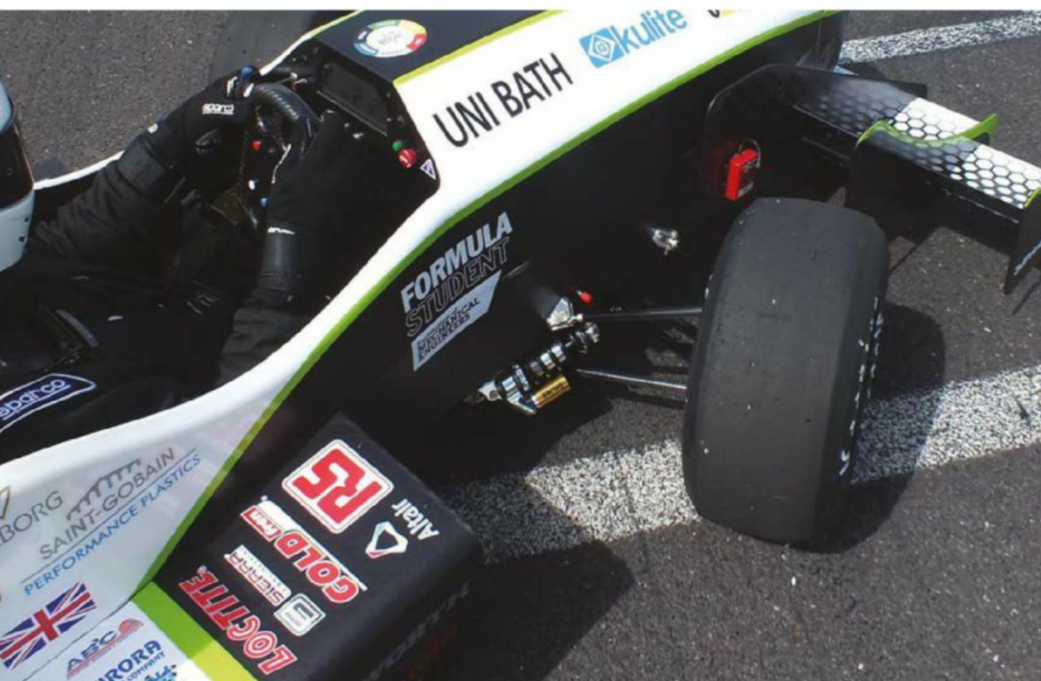
The team opted for a conservative approach to the suspension, reasoning that a double wishbone layout gives good camber control in bump and rebound without the complexity of multi-link suspension. It's pullrod up front and pushrod at the rear
