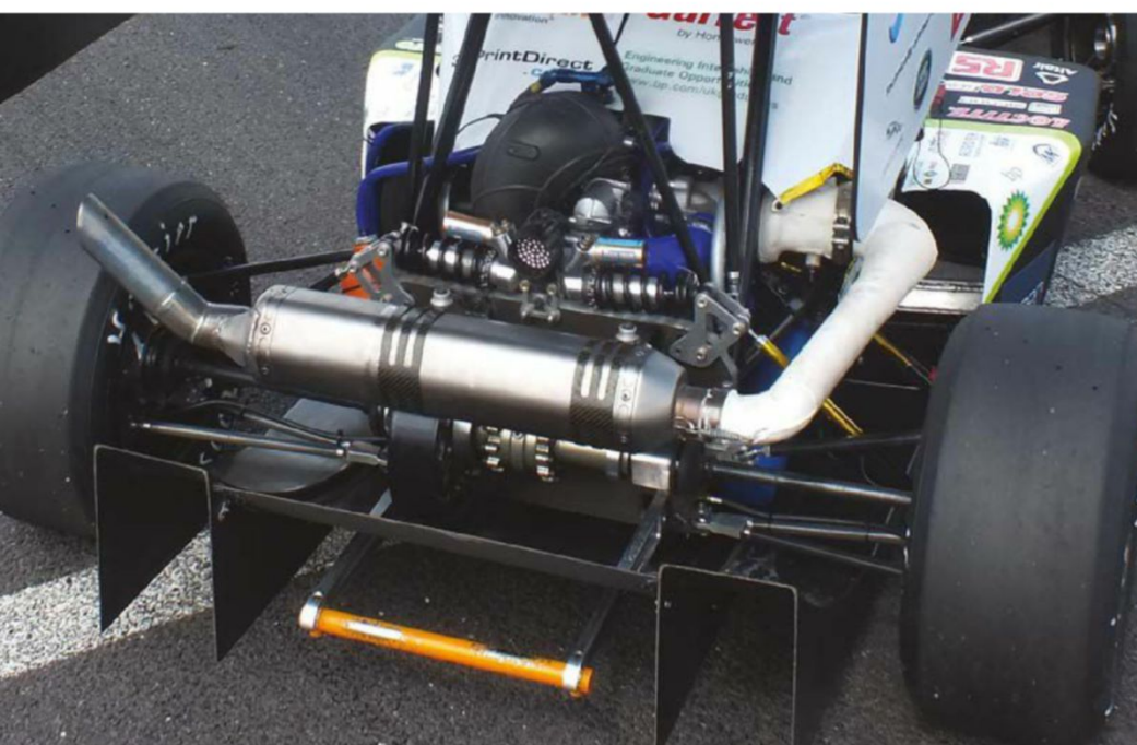
Bath chose a turbocharged internal combustion power unit over electric. The engine is a single-cylinder 510cc KTM EXC, more commonly found propelling an enduro race bike, and it was chosen because of its light weight and proven reliability
