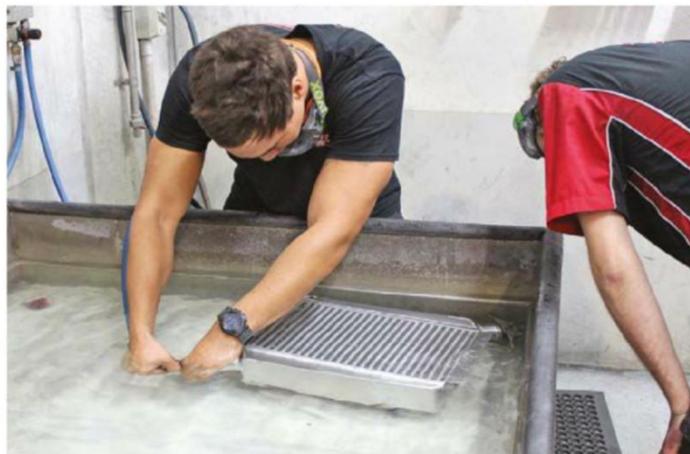
Pressure testing of a welded cooler in the water bath to make sure it's perfectly sealed
