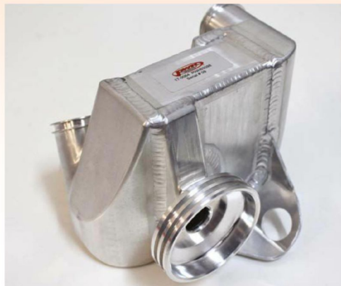
Oil/water heat exchangers (above) can also be tested here. This one is from a rally car
