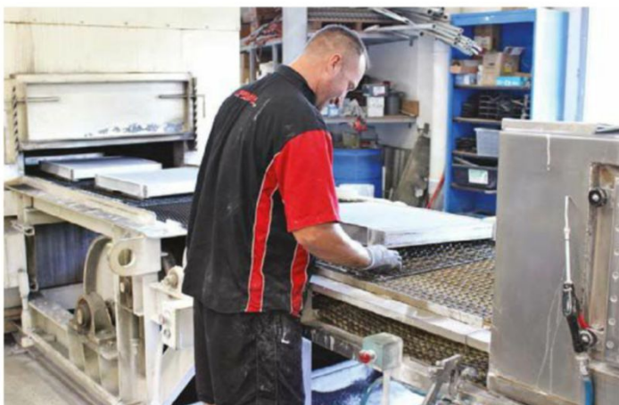
Loading the 'controlled atmosphere brazing' or CAB furnace with clamped core stacks
