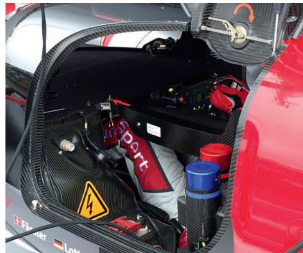
The battery is mounted high in the nose of the Audi R18, by the drivers' legs, in an effort to move weight further forward
