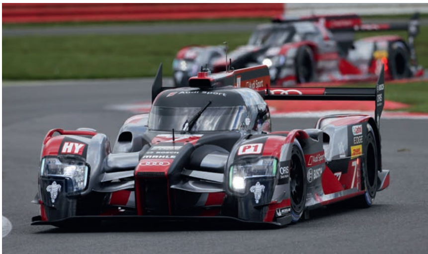
Audi's R18 has changed radically for this year. The cockpit has been moved back to free up space at the front, and air is now channelled through the racecar, while a greater aero emphasis is now placed on the front wing
