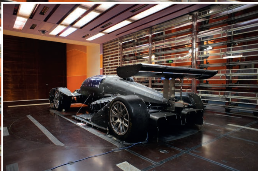
The radical prototype was initially tested in the wind tunnel without some parts of the bodywork in place. The car's aerodynamic concept is based on a single seater and it will also make use of some active aero devices
