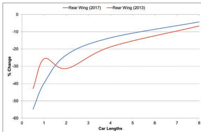
Figure 15: Comparison of changes to rear wing downforce on the racecar following another. Rear wing losses were generally less on the 2017 car than the 2013 car
