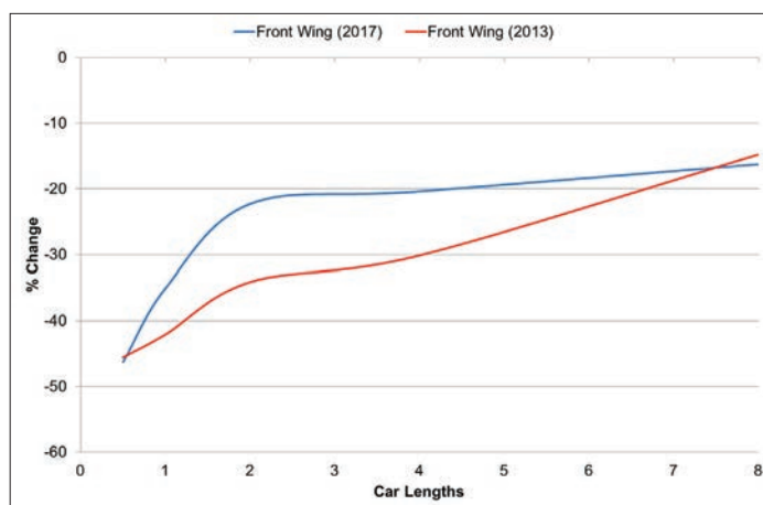
Figure 14: Changes to front wing comparison. The following 2017 car lost a lot less downforce at all the intermediate separations, which should make it easier for the driver
