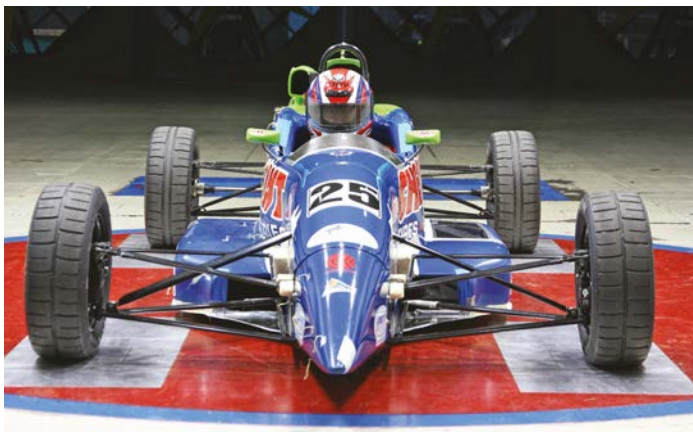
The Spectrum we tested back in 2007 had lower overall drag than the earlier Swift despite the presence of those wider sidepods, which house lateral intrusion structures
