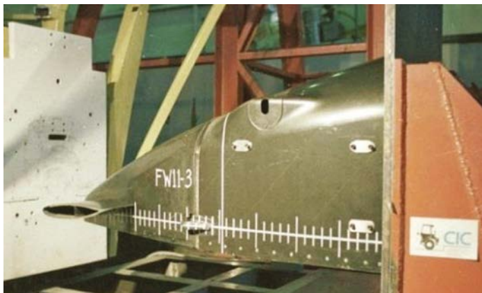
A Williams FW11 F1 nose-box in 1986 testing, moments before it takes the impact
