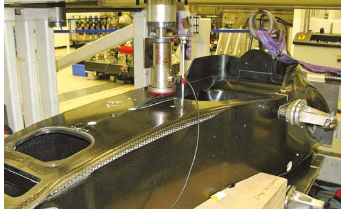
The front roll protection structure on the Williams chassis is subject to a 75kN push test
