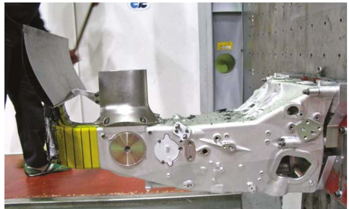
Rear impact structure after the test. The effectiveness of the deforming area is clear
