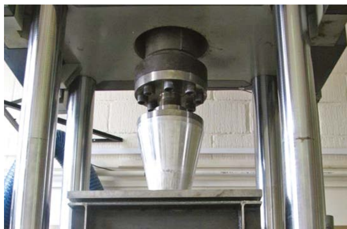
The panel penetration test rig with its a solid metal cone, designed to act as a nose-box
