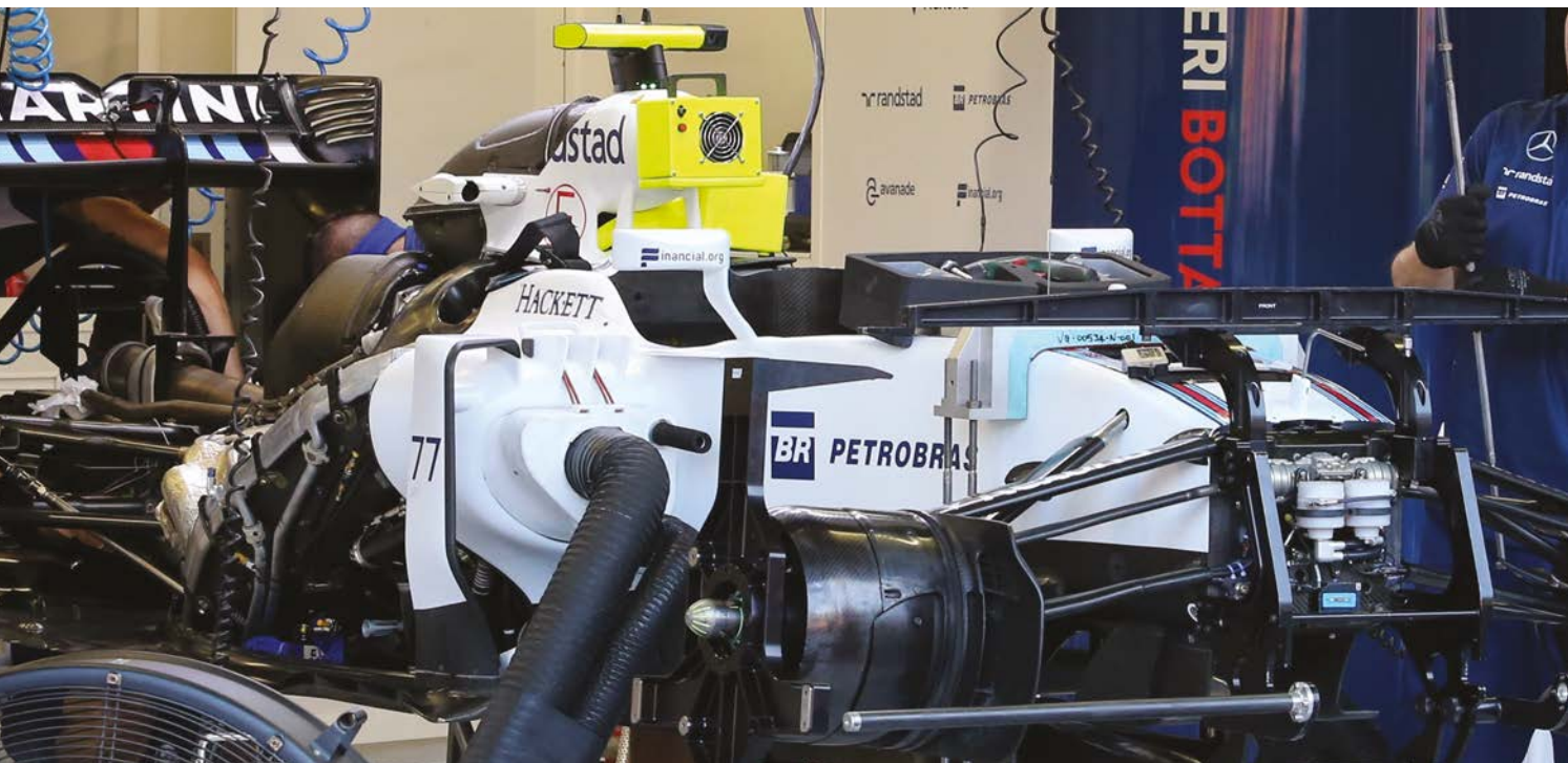
A half naked Williams FW38, showing pull rod rear suspension and the very neatly packaged cooling system. The car is in many ways an updated FW37, but with many refinements
