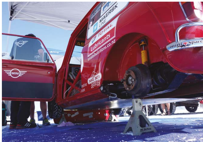
Suspension was the Hi-Lo adjustable rubber coned system that was used on all early Minis, but with new uprated shock absorbers added. The body and chassis was near-standard, with a flat floor and undertray
