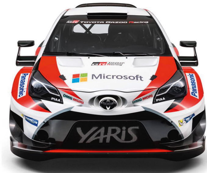
The splitter has received much attention. Thanks to the allowance of multi-layer carbon for aerodynamic devices this is now strong enough to survive the rough special stages
