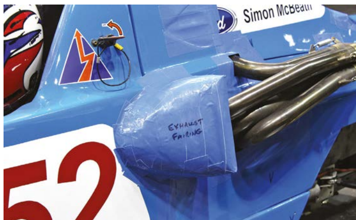
A fairing positioned ahead of the exhaust actually seemed to cause a small drag increase
