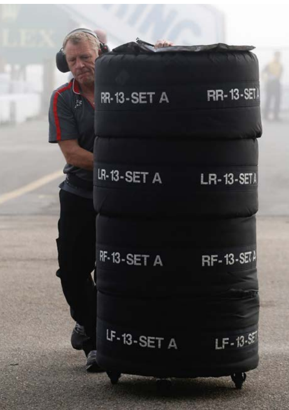
Rebellion brought new tyre blankets to Sebring to replace the ovens that are more traditional in endurance racing. It wanted to use the test to establish the warm up times for the new season
