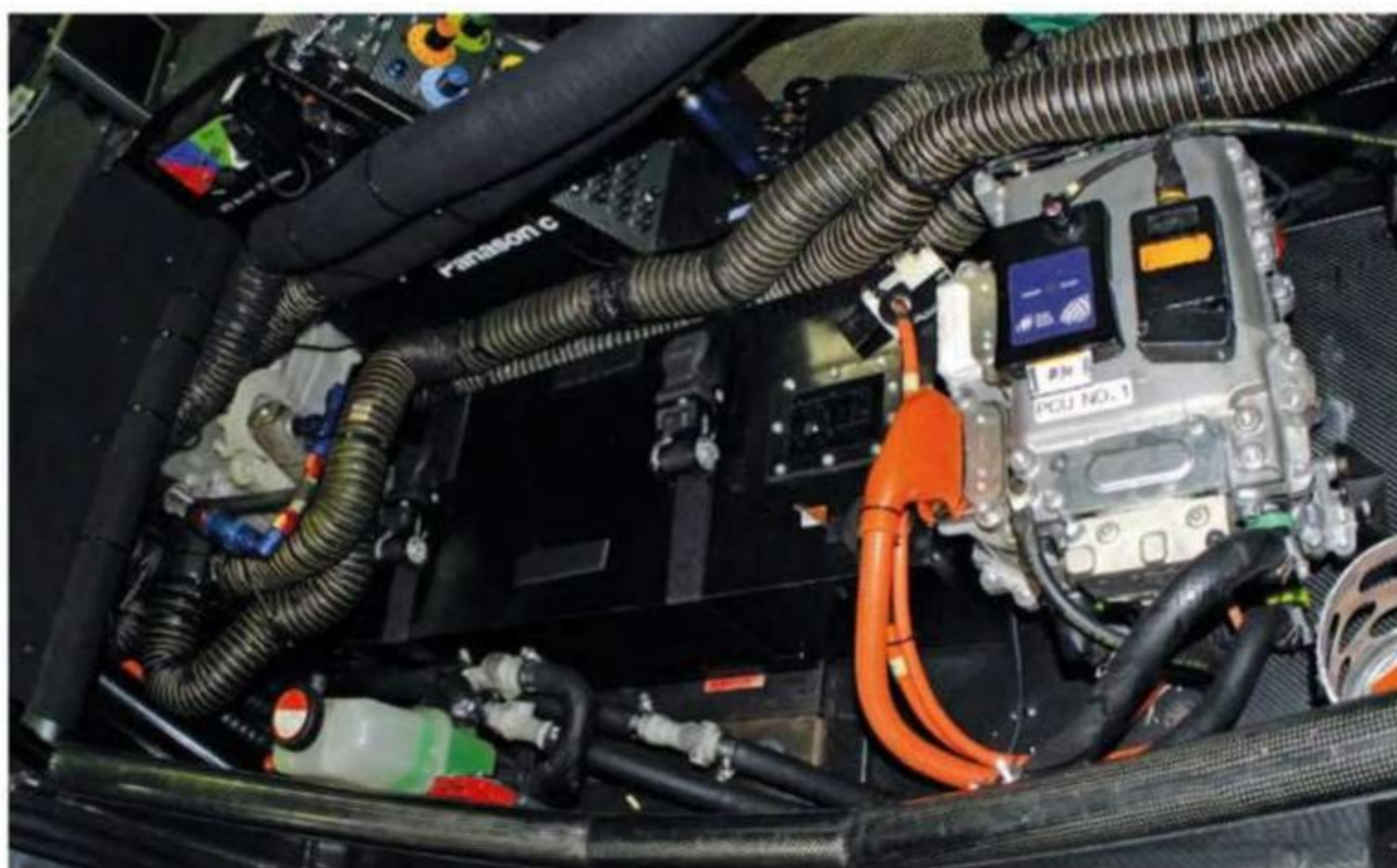
Hybrid system PCU (the silver component) is mounted in the space passenger seat would normally fill. It's from a road car but is mated to a Pectel ECU. The black battery pack is also visible; casing is bespoke but cells are from the production car
