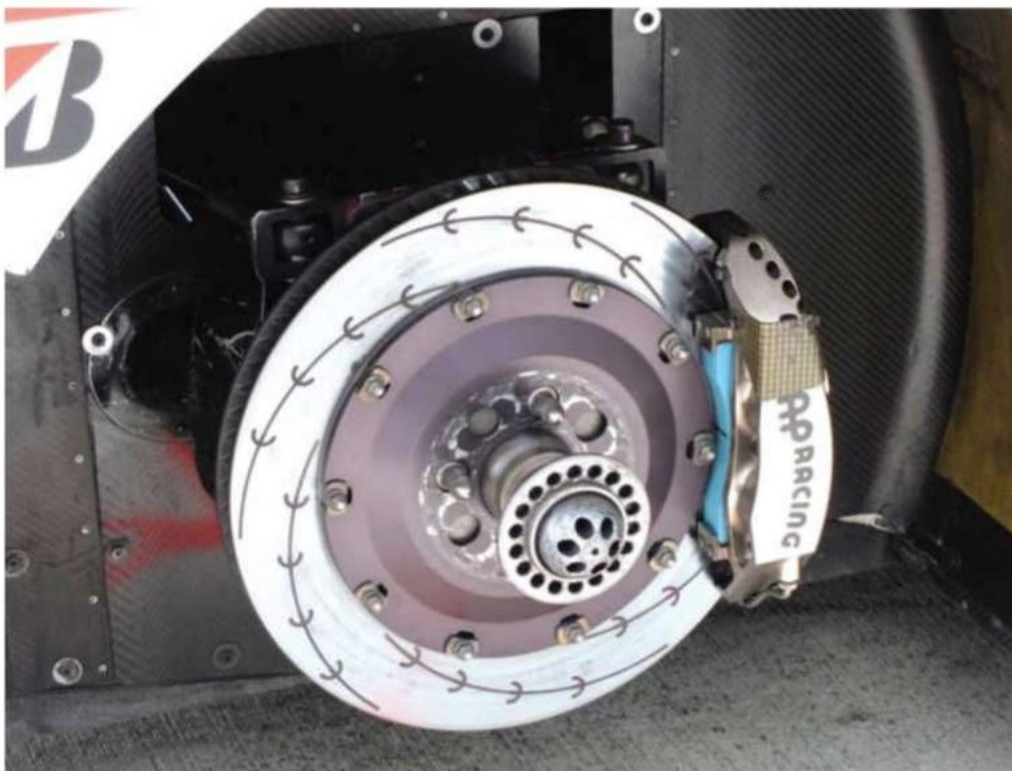
AP racing brake calipers were previously used in GT500. There's no link between the hybrid system and the braking system
