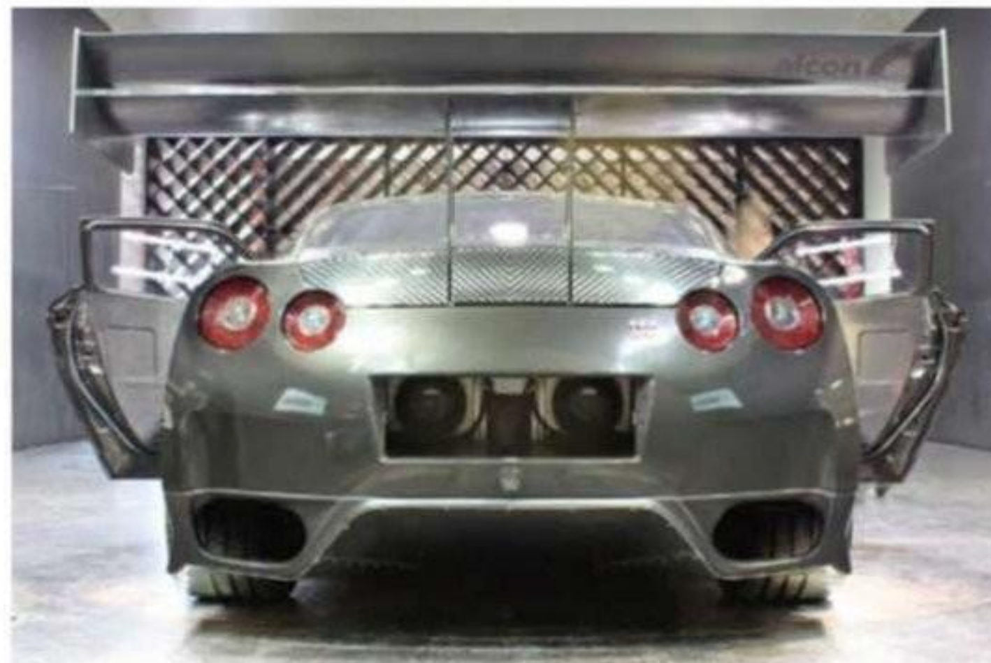
The rear wing dominated the early runs and was over-powering the front end of the car
