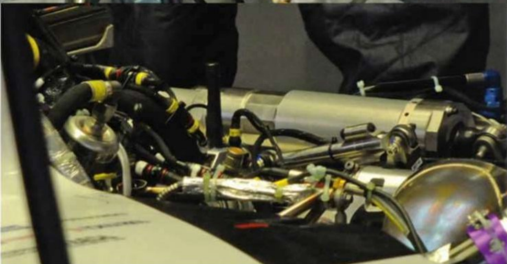
The cylinder on the rear suspension sits transversely across the gearbox in preparation for a third ERS
