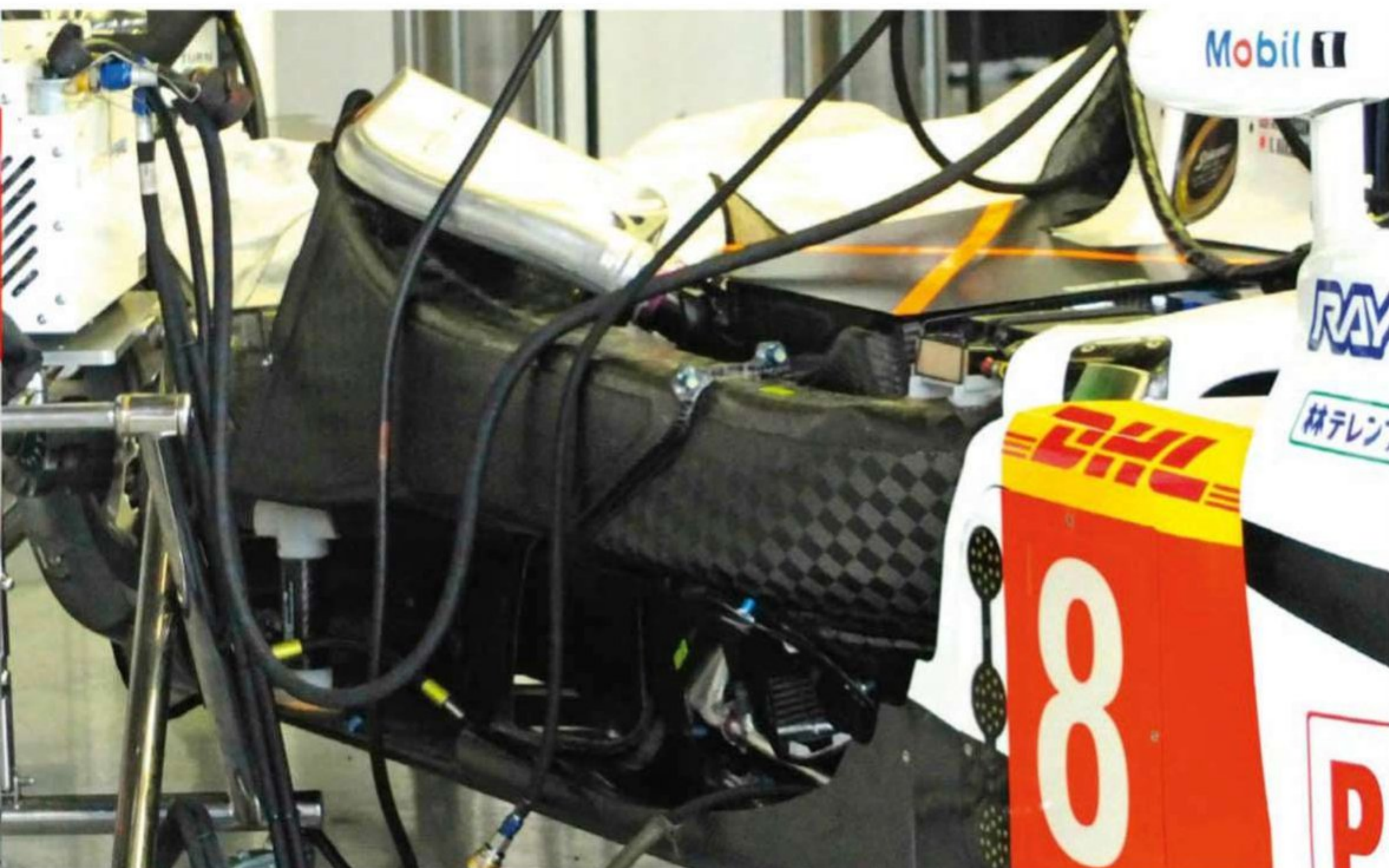
Note airflow routed upwards from the sidepod, and the tight packaging which is a stand-out feature of the revised TS050
