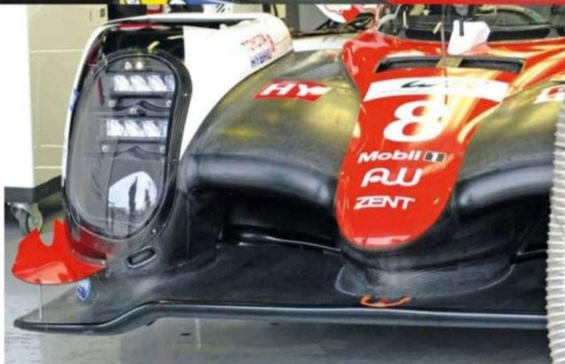
The TS050 focusses on though-car airflow, hence the high nose treatment. The front impact structure is new
