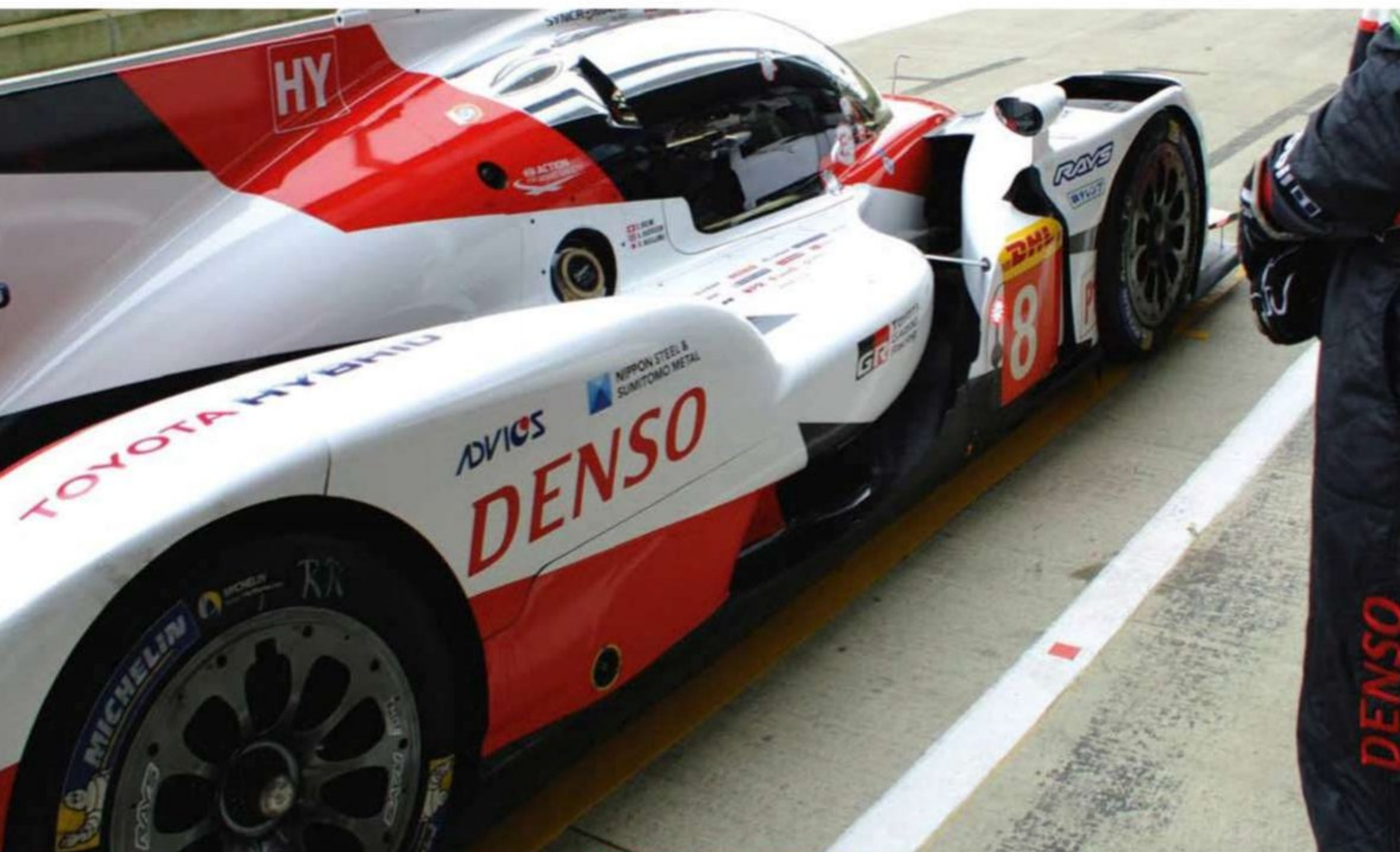
Sidepod shape from rear showing interaction with front wheel pod and nose ducts. Toyota says aerodynamic efficiency has improved
