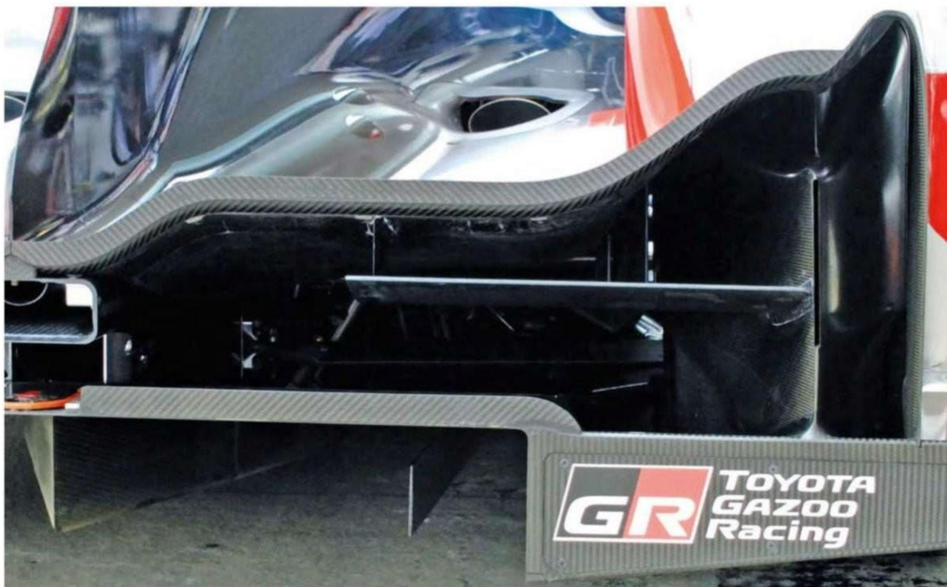
Toyota diffuser and engine cover. Note daylight entering from the side and the air jack hole in the floor. Further aero benefits have been found with the battery, which requires less cooling
