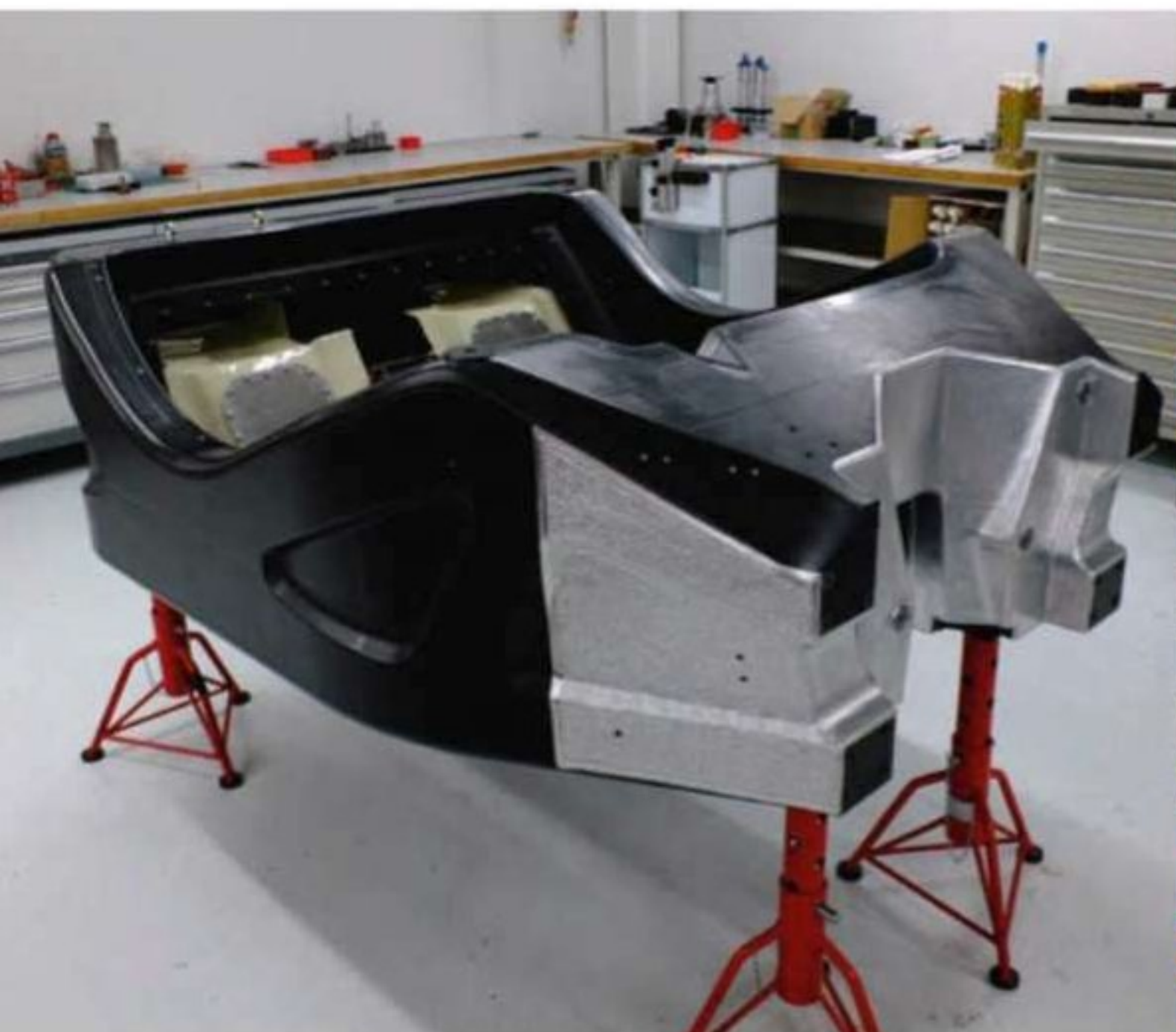
Mother's heart: the MC chassis showing Fuel Safe fuel cell. The Dome-developed monocoque uses coreless design and is said to be stiffer than the GT500 chassis
