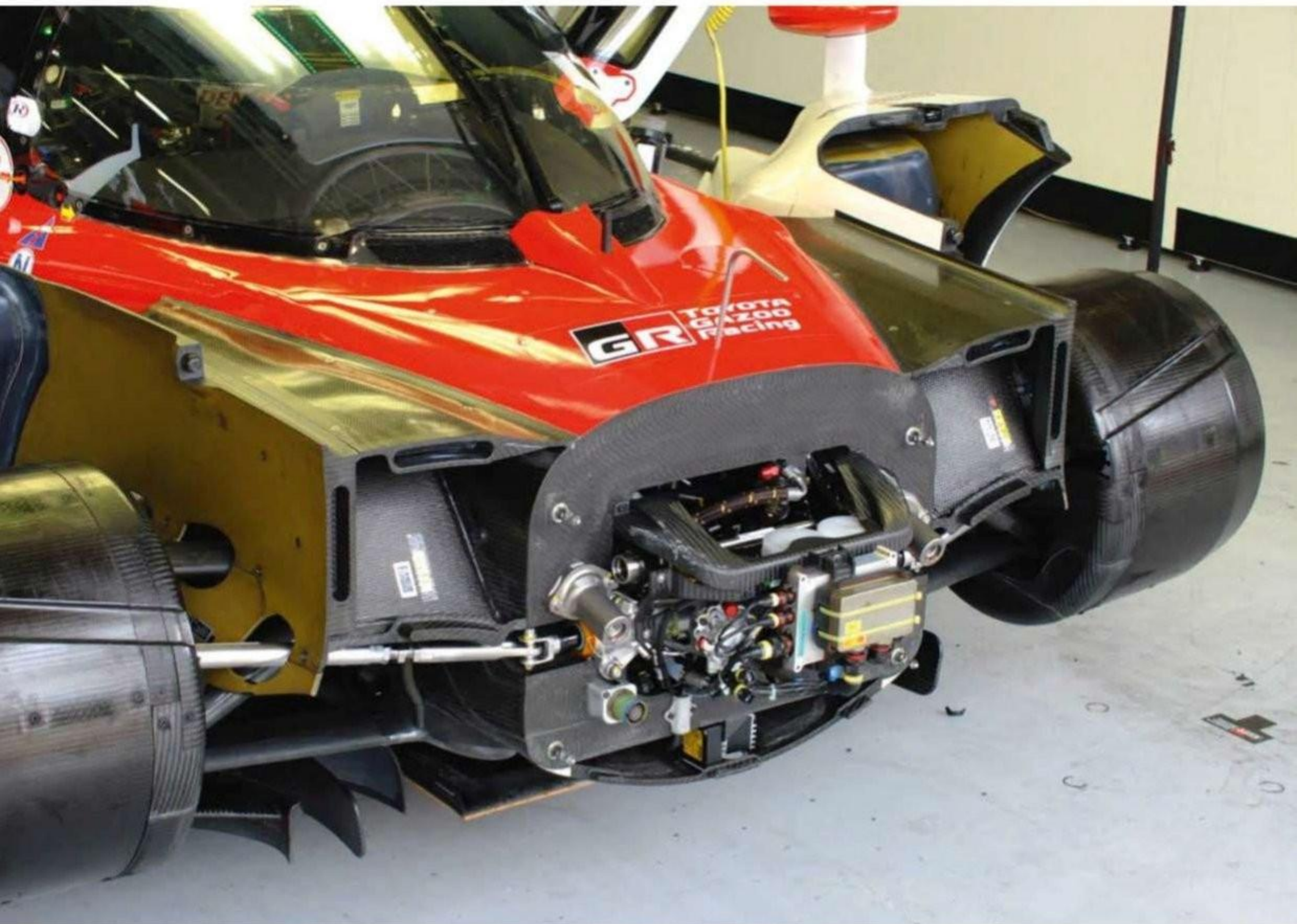
Front bulkhead. The monocoque carries over from 2016 which has restricted development of the front suspension. Porsche and Toyota have agreed not to develop chassis until 2020
