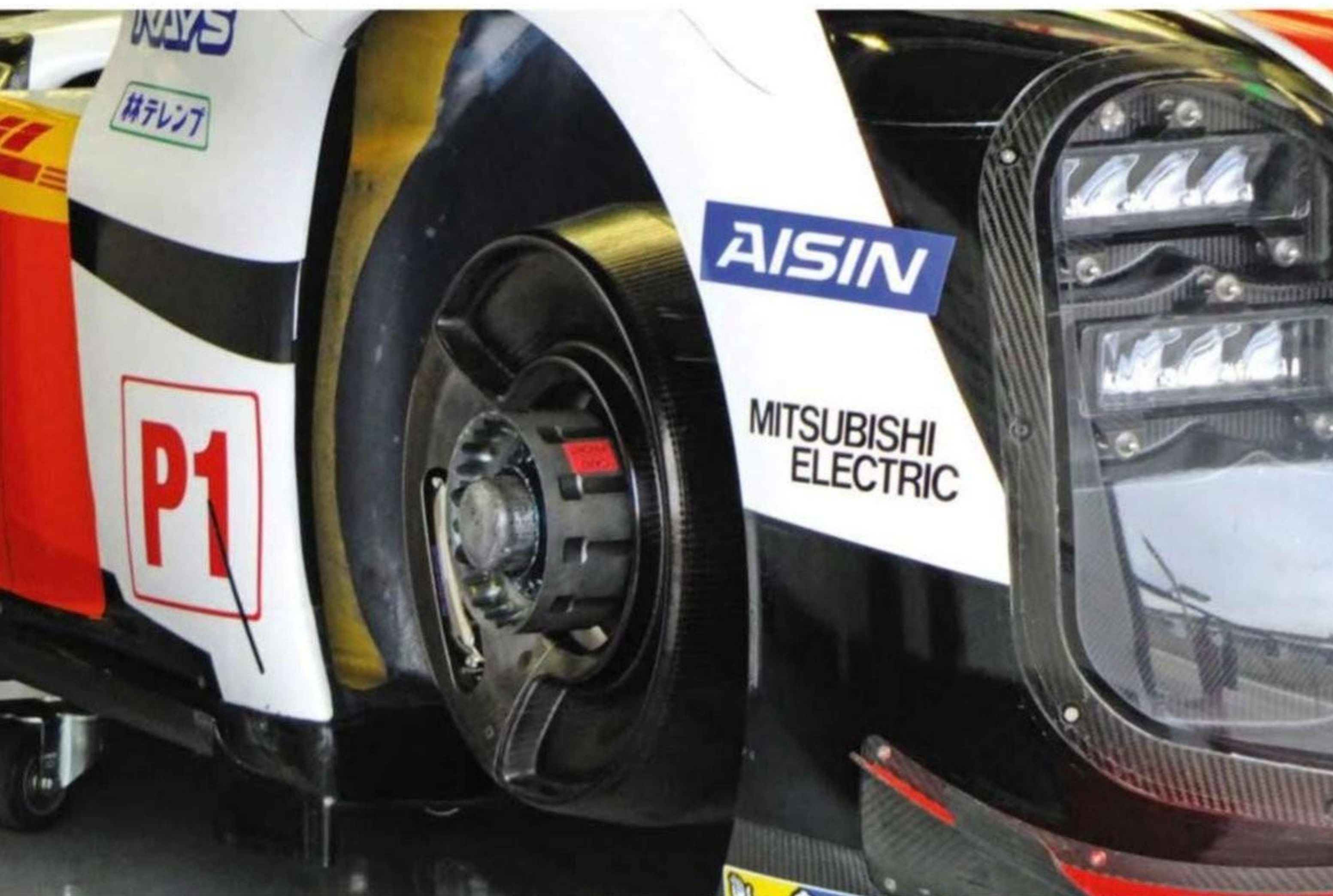
The front brake uses Akebono mono-block light-alloy calipers and ventilated carbon discs. Pad material changed mid-2016
