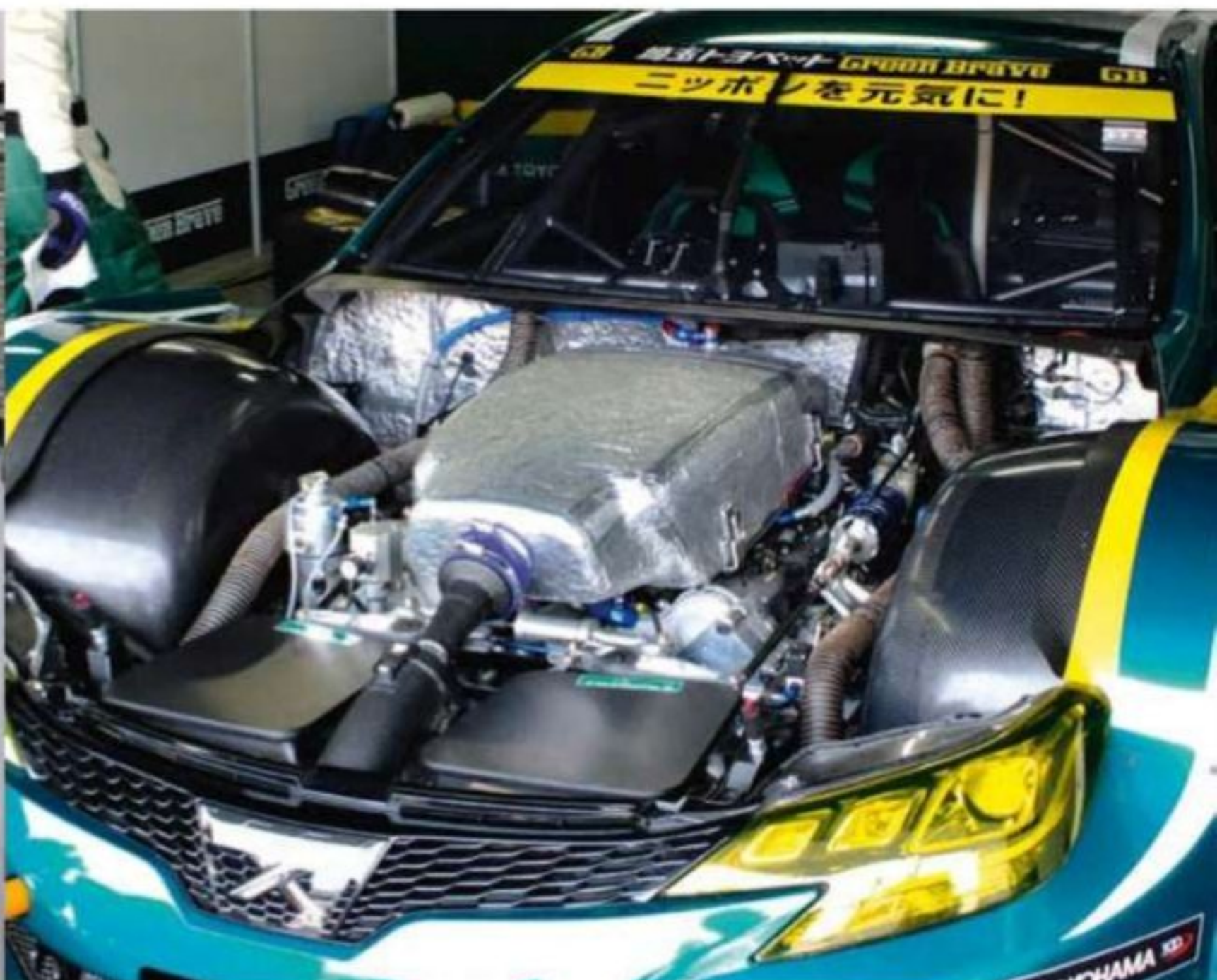
The 4.5-litre GTA engine is spec issue for Mother Chassis racers, but with the entry of the Mark X the supply of this unbranded unit has now dried up. Promoter GTA is looking for a new source
