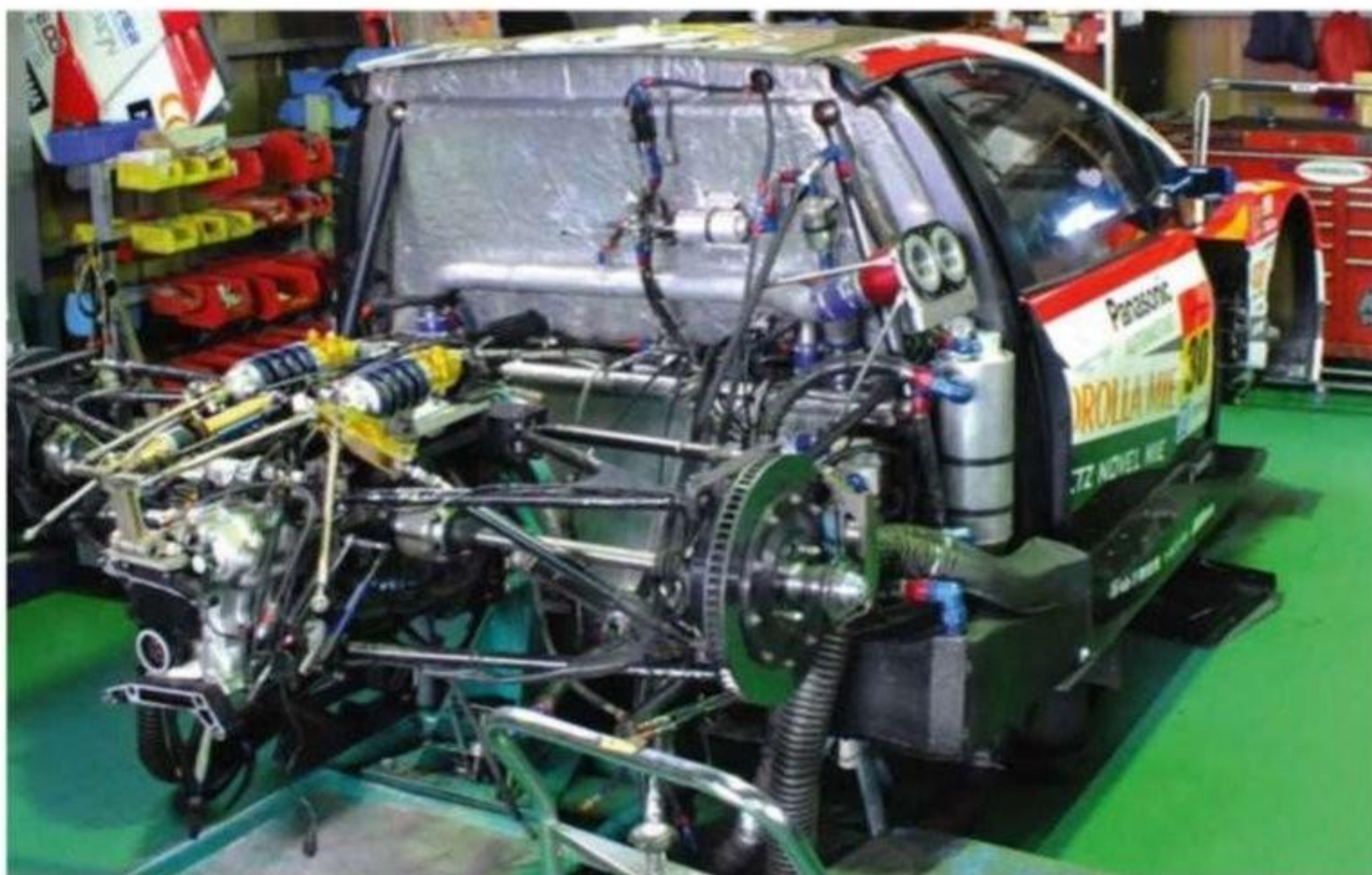
Number 30 car being prepped for first race of 2017. The 3.4-litre normally aspirated Toyota V8 RV8K engine has been used at the very highest levels of racing, including LMP1. Regulations allow the use of any engine from the manufacturer's range
