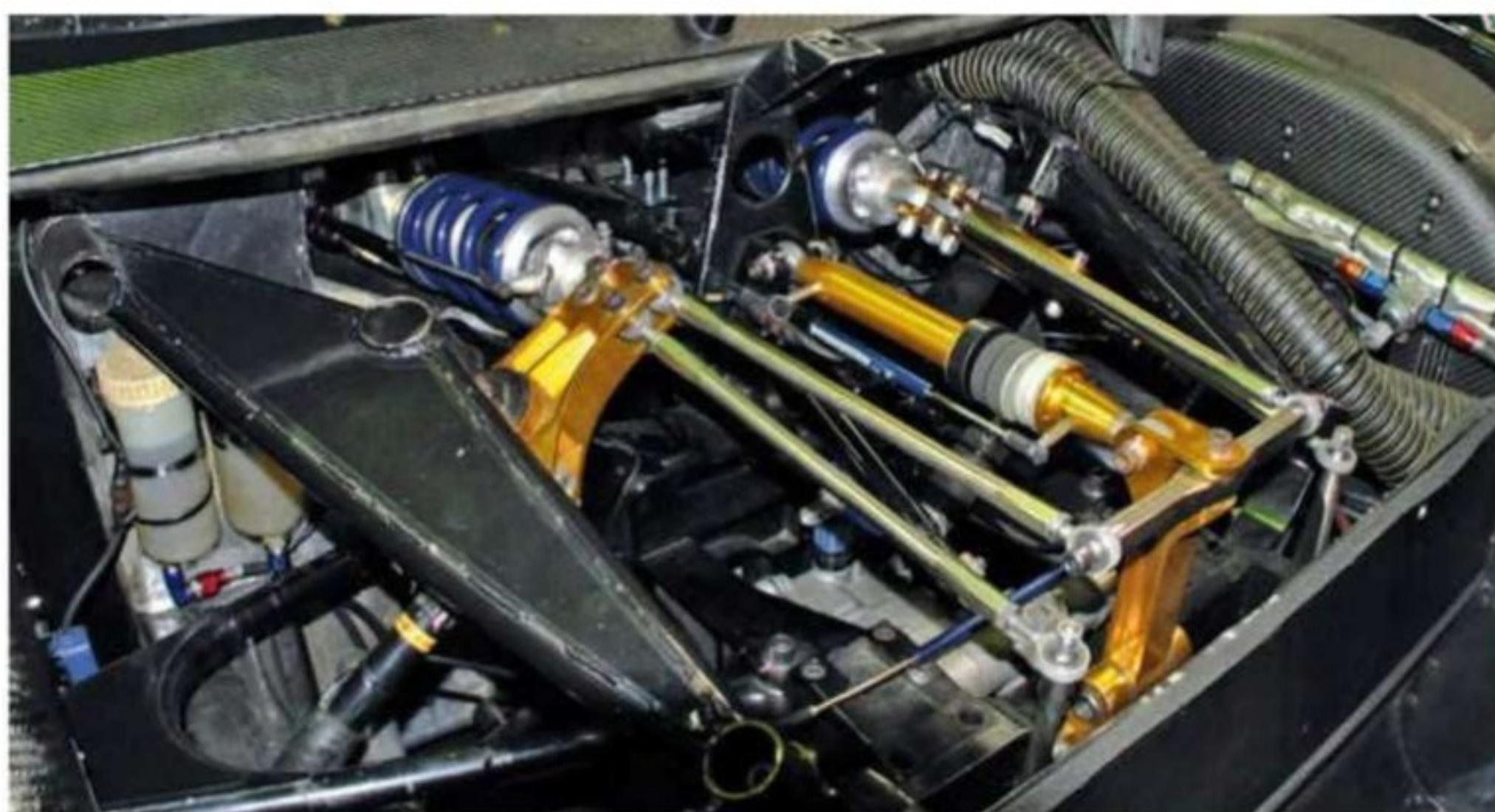
Front suspension. The car uses a third element on front and rear. Geometry differs on both cars due to use of different tyres
