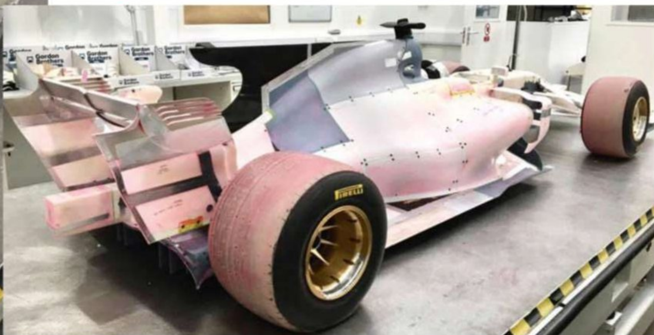
The pics seen here are the first detailed images of the 60 per cent model of the MRT06. Like many of the 2017 F1 cars the Manor would have used a dorsal fin, which is to help with stability in yaw. Its fin is not as large as those seen on other cars
