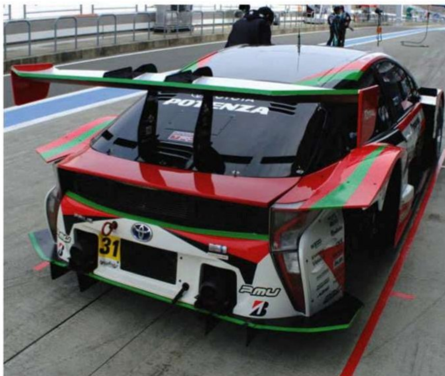
The rear wing concept on the Prius dates back to the MR-S. The swan neck supports come from the previous generation Prius and they also bear a resemblance to the aero approach of Super GT's technical cousin, DTM
