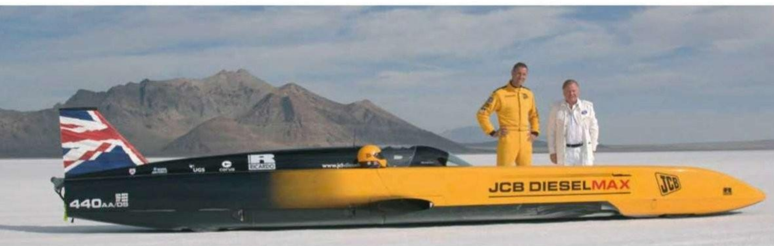
Andy Green (left) says the Dieselmax was fully controllable for each run, even at peak speeds of 365mph. The fin at the rear of the projectile is for yaw stability at high speed
