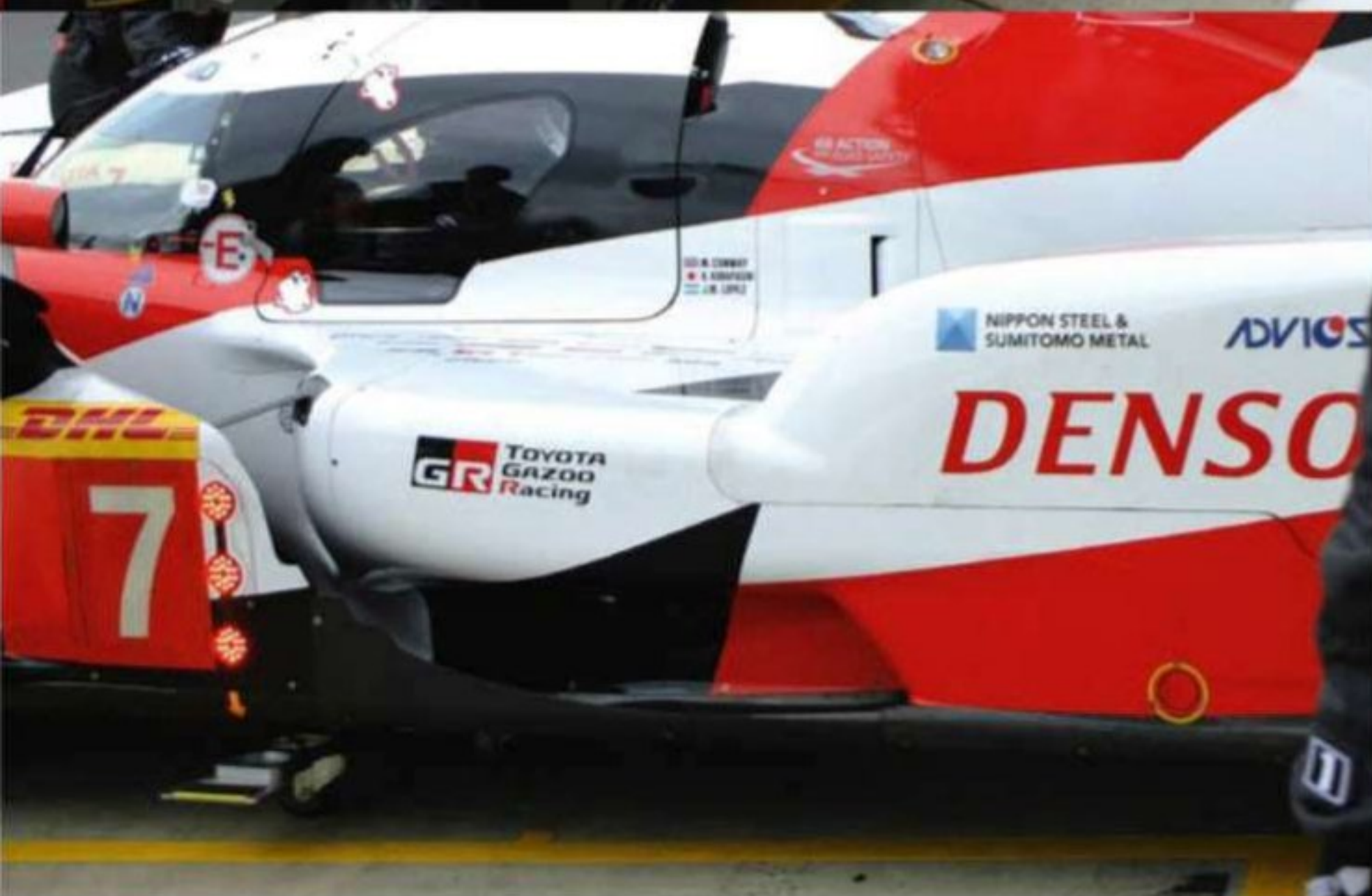
Sidepod undercut. Note the duct under the D of Denso. This feeds directly into the volume above the diffuser
