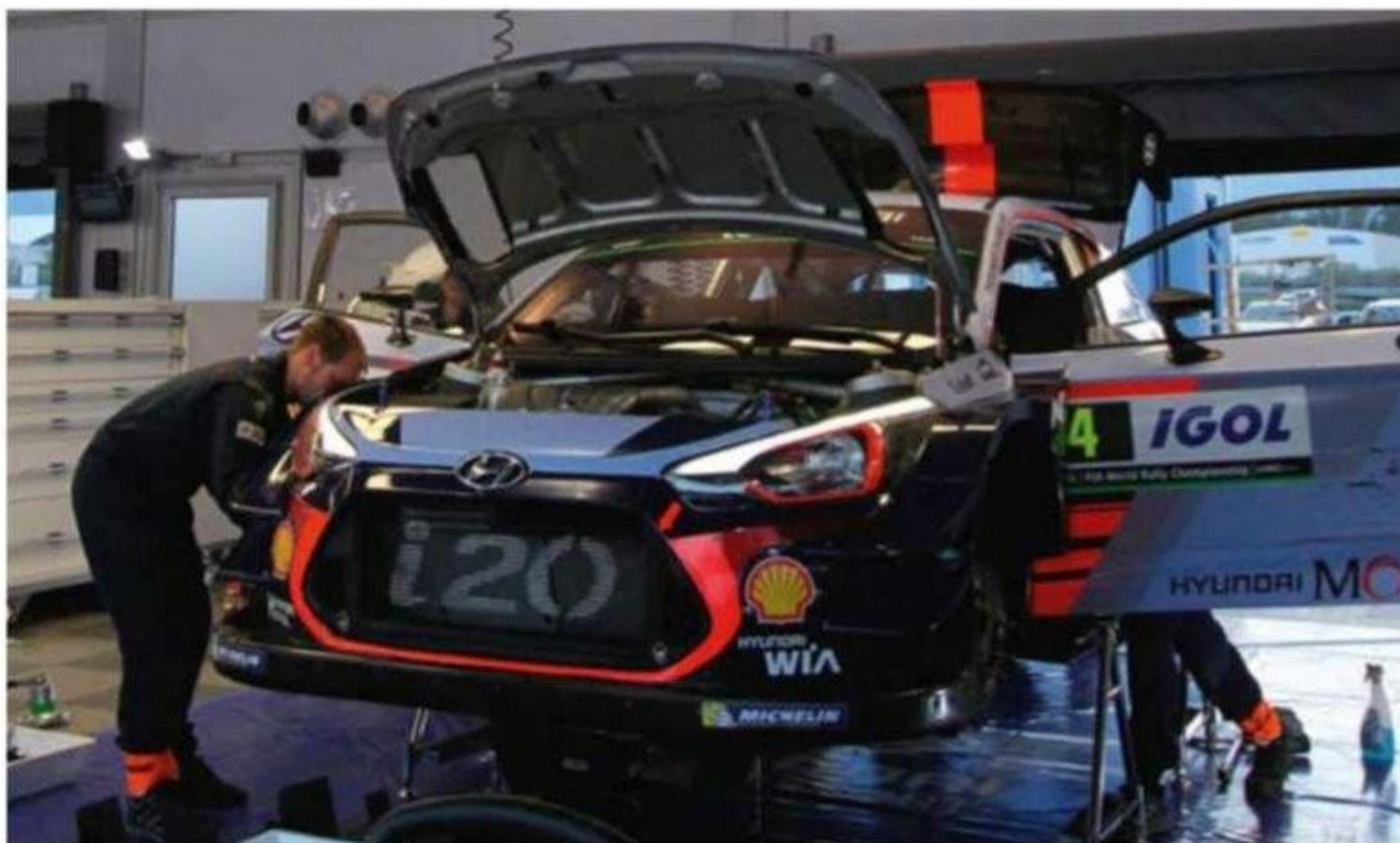
Front wheel arch area has been redesigned because of new suspension rules. Engine has new head and gives more power
