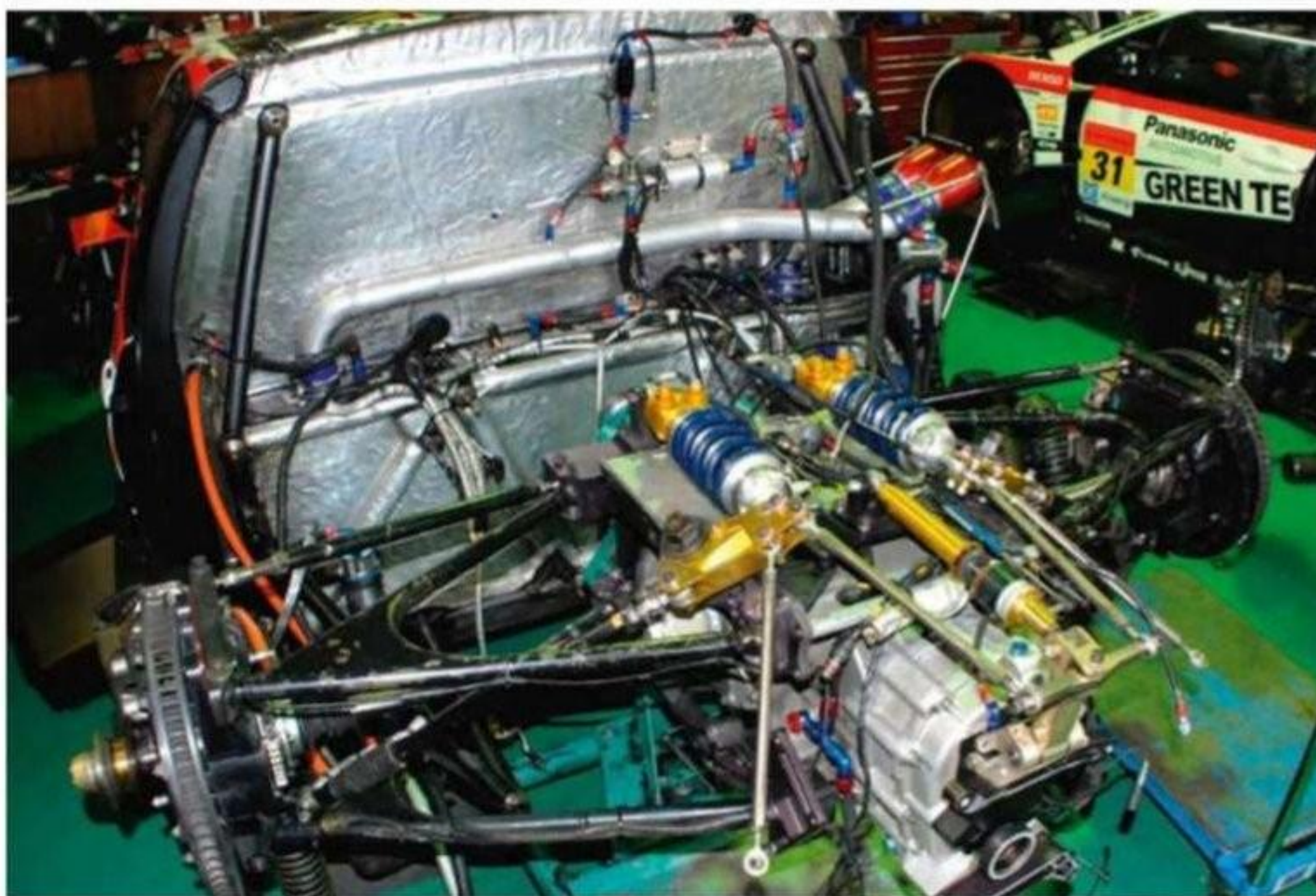
Gearbox is a Hewland NLT. The apr team is beginning to have some problems sourcing parts for this tough transmission
