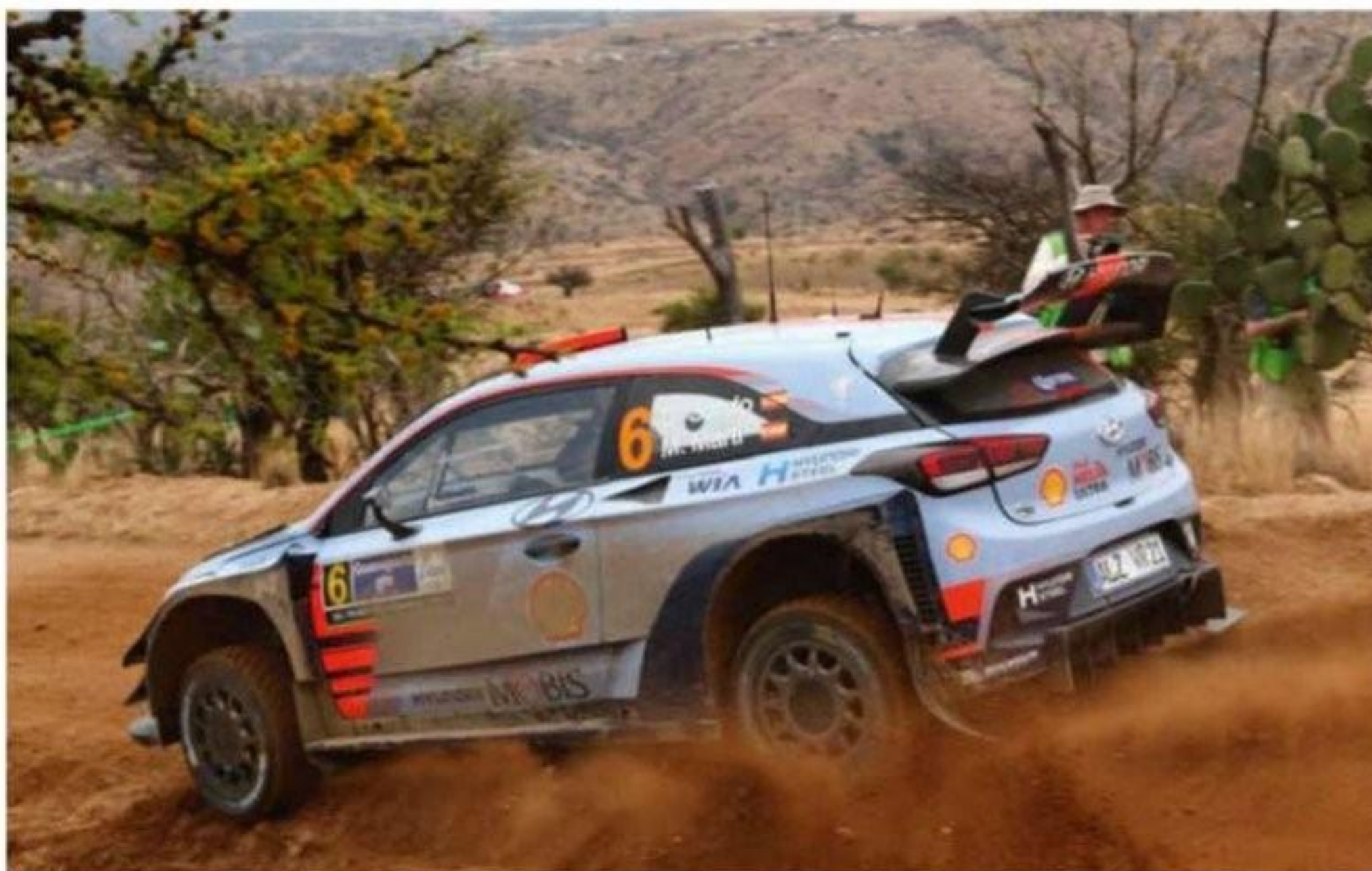
The new aero package, including flick up rear wing, has been designed to be tough enough to survive rough WRC stages
