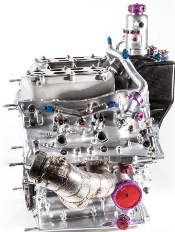
Much of the development has been focussed on the tiny V4 internal combustion unit that sits at the heart of the 919, Porsche working on its reliability, performance and efficiency
