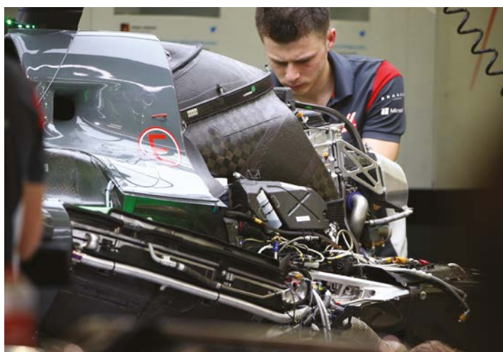
The power unit installation in the VF-17. The way Haas has worked with Ferrari has been an undoubted success, to the extent that other teams are looking at using this approach
