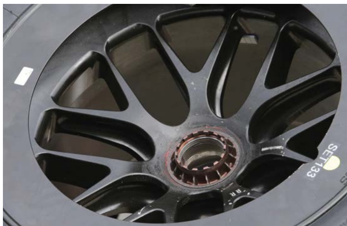
Porsche has introduced an F1-style wheel nut retention system that is supposed to increase speed and accuracy of its wheel changes. It's a risk with new tyre limits this year
