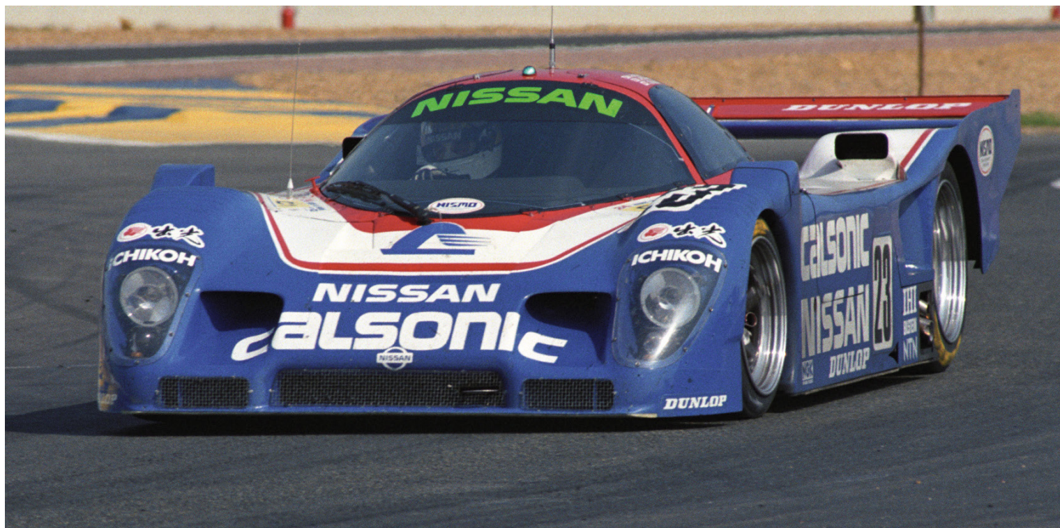
Nissan R90CP in 1990, when the company debuted carbon fibre brake discs at Le Mans, as produced by Carbone Industrie. The car also had 1100bhp on tap! (Jean-Marc Teissedre)
