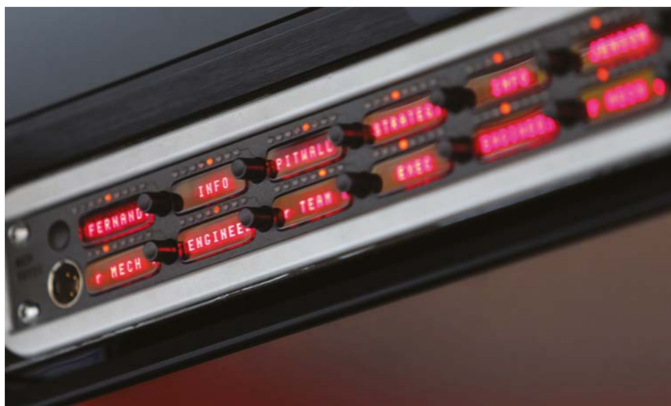
Communications console on the pitwall. The team at the track needs to be hooked up to each and every important member of the operation, whether they are at the circuit or calculating strategies and monitoring data back at its HQ's mission control
