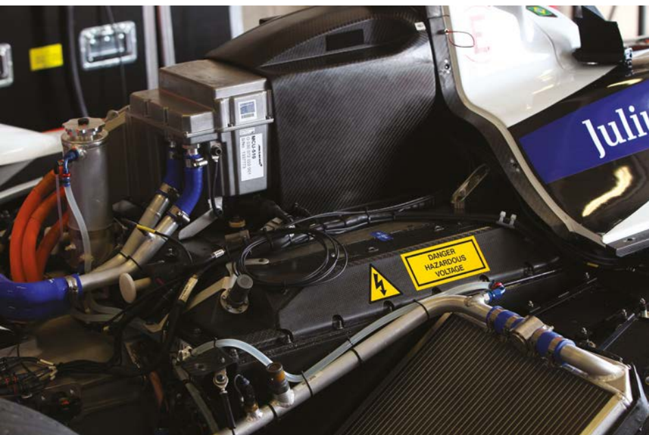
Formula E power pack with hi-vis warning for mechanics. Part of the reason motorsport has been slow to develop both battery and battery management technology is because of the safety issues that are involved
