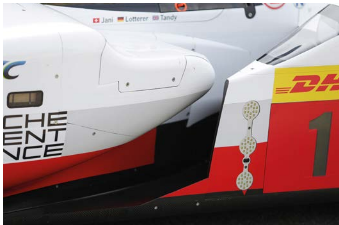
Sidepods have been revised to improve air flow to the rear and a new channel has been opened up between the cockpit and wheel arch to improve safety at high speed
