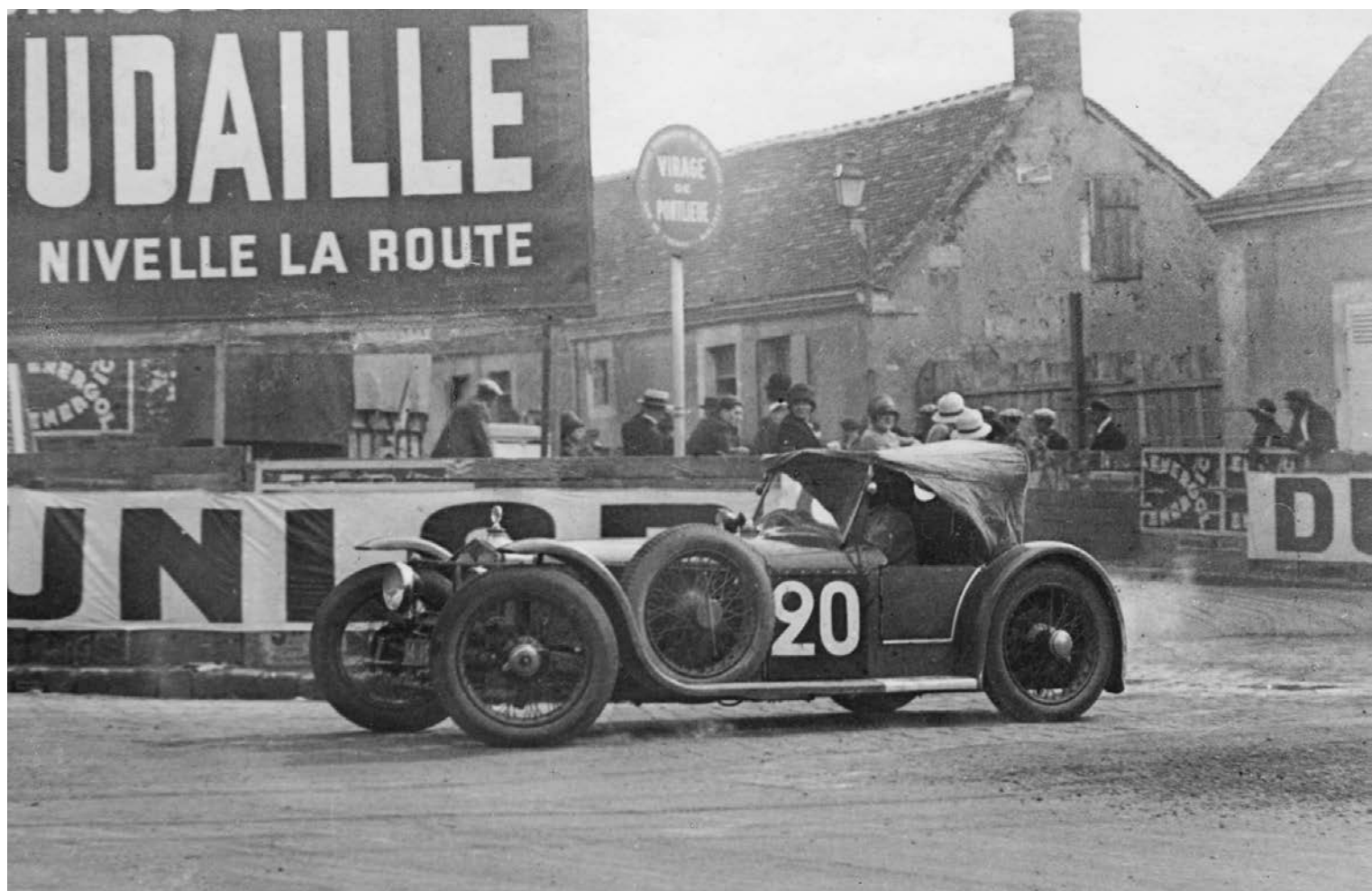
The 4-cylinder 1.1-litre Tracta-SCAP was the first front-wheel-drive car to race at Le Mans in 1927. It finished in seventh overall, 40 laps down on the winning Bentley (ACO Archive)
