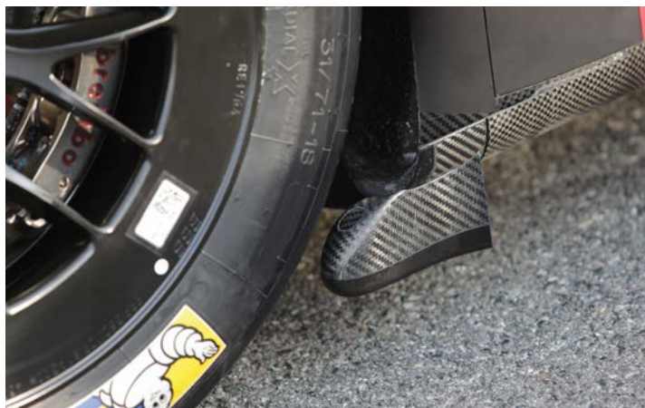
A great deal of detail work has been undertaken to reduce the wake signature of the racecar and clean up airflow to the rear, particularly around the front wheel arches
