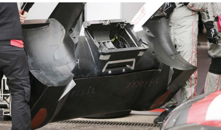
New regulations have seen the front splitter raised in the centre to reduce downforce, but Porsche and Toyota have both developed this area heavily to regain performance
