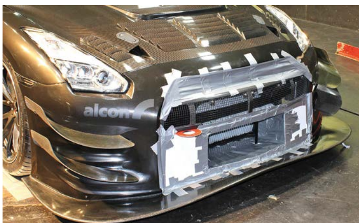
Final step was to tape over the upper aperture completely, further reducing the inlet area
