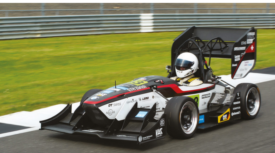
Electric power is making its presence felt at all levels of motorsport these days. The ETH Zurich Formula Student car has 220 cells in its battery pack and its BMS can adjust the voltage to each cell individually
