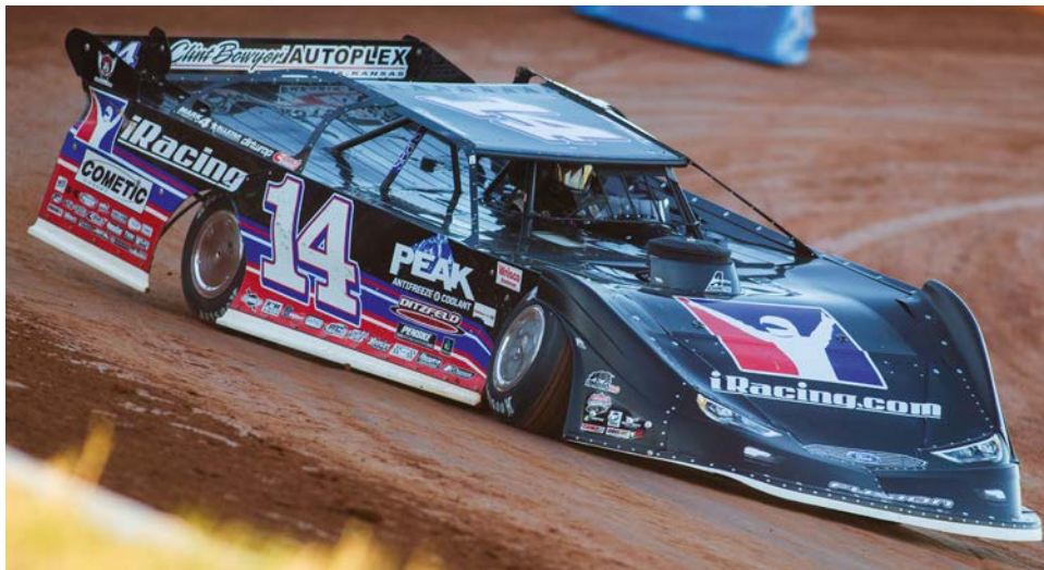
The right attitude for a Late Model dirt car: nose down, tail up and sideways. This generates downforce from the car body
