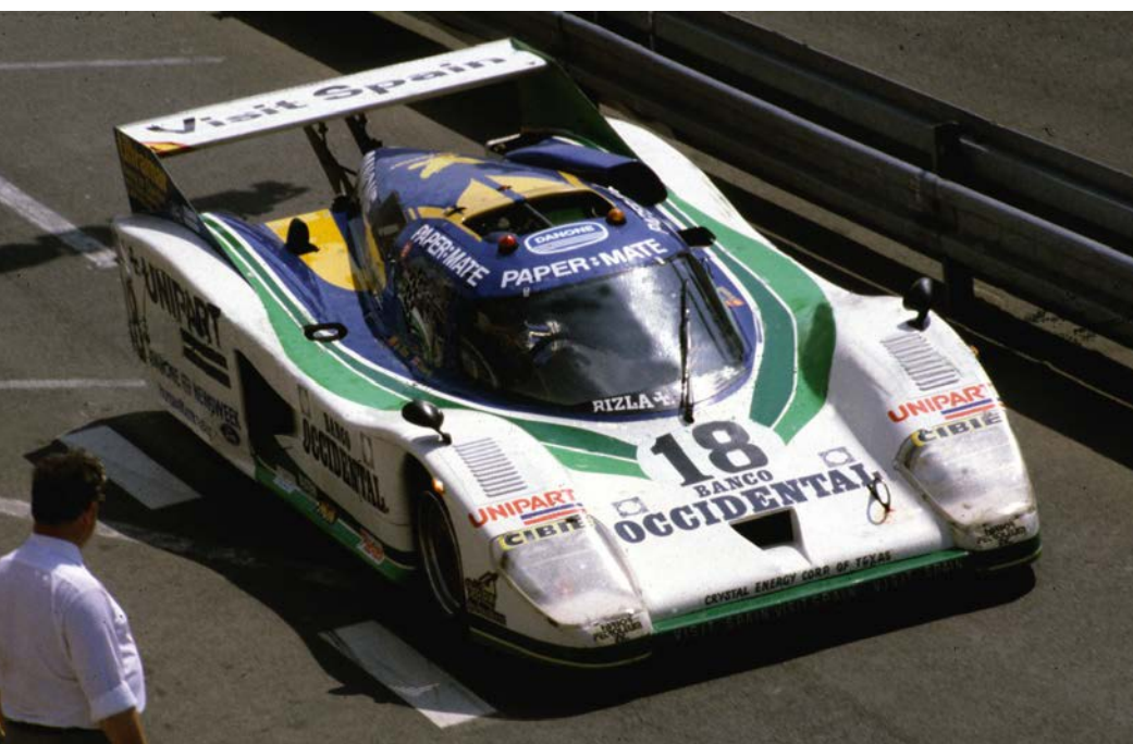
Lola-Cosworth T600 was the first car to run ground effects at Le Mans in 1981. Since the Group 6 category only catered for open-top cars, an inelegant hole had to be cut in the roof of what was actually an IMSA GTP machine (Jean-Marc Teissedre)
