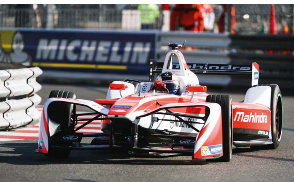
Formula E (pictured at Monaco) and LMP1 both have more complex battery management systems than those that are currently seen in Formula 1. This is mainly down to the fewer cells that are used in the F1 batteries
