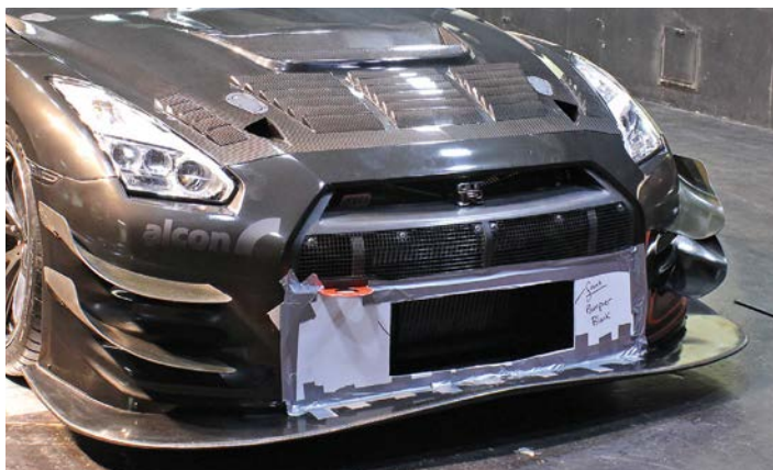
Main front aperture was reduced in size by taping a foam board with smaller inlet over it
