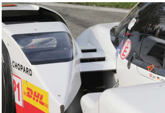
Mirrors are embedded in the wheel arch. Toyota challenged this, on whether it could affect driver visibility, but Porsche says this has improved thanks to reduced vibration
