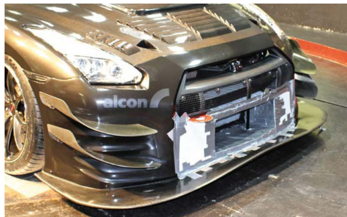
The internal ducting inside the aperture was mocked up with tape and foam boards
