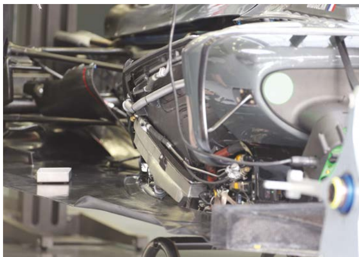
The cooling system is largely a carry-over from the VF-16 with a distinctive V shape arrangement of heat exchangers in the sidepod; a feature of Ferrari's 2017 car, too
