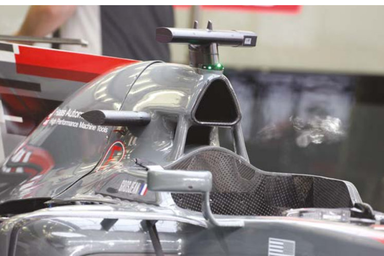
Haas has carried over its 2016 roll hoop but the charge cooling layout has changed, with now just a single duct within the hoop. Lower duct behind it cools electrical parts
