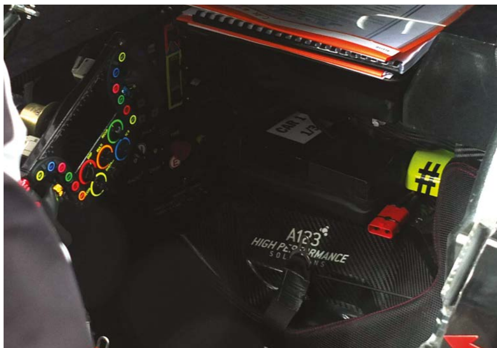
The Porsche 919 Hybrid LMP1 car uses an A123 Systems battery located in the cockpit. Really big developments in battery systems are likely to be focussed on chemistries rather than the BMS; the latter simply a tool to get the most from the battery
