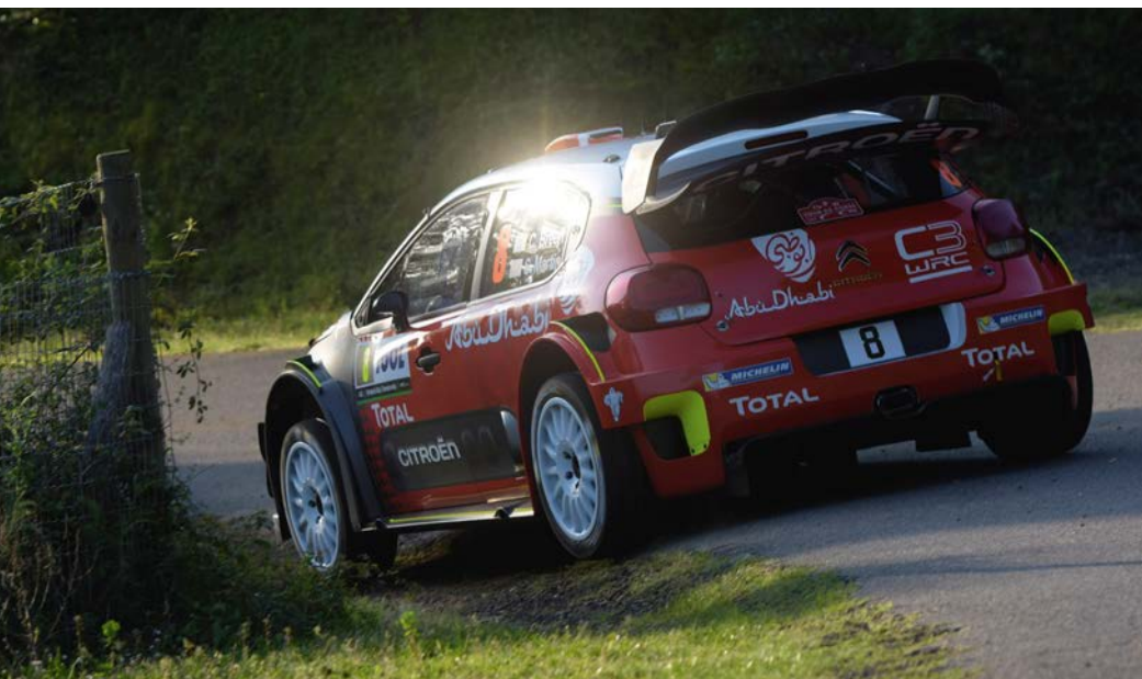
Some of the aerodynamic parts have proven fragile, especially the front splitter. Note the large 2017-spec wing and diffuser
