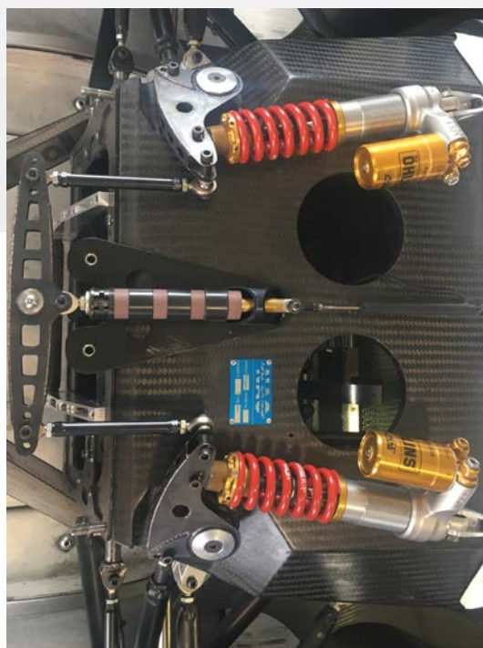
To deal with the bumpy and rough track (at the top of the course at least) PKM Consulting has modified the Ohlins TTX36 shocks from last year's car to produce clever 4-way adjustable dampers
