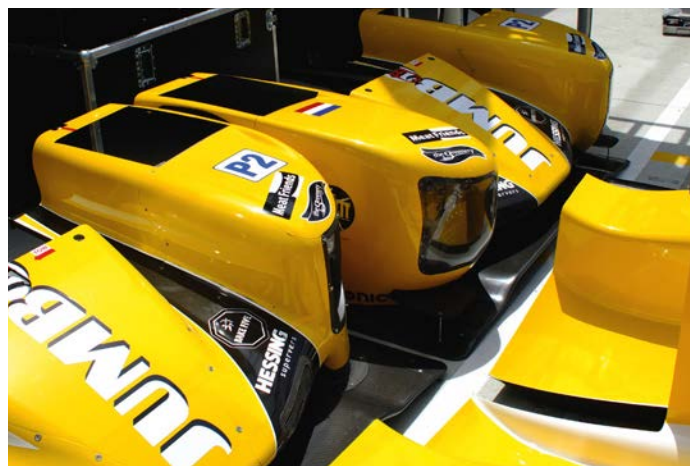
Dallara low drag nose next to WEC spec high downforce example; latter in foreground
