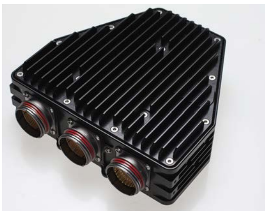
As well as F1, TAG-320 is also used in LMP1 and autonomous vehicles. It is capable of monitoring over 1000 parameters of data
