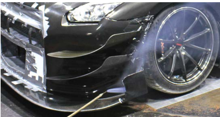
Larger splitter end fences added upwash to join flow off undersides of lower dive planes
