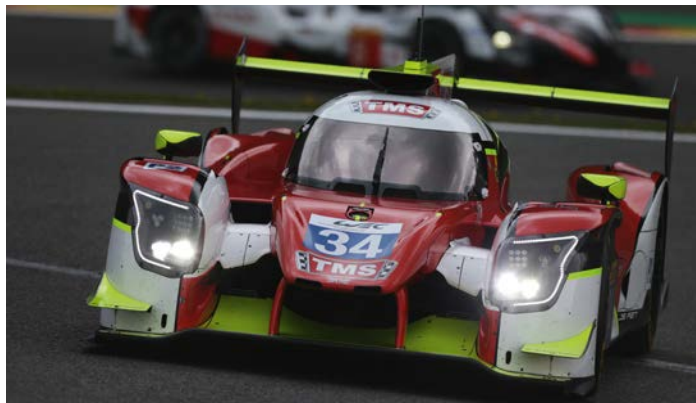
Ligier in WEC spec. At Le Mans it struggled for both straight-line speed and downforce
