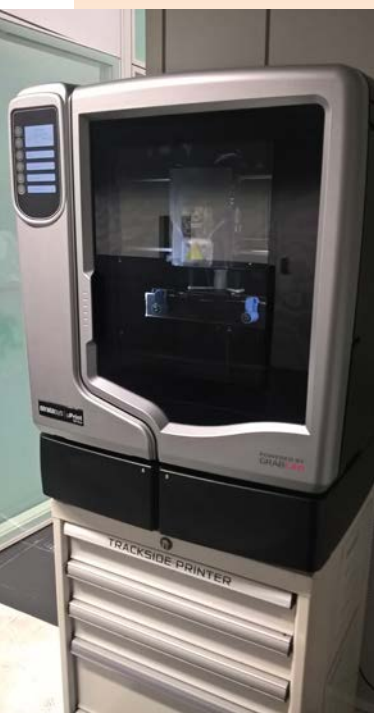
Stratasys Trackside Printer. This FDM machine has been used at the circuit by McLaren already this year and the technology is becoming common in F1
