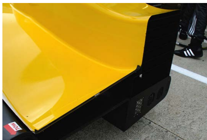
WEC spec rear of Dallara – Gurney was removed for Le Mans kit (see previous image)
