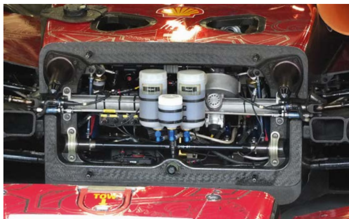
... Which in turn was based on Rebellion R1 LMP1 car. R1 bulkhead is shown above
