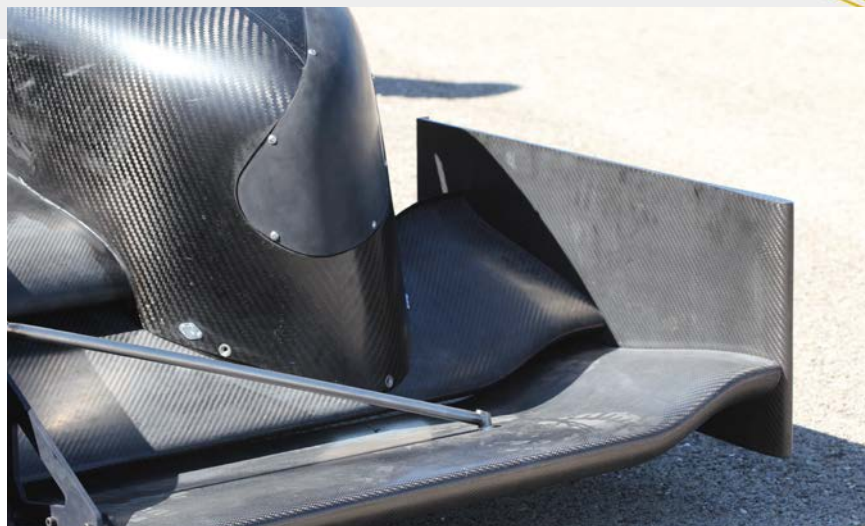
The front wing endplates help to generate strong vortices which flow around the front of the tyres. The aero package has been developed with help from a cadre of former Stuttgart Formula Student team members
