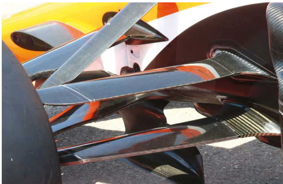
Suspension components are notably larger than in 2016 due to the much higher loads they must withstand this season
