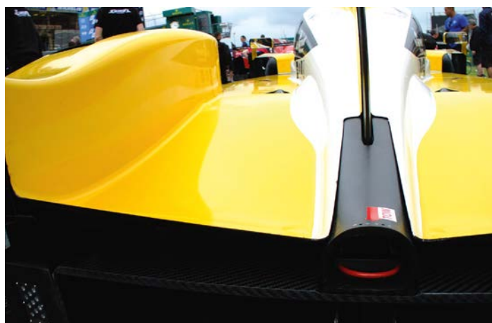
The Dallara's Le Mans spec trailing edge – its low drag kit was perhaps the most extreme
