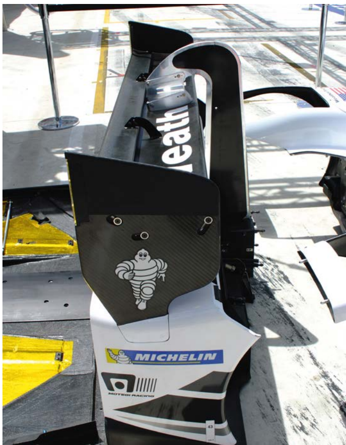
Riley's new rear wing endplate had reshaped upper section and a lower wing position
