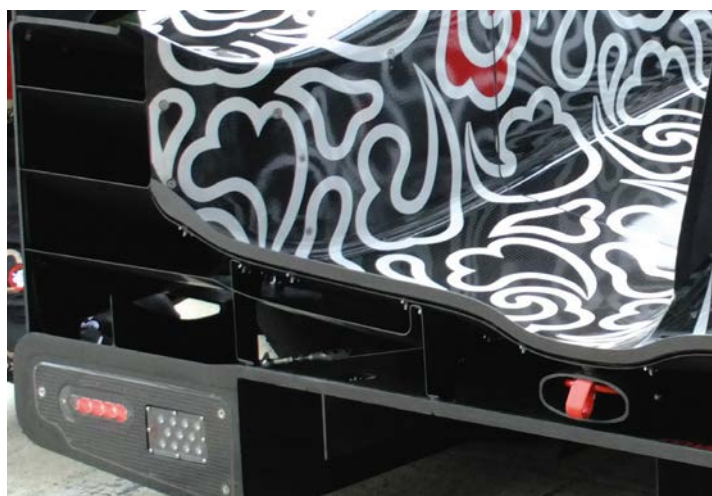
Gurney on the rear of the WEC spec 07 is much larger. ORECA develops aero in CFD
