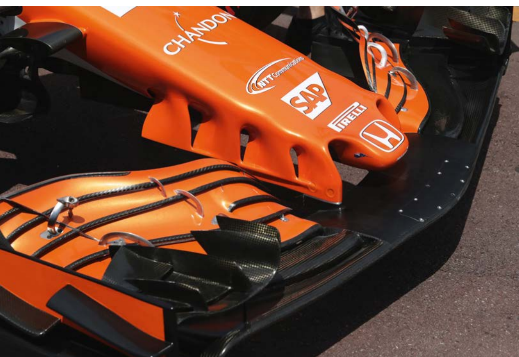
Note slots in the panels from which the front wing is suspended. McLaren says front wing treatment carries over from 2016
