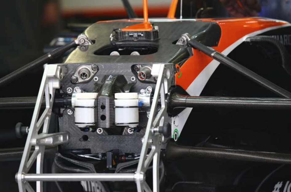
Front bulkhead showing torsion bars and inboard suspension pick up points. In common with the rest of the 2017 Formula 1 field the MCL32 uses pushrod actuated suspension at the front and pullrod at the rear
