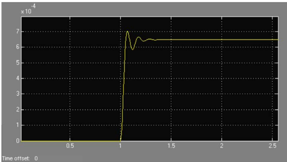
Figure 4: Step input response of pitch to a moment of 500Nm. There is still an initial overshoot here but it is much reduced
