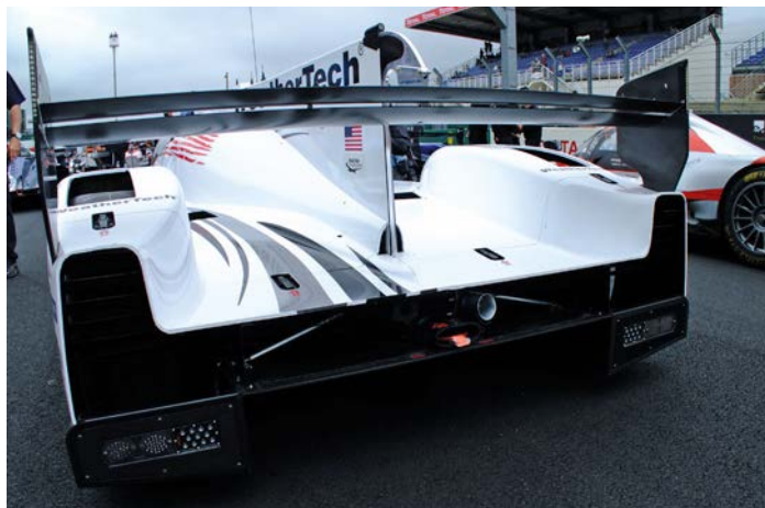
The Riley Multimatic had a lower wing position with no Gurney on trailing edge of body
