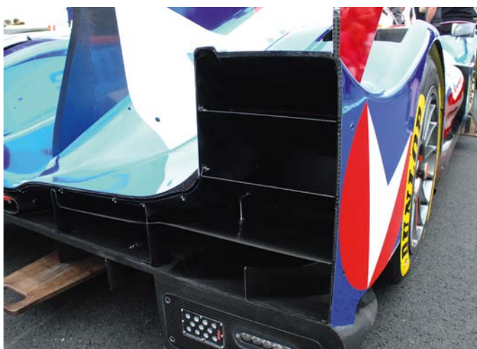
The Le Mans spec rear has a smaller gurney to promote higher straightline speeds
