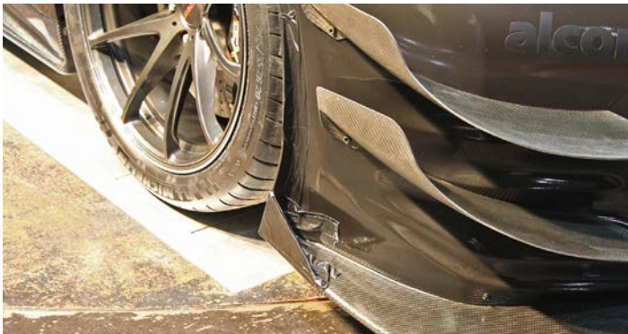
Adding these small splitter end fences produced some extra downforce at the front end
