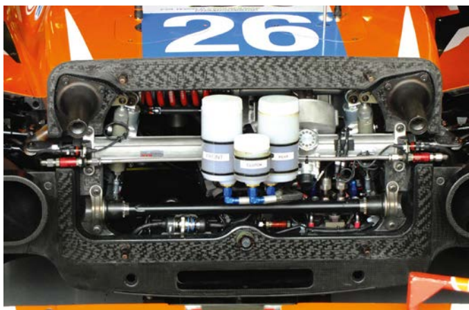
The ORECA 07's front bulkhead. Monocoque was carried over from previous 05 ...
