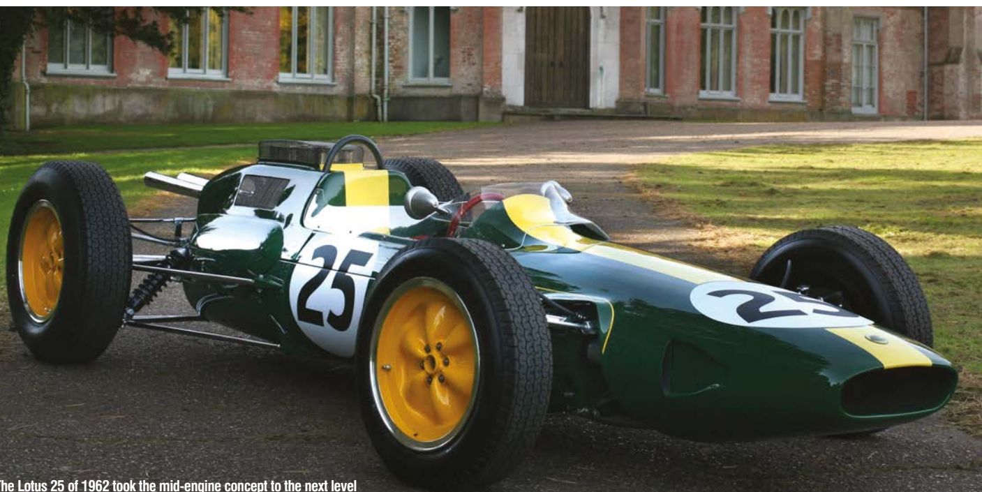
The Lotus 25 of 1962 took the mid-engine concept to the next level with the introduction of fully-stressed monocoques in to Formula 1
