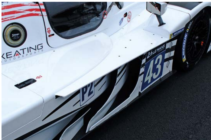
Riley Multimatic's Le Mans low drag kit. This shows extended top panel arrangement
