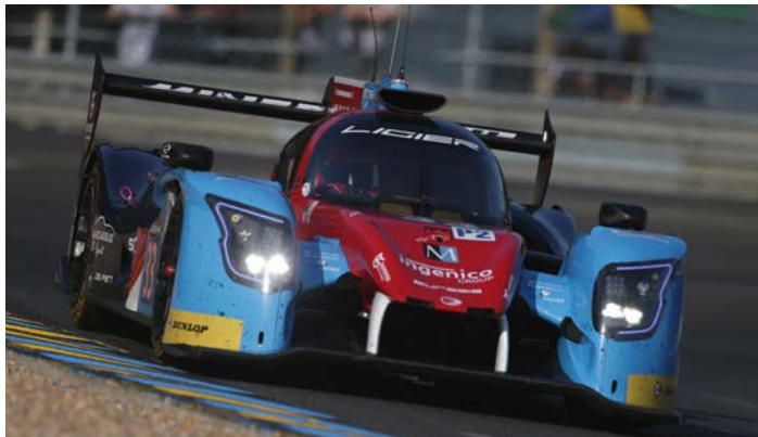
Ligier Le Mans kit. There were few changes from WEC spec beyond a lowered rear wing
