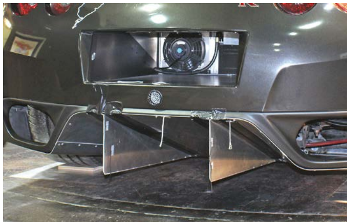
Strakes, which divided the diffuser exit into three parts, added some rear downforce
