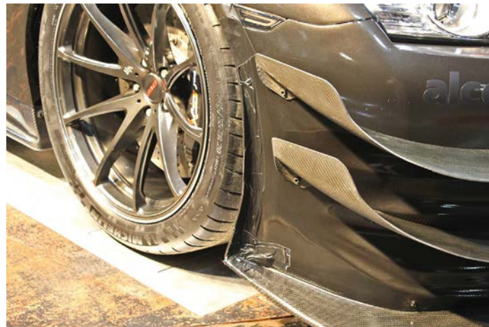
This front wheel arch Gurney helped with balance, but the mod was not very efficient
