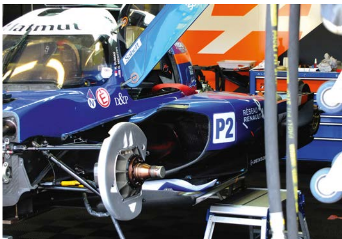
ORECA 07 runs double wishbone front suspension with pushrod actuated torsion bar
