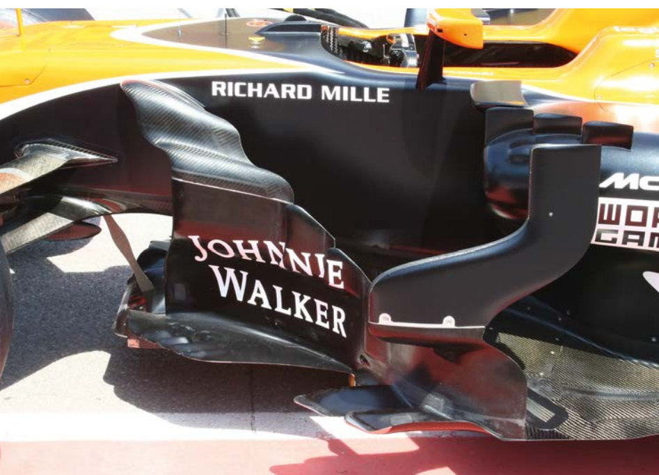
McLaren says it has invested much time in developing the aerodynamics around the bargeboard space and it sees this newly opened up avenue as an area of further exploitation during this season and in years to come
