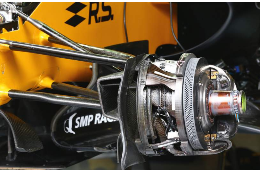
The front brakes, with interesting curved disc section. RS17 uses carbon discs and pads, calipers are courtesy of Brembo while master cylinders are supplied by AP Racing. The racecar has shown some aero sensitivity around the rear brake area
