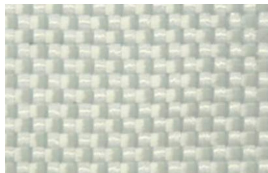
Diolen is a white material with high strain-to-failure properties
