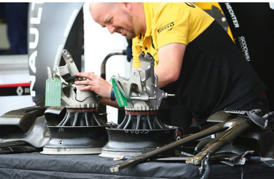
The aluminium uprights have to cope with higher loads this year due to the extra downforce and wider rubber available. Renault says that not knowing what these loads would be was frustrating during the RS17's design
