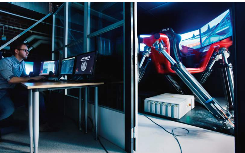
Chalmers University purchased its own Cruden A646-D3 platform simulator, which is entirely run by the students under a project dubbed CASTER. This initiative helped develop the vehicle models for the establishment's Formula Student Team
