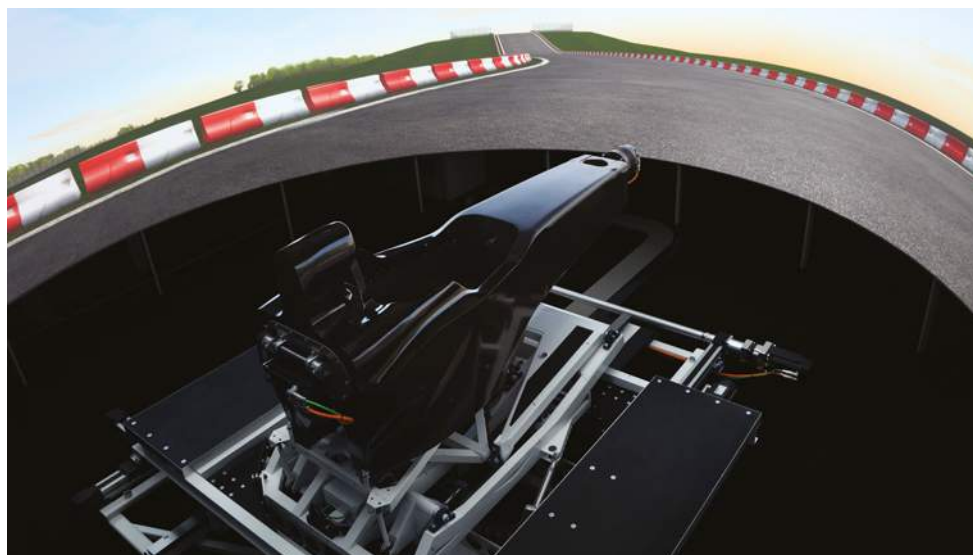
With the very best simulators immersion in the virtual world is the aim and to help foster the illusion a real monocoque will be used in conjunction with a wraparound screen. Torque forces will also be applied through the steering wheel and the belts
