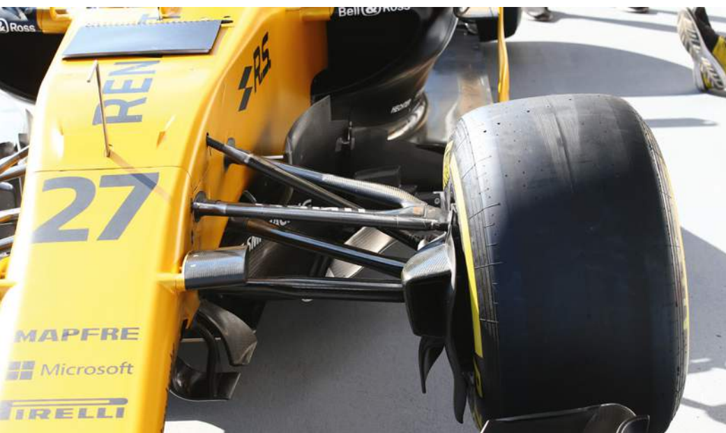
Front wishbones are noticeably beefier than last year's to cope not only with the higher loads from cornering but also more unpredictable loads from kerbs. While Renault was cautious when it came to strength it did not design in extra adjustability
