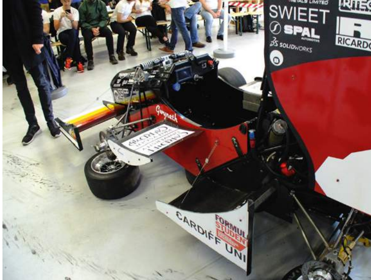
The aero philosophy is not to work the air too hard at the front of the car so as to make better use of the side wings and the three-tier, six element, rear wing stack
