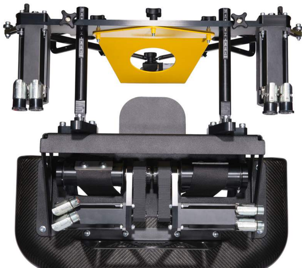
The Helmet Loading System is fitted to the top of the race seat and it applies torque loads to simulate cornering force
