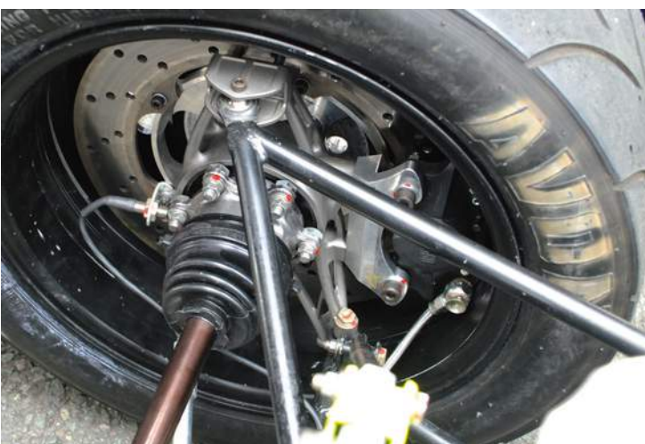
Wolverhampton's uprights were highly intricate and quite a feat of engineering given the tight space allowed with those tiny Formula Student wheels and tyres
