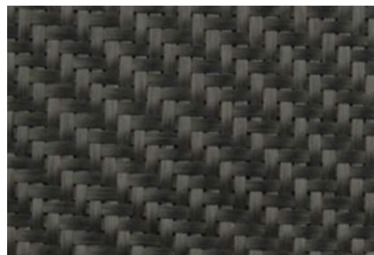
Carbon's strength is in the direction in which the fibre is woven
