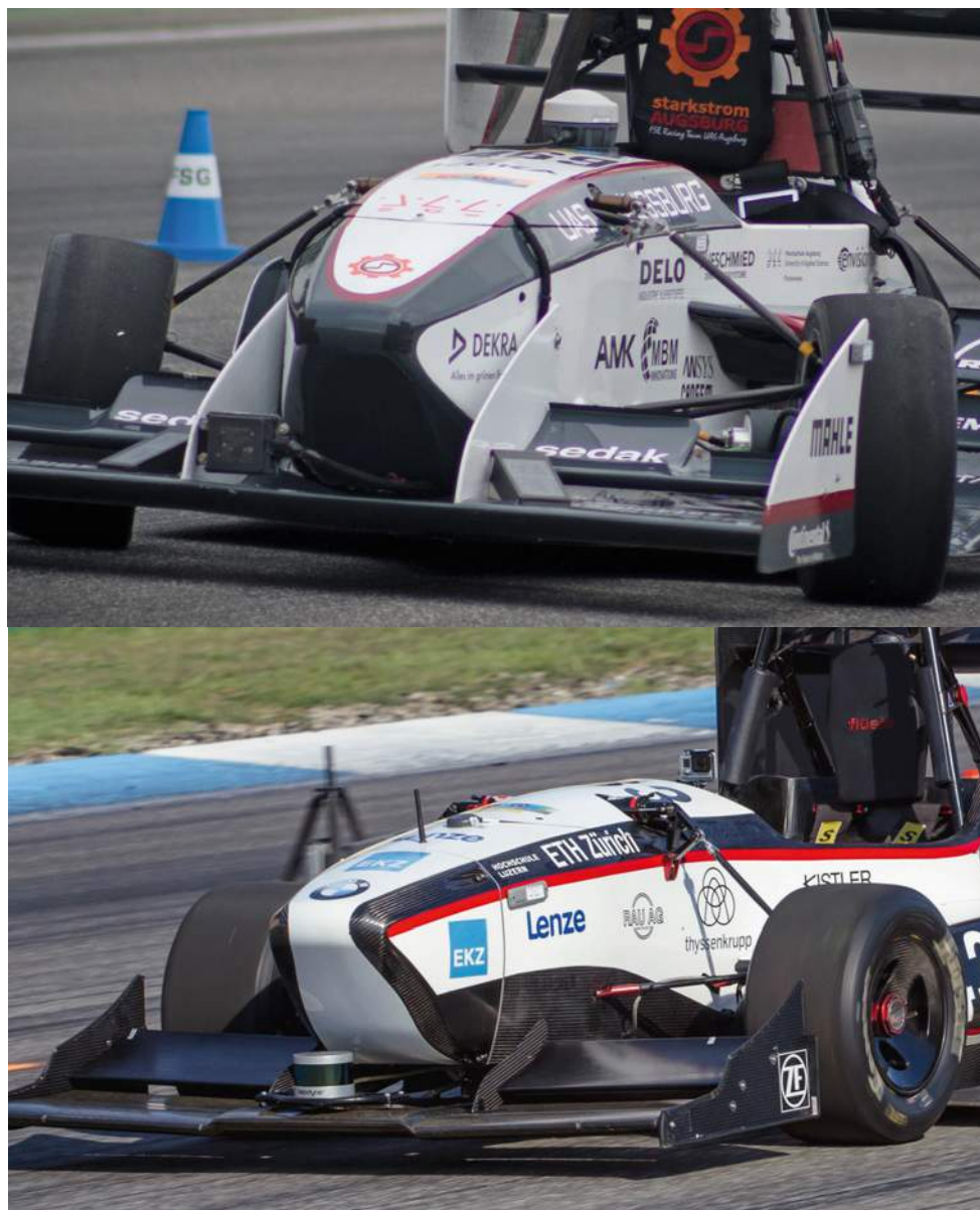
There were different approaches to locating the LiDAR (light detection and ranging) sensors. UAS Augsburg (top picture) situated its LiDAR on top of the monocoque, while ETH Zurich put it between the nose and the front wing (bottom picture)
