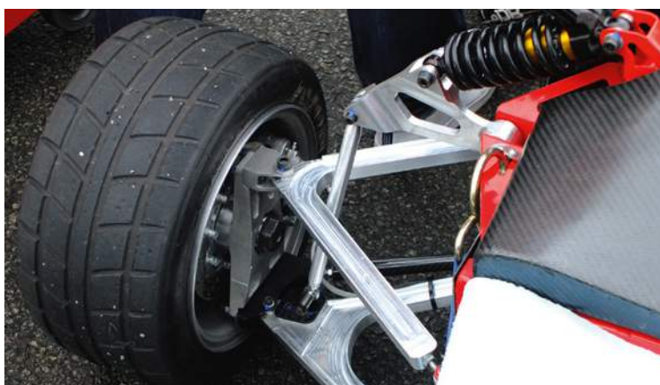
Detail of the front suspension showing damper actuation on the UCLAN entry. Despite the innovative approach the team could do no better than a midfield finish at this year's event
