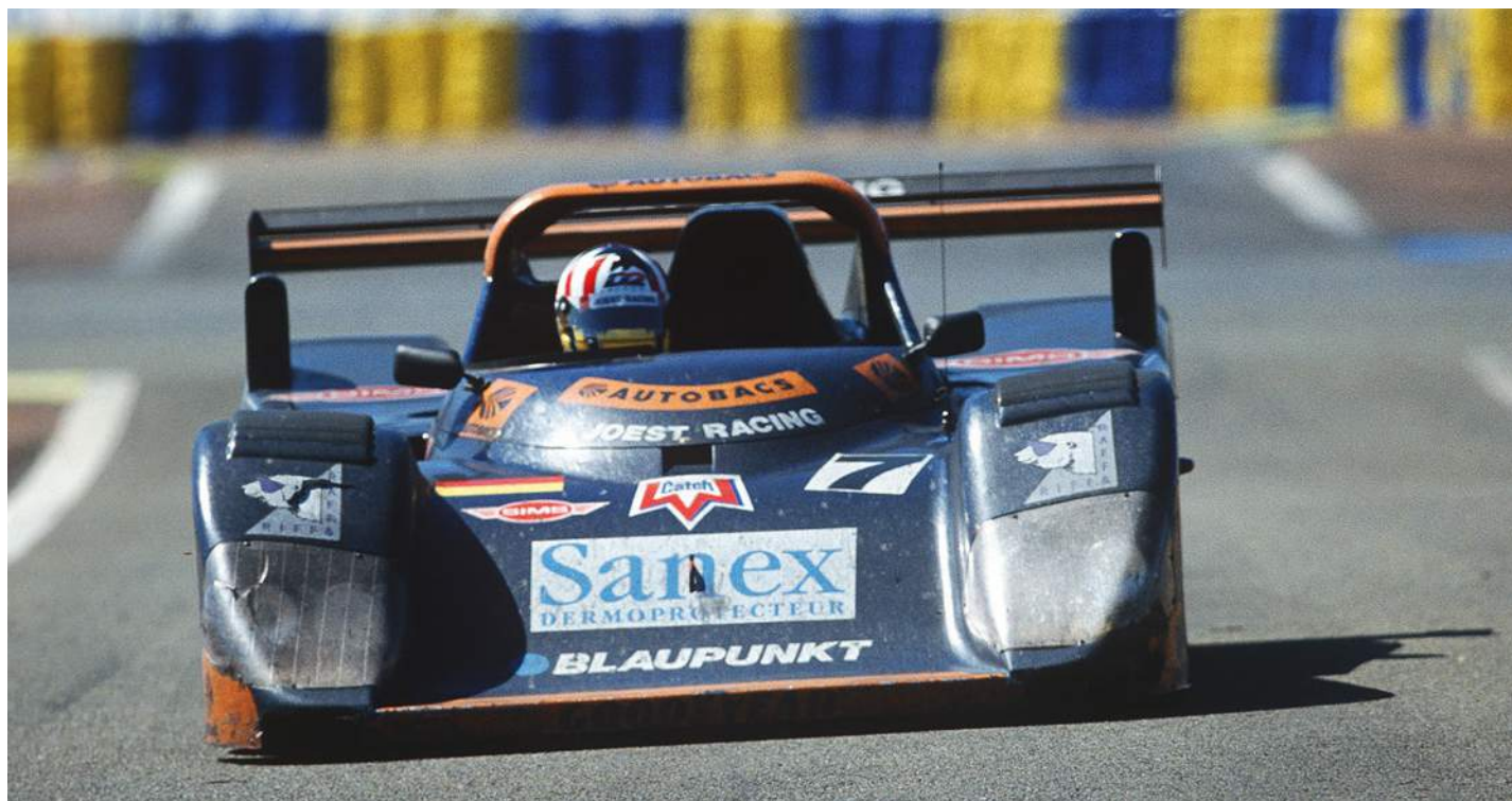
Porsche's WSC95 was in reality a 1991 Jaguar XJR-14 chassis with the roof chopped off, mated to a 935/85 engine and 956 transmission. Joest won Le Mans with it in '95 and '96
