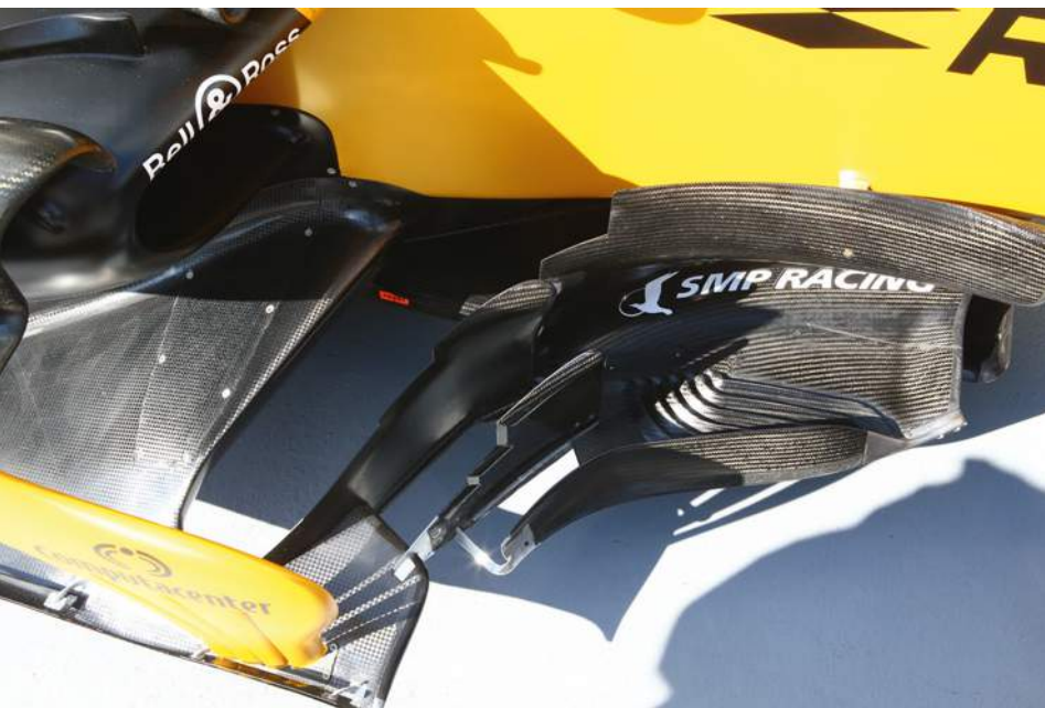
The bargeboard area has been freed up for 2017 and hence it's also been the subject of much aerodynamic development by all the Formula 1 teams, and Renault is no exception, filling the space with this array of flicks
