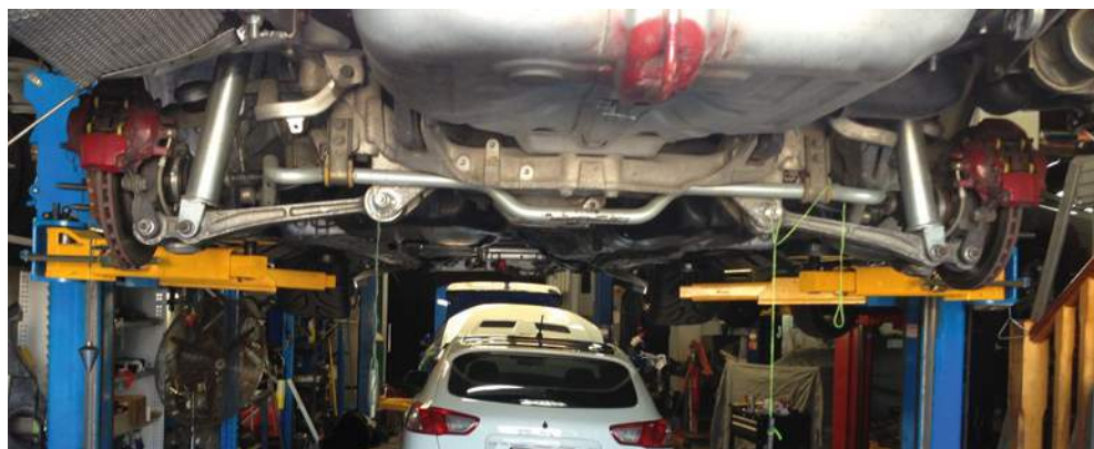
Using a plumb bob. This low-tech device is useful as it gives you a ready made reference to measure the points across a car
