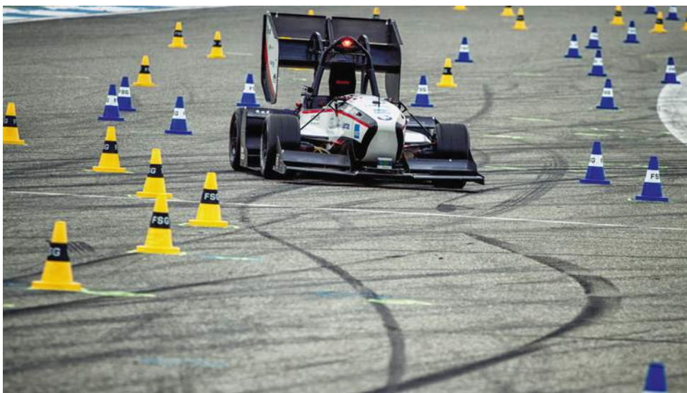
There are different coloured cones for each side of the track to help the stereo camera systems, which can pick out the different colours, to distinguish between the right and left side of the road. The finishing area is made up of orange cones
