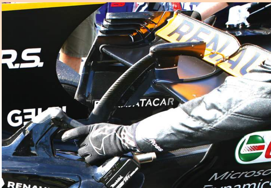
To meet the regulations a plate had to be added to the underside of the rear wing pylon for the season opener in Australia
