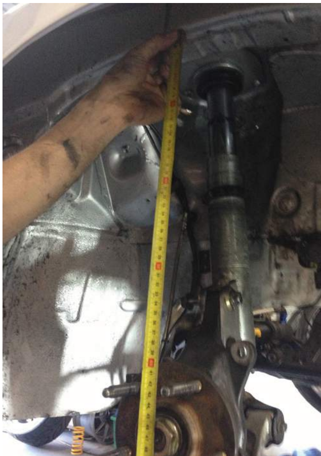
On a touring car or a GT car you measure the wheel movement to the wheelarch
