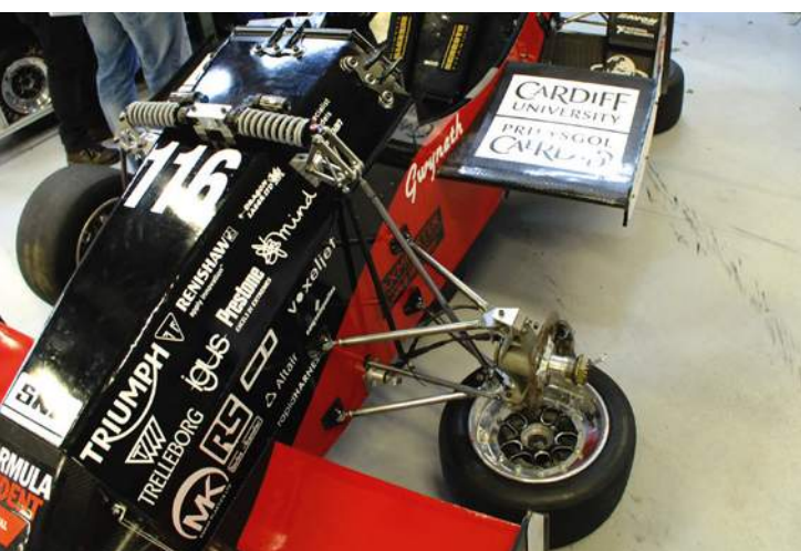
Front dampers and spring assemblies are mounted on the upper side of the car's bodywork. Cardiff switched to Avon race rubber this year as it warms up quickly
