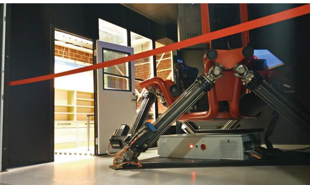
Formula Student teams have embraced simulators and found uses for the technology in both driver training and racecar development. Some universities are now also using them for teaching and research. The Chalmers simulator is pictured
