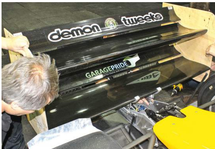
Moving the beam wing yielded some interesting results and is a worthwhile modification
