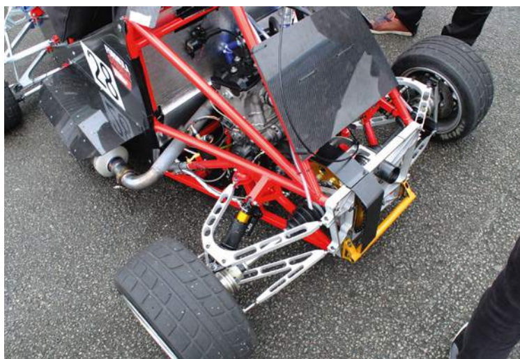
The University of Central Lancashire's (UCLAN) racecar had interesting and very intricately machined rear suspension, boasting perforated wishbones with some imaginative profiles
