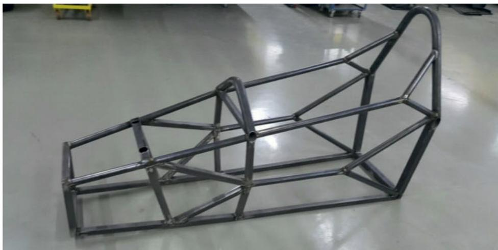
The classic spaceframe, with separate subframe for engine, was chosen over an expensive and impractical carbon chassis
