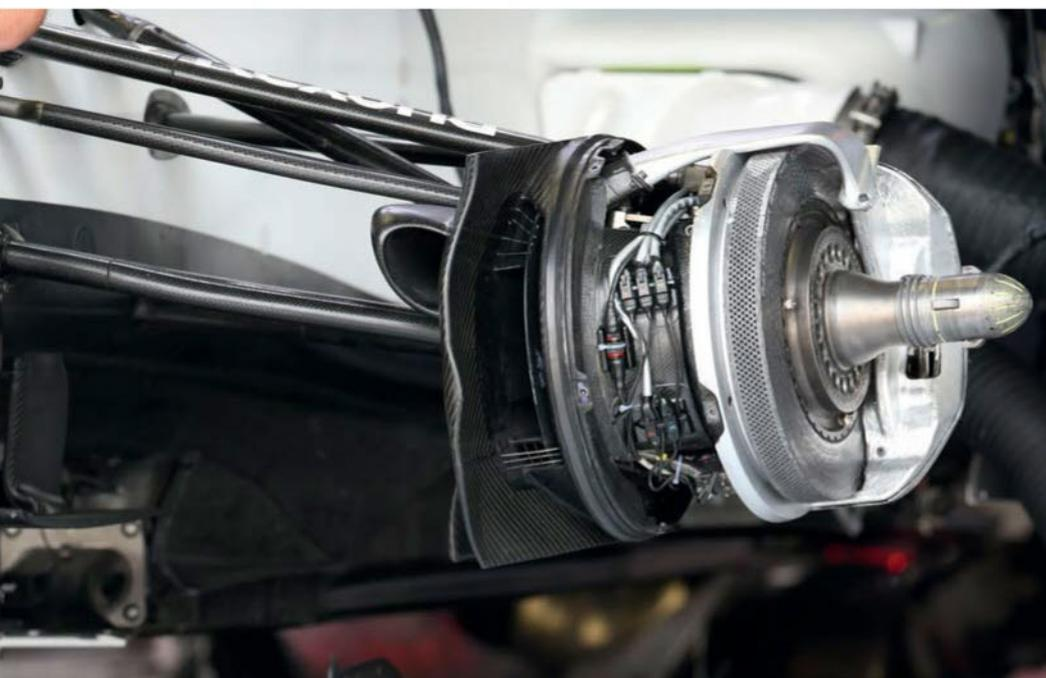
Brakes are AP Racing 6-piston front (above) and 4-piston rear calipers with carbon discs and pads. Wishbones are beefier this year to cope with the higher loads while cornering, which are a result of new-for-2017 aero regulations and wider tyres
