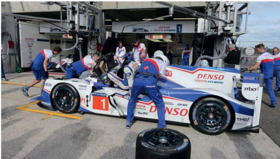
Toyota practices changing the FFM, located behind driver's door on LMP1 cars. Flow meters measure average flow in WEC
