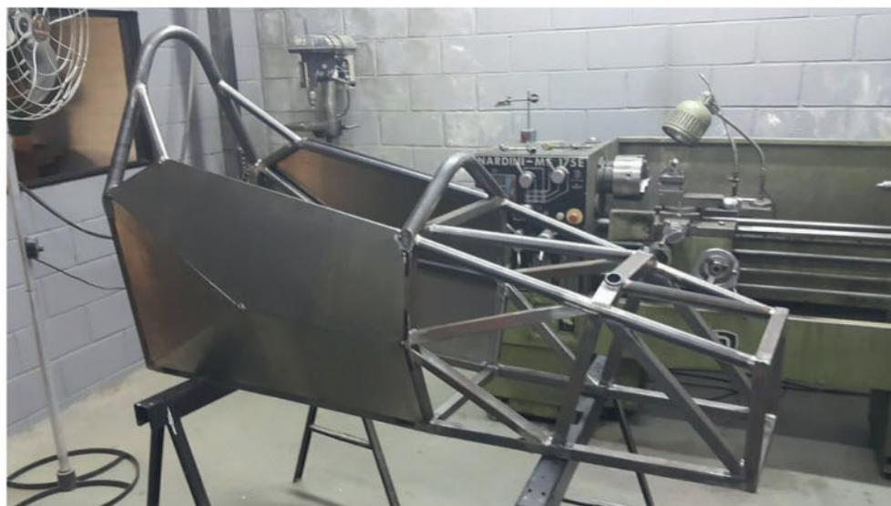
Main bulkheads were of rectangular section and perpendicular to chassis base, making for easier manufacture and jiggling
