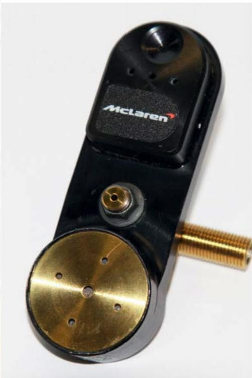
The TPMS sensor is located on the rim where the tyre bead seats. These not only measure tyre pressure but now also include IR elements to measure the temperature of the tyre carcass
