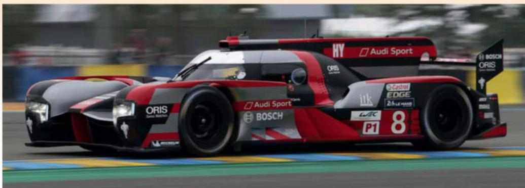
When it was in the WEC Audi's R18 suffered with fuel flow meter accuracy problems caused by the high diesel return temperatures
