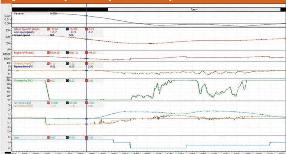
The extra detail is clear to see here. Note the near 1km/h differential on turn in and the 0.03s variation in the compare time
