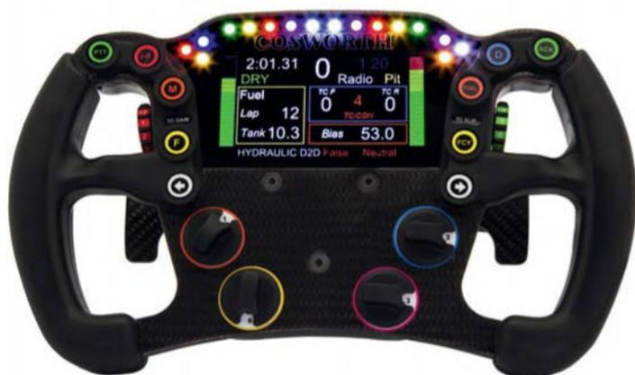
CCW Mk2 display has a row of 10 shift lights plus six alarm LEDs
