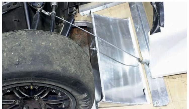
The Aries team fabricated these adjustable diffusers. Lock-nut arrangement (centre) allowed the front diffuser ramps, hinged below with tape at the transition, to be adjusted for angle
