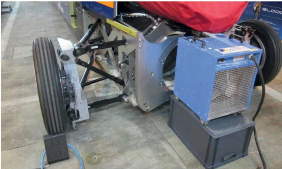
Rear wheel track width needed to be minimised to help counter aerodynamic lift problems caused by the rear shock wave
