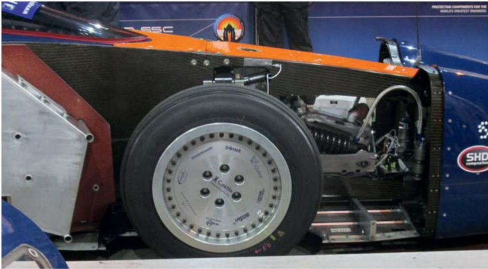
At 1000mph the Bloodhound's wheels will be spinning at 10,200rpm (170 times per second) and generating 50,000 radial g
