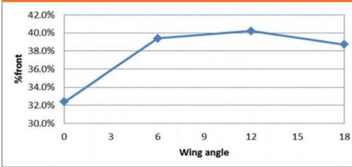
Figure 1: This shows that %front appeared to peak at the 12-degree front diffuser angle
