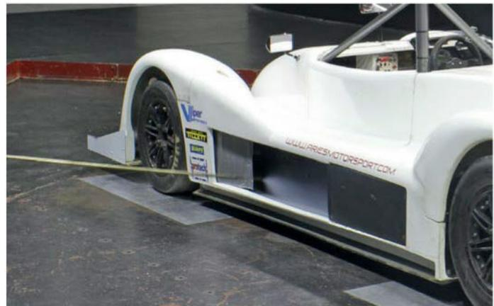
Silver-taped wheel fairings can be seen behind the front wheels; the results were better without these in place. Sidepod undercuts are just above the running boards
