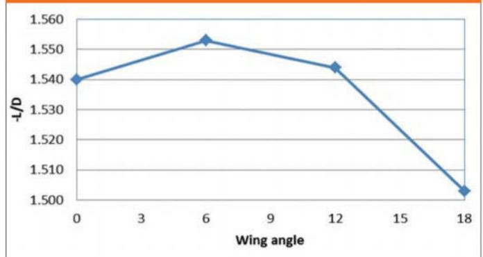
Figure 2: The aero efficiency appeared to peak at the 6-degree front diffuser angle
