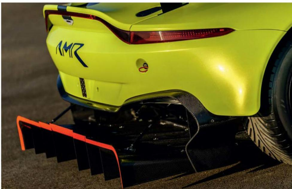
Carbon fibre and steel five-piece floor features splitter, three mid-car sections, and runs into a whopping diffuser at the rear
