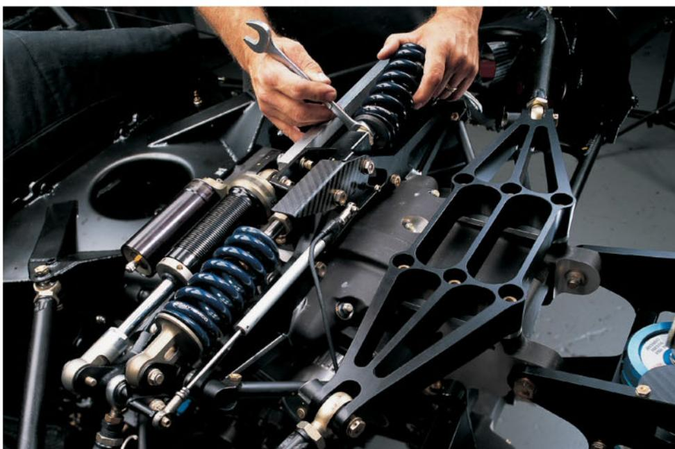
Race engineers adjust the dampers by clicks, altering the valving within the shocks to increase or decrease the resistance
