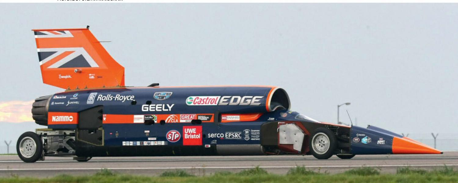
CFD analysis of even the smallest configuration changes takes about 30 hours and so homing in on an acceptable aerodynamic package has required close to three years of work
