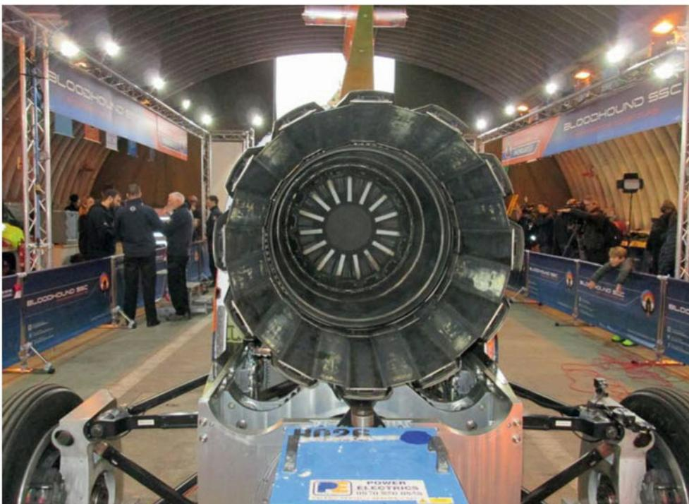
The 800mph tests will require the EJ200 jet engine and a single rocket, but for 1000mph it will need the jet and three rockets
