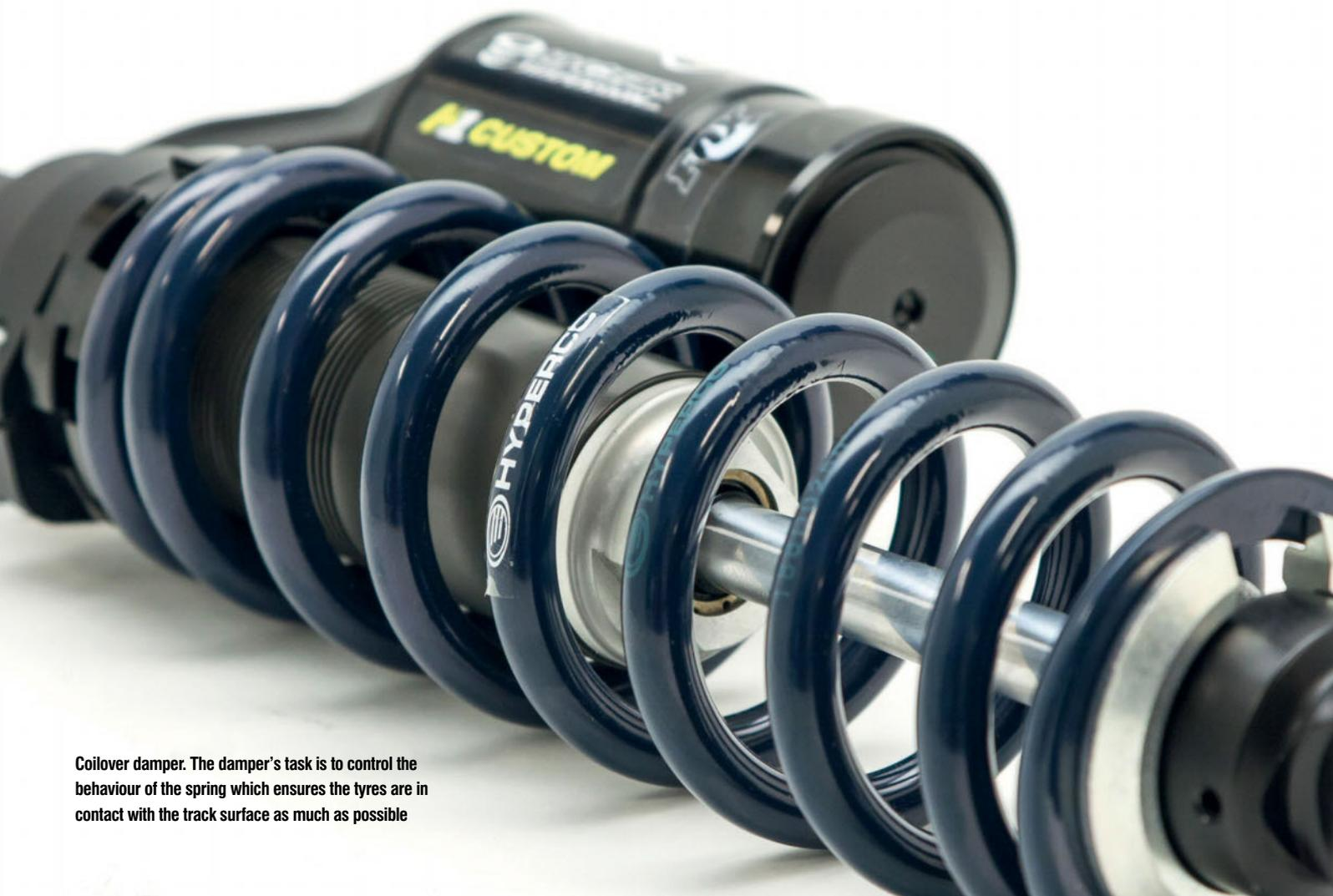
**Coilover damper.** The damper's task is to control the behaviour of the spring which ensures the tyres are in contact with the track surface as much as possible
