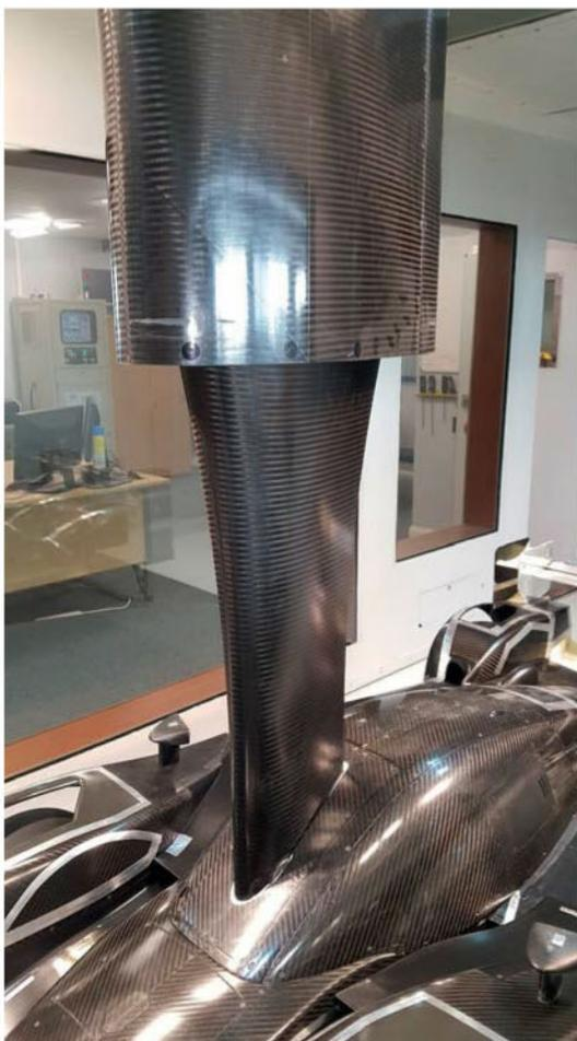
The wind tunnel model is attached to a carbon support strut that is connected to a six-component pyramidal virtual centre balance
