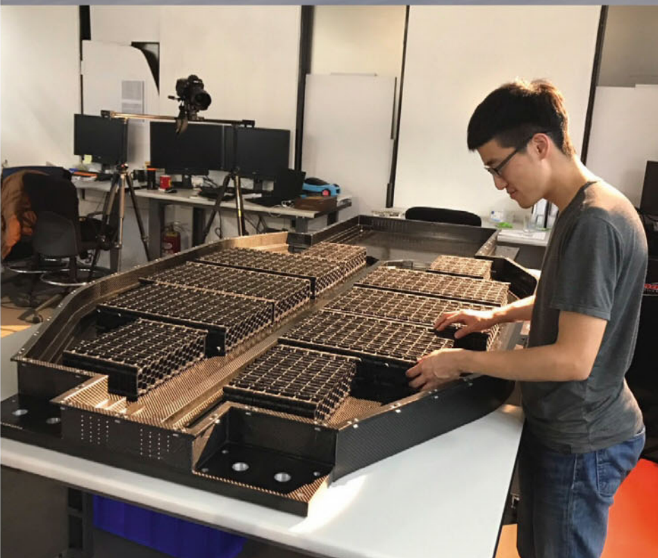
Left: Modular battery packs mounted in the floor of the Miss R car. Xing's approach allows for battery packs to be built up to suit the application and it is aimed at low volume electric vehicle projects Above: The Xing battery system is fully sealed and cooled by Novec fluid – a non-conductive liquid that has long been used for solvent cleaning, fire suppression and supercomputer cooling
