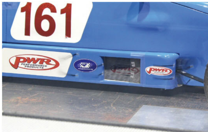
Satisfactory flow into and out of the radiators is revealed here with the use of wool tufts, although the flow ahead of the lower inlet did seem to prefer to go under the car
