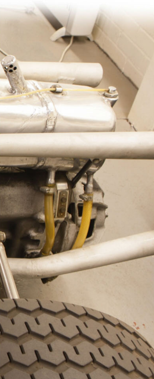
The first Formula 1 car to pack the H16 was BRM's 1966 entry, the P83. Note the routing of the water pipes outside the car
