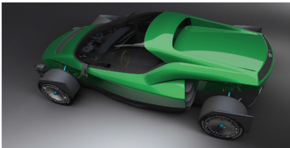
Miss R is designed as a niche road car, though Xing hopes it will be used in competition. It uses the GT300 Mother Chassis
