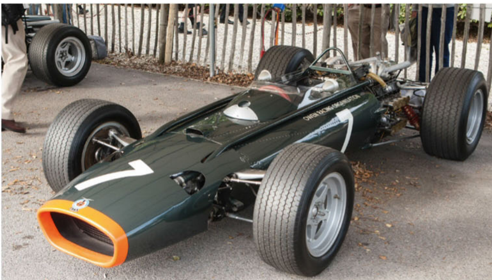
The first Formula 1 car to pack the H16 was BRM's 1966 entry, the P83. Note the routing of the water pipes outside the car
