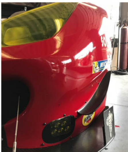
Above: A rare glimpse of the engine and gearbox of the Porsche GTE out of the car Right: Ferrari's update kit includes a new front bumper shape with recesses to allow for the dive-planes to be better located. It also has a new front splitter profile
