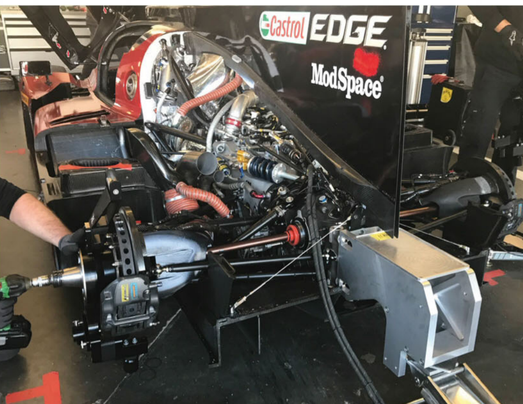
Switching to a more conventional rocker pivot installation pushrod, with longitudinal dampers, has not only helped to stiffen the rear but has also taken weight out of the racecar. The suspension mods had to be worked around the Xtrac transmission
