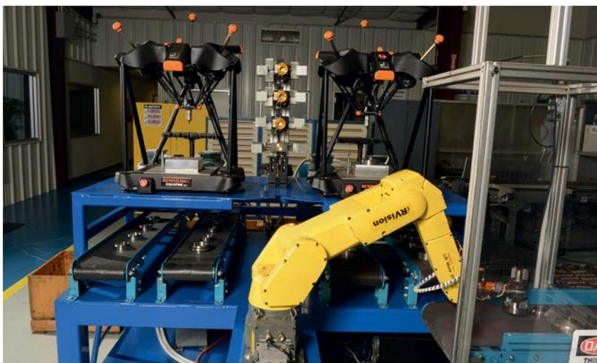
The Equator Gauge can be fully integrated into the manufacturing process and used to check parts as soon as they have been made. Robots move parts from the machine and automatically load them on to the Equator
