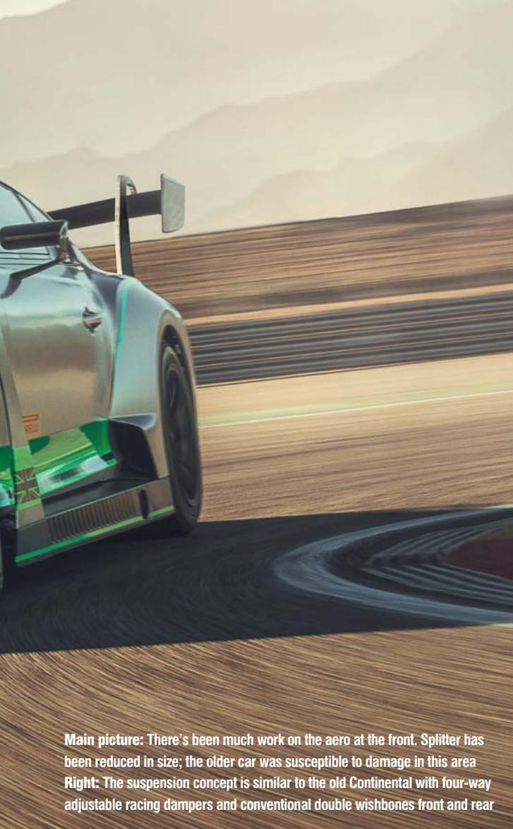
**Main picture:** There's been much work on the aero at the front. Splitter has been reduced in size; the older car was susceptible to damage in this area
