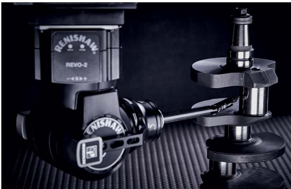
Measuring surface roughness has traditionally been seen as a black art but with Renishaw's SFP2 probe the roughness of a surface can now be measured in a controlled way, ensuring the smooth surfaces essential for engine components
