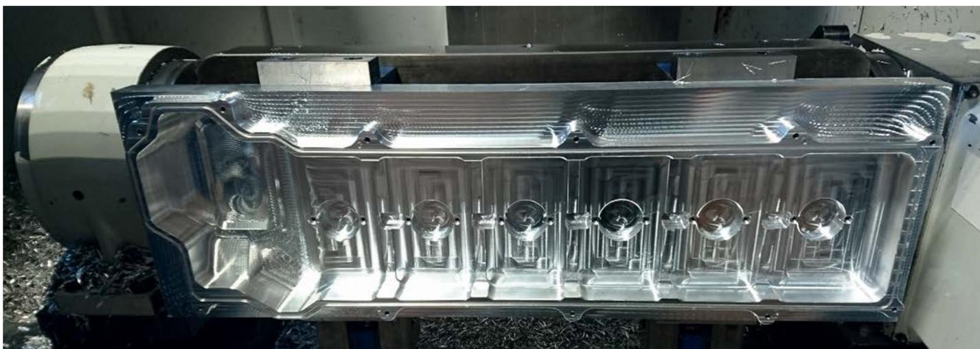
Underside of left-hand billet tappet cover during machining. Hartley sees the V12 as a great advert for the New Zealand-based company's powerplant design and CNC capabilities
