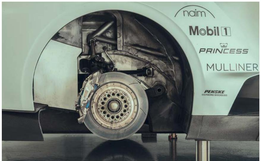
New body means the suspension pick up points are different and this has impacted on the car’s kinematics
