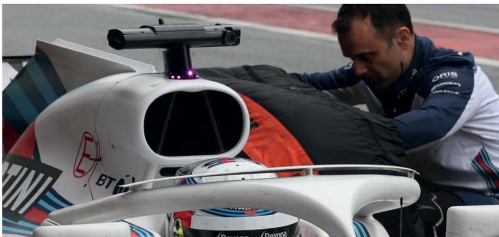
Williams uses centreline cooling. The 'A' of the roll-over structure is clear to see here. The outer segments of the intake feed air to coolers over the bellhousing, while the centre portion is for the air to the internal combustion element of the power unit
