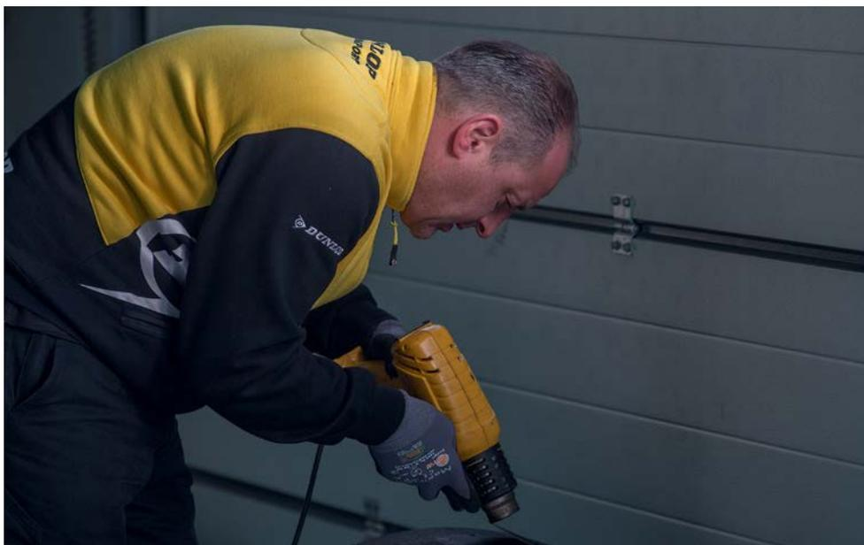
To measure tyre wear first the pick-up on the surface of the tyre needs to be heated up and then scraped off. Only then can a wear gauge be used to measure the depth of the wear holes and therefore the amount of rubber that has been worn away
