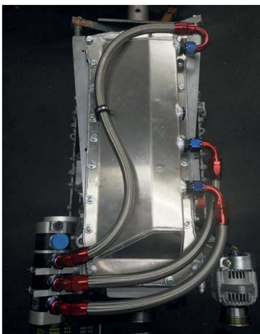
The underside of the engine showing the fabricated dry sump and the oil pump feed and return. All the work is high-end specification
