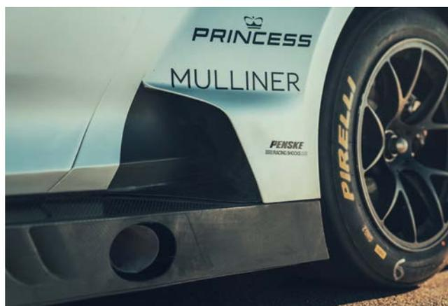
New sills increase the floor's width and are also designed to help brake cooling
