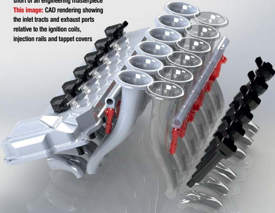
**CAD rendering showing the inlet tracts relative to the cylinder positions**
