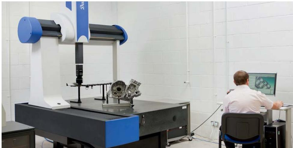
A 5-axis CMM using REVO. The CMM head automatically selects a stylus from the rack via magnets in the probe's head
