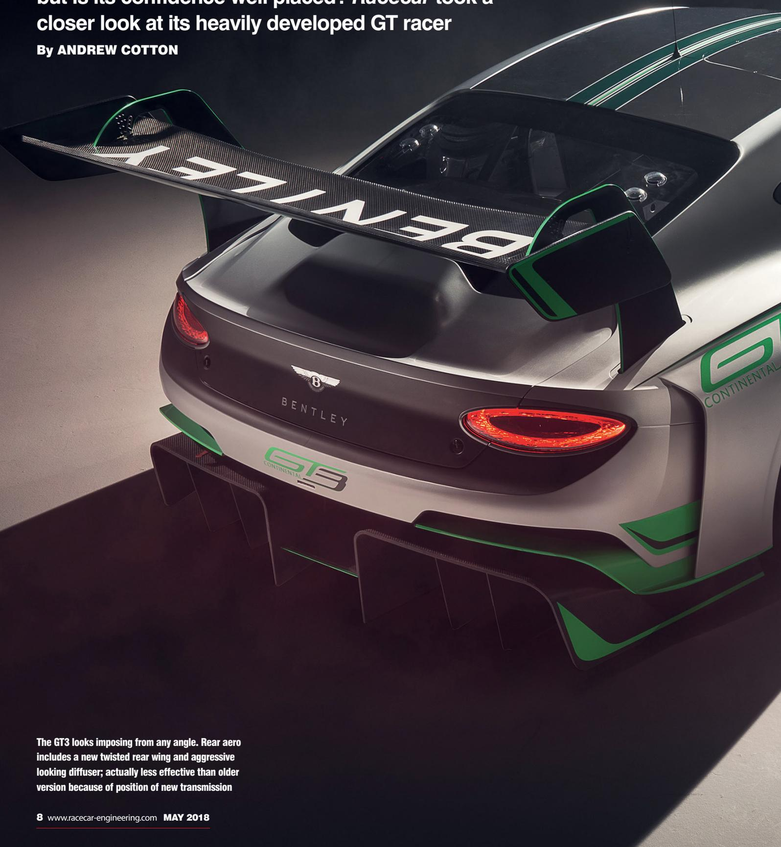
The GT3 looks imposing from any angle. Rear aero includes a new twisted rear wing and aggressive looking diffuser; actually less effective than older version because of position of new transmission
