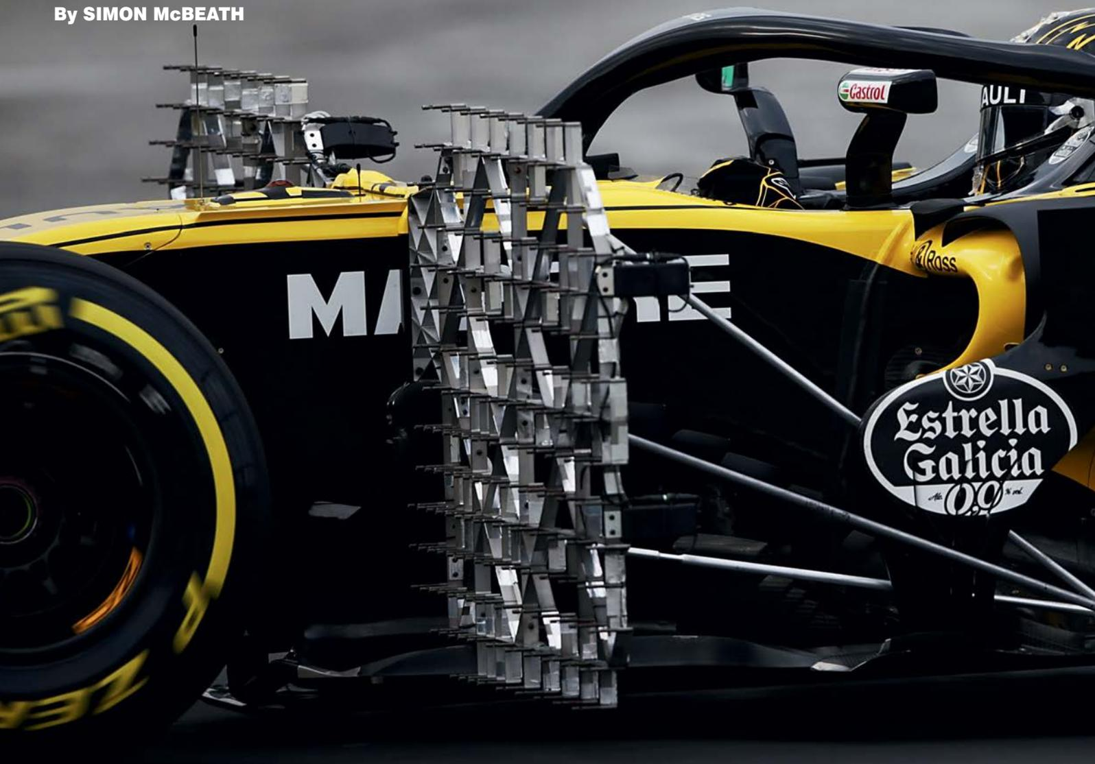
**P**hotographs of pre-season and pre-race testing often show top race teams, especially in F1, measuring aerodynamic pressures around their cars. The most obvious manifestation of this is the pressure sensor array, like a two-dimensional rake with pressure sensors arranged over the area of the rake, positioned on the racecar in key areas where what might be described as partial plane pressure plots can be logged and recorded.
