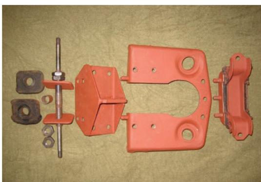
**Top:** The sub assembly and how it relates to the torsion bars
