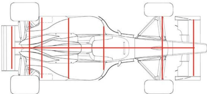
Figure 1: Schematic layout of tube runs in a conventional pressure scanning system
