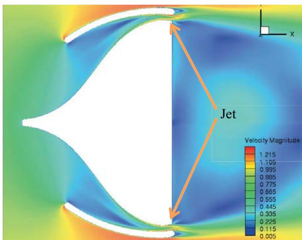
**Above:** Greg Woyczynski has suggested in an academic paper that the use of a duct on the leading edge of the wing mirror housing might be a good way to cut drag **Right:** These CFD images show the difference the internal shapes within the mirror's housing can make on the airflow
