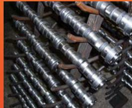
Operating CNC Landis and Adcole machines Polgain Limited manufactures Camshafts, from any material including chill iron castings, nitrided, tuftrided and case hardened steel. Customers include the OEM as well as the after-market and engine re-conditioners. Polgain can manage your camshaft project from profile advice and
