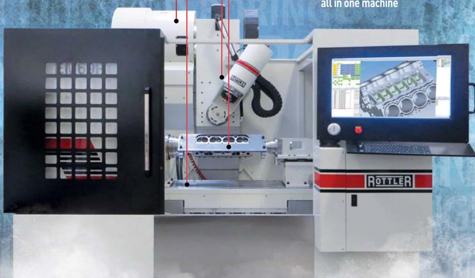
Linear Roller Bearing Slideways for faster movement and improved positioning accuracy
