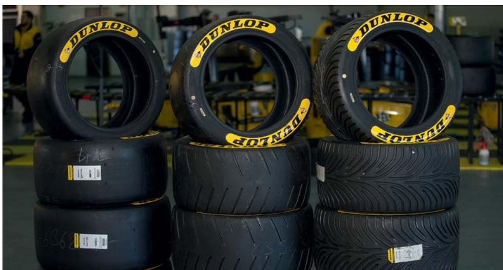
Dunlop supplies five different tyre specifications to its LMP2 teams: three types of slick, an intermediate and a wet. All five specs are new for 2018 and each of them features modified constructions and compounds as well as a wider working range
