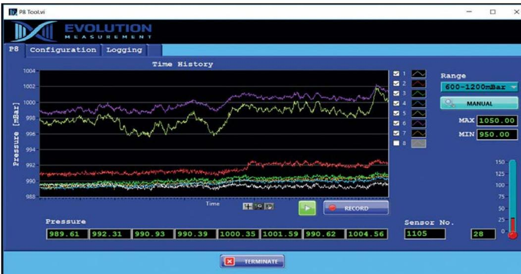
Figure 3: Screenshot of EvoScann GUI. Device has an onboard integral microprocessor so the output is in engineering units of pressure
