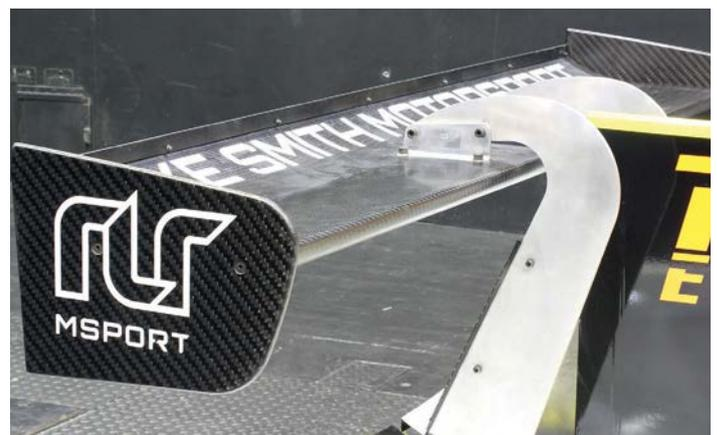
Steeper wing angle. It was possible to shave drag from the car with wing adjustments
