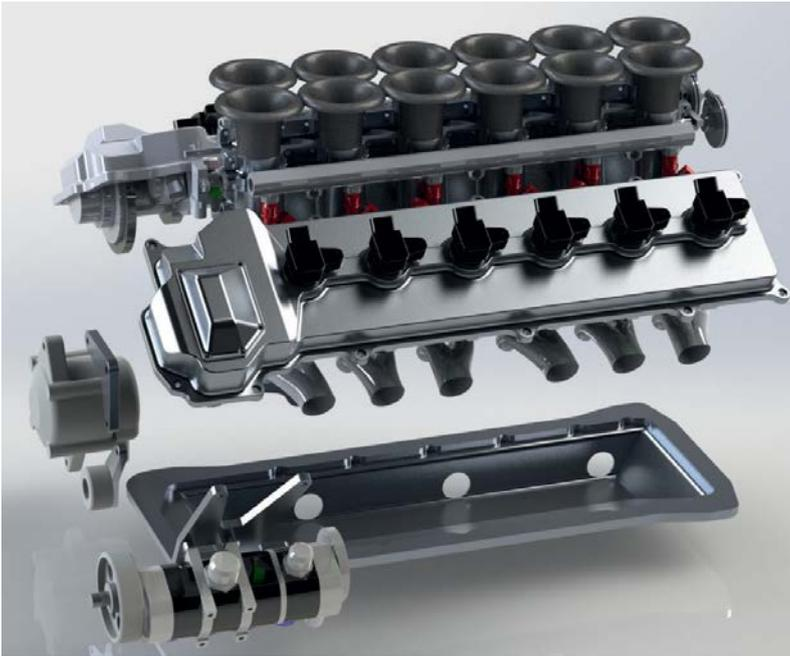
**Above:** Exploded view. The Hartley V12 is nothing short of an engineering masterpiece
