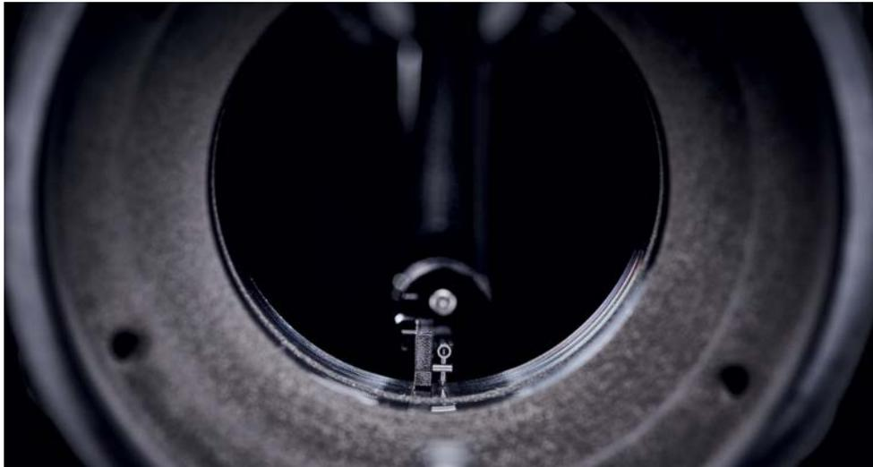
The SFP2 consists of a two micron radius diamond tip which deflects vertically as it's dragged across the surface of the component, going across the grain of the machining, thereby generating the signal in a similar way to a record player
