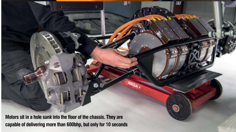
Motors sit in a hole sunk into the floor of the chassis. They are capable of delivering more than 600bhp, but only for 10 seconds
