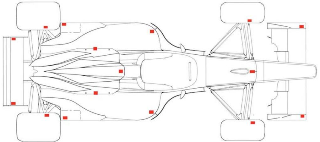
**Figure 2: A distributed pressure sensor system vastly reduces the length and complexity of the tubing and installation. It puts local scanners at the point of measurement, with the tubing installation then connecting via a single CANBus cable to the nearest node**
