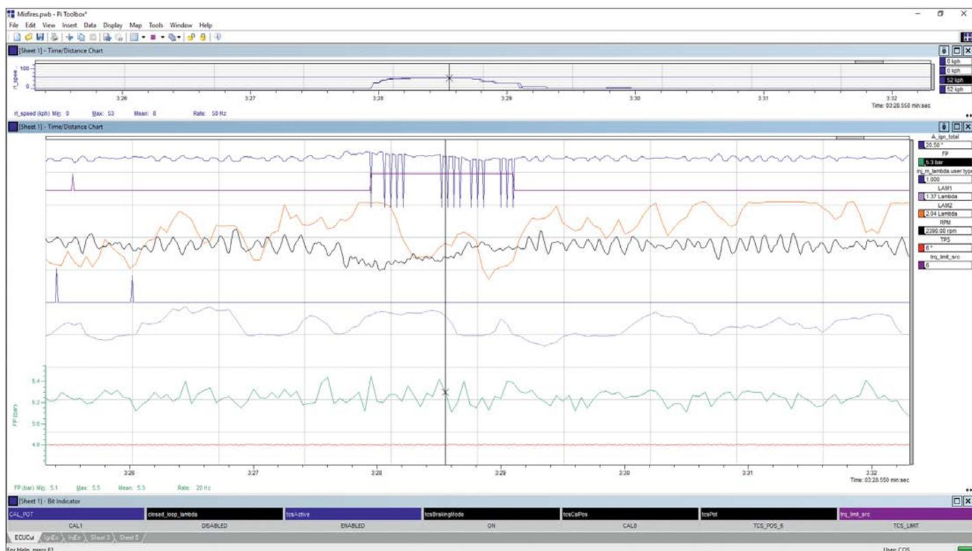
Figure 1: The fields along the bottom of the screen allow for a very quick diagnosis as to why the ignition cuts are being scheduled, so this is easily resolved
