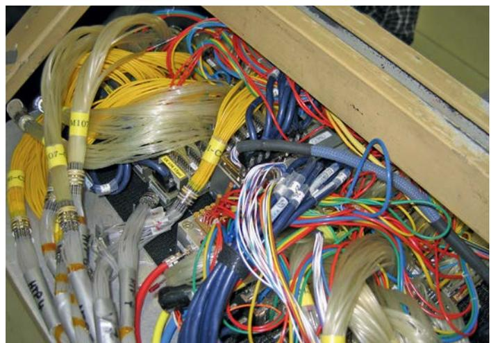
The schematic in Figure 1 might not look so complicated but in reality on a wind tunnel model (or a racecar) a conventional pressure scanning set-up can look more like this
