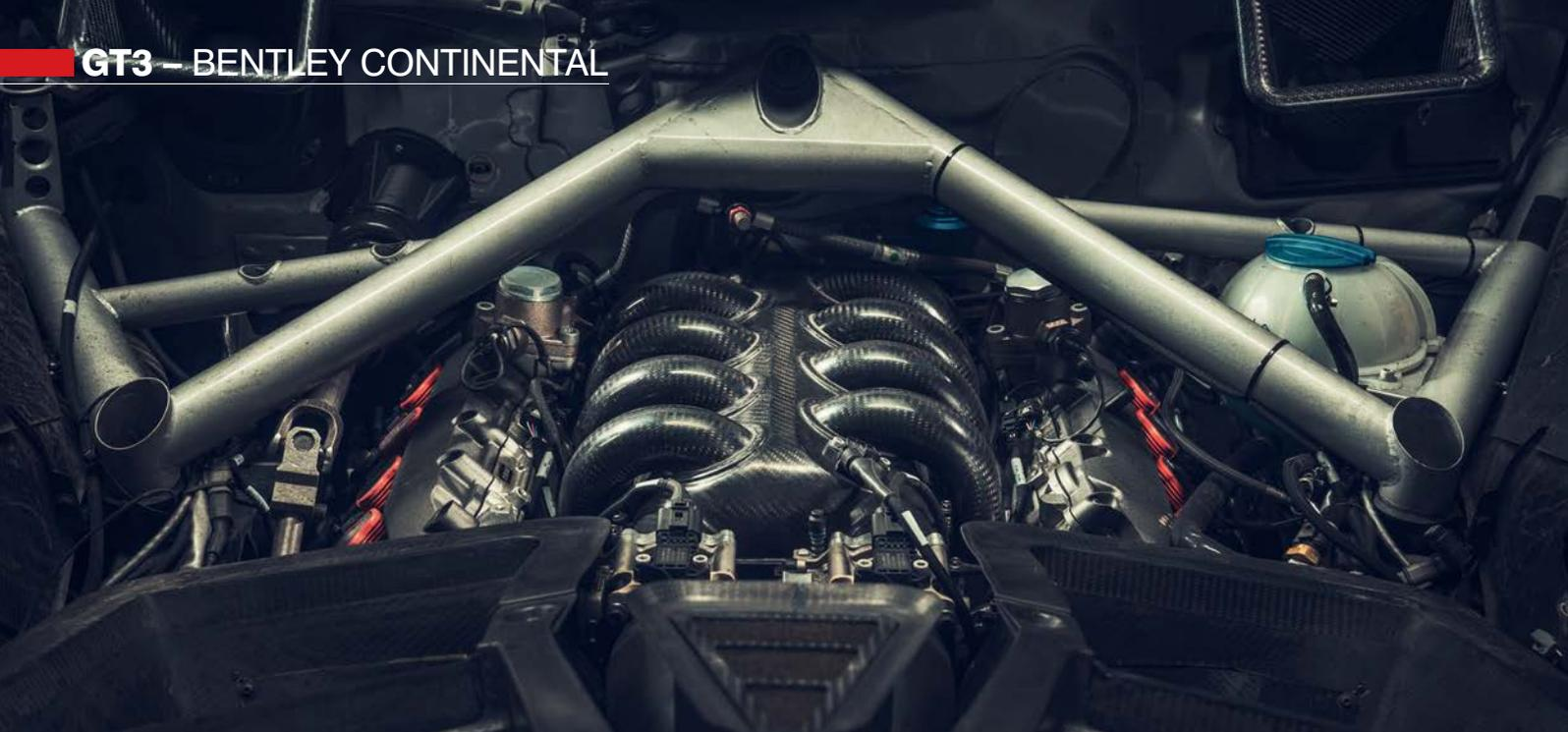
Bentley's opted to stick with the 4-litre V8 rather than switch to the W12 that's in the production version of the car; its decision based on the V8's proven reliability and fuel efficiency
