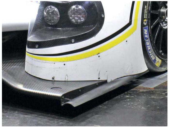
Removing the dive planes reduced drag by over four per cent, with a nice balance shift
