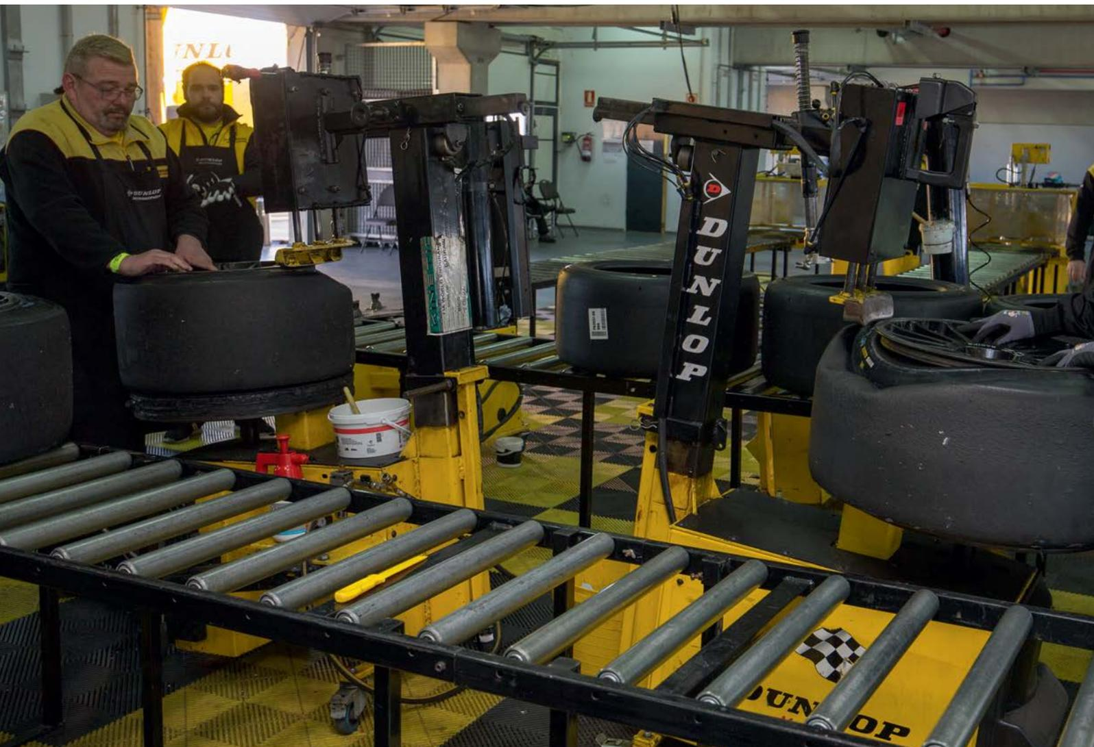
Race tyre manufacturers will fit the rubber to the race teams' rims. After they have been used the tyres are then removed by a machine, once the air has been bled out of them
