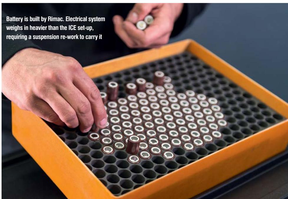
Battery is built by Rimac. Electrical system weighs in heavier than the ICE set-up, requiring a suspension re-work to carry it
