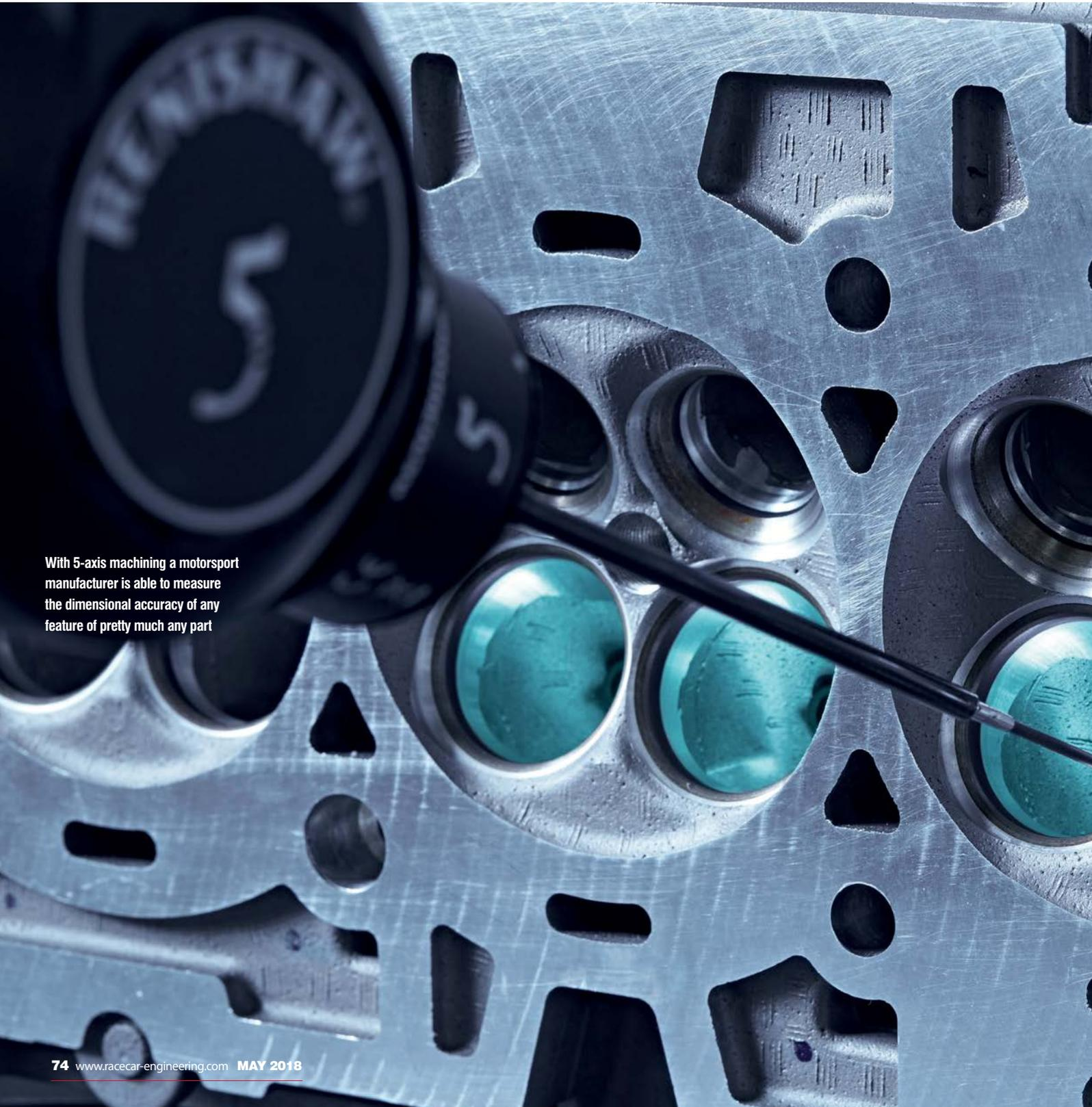
With 5-axis machining a motorsport manufacturer is able to measure the dimensional accuracy of any feature of pretty much any part
