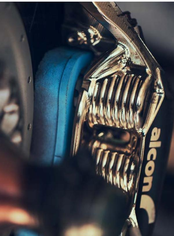
One of the big changes to the new Continental GT3 is a switch to Alcon brakes. The company now provides the discs and calipers (6-piston on the front and 4-piston on the rear) and the pedal box
