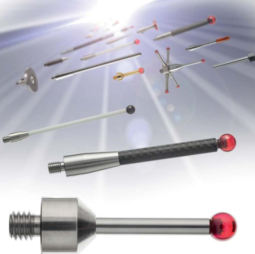
There are many different stylus combinations to suit any application or component. The stems are often made from carbon fibre while tips are usually ruby balls, as this is one of the hardest materials. Ceramic or tungsten carbide tips are also used
