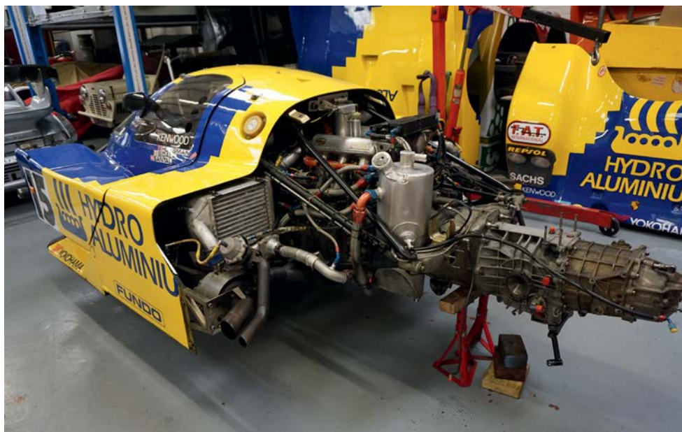
Disassembly begins. The gearbox was fully stripped and crack-tested and then rebuilt with a new crownwheel and pinion
