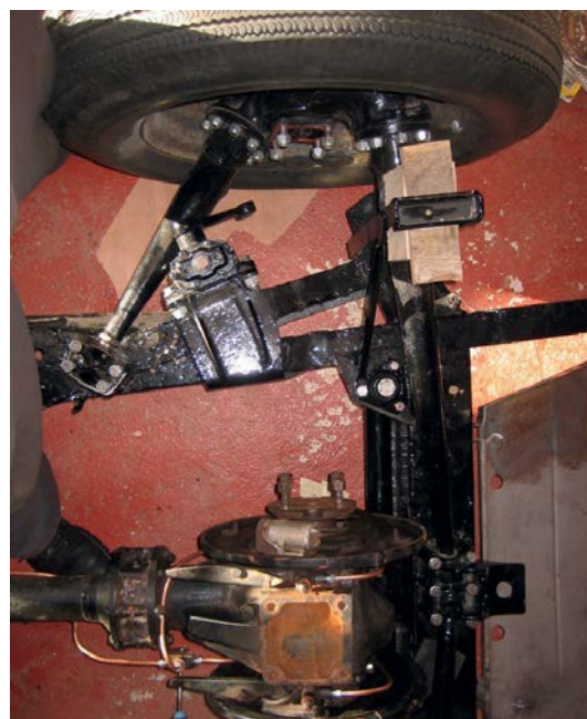
Typical Lagonda rear suspension; the wooden blocks are in place of the bump stops. The diff can be seen at the bottom
