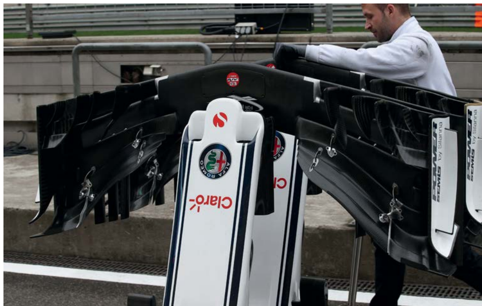
The front wing design is the result of an innovative new aero concept – note the ducts on either side of the impact structure
