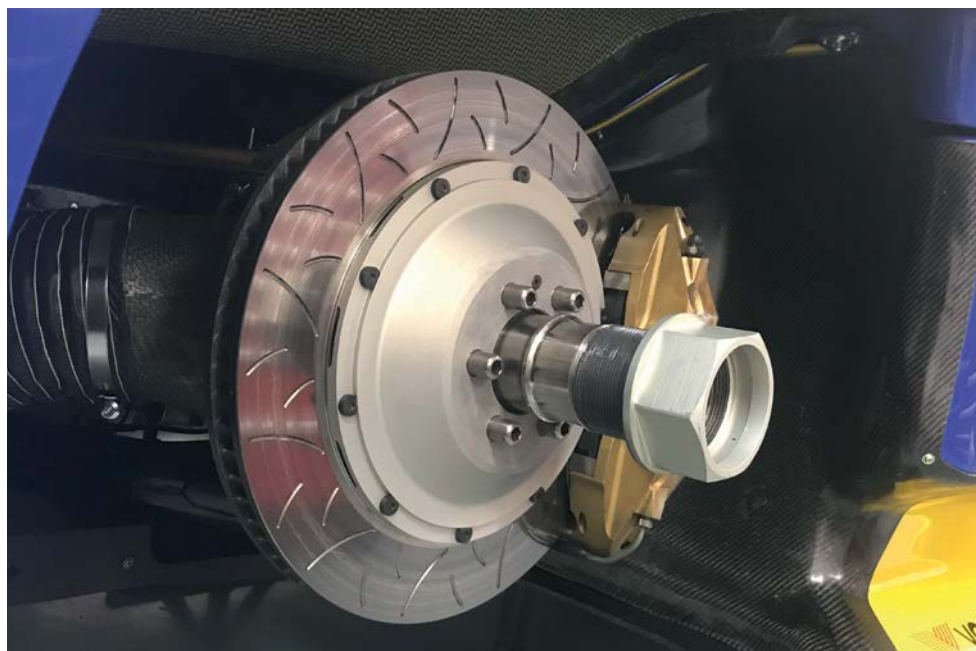
The car is still capable of 300kmh so many original parts were re-manufactured for safety reasons, including brake discs
