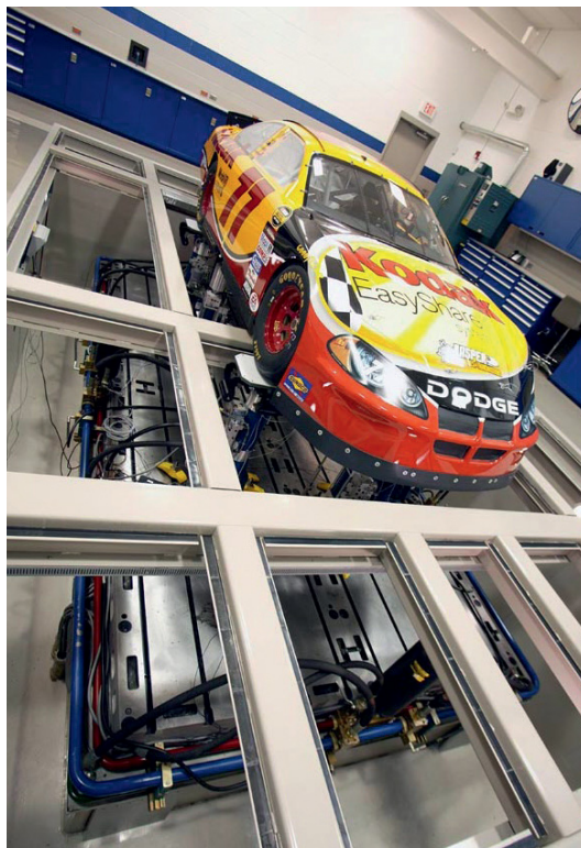
For oval track racers such as NASCAR stock cars the triangular configuration of the aeroloader actuators are often placed with two on one side and then one on the other, rather than one at the front and two at the back. This is to help replicate the lateral forces
