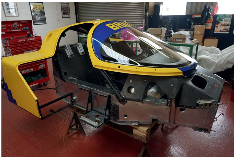
The tub is straight as the car was never involved in any major shunts when it raced, but there was a problem with the floor
