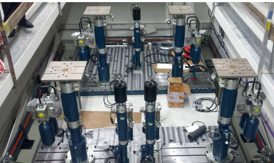
The seven-post rig at TRE, which is equipped with Servotest running gear. You can see in this picture the four wheel-pan actuators as well as the three aerolader actuators, complete with the compliant link at the top (the black cylinder section)
