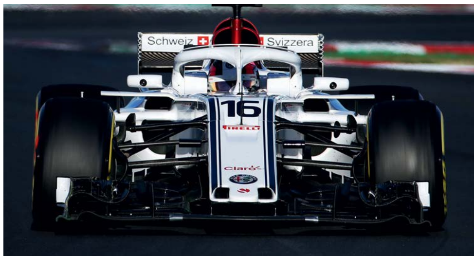
The C37 has a unique double-entry narrow sidepod design, said to be 10 per cent more efficient than a conventional layout
