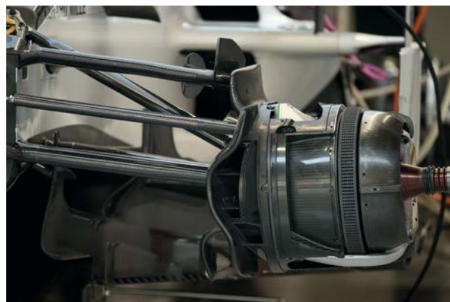
Sauber uses the upper front wishbone concept pioneered by Toro Rosso in 2017
