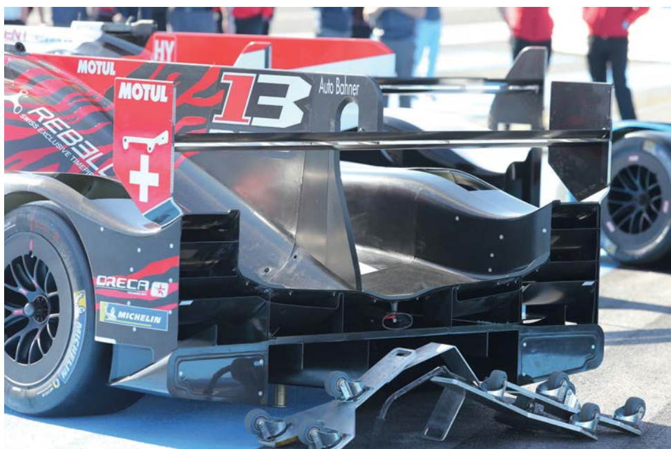
The rear diffuser is a tightly regulated part so ORECA has concentrated on improving the under-car airflow that feeds into it
