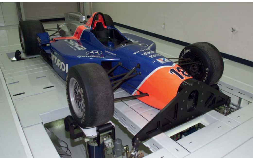
The main tests conducted on seven-post rigs are sine sweeps which help to characterise the suspension, and track replays where constructors or teams can tune the suspension set-up to optimise performance before the car actually hits the track
