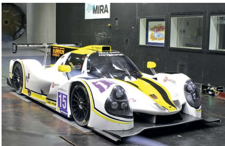
The mandatory front wheel arch apertures do allow the air to escape in a helpful manner
