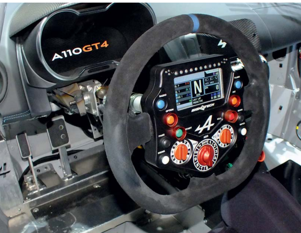
The steering wheel and dash has been especially designed by XAP for the A110 and is similar in concept to an LMP2 wheel
