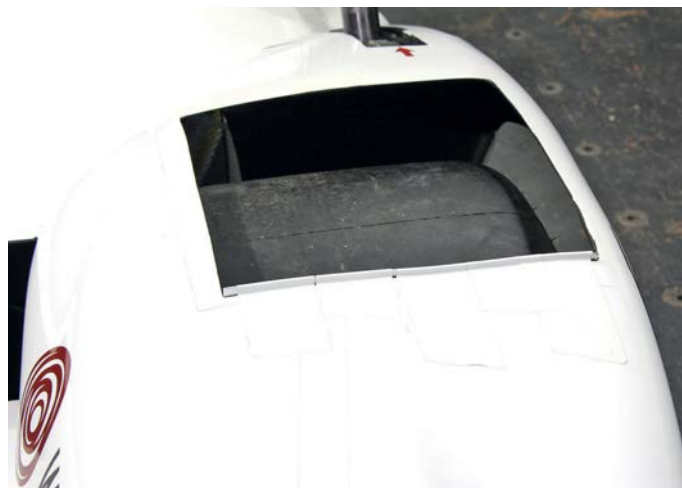
Gurneys on the leading edges of the front wheel apertures were found to be beneficial
