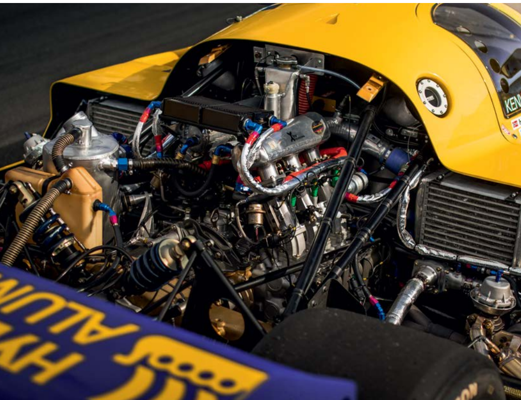
New water radiators were fabricated while the original oil coolers and intercoolers were restored to an as-new condition
