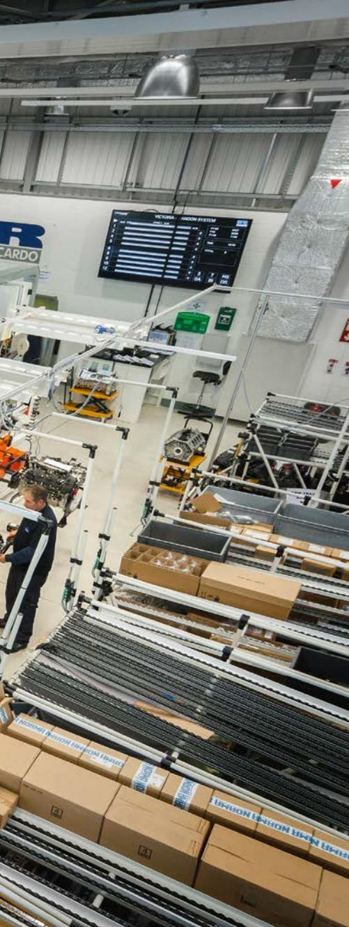
The process consists of 10 stations, each with a 40 minute cycle time. The engines move through each stage along the horizontal indexing line
