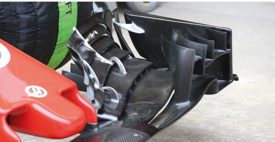
Arrays of additional front wing elements, as seen here on the Haas at the leading edge of the wing, have been used by all of the Formula 1 teams in 2018. These have now been banned in the new 2019 aero regulations
