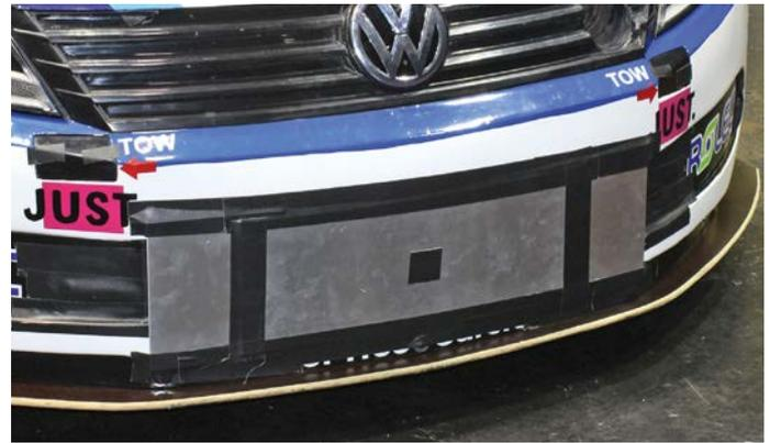
Blanking of the front ducts completely resulted in a modest decrease in the car's drag
