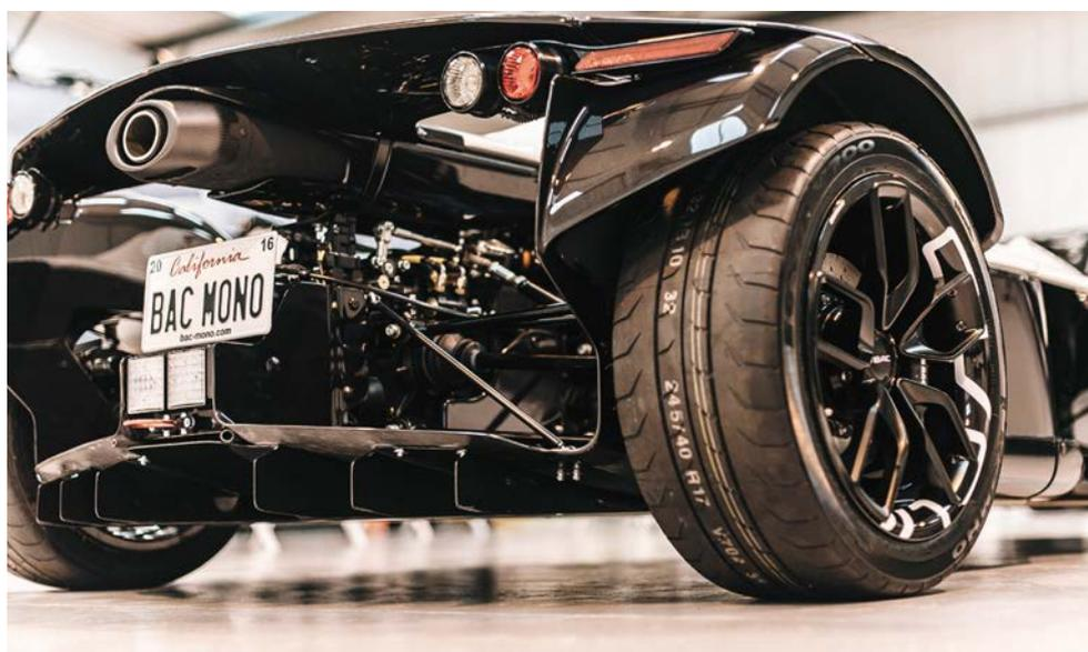
A Mountune-built Ford Duratec sits in the back of the Mono. Rear arches are made of graphene-enhanced carbon composite
