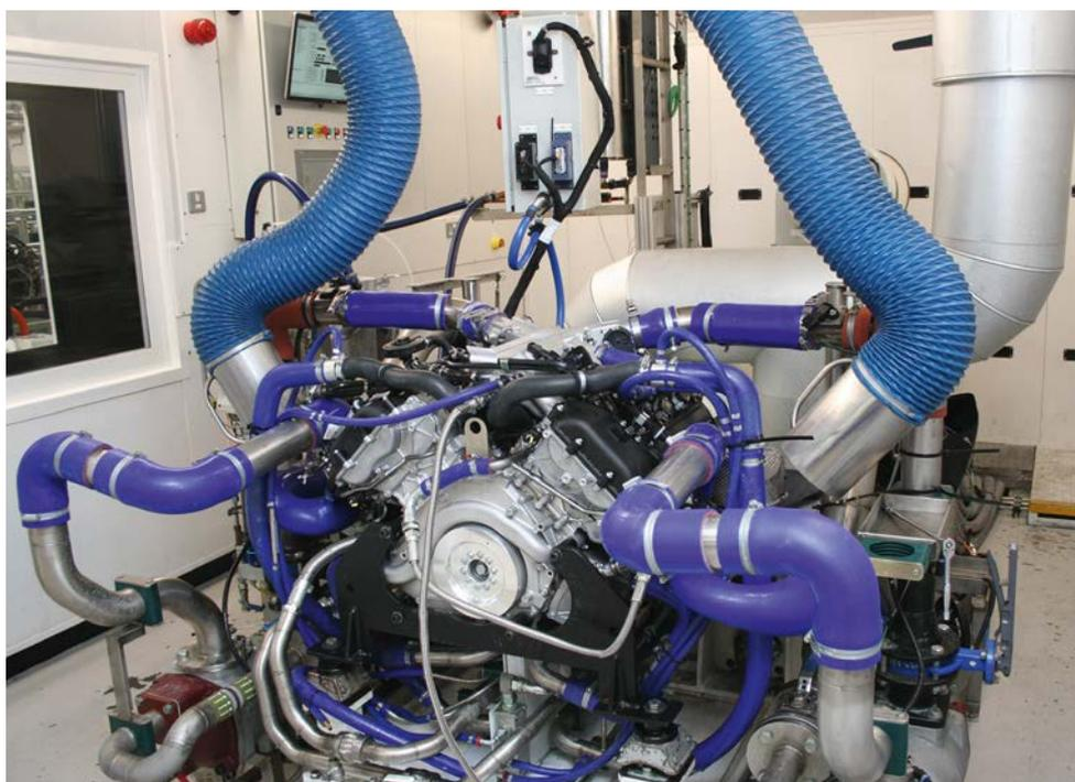
Once the McLaren engines come off the production line they are secured into moveable palletised engine subframes where the necessary piping is connected so that the finished powerplants can be run on the dyno. Every single engine is hot tested
