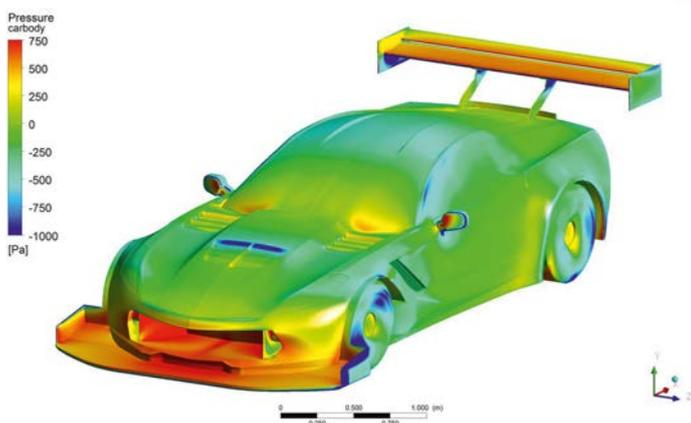
Figure 18: With wide splitter a near maximum wing angle was needed for aero balance
