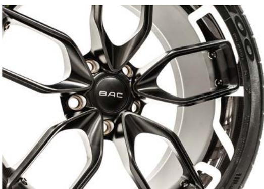
The Mono uses a carbon fibre/aluminium hybrid wheel to help save weight. The tyres have been specially developed by Kumho
