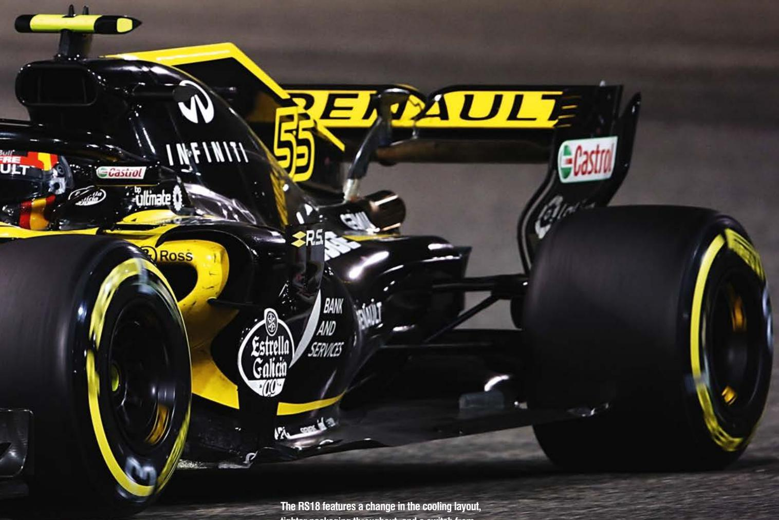
The RS18 features a change in the cooling layout, tighter packaging throughout, and a switch from a titanium to a composite gearbox. At the time of writing Renault was fourth in the championship
