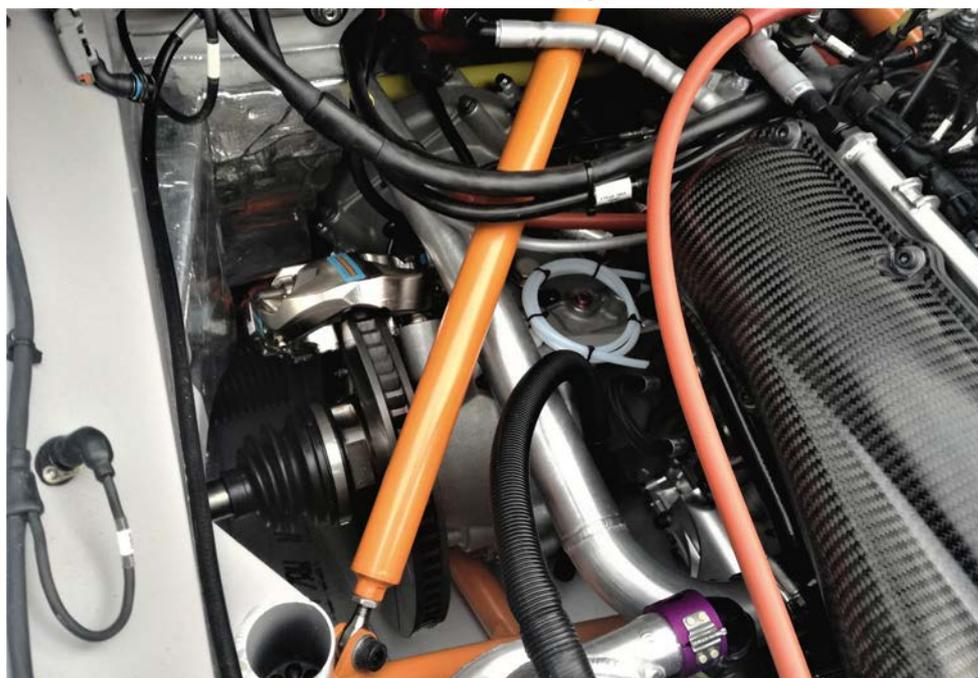
Prodrive decided on an inboard braking system to reduce unsprung mass while also allowing a degree of freedom with the suspension geometry. The brake calipers are fixed to the gearbox on the front axle and to the differential on the rear axle
