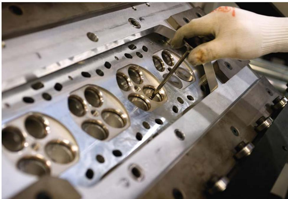
Ricardo's quality control is stringent. Here CMM probes are used to measure the geometries of the inlet and exhaust ports
