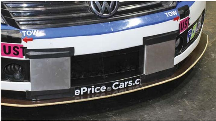
The front cooling duct was partly blocked; this reduced drag and gained some downforce
