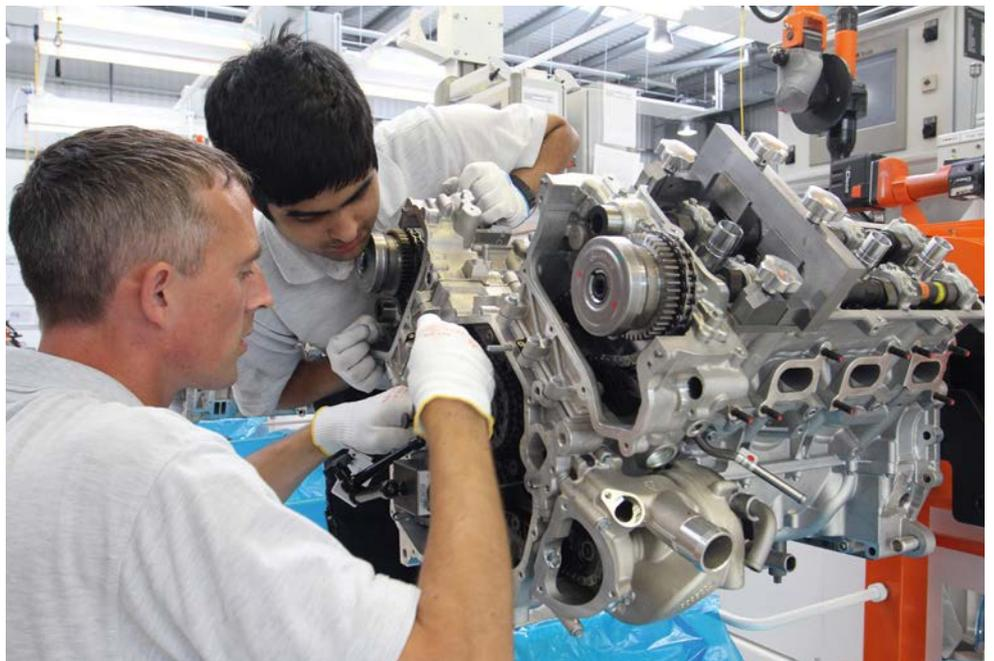
Each of the stations on the production line is equipped with an HMI screen which walks the Ricardo technician through the required tasks; from the tool that they should be using for the job to how much torque should be applied to each of the bolts
