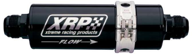
**71 SERIES** - Our largest capacity filters. 2.47" diameter; Two lengths. Reusable SS elements: 10, 20, 45, 60, 75, 100 or 120 micron; High-pressure core. Choice of AN style or Quick Disconnect end caps. Options include: differential pressure by-pass valve; auxiliary ports for temp probe, pressure regulator, etc.; Outlet caps with differential pressure gauge ports to measure pressure drop.
