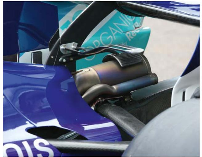
Aerodynamic parts around the exhaust tail pipe are very much track dependent
