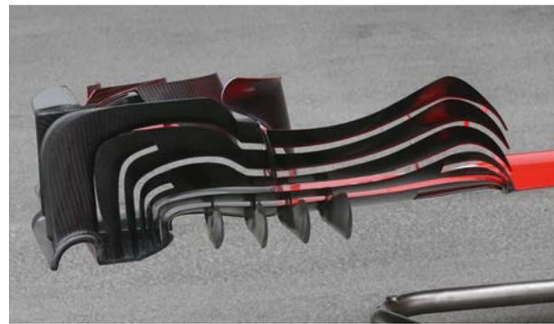
Only two strakes on each part of the underside of the front wing will be permitted when the new rules come into force. This year some teams have been using as many as four (Ferrari pictured)
