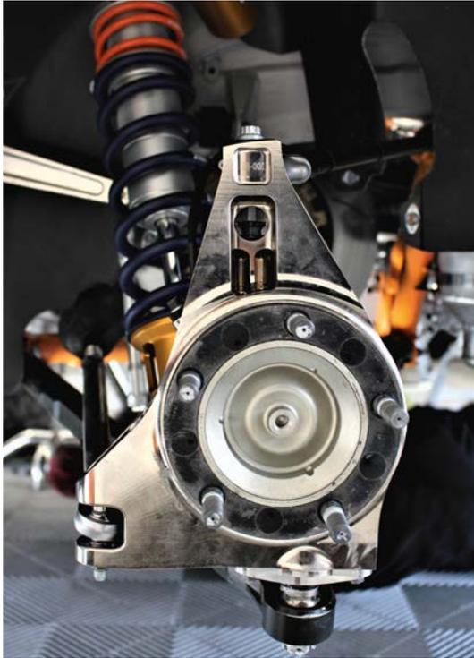
The wheel hubs do not need to accommodate brake calipers, discs or pads because of the Megane's clever inboard braking system
