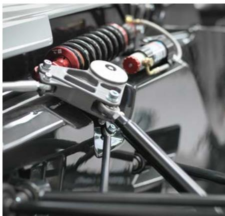
The suspension is a fully adjustable pushrod system with Sachs dampers. Such adjustability is crucial on a car that can be used both on the road and on the race track
