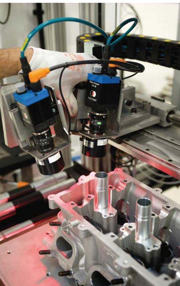
The inspection regime includes using vision sensors. These are used to check the quality of the components, specifically the surface finish and fitting, both essential to engine performance
