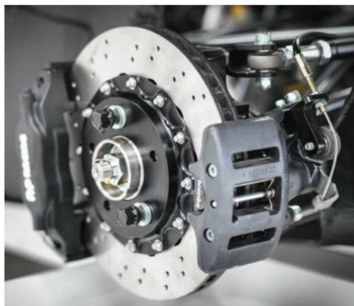
The brakes are race specification, featuring 295mm ventilated discs clamped by AP Racing calipers. Hi-tech ceramic brakes for the BAC Mono have been developed by Surface Transforms
