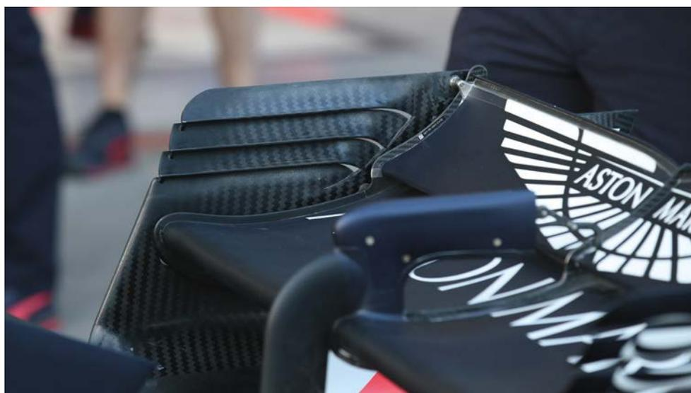
The rear wing endplates will increase in size but the vented sections (as seen here on this year's Red Bull) are to be banned
