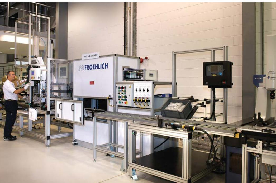
The cylinder head assembly line. This uses the same controlled manufacturing process as is used with the engines. The cylinder head is scanned at the beginning and the system then tells the technician exactly what to do and when to do it
