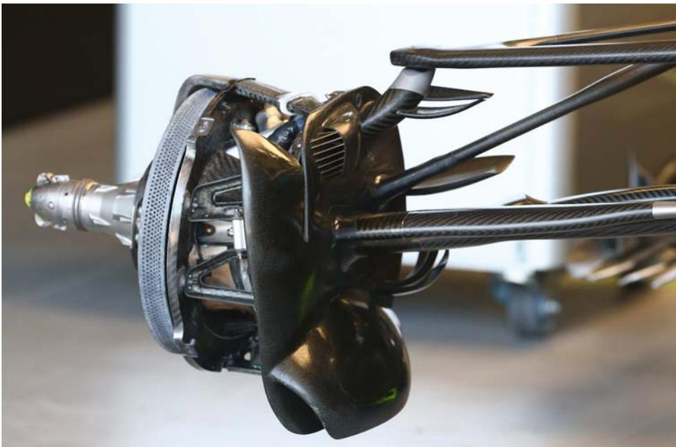
Currently there is a regulatory box around the inside of the front wheels where aero parts are essentially free but in 2019 the plate on the inner face of these wheels is to be simplified; so winglets such as these on the Mercedes will be outlawed
