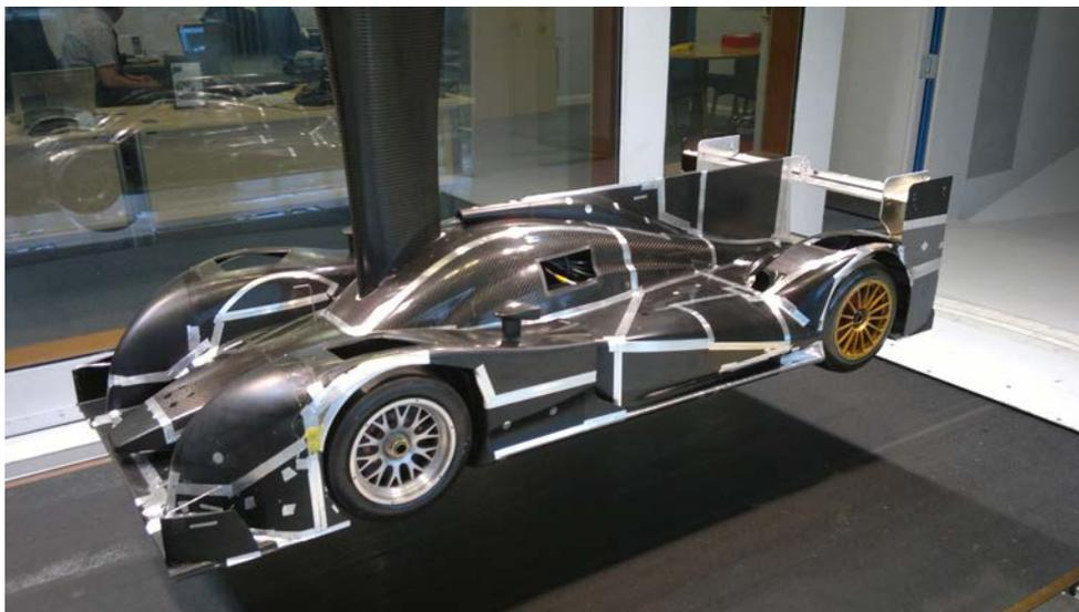
Each wind tunnel features a different design of boundary layer control, test space geometry and moving belt, which can lead to inaccuracies between them, so teams have to establish the correlation between the different tunnels (*Lola Wind Tunnel*)
