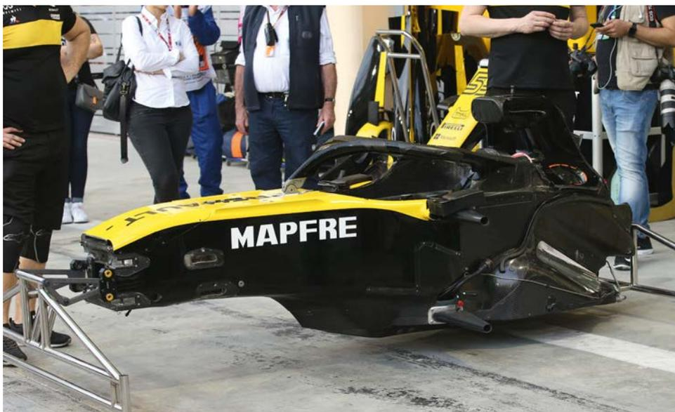
RS18 monocoque stripped down to its bare essentials. Weight reduction in the chassis was a major element of the car's design philosophy but Renault says this is still marginal and it has struggled to hit the weight limit
