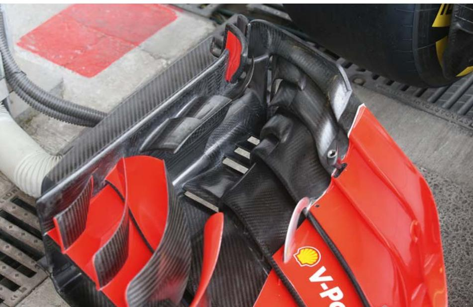
At the heart of the new regulations is a desire to do away with the vastly complex front wing arrangements that are a part and parcel of F1 (as seen here on the Ferrari) and the out-wash they are designed to create
