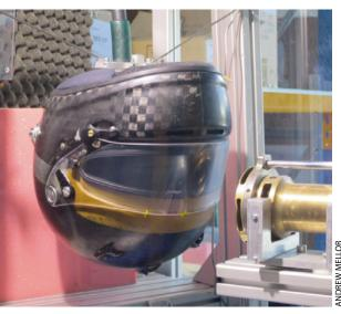
Being suspended, the helmet and headform are free to move longitudinally and laterally to achieve the right body dynamics
