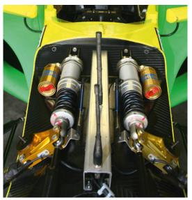
Shocks and coil springs in the usual relationship to each other. But what about springs that are placed within the dampers?
