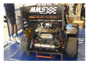
Both Monash cars feature pneumatically-controlled DRS on their substantial three-element rear wings. Note large rear diffuser, too
