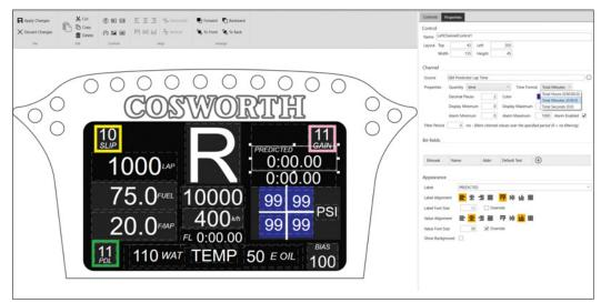
The display has an overlay feature which allows the driver to show only the relevant data at any appropriate time
