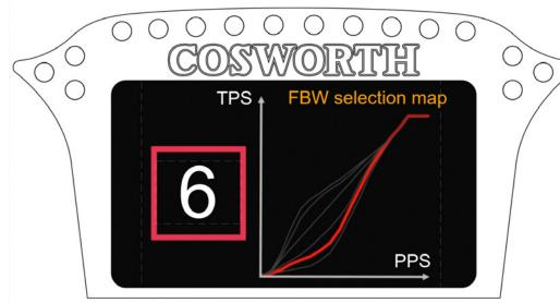
This overlay is driven by one user-configurable maths channel which is written within the Pi Toolset interface
