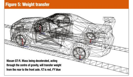
is commonly used in most turns; the driver coming off the brake gradually. Braking can also be used on a nominally full throttle corner to balance the racecar, as it will change chassis reaction either by anti-lift or anti-dive through its reaction of braking torque through the wishbones or suspension links.
