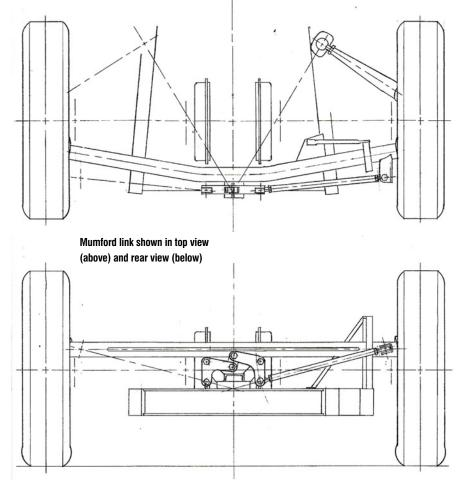
through the stock bump stop frame, which I have shown only on the right side; the left side has a mirror image one as well. These frames bolt to the main frame rails, so they can be slipped down over the De Dion tube.
