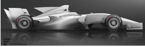
The SF19 is especially striking in profile thanks to its low nose, neat dorsal fin and the steeply raked rear wing assembly
