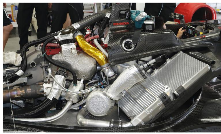
The elegant cooling system on the SF19 has been carried over from the SF14 – although like other parts of the car it has needed a rework as a result of the new low nose design
