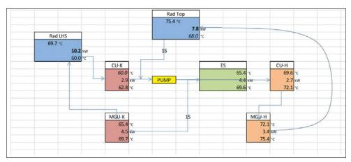
Figure 5: Team looked at integrating energy store cooling into the MGU-H circuit and making greater use of centreline cooler
