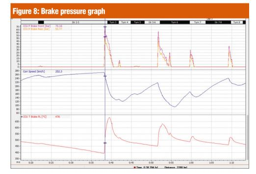
ceramics also coming into use on high range cars. Cast iron does not have a minimum operational temperature, they just have to be monitored to be sure they do not overheat, which can then boil the fluid in the calipers and 'lose' your pedal, but carbon has an ideal temperature for use. Carbon discs, for example, should be used above 350degC. If not they might glaze, which reduces the braking capacity, or worse, increases the wear.
