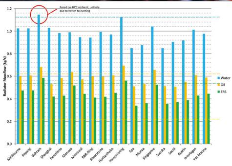
Figure 1: The first step was to map out the expected cooling demands over a season, including the extreme temperatures
