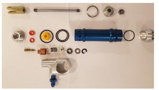
Edith Cowan produced many of its car's parts in-house including its own dampers, which are based on a design from Ohlins
