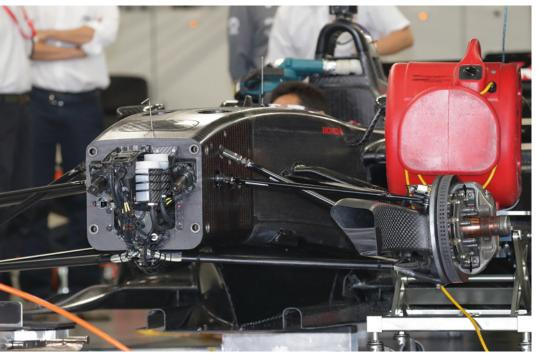
Despite the low nose the monocoque sits higher than its predecessor; this is to help increase the airflow to the underfloor
