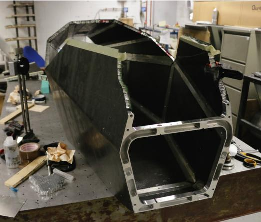
Despite the challenges of folding carbon fibre this seems to be the preferred solution for some teams, including Oxford Brookes which uses carbon fibre skins and aluminium honeycomb as shown here: top image is front and bottom is rear
