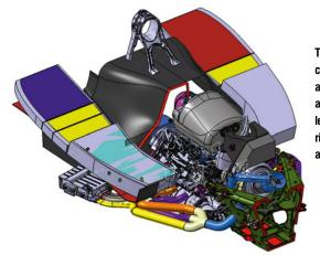
The final Caterham CT06 cooler layout. Two charge air coolers with ERS and oil and water coolers are on the left side, water cooler on the right. The gearbox cooler is above the turbocharger
