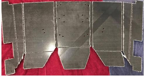
Cut and fold is a cheaper alternative to making moulds and doing a full composite layup. This is Edith Cowan's pattern for its monocoque. Note where the carbon fibre skins and the honeycomb have been CNC routed to allow the material to bend
