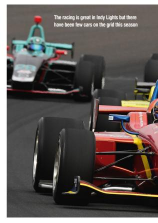
Tatuus-built USF-17, a full carbon composite and aluminium honeycomb monocoque chassis. Meanwhile, Pro Mazda has received its new car this season, the PM-18, which also uses the USF-17 chassis as a base, to help control the costs for teams who want to move up from USF2000.
