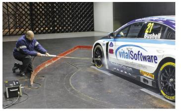
Boundary layer trip fence (the red strip above) had to be removed to fit a second car in
