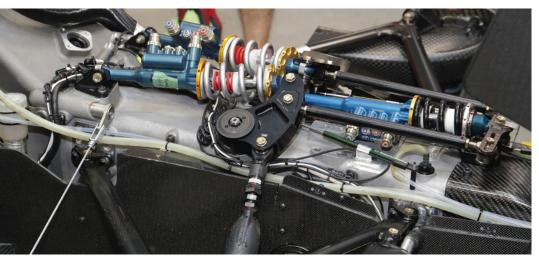
Rear suspension is a carry-over from the SF14. Dampers are free, which gives the engineers some scope to tune the cars
