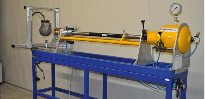
The projectile is loaded into the barrel of a pneumatic gun powered by a pre-charged reservoir of compressed air (this test rig was developed by the FIA and Newton Laboratories)
