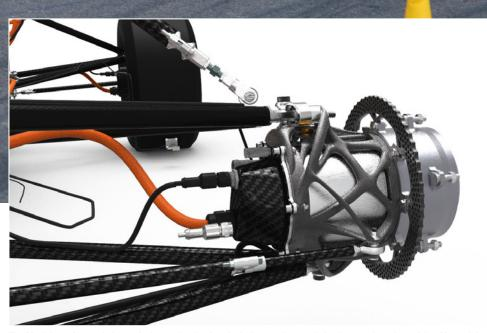
The Munich car featured plenty of advanced technology including topology optimisation to reduce the weight of its upright. It also made use of GKN metal additive manufacturing techniques to minimise the motor housing so to fit within the wheel hub
