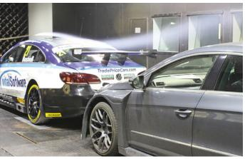
Pic 4: A closely following car reduced the effective angle of incidence of the rear wing
