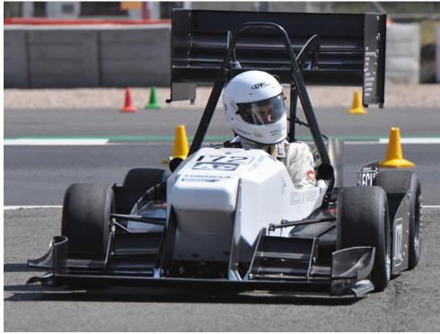
Top: A fully moulded monocoque, shown here on the Bath car, can achieve a much smoother curved profile which can be more aerodynamically efficient. Bottom: A car that makes use of a folded monocoque can have a more boxy appearance
