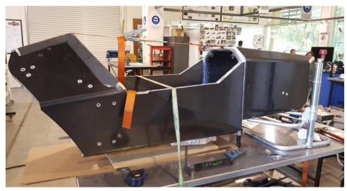
Once bent into shape the material needs to be accurately jigged and held together with ratchet straps while the glue cures, otherwise the chassis can move during the curing process which could result in inaccurate suspension mounting points
