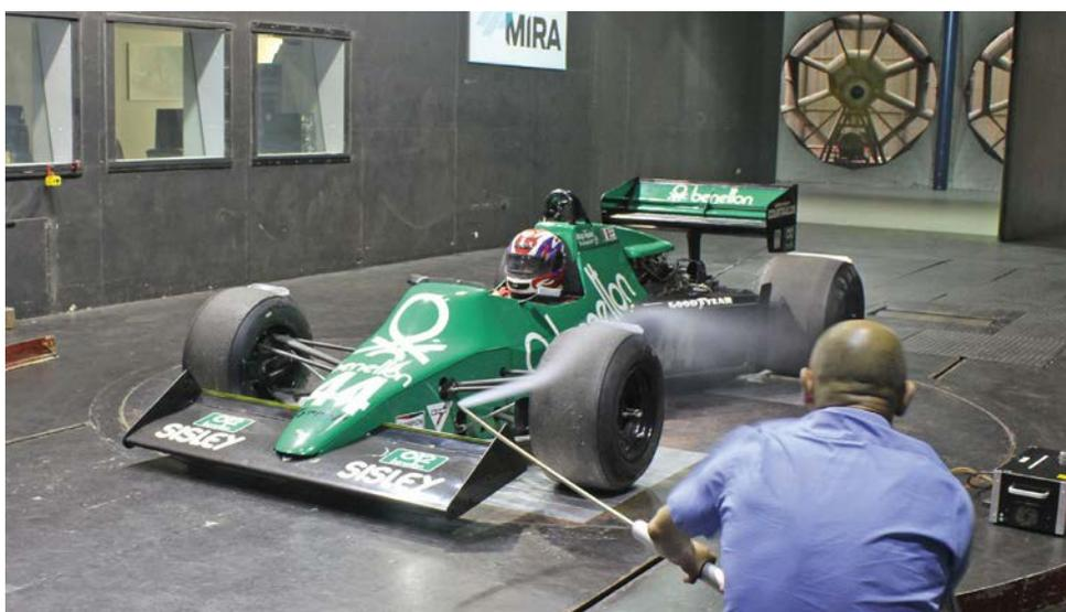
Tyrrell's 012 was the team's answer to the banning of ground effect sidepods for 1983. It featured a simple wing package, no sidepods and minimal floor area. Note the trip strips fitted to the wheels to better simulate the flows when wheels rotate
