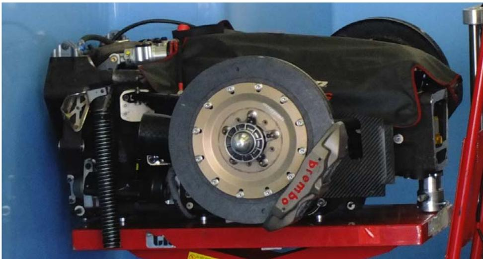
LMP1 brake discs have a larger diameter than those used in F1; it is possible the latter might use similar discs from 2021
