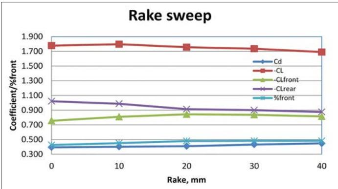
Figure 16: The rake at 60mm front ride height versus the car's aerodynamic coefficients
