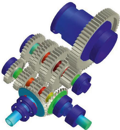
Real duty cycle data can be put into the Romax software which then helps Hewland determine exactly which bearing or gear mesh could be a limiting factor
