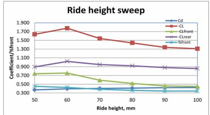
Figure 14: The effects of the ride height changes on the car's aerodynamic coefficients
