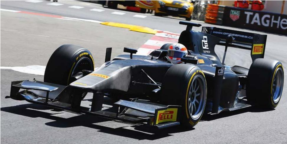
Pirelli tested 18in wheels fitted with low profile tyres on a GP2 car during a demonstration run at Monaco three years ago
