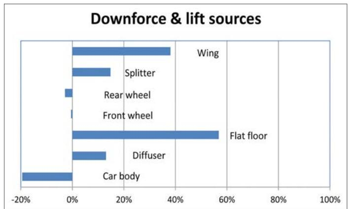
Figure 2: The sources of the downforce and lift; the car body also generated some lift
