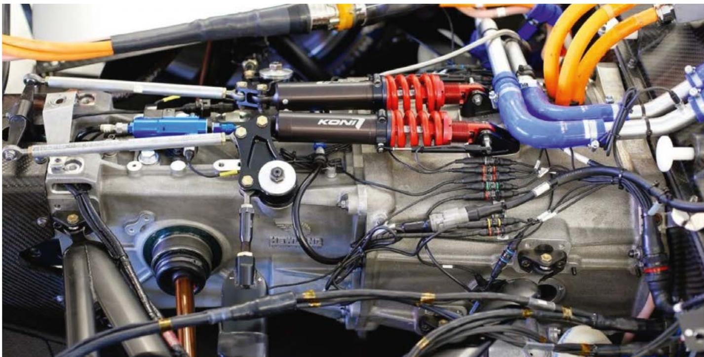
Hewland Formula E gearbox. Despite the slower speeds in FE designing a transmission to cope with the high regenerative loads from the electric motors has been a real challenge
