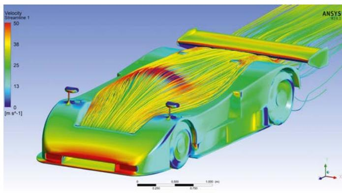
Figure 12: Streamlines from the car's radiator outlet impinged on the rear brake cooling
