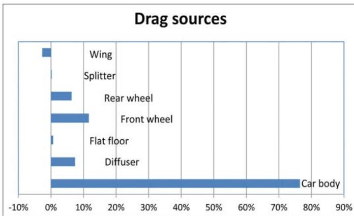
Figure 1: The sources of drag by major components; note the high number for car body
