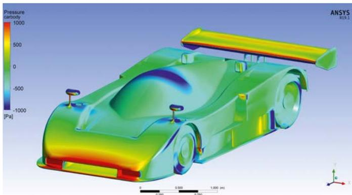
Figure 3: Surface pressure distributions; reds and yellows show the increased pressure
