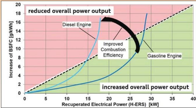
For a diesel engine the amount of electrical power that can be recuperated can lead to an increase in BSFC, resulting in increasing losses and overall lower power output
