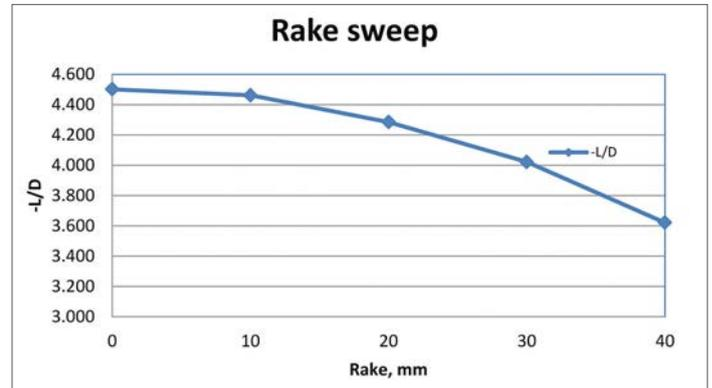
Figure 17: The rake at 60mm front ride height versus the aerodynamic efficiency (-L/D)
