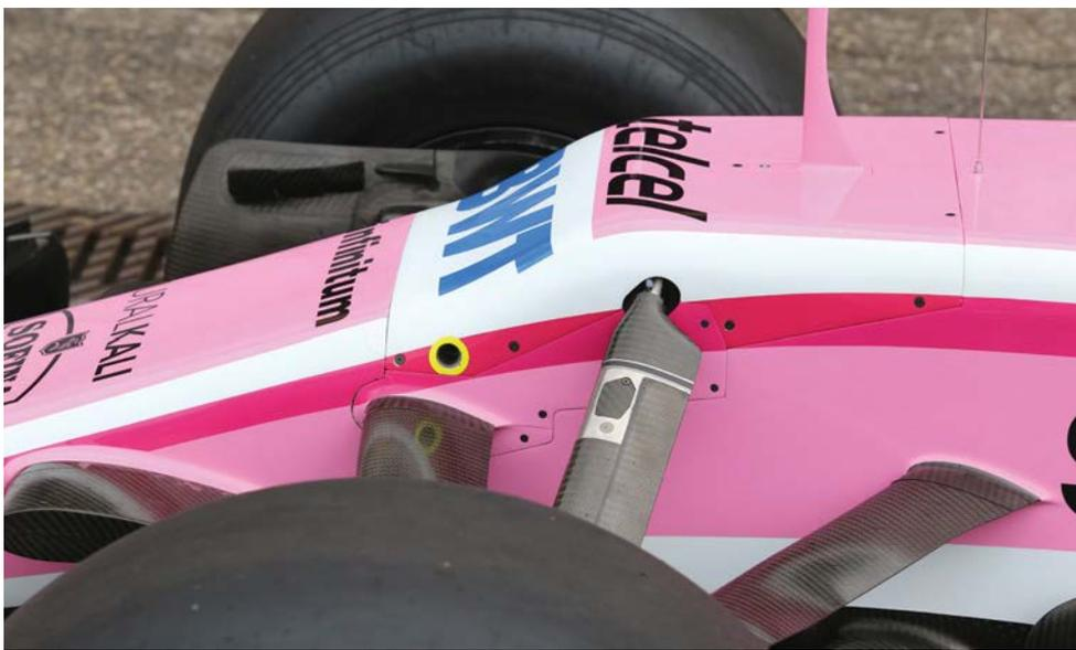
VJM11 retains the VJM10 nose with its slots either side of the front impact structure and unsightly hump on the chassis
