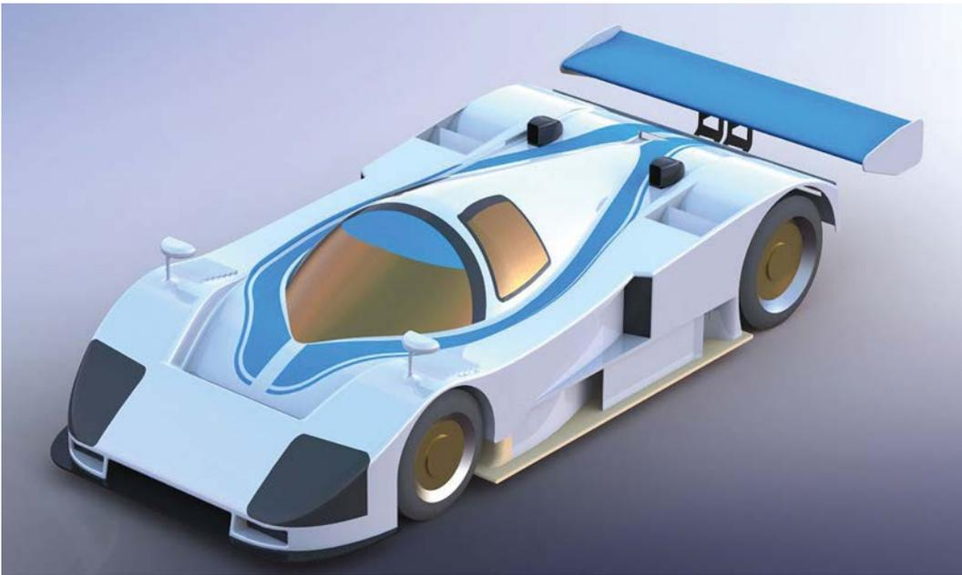
CAD rendering of Project MP787B's upper surfaces. The car is to be a full scale replica of the 1991 Mazda; MP stands for Mark Peters
