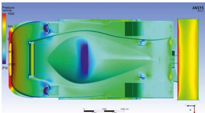
Figure 5: Top view shows where lift is generated over convex surfaces like wheel arches
