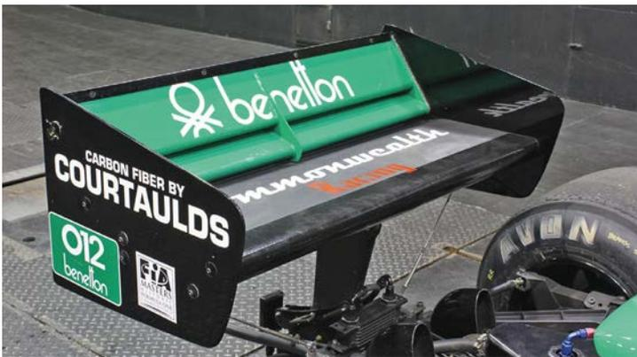
The O12's rear wing features a thick main element as well as a pair of steeply inclined flaps
