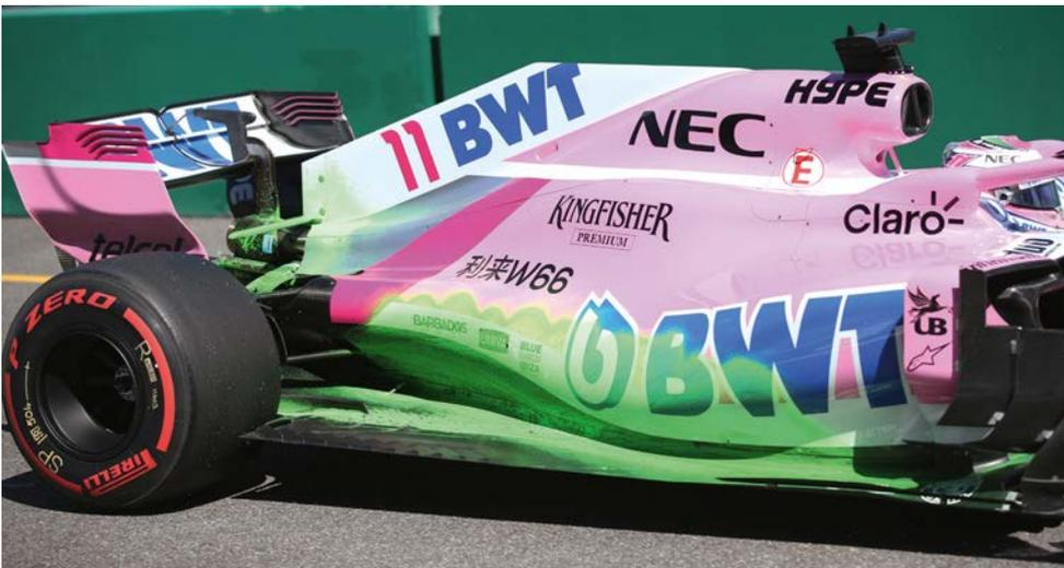
The flow around the sidepod was not behaving as expected and the team identified a correlation issue with the wind tunnel
