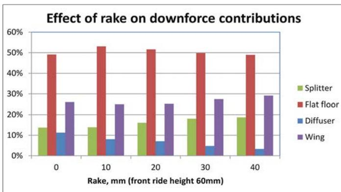
**Figure 18: Contributions of main downforce producers with 60mm front ride height rake**
