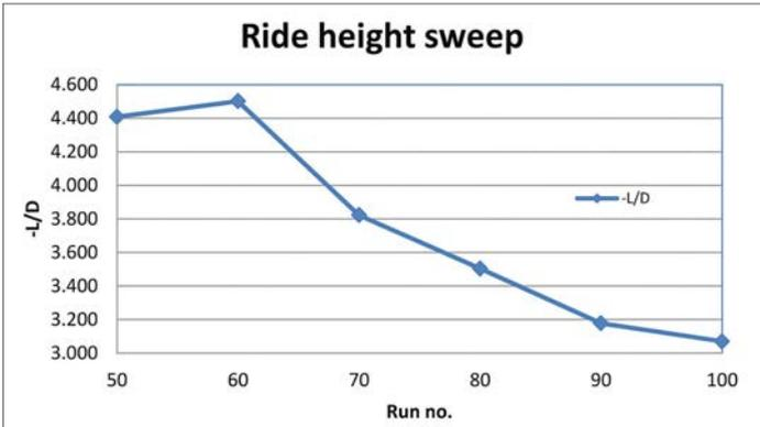
Figure 15: Ride height versus efficiency (-L/D). Drag reduced with each height reduction
