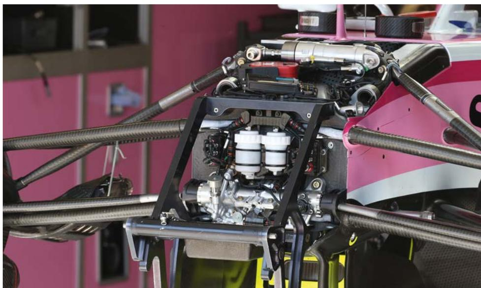
The front bulkhead showing the relocated steering rack. Torsion bar position has been carried over from last year's VJM10
