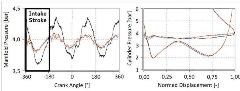
Figure 4: Comparison of the Y-cone airbox (blue) and single cone airbox (orange) against the original (black); see Figure 5
