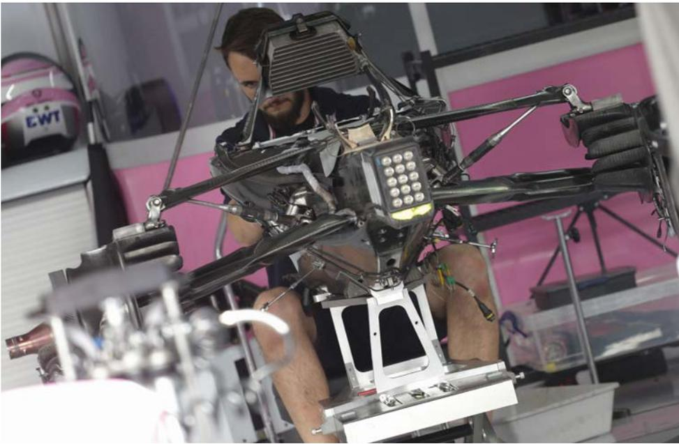
Use of the Mercedes transmission has meant Force India has had to develop a bespoke hydraulic rear suspension system
