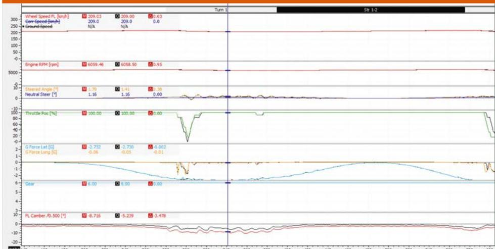
of the lateral forces divided by the racecar's wheelbase. As rough rules of thumb you want to be aiming for mid corner values of 0.05 with the occasional venture to 0.1 on turn-in. However these are *rough* rules of thumb.
