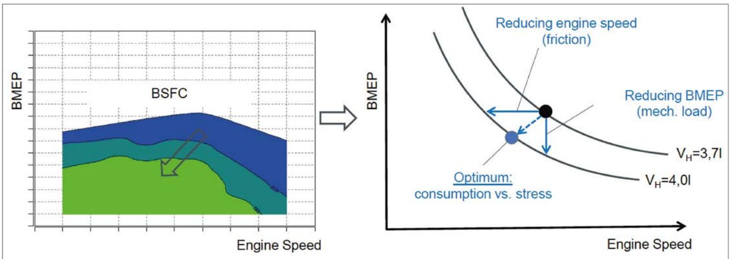
Figure 3: The increase in displacement from 3.7 to 4.0 was chosen on the basis that it not only improved fuel consumption for the same power but also reduced mechanical loads
