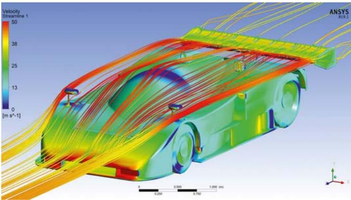
Figure 13: Rear wing received more or less freestream velocity flow despite low position
