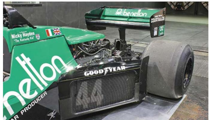
With no real sidepods the car's coolers were mounted in simple cowlings at the rear
