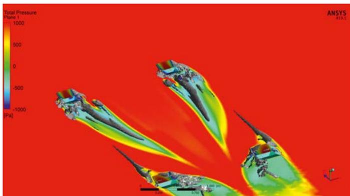
Figure 9: Vortex cores can be seen in the front wheel wakes; note the inward flow here
