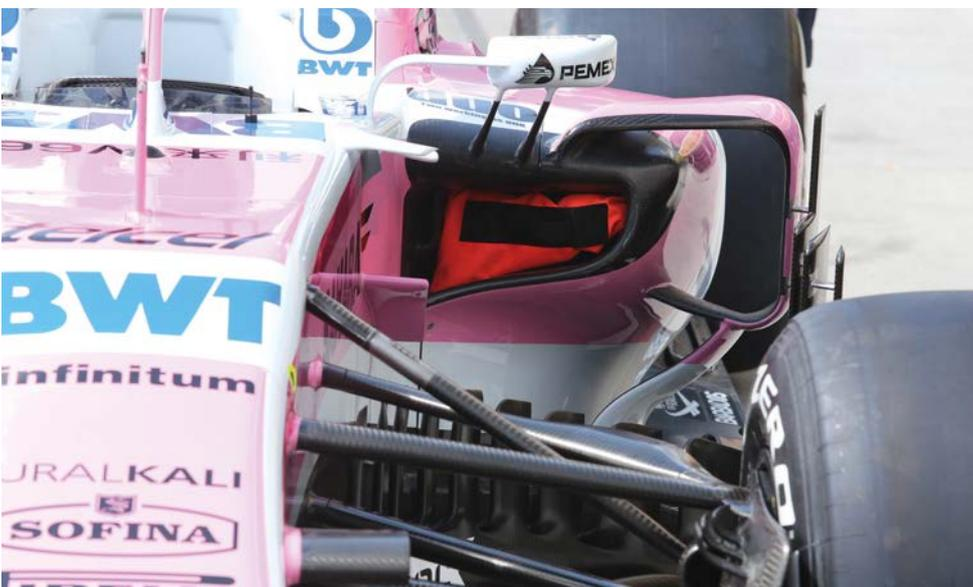
There has been work on the parts around the leading edge of the sidepods to keep the flow attached around the car's sides
