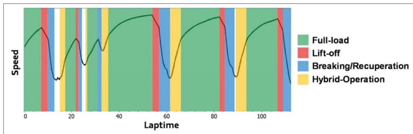
Figure 9: The driving strategy used during a Le Mans lap to stay within the regulations while achieving optimum use of the allowable fuel and hybrid energy restrictions
