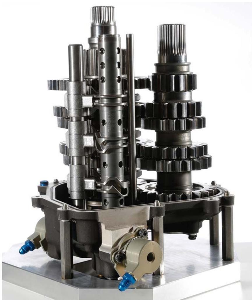
The gear cluster from Hewland's LMP2 transmission. The contact patches between the gear teeth need to be designed so the gears do not deflect or slide under load as this can generate heat, leading to inefficiencies
