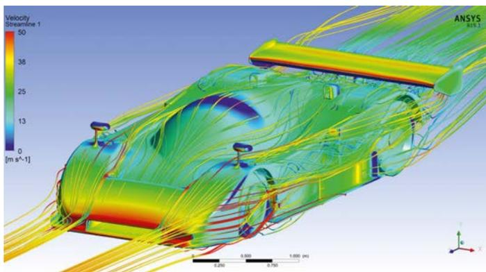
Figure 11: While the flow over the top of the car was tidy, it was less so along the sides
