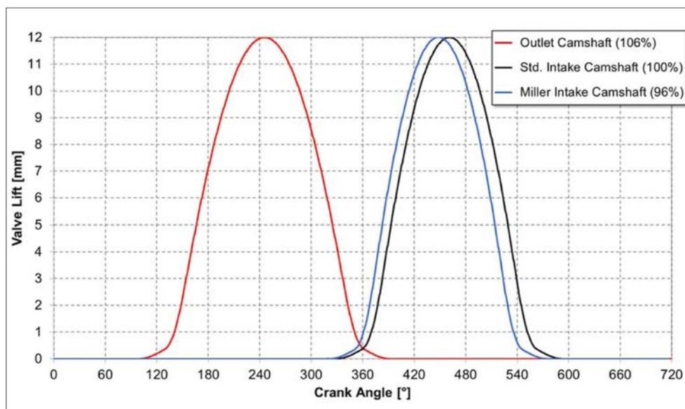
Figure 6: Valve lift curves comparing original inlet camshaft timing (black) with Miller inlet camshaft timing (blue). The latter opens the inlet valve earlier, allowing it to be larger and therefore maximising the inlet airflow into the combustion chamber
