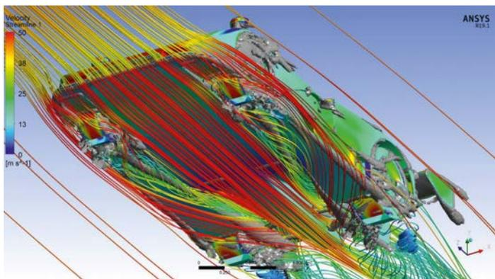
Figure 7: Superimposing the 'vortex core' feature highlights the vortices on underbody
