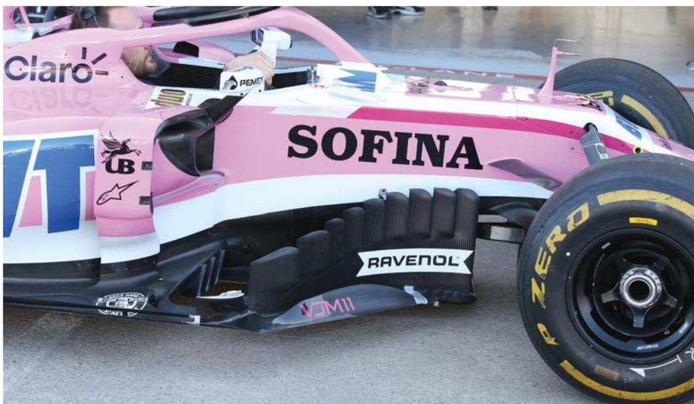
The area behind the front wheels is crucial for performance and its importance will grow in 2019 with the new aero regs
