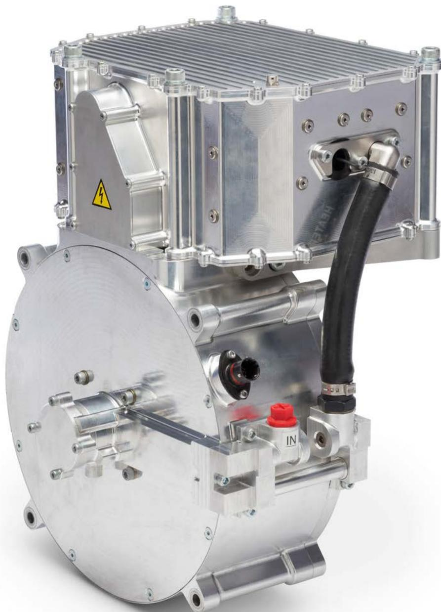
**Integral motor and inverter.** The front package weighs just 30kg while the rear is 5kg under that. Performance for the front motor is 270Nm and 270kW, while at the rear it is 460Nm and 280kW
