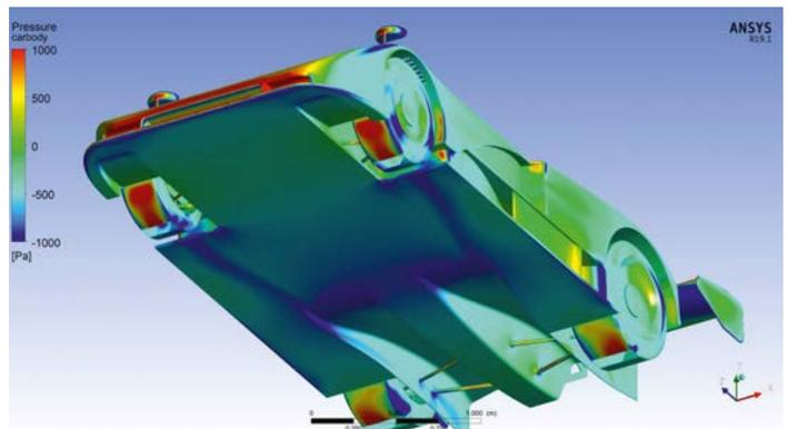
Figure 4: Pressure distributions on underside. Blue and green is decreased pressure
