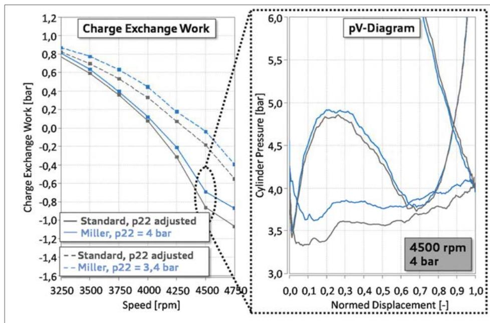
Figure 7: Comparison of the charge exchange work and the gas exchange loop of the original and the Miller camshaft timing
