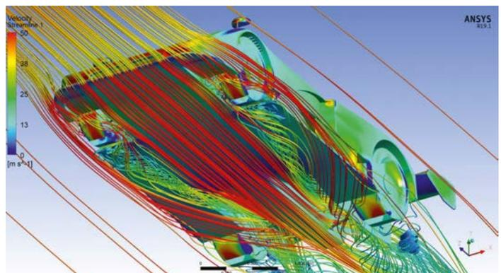
Figure 6: The streamlines show the 3D nature of the flows. Note the front wheel wakes
