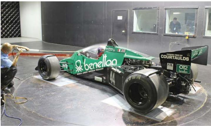
Note disrupted flow on centreline; one reason why low aspect ratio wings can be inefficient
