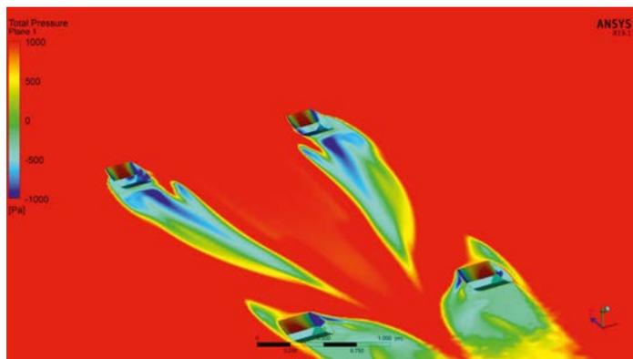
Figure 8: Plotting total pressure on a plane at 50mm above ground shows wheel wakes
