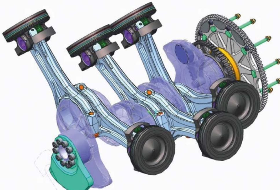
Engine architecture showing crankshaft and connecting rods. The location of the piston bowl (designed to ensure that fuel reaches the outer reaches of the combustion chamber) can be clearly seen along with other design elements of the piston
