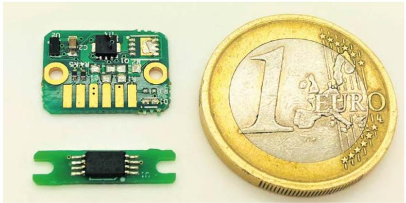
Top: Reventec's 2015 TMR sensing head. Bottom: Its tiny new 2018 150degC rated TMR sensing head
