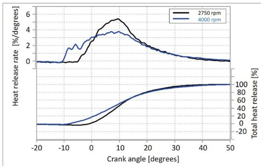
Figure 2: Heat release rate comparison between 2750rpm and 4000rpm. This shows optimum crank angle for maximum efficiency is 50 degrees which equates to 50 per cent mass fraction burned point of the combustion
