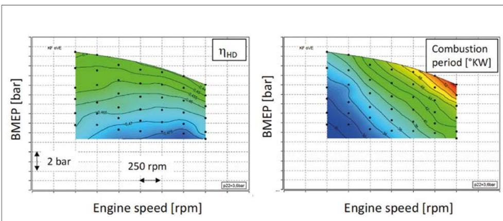
Figure 1: Typical map of 2013 unit. Left shows indicated combustion efficiency; right shows the period in the engine map
