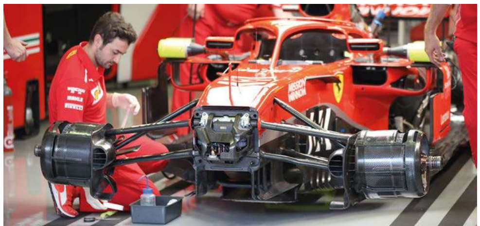
The maximum front overhang has been increased by 225mm to 1225mm. Could this be a new area for aero development?
