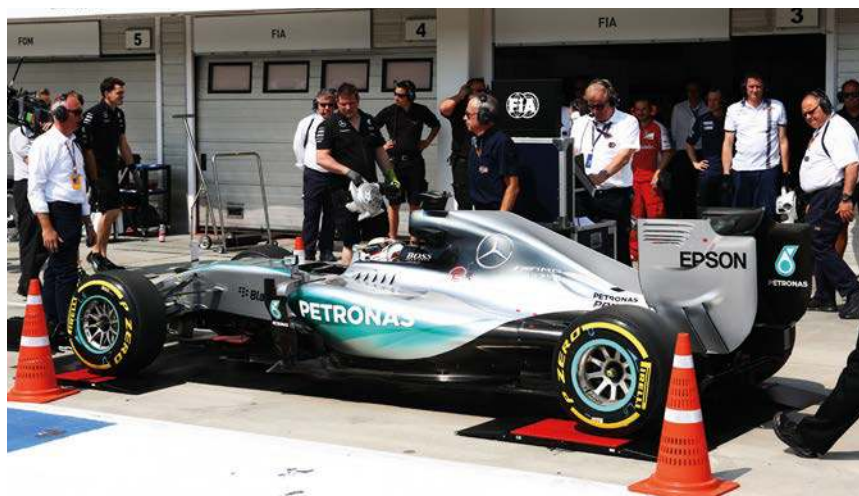
The minimum weight has been increased by 7kg to 740kg, making 2019's racers the heaviest F1 cars ever
