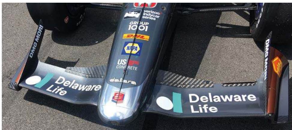
Front wing extensions were made available to the teams at Pocono in 2018 and will now also be used in the 2019 Indy 500
