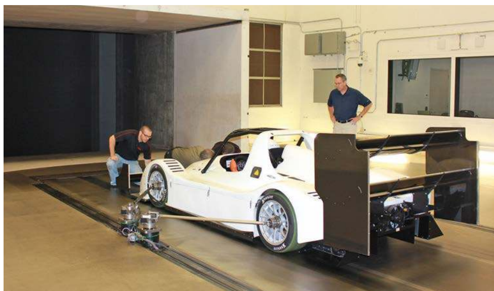
The sophisticated Windshear tunnel in North Carolina has a full width moving ground belt – this is the 2014 spec TRD/TMG EVP002 Pikes Peak electric Radical (Courtesy TRD). Other wind tunnels will have a central belt between the car's wheels
