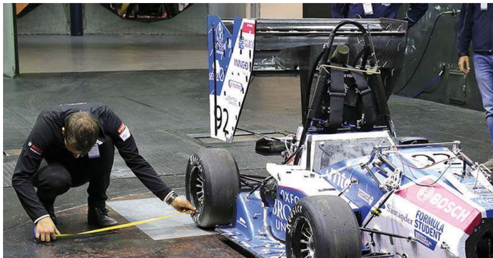
The car being carefully aligned on the load cells; supplying the wind tunnel with its dimensions before the session is crucial
