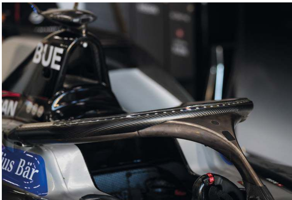
Another addition to the Gen2 car is the Halo, which is the exact same specification as that used in Formula 1
