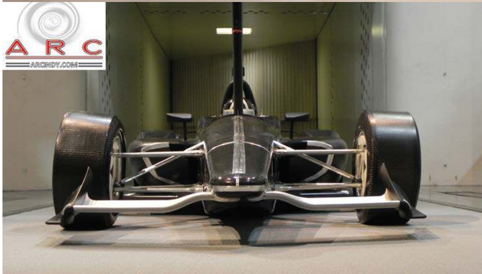
The 50 per cent scale UAK18 model in the ARC Wind Tunnel during aerodynamic testing. Courtesy of ARC
