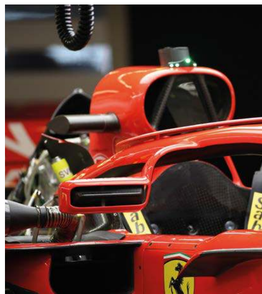
Ferrari's trick wing mirror designs in 2018 prompted the FIA to clamp down on the use of the supports as aerodynamic devices
