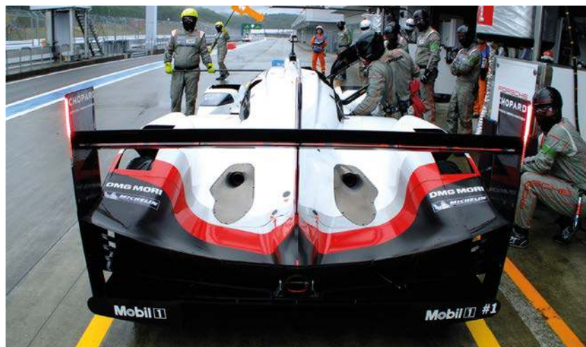
Formula 1 will now feature LED lights in the trailing edge of the rear wing endplates; as used on LMP cars
