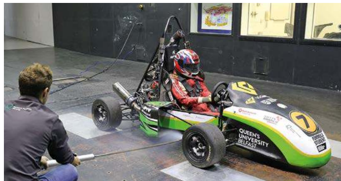
Visualising the flows into the 2017-spec radiator intakes on the Queen's University car
