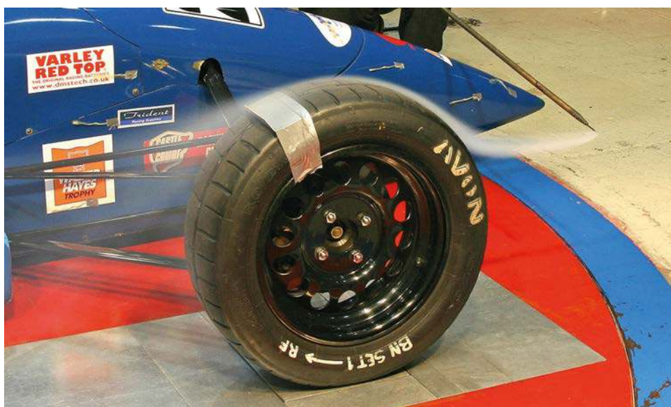
On open wheelers racecars trip strips can be used on stationary wheels to simulate their rotation more effectively
