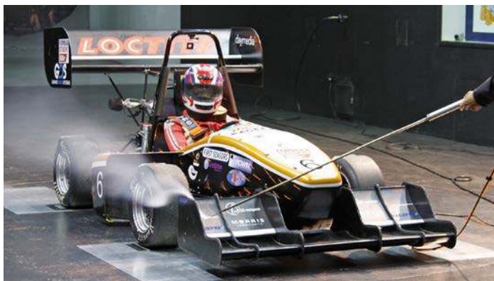
The University of Hertfordshire's 2013 Formula Student car ran with dual-element wings
