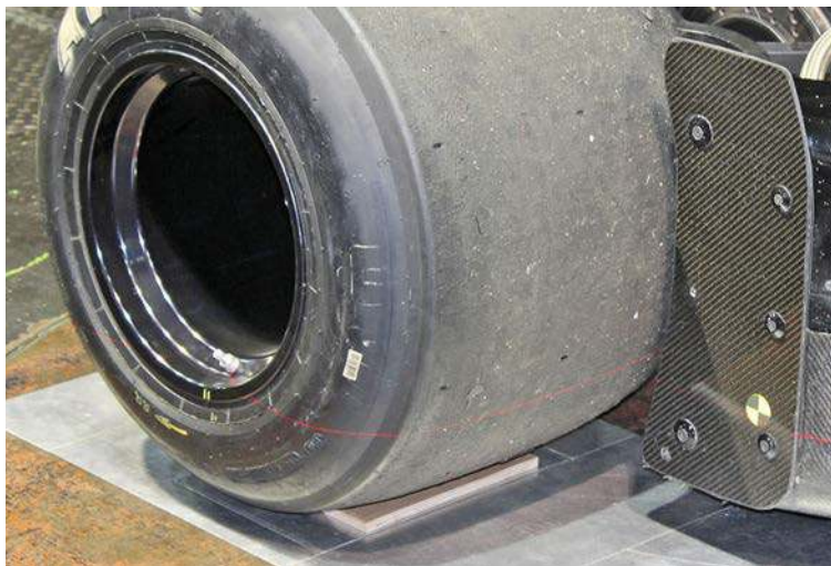
Wooden wheel shims that fit within the load cell periphery can be used to adjust the ride height
