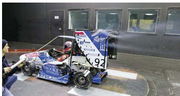
Here the smoke plume reveals the rear wing flow characteristics on the OBR18 FS car
