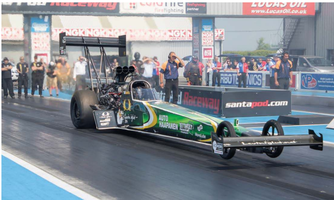
While combating drag is the name of the game, with so much power on tap a huge and very high rear wing is required. The more modest front wing is there to stabilise the dragster
