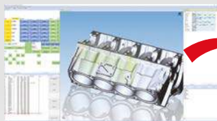
STEP file of V8 block imported into the machine computer
