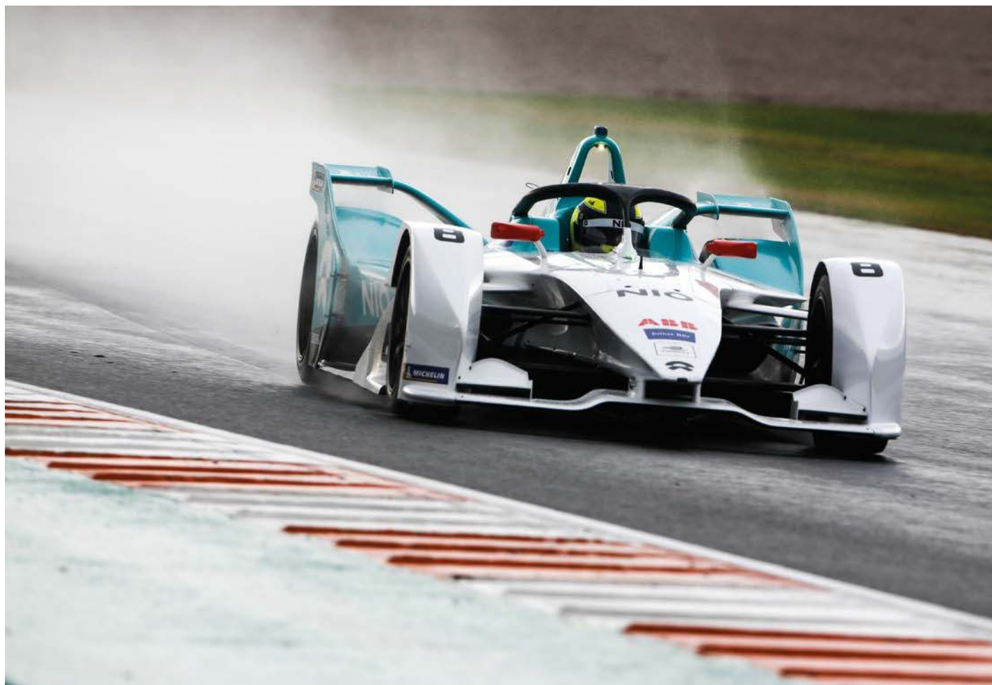
The Formula E car consumes so little energy driving around at 50km/h behind the safety car that the subsequent laps of the new time-based races can be completed at a faster pace
