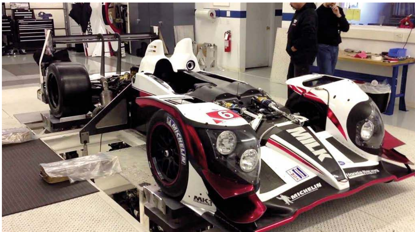
The closest a simulation gets to real life track action is probably when the actual racecar is strapped to a shaker rig. The car's wheels are worked through the pads
