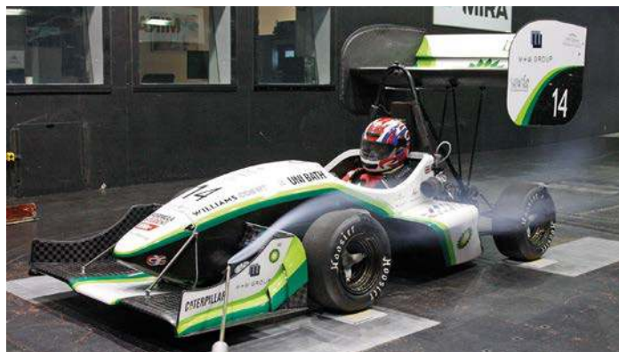
Team Bath Racing's Formula Student car, as tested in 2014, sported triple-element wings
