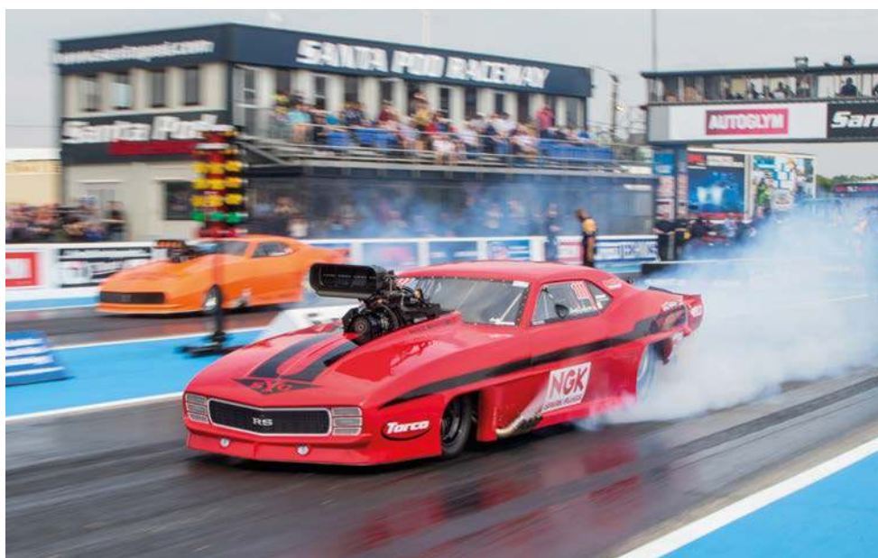
Pro Mods are said to be the world’s fastest saloons. Their rear axles are skewed to compensate for the huge chassis torques
