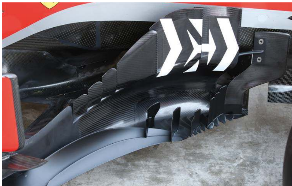
The bargeboard height will be reduced in 2019; giving the teams less scope in what is a fruitful area for aero development
