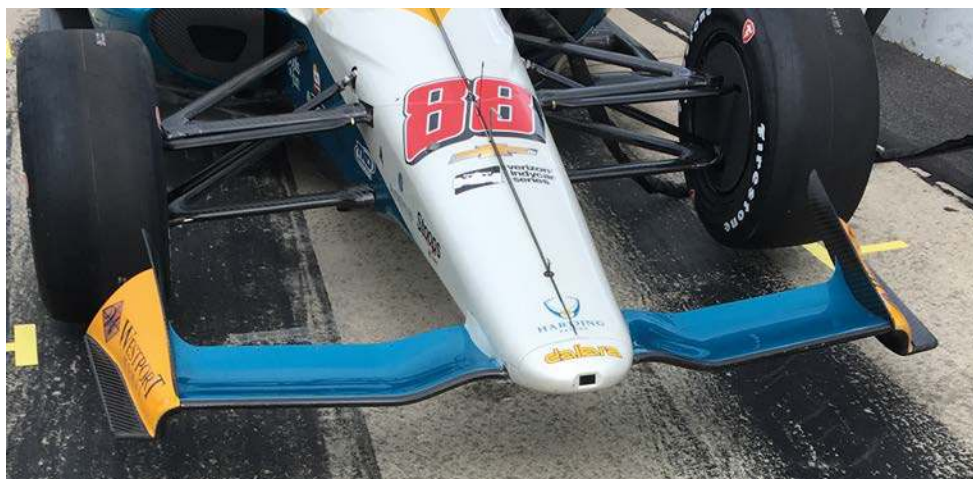
The biggest discrepancy between the two aero kits was the loss in performance experienced by the UAK18's front wing
