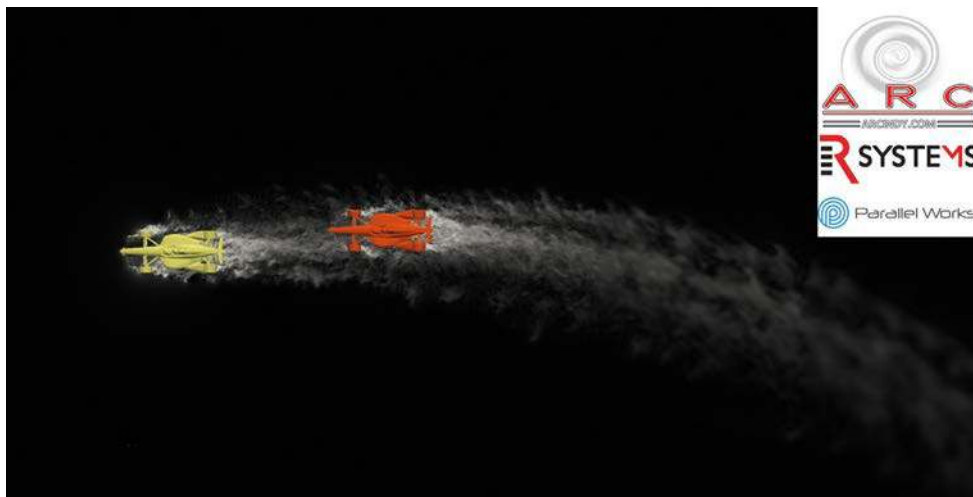
Figure 10: Velocity contours for two UAK18 kits. The predictive map for following-car aero will be used in DIL simulators
