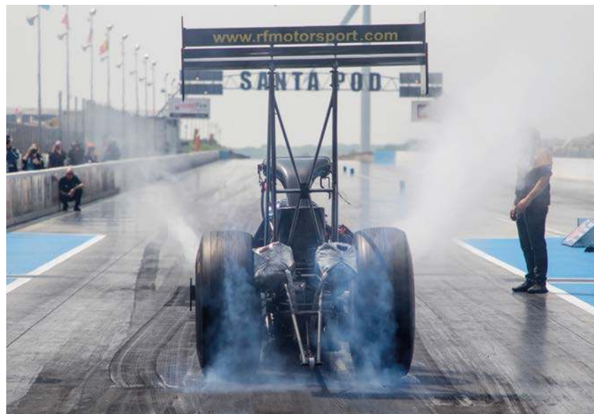
Dragsters 'burnout' on the start-line to warm the tyres and put down a layer of rubber for extra grip at the start
