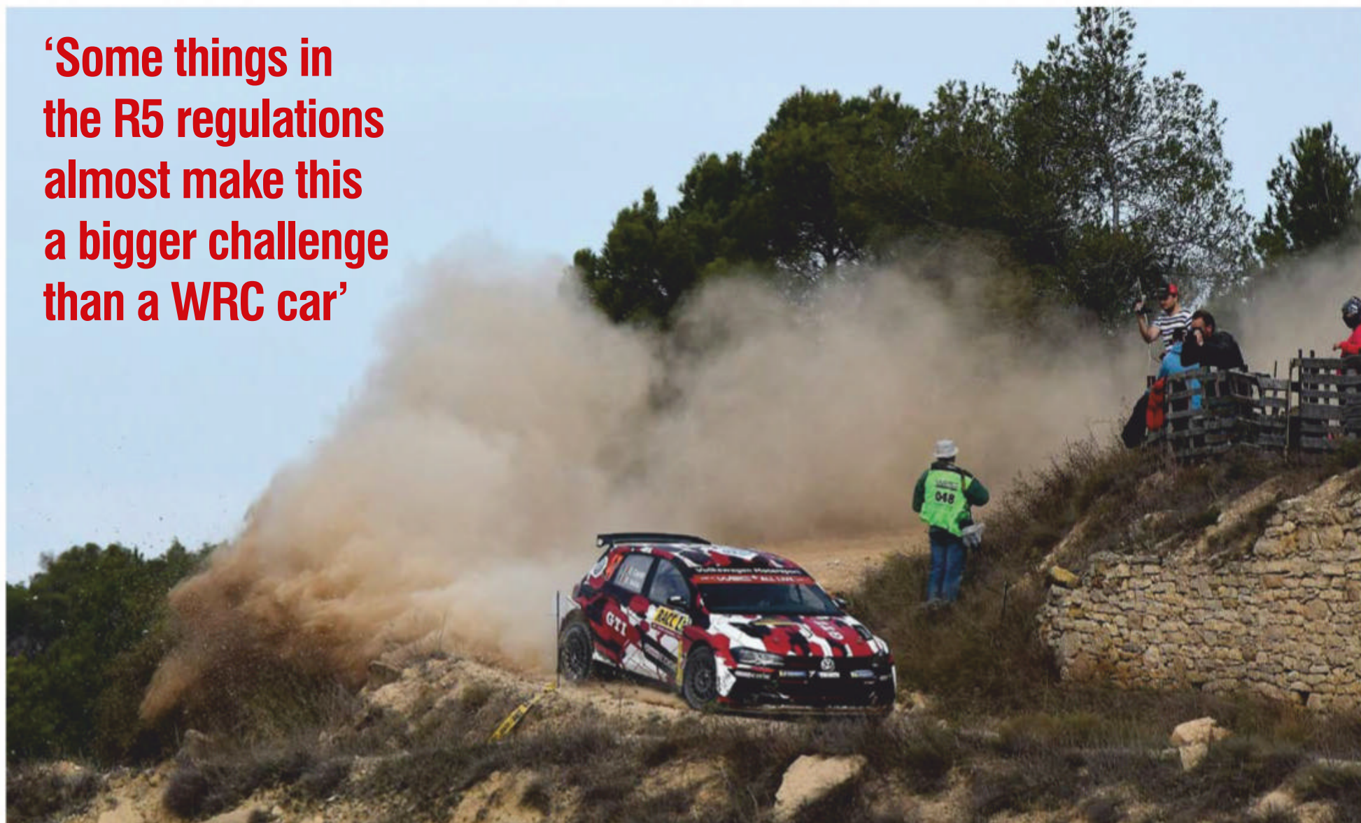
The Polo packs a 1.6-litre turbocharged straight-four powerplant that produces 272bhp. That power is transmitted through all four wheels via an Xtrac sequential 5-speed gearbox
