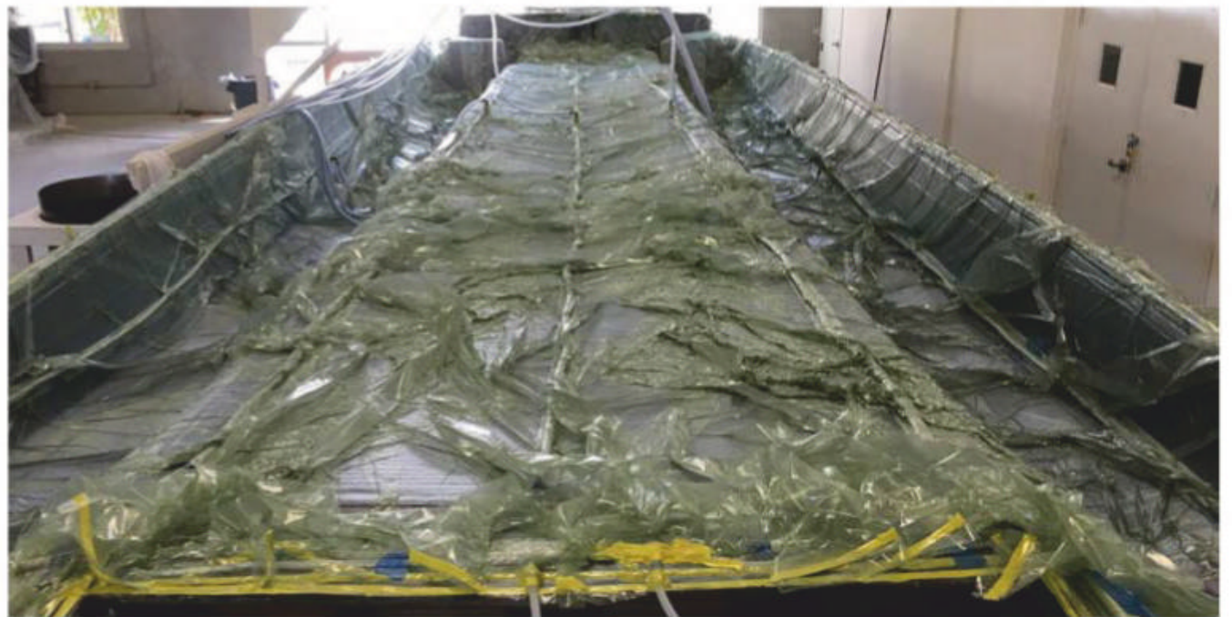
Extremely large structures can be made using resin infusion, such as boat hulls and turbine blades but until now the process is almost unheard of in motorsport although the company is working to change that through its Revolution racecar
