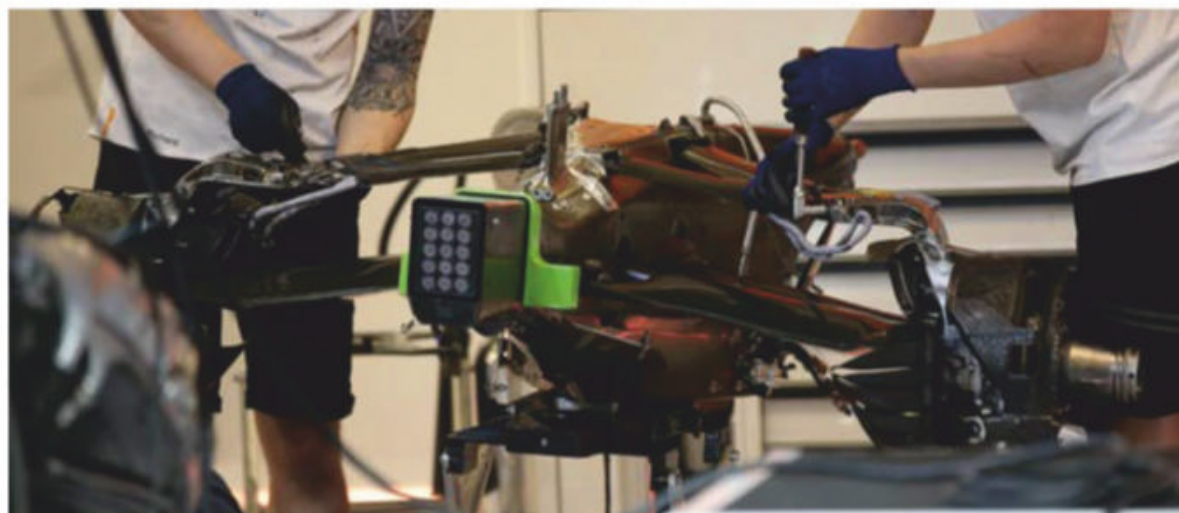
Composite gearbox and rear suspension. Note the short upper wishbone that picks up the extended upright
