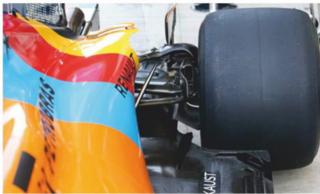
The upper wishbones at the rear of the car were covered in a composite shroud which gave them the appearance of a single piece component
