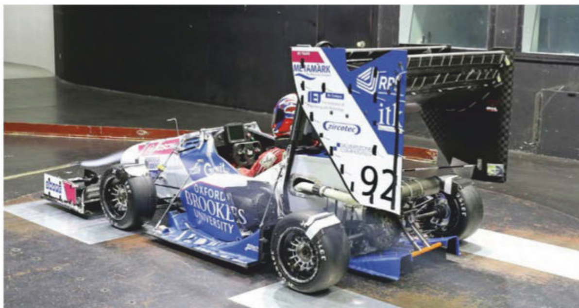
The Oxford Brookes OBR18 Formula Student car sports a complex aero package which was developed in CFD
