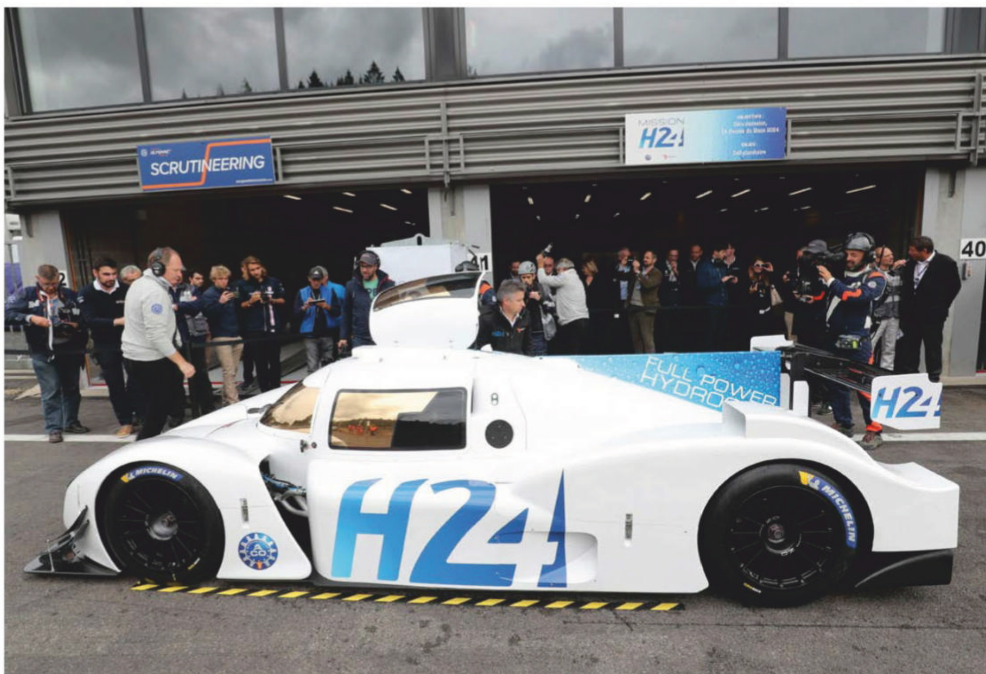
GreenGT's LMPH2G has been built to demonstrate the possibilities of hydrogen fuel cells in racecars. It can reach 100km/h in 3.4 seconds and has a max speed of over 300km/h
