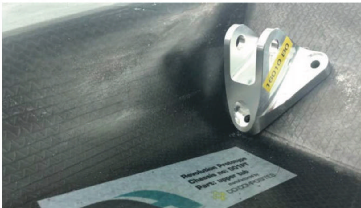
All the mounting points on the tub are made from high-grade aluminium to offer the strength needed
