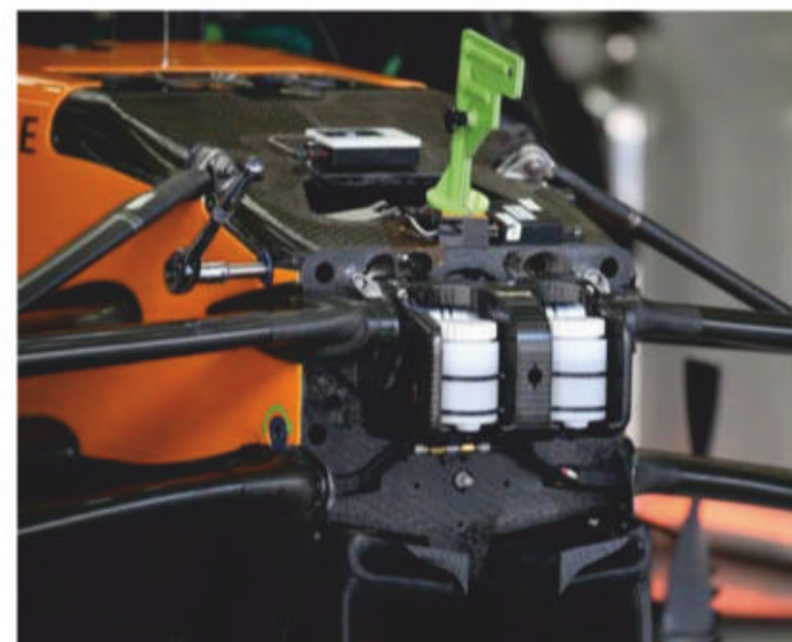
Pushrod actuated torsion bars and dampers were used at the front
