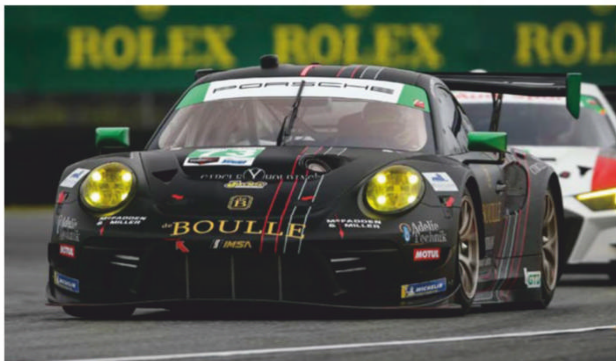
The front splitter is raised to reduce pitch sensitivity under braking, and maintain airflow to the rear diffuser
