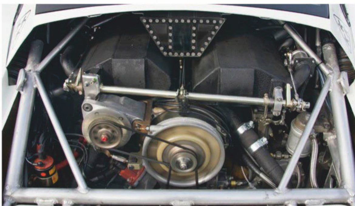
The twin turbo engine with its new twin-cam, 24-valve, cylinder head produced in the region of 750 to 800bhp
