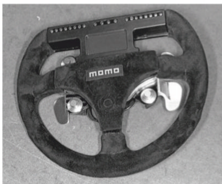
The wheel includes paddles for hydraulic corner weight jacks
