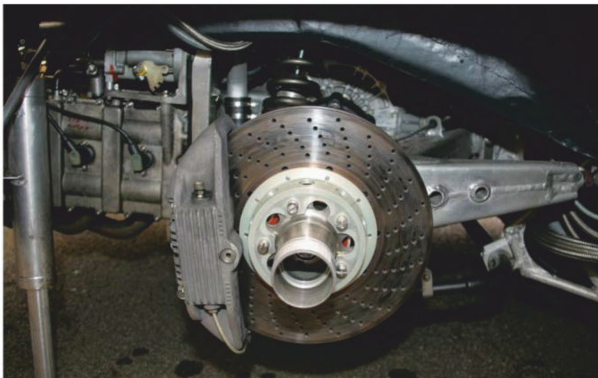
The 935/78's discs were an improvement over the standard 935 spec, with greater diameter and thickness
