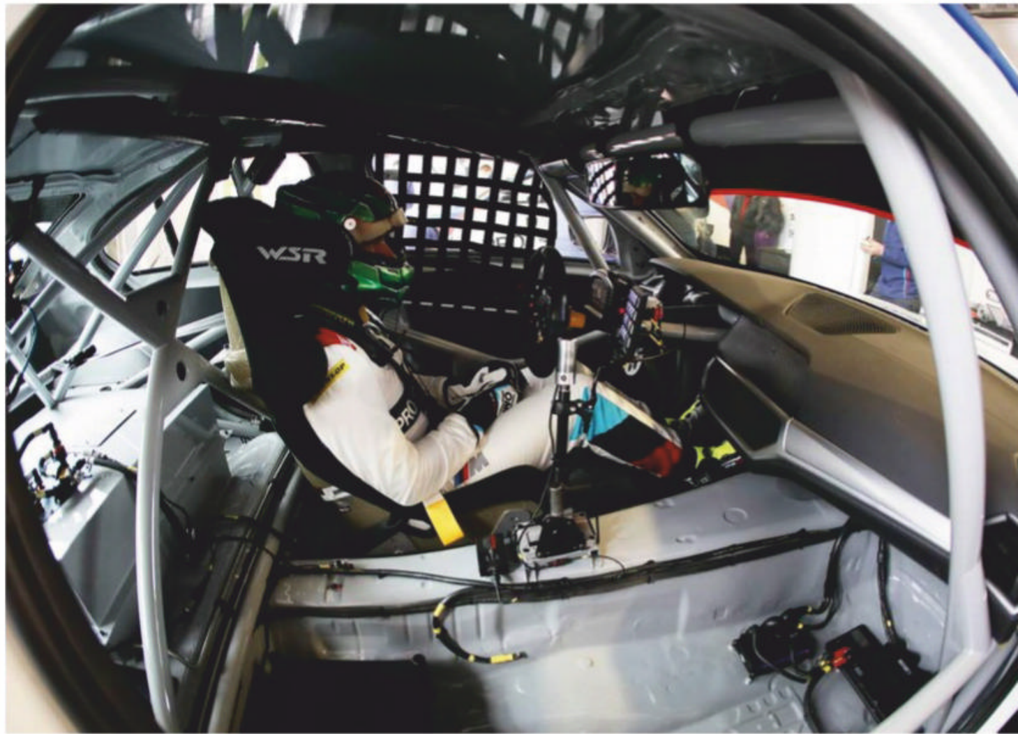
WSR has made the most of the larger cabin and has moved the driver towards the rear to improve the car's weight distribution
