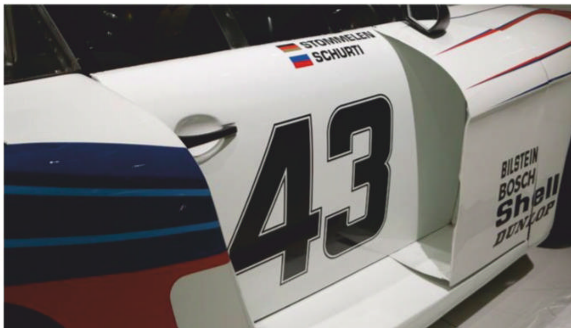
The 911 doors were originally hidden behind cowlings but the rule makers told Porsche to get rid of these
