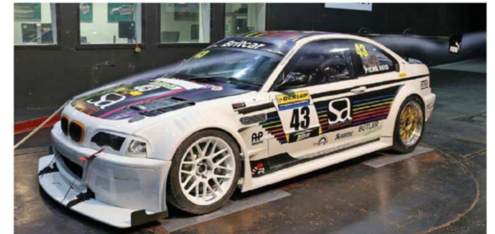
The Britcar BMW M3 E46 undergoing tests in the MIRA wind tunnel. It came to the session with a wet set-up
