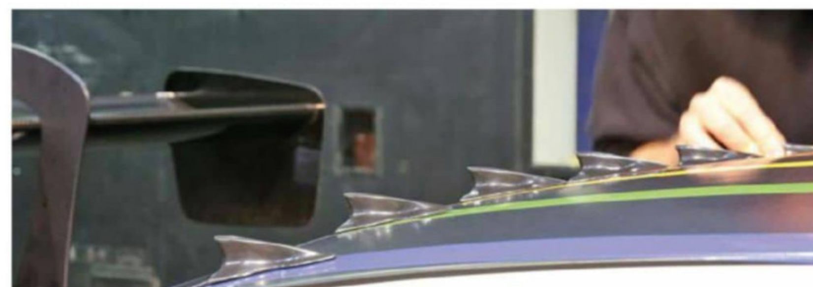
Would the Mitsubishi Evo style vortex generators on the roof of the BMW really have a noticeable aero effect?
