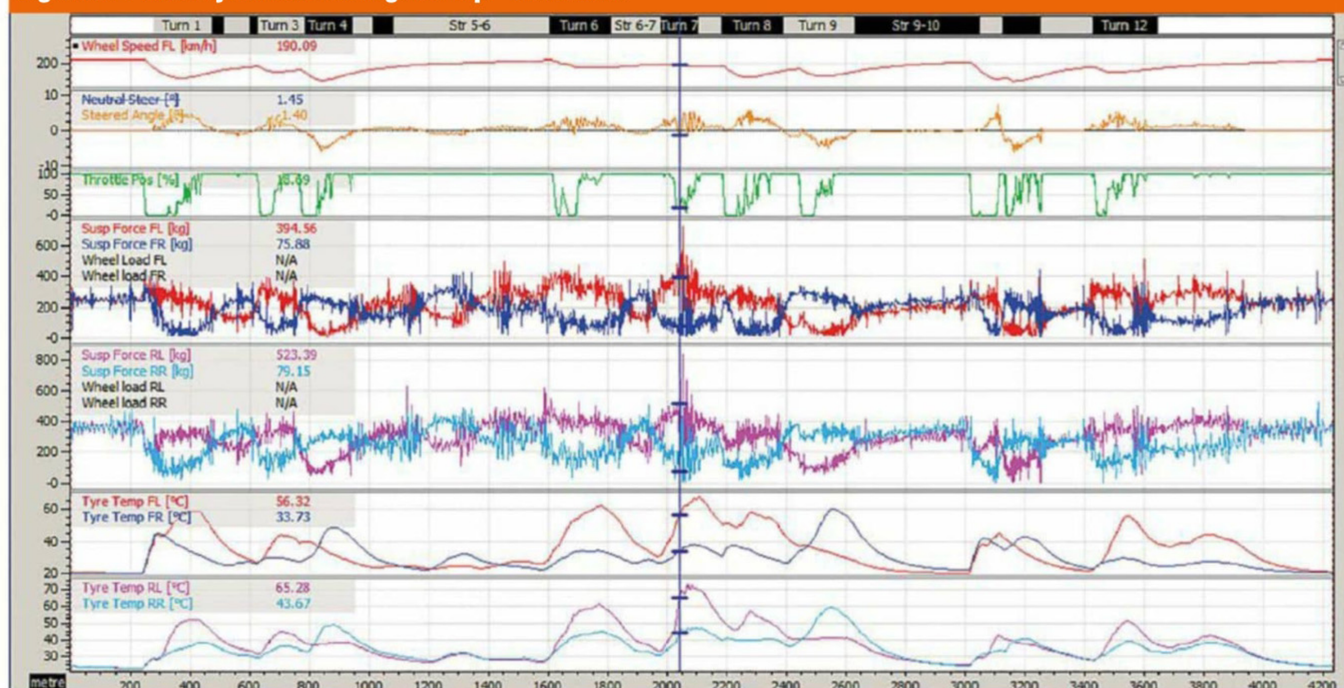
Figure 5: Plot of tyre loads for a given lap – simulated
