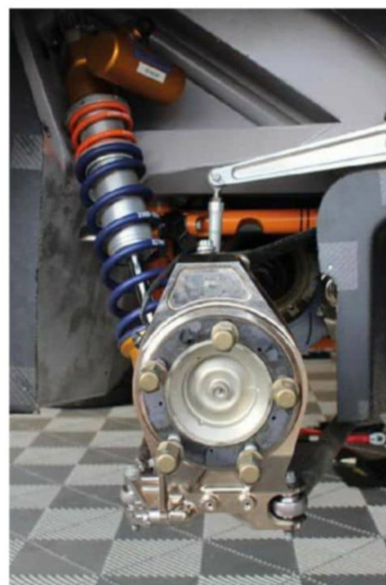
The front (left) and rear (right) wheel hubs and inboard brake design of the GCK Renault Megane RS RX
