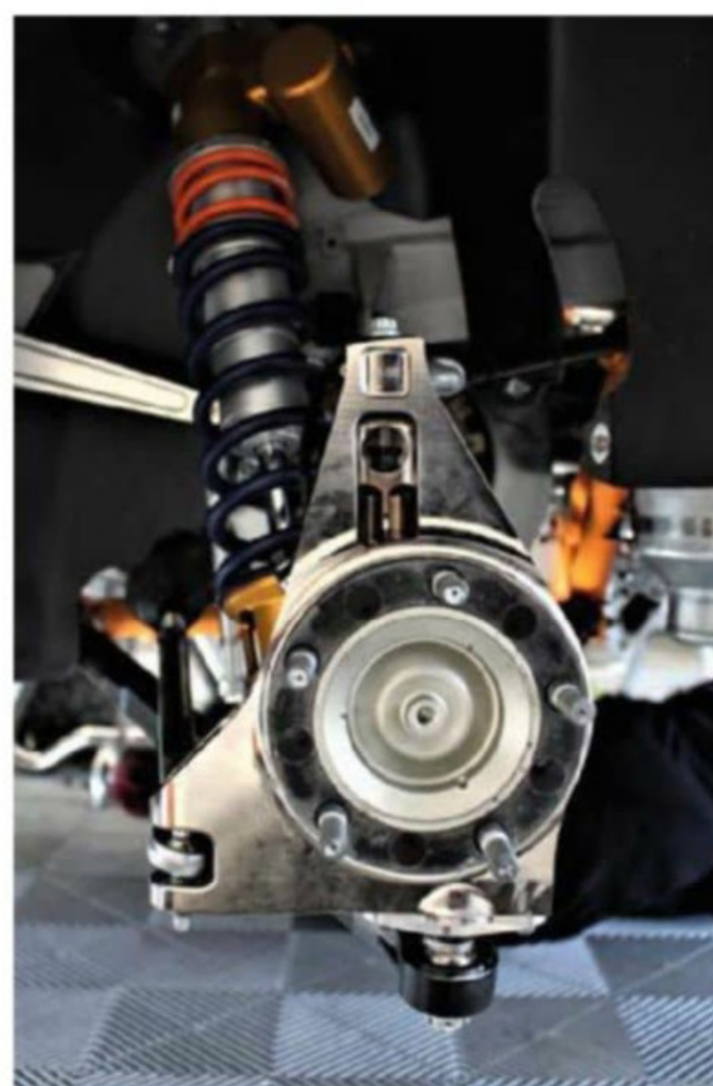
The front (left) and rear (right) wheel hubs and inboard brake design of the GCK Renault Megane RS RX
