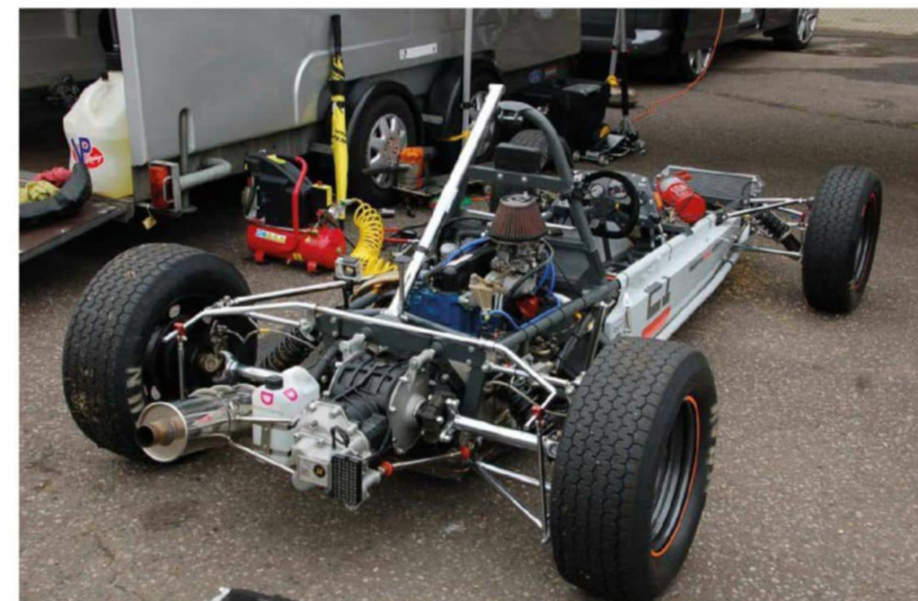
Old style anti-roll bar on a Formula Ford 1600 – it's adjusted by sliding the vertical rods on either side along the bar
