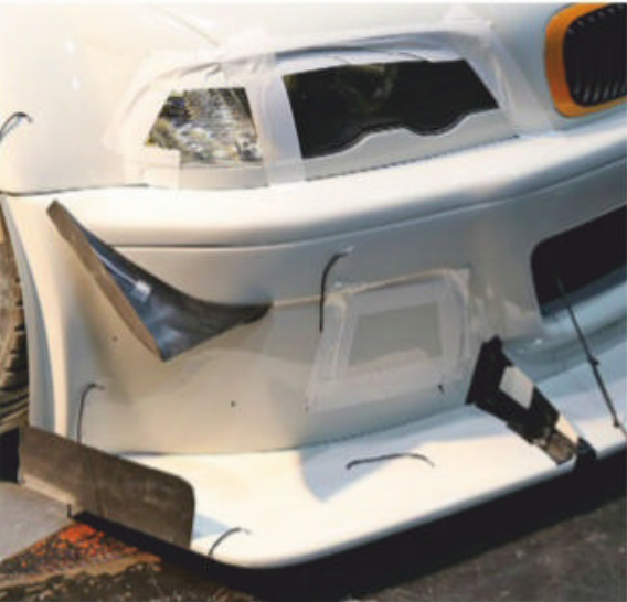
Here the lower dive plane had been taken off the car
