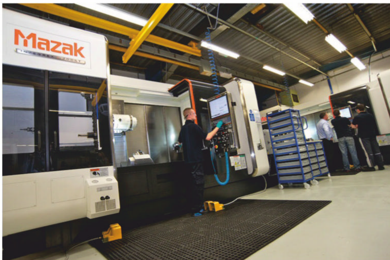
CNC gear-cutting equipment at Ricardo. Modern machinery allows the manufacture of extremely complex cog geometries
