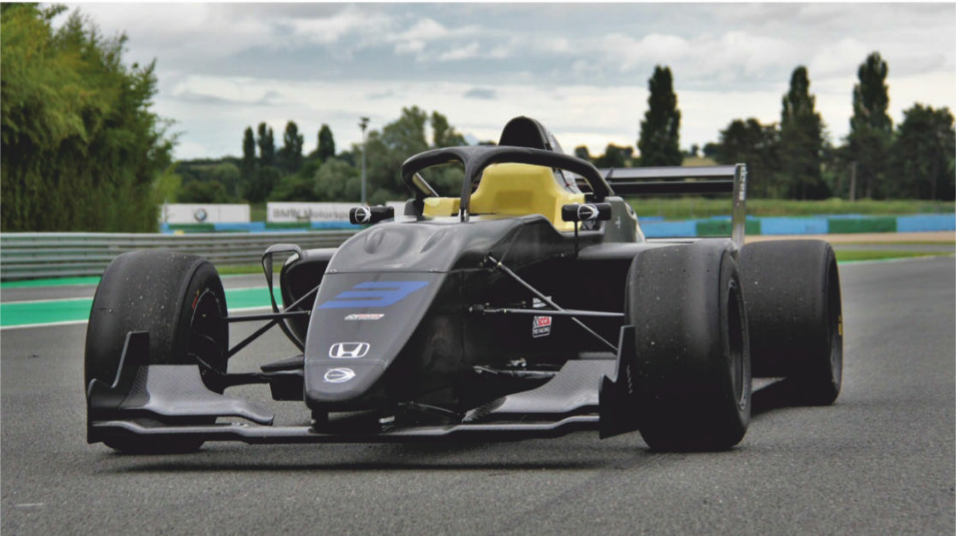
The Ligier JS F3R. Halos are mandatory while the design of the nose is tightly controlled for safety reasons. This means that all F3R racecars will look very similar from the front
