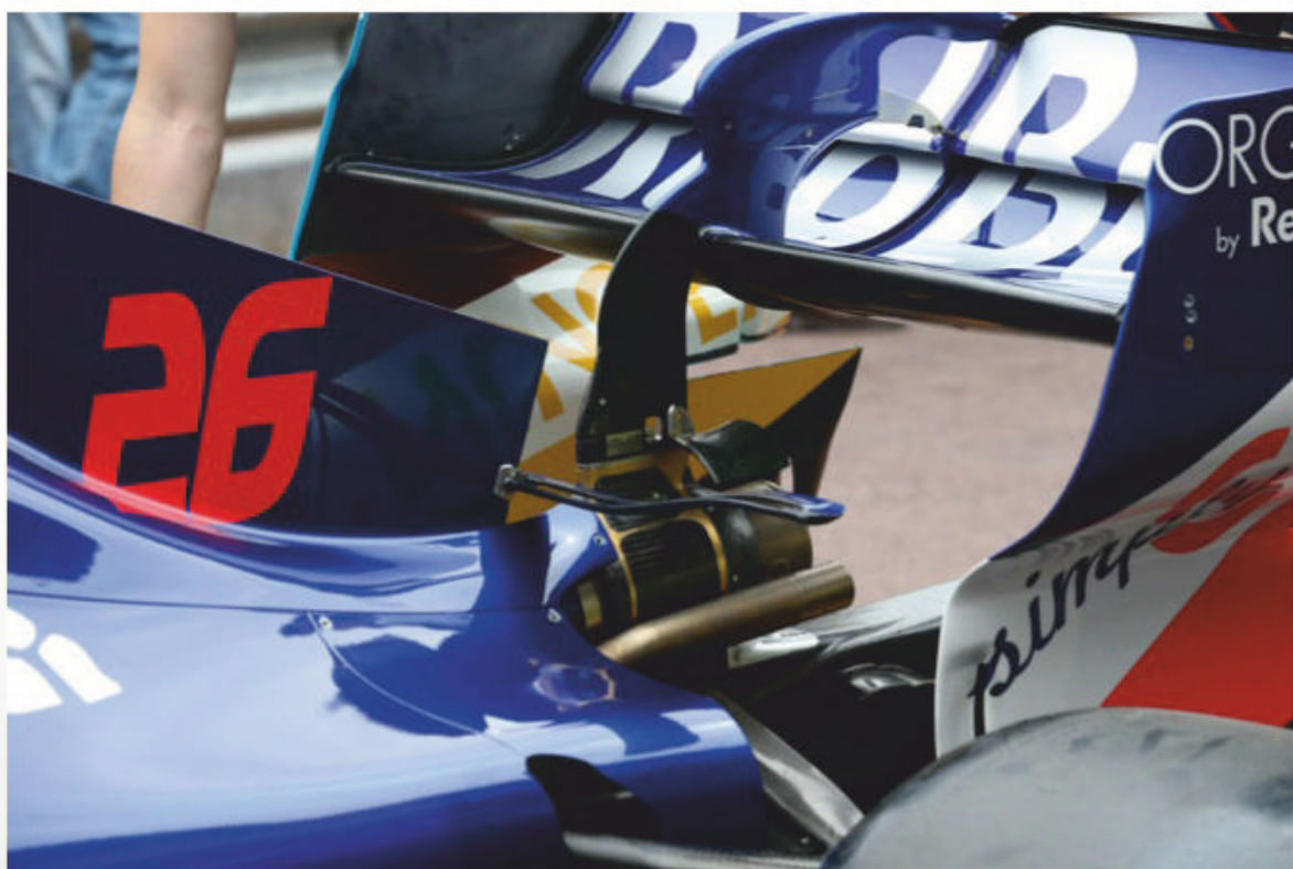
The rear wing on the STR14. Toro Rosso has changed its aerodynamic development methodology this year
