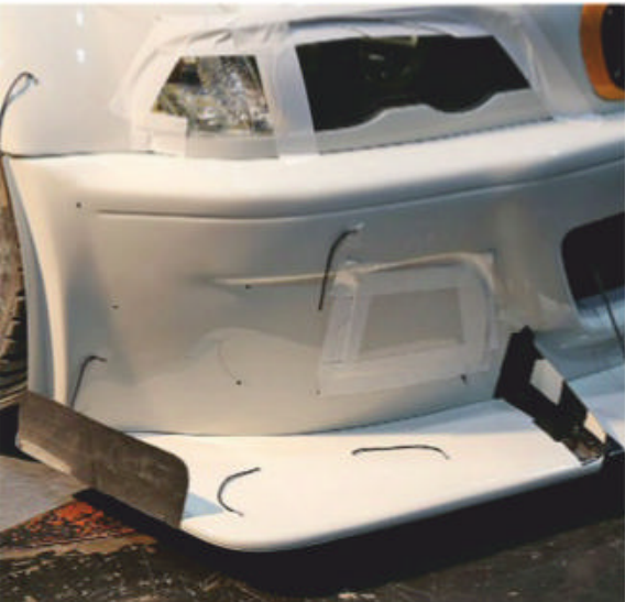
No dive planes; as featured in the lower drag set-up
