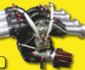
Greenwood "Spirit of 76" LeMans Corvette. Ran Kinsler crossram manifold with Lucas mechanical metering.
