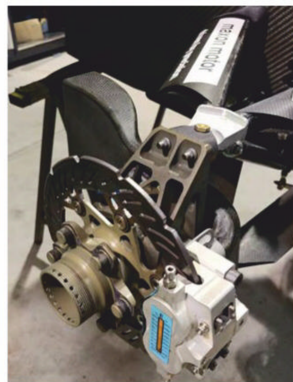
The M-19L's very neat brake and upright assembly
