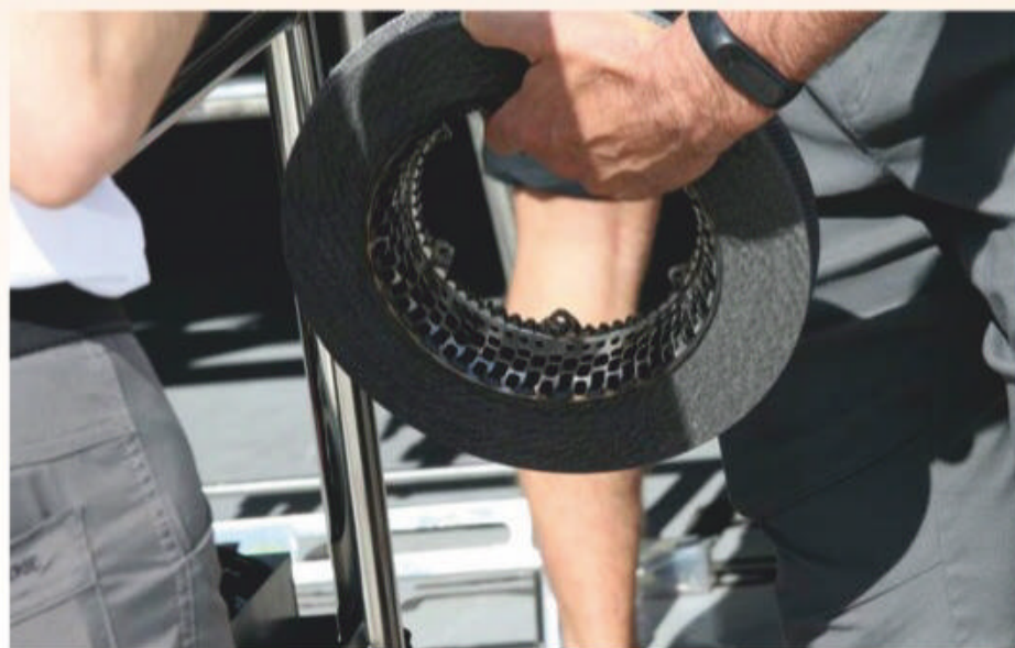
A rare shot of a Brembo F1 disc, as used by Haas, showing internal cooling channels
