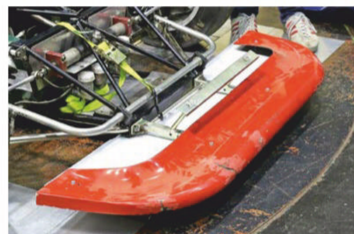
A flat underside (white) in the splitter brought surprising results
