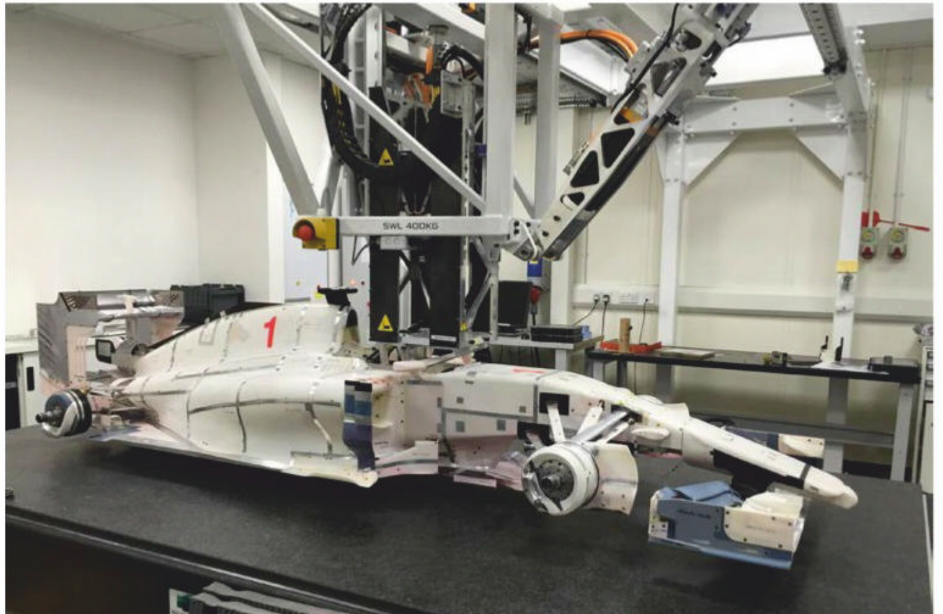
Strut with actuator and model. These days models are intricately detailed pieces, nothing like the clay items of yesteryear
