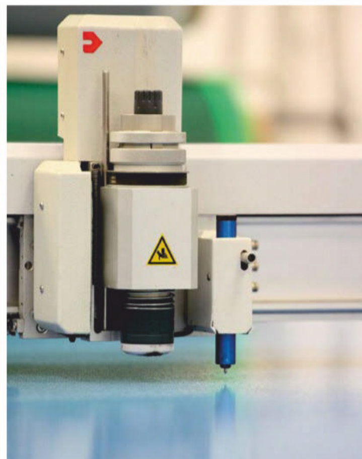
This kit cutting machine, which is used in conjunction with a digital manual, provides the laminators with everything they need in order to accurately lay-up a composite component in a repeatable way
