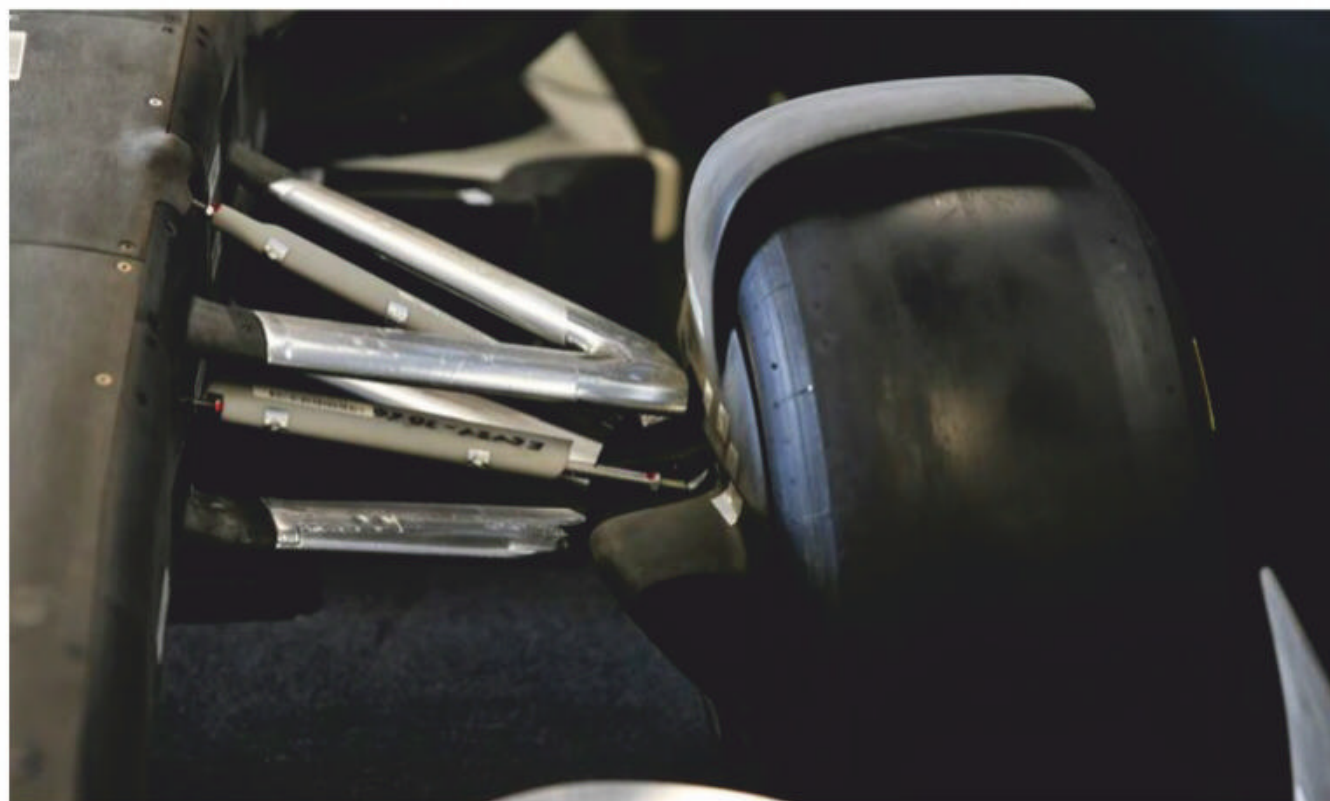
These quirky winglets will sit above the front wheels to help reduce the wheel wakes, while also guiding the airflow inboard
