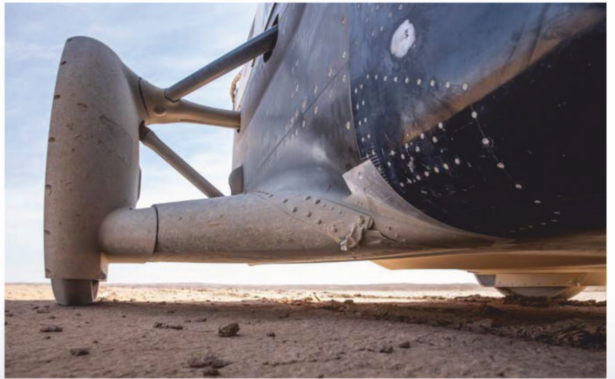
These solid aluminium wheels have been specially designed for the desert surface and can spin at 10,200rpm
