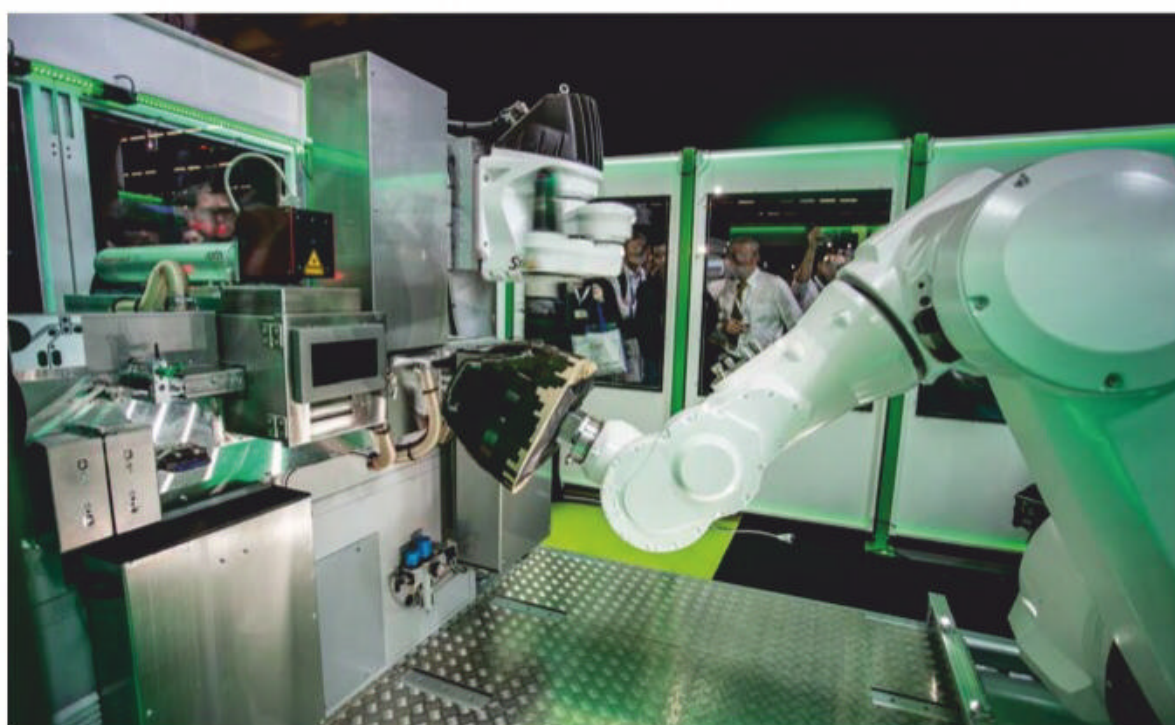
The mould is controlled by a robot and it is able to rotate and move freely as the tape is being applied to it
