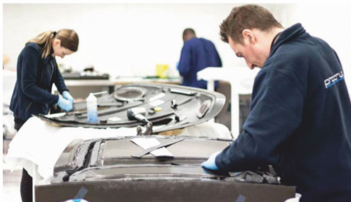
While there’s ever more automation in motorsport composites much of the skilled work is still done by hand
