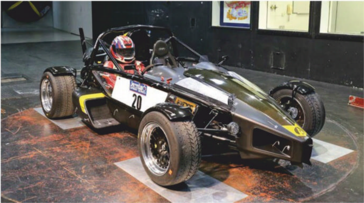
With the wings removed from the car the vertical forces were very different, although drag did not change much
