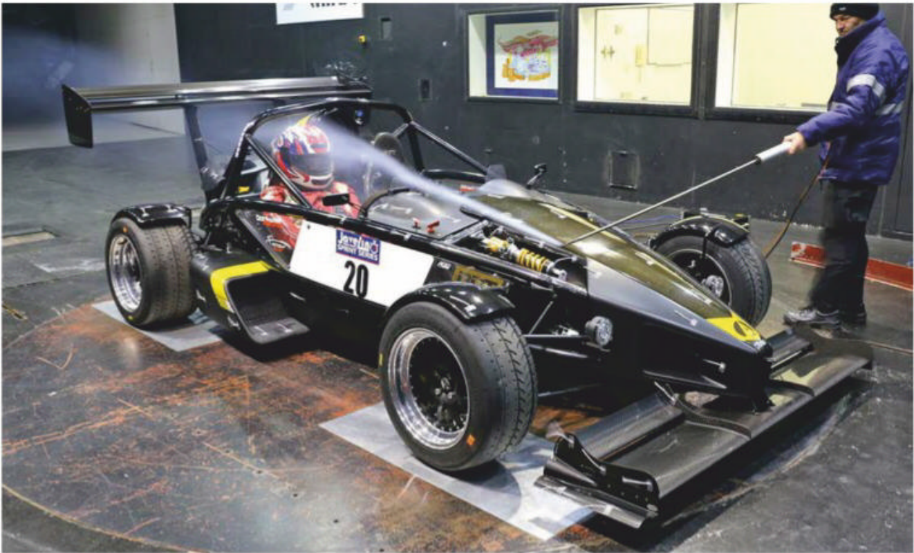
This Ariel Atom sprint car sports wide span, dual element wings front and back to help generate some useful downforce
