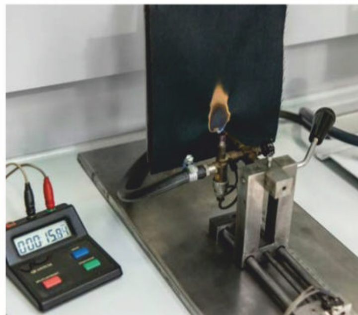
The material must withstand a direct flame for at least 12 seconds
