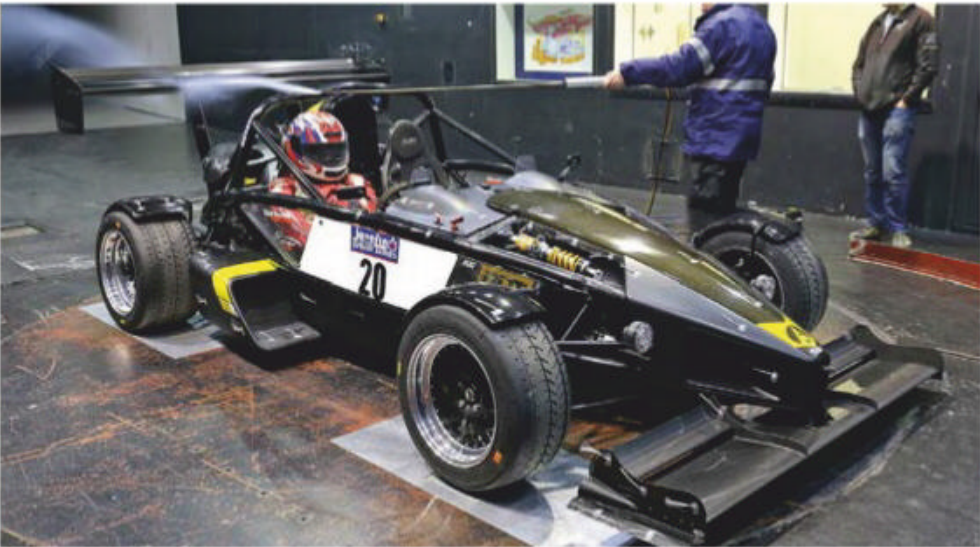
With a large frontal area plus those wings it was no surprise that drag was relatively high
