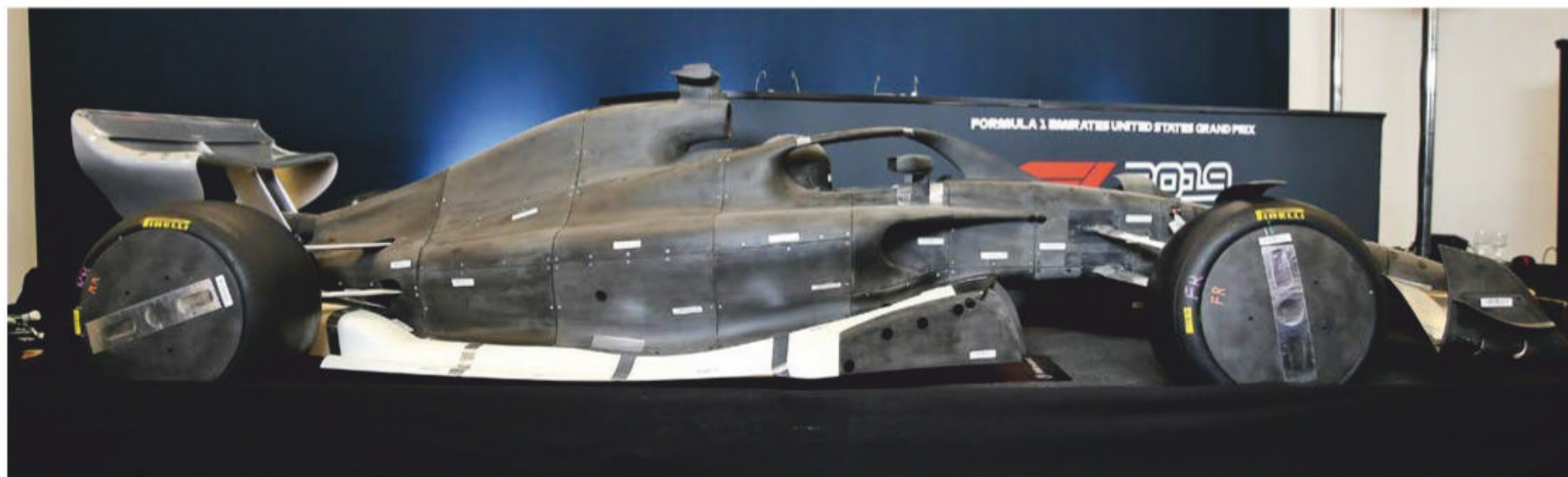
The 2021 cars will feature 18in wheels. Covers will also be used so teams will no longer be able to blow air through the rims for tyre heating, or to force the wheel wakes outboard
