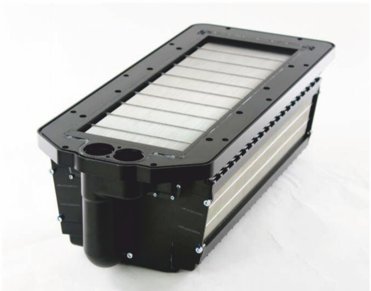
Micro tube intercooler. This example was used in drag racing and provided a good performance improvement
