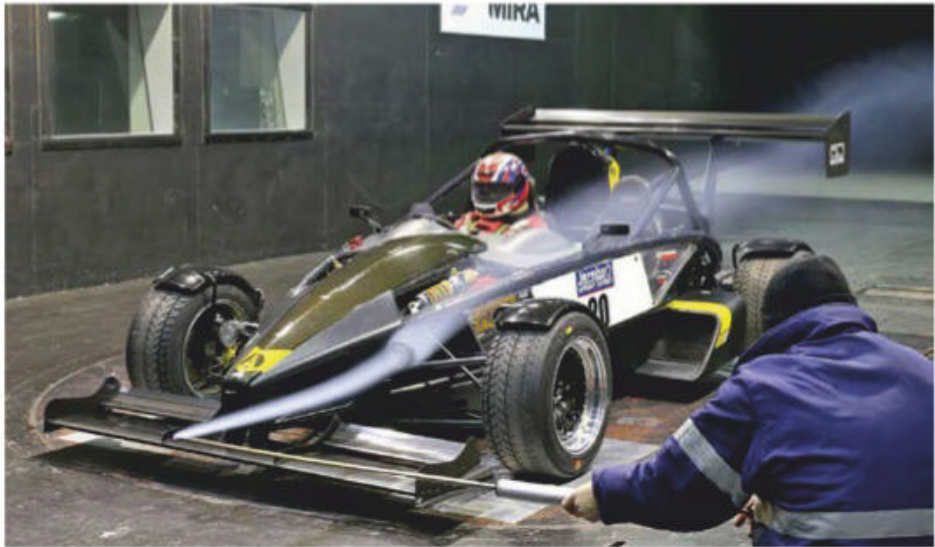
Headlamps are drag contributors while their wake also impinged on the rear wing flow
