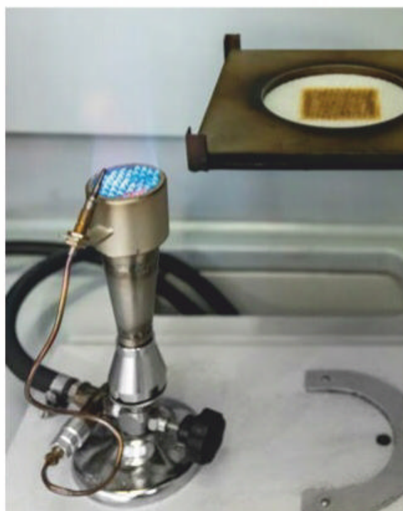
The underwear material is stretched in a frame ...
