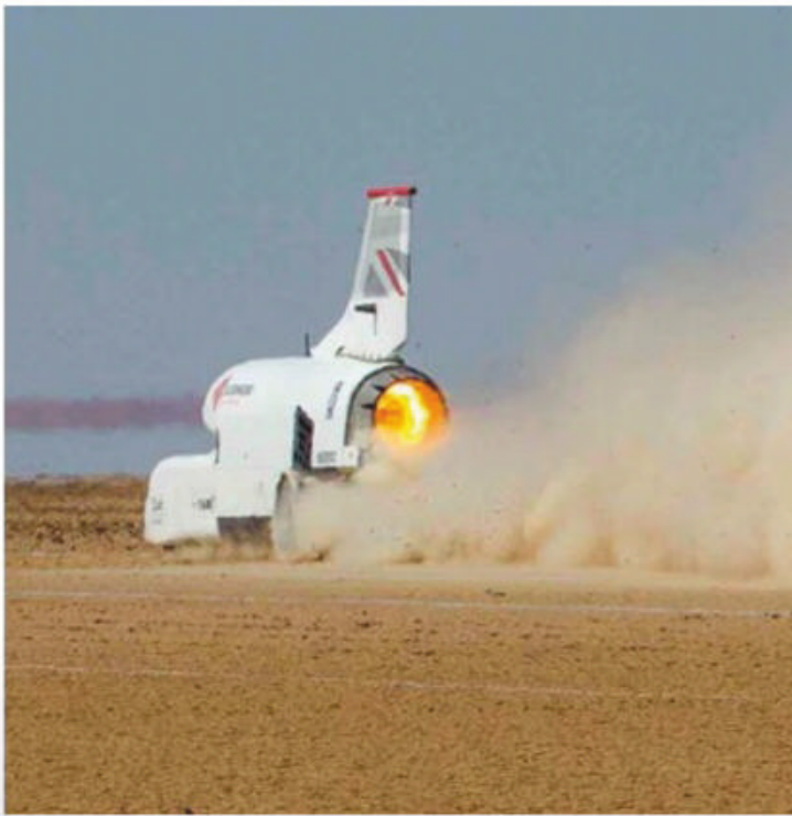
The jet engine is the same as the one used in a Typhoon fighter
