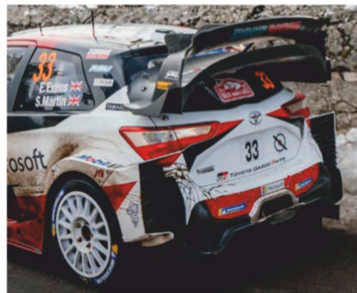
Higher rear brake cooling inlets are now a feature of the Yaris WRC
