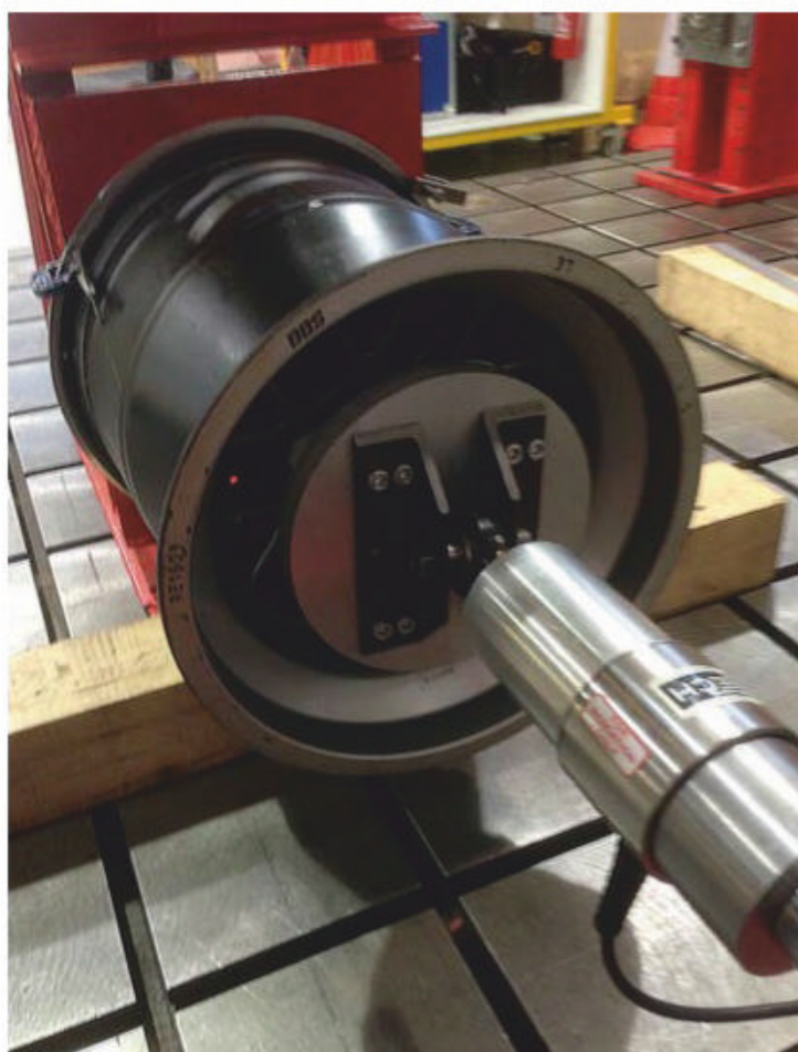
New for 2015 was a wheel retention test; shown here at Cranfield
