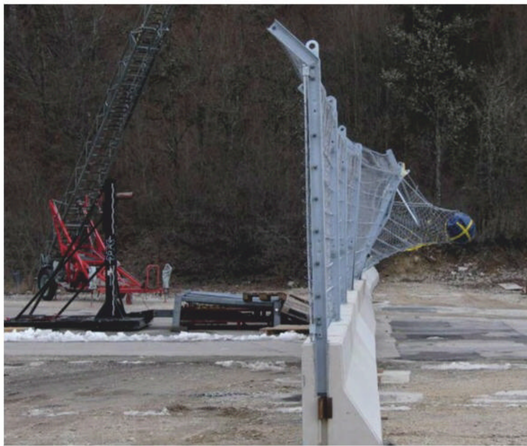
The sphere test involved a 780kg steel ball hitting a fence at 65km/h at a height of 2.2m. This was to simulate a Formula 1 car getting airborne and then crashing into the structure
