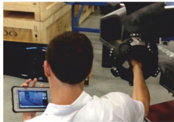
3D scanning with the first generation Creaform Metrascan 210
