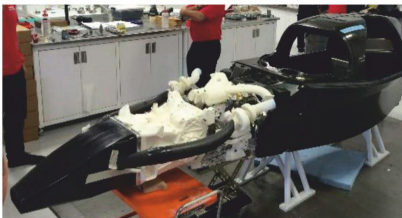
Parts were mocked up using 3D printing so work could continue even though long lead time items were still being made
