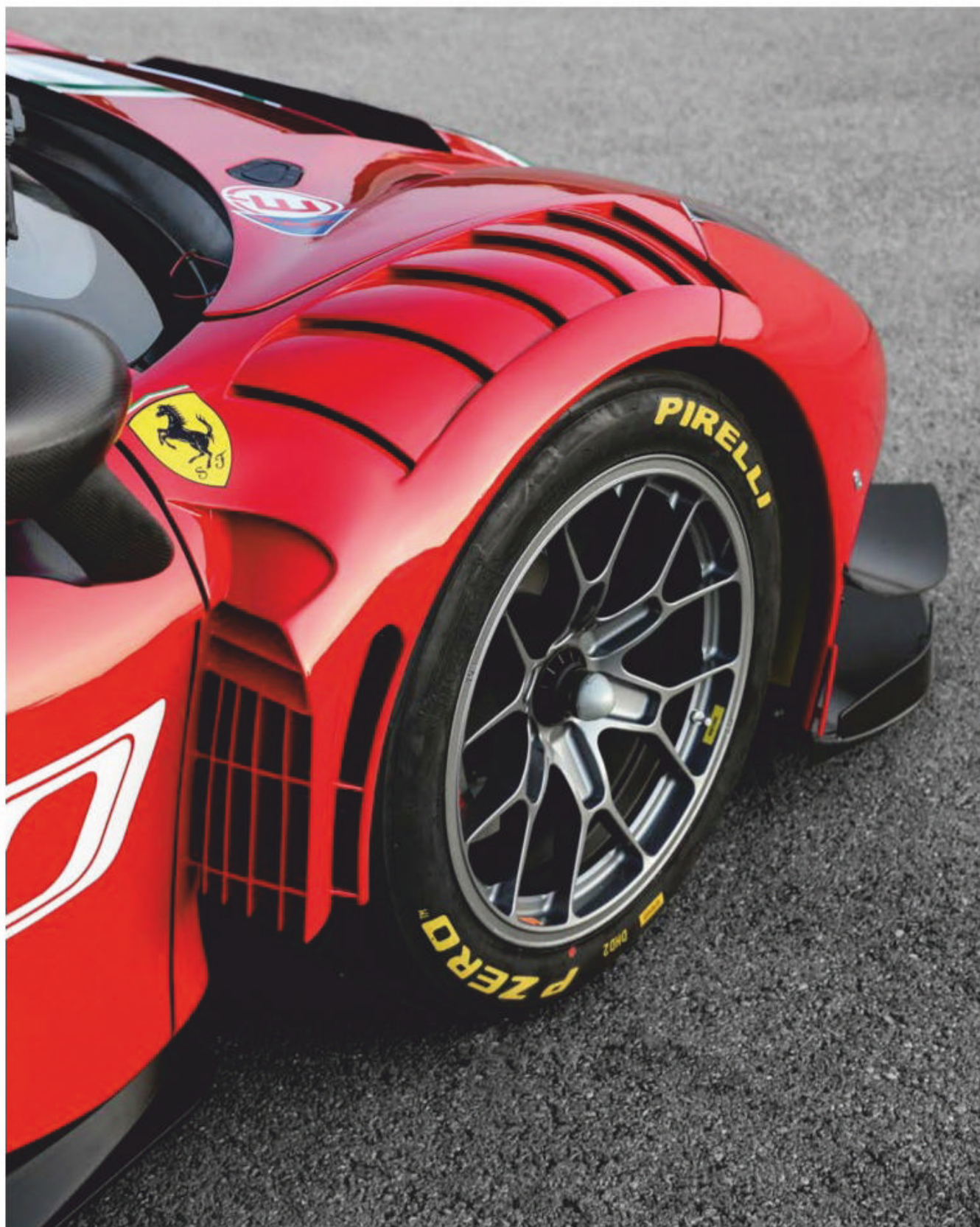
Some of the more obvious aerodynamic development on the 488 Evo can be seen in the area behind the front wheel arch
