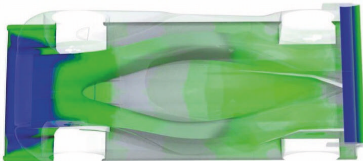
Figure 9: The overall aerodynamic approach, showing the pressure values on the front diffuser and the through tunnels
