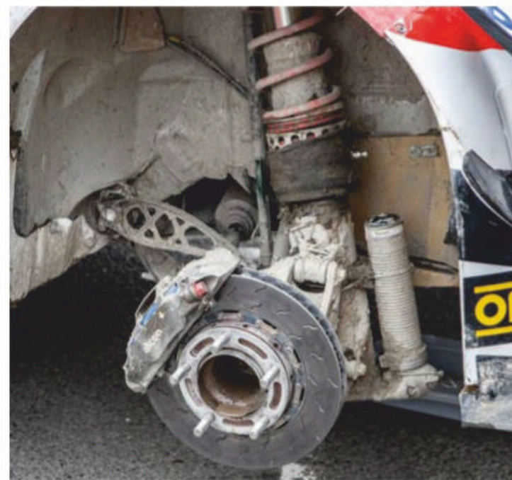
Toyota introduced a revised upright and hub assembly for 2020
