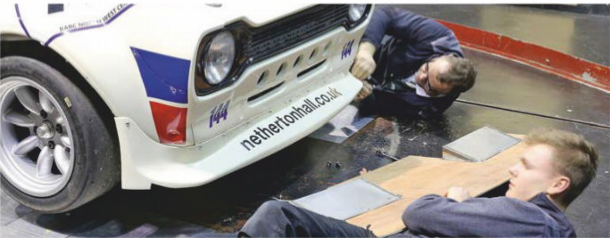
Installing a test splitter fitted with front diffusers; just one of the options employed to find some front downfoce
