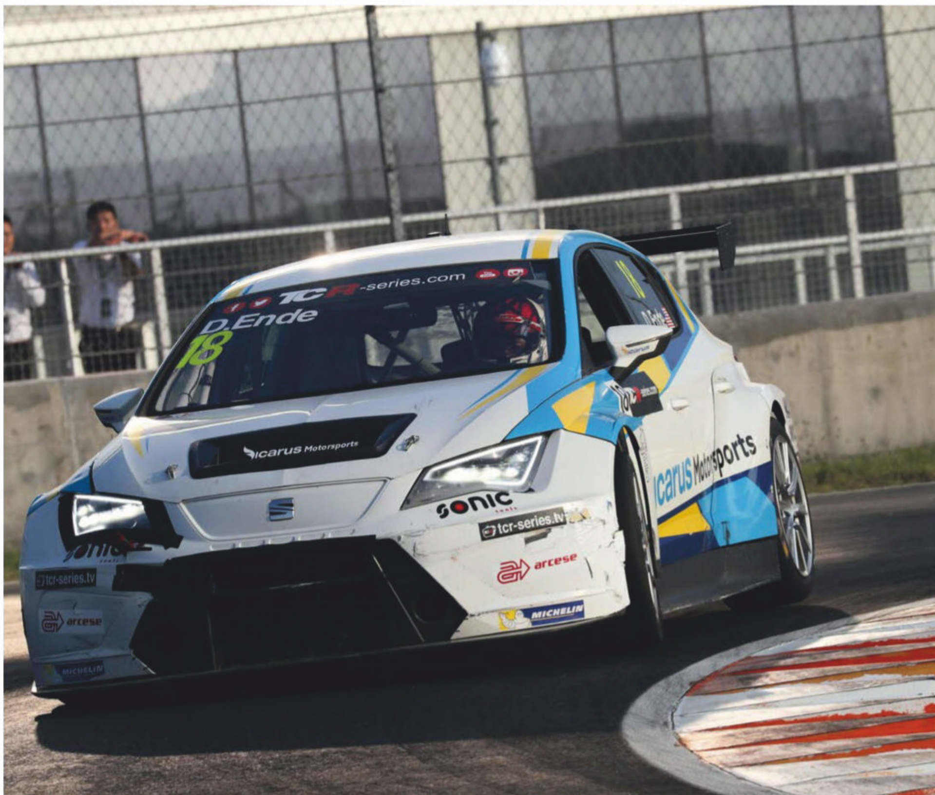
A TCR racer loads up its front right tyre in a corner. The relationship between vertical load and mechanical grip is a key factor when it comes to damper spec and spring rates
