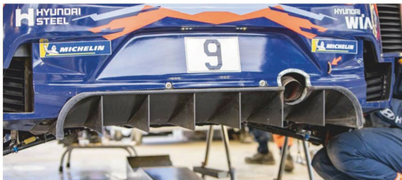
Hyundai's new rear diffuser. One with a centrally-mounted exhaust was tested pre-season, but this was not used on the rally
