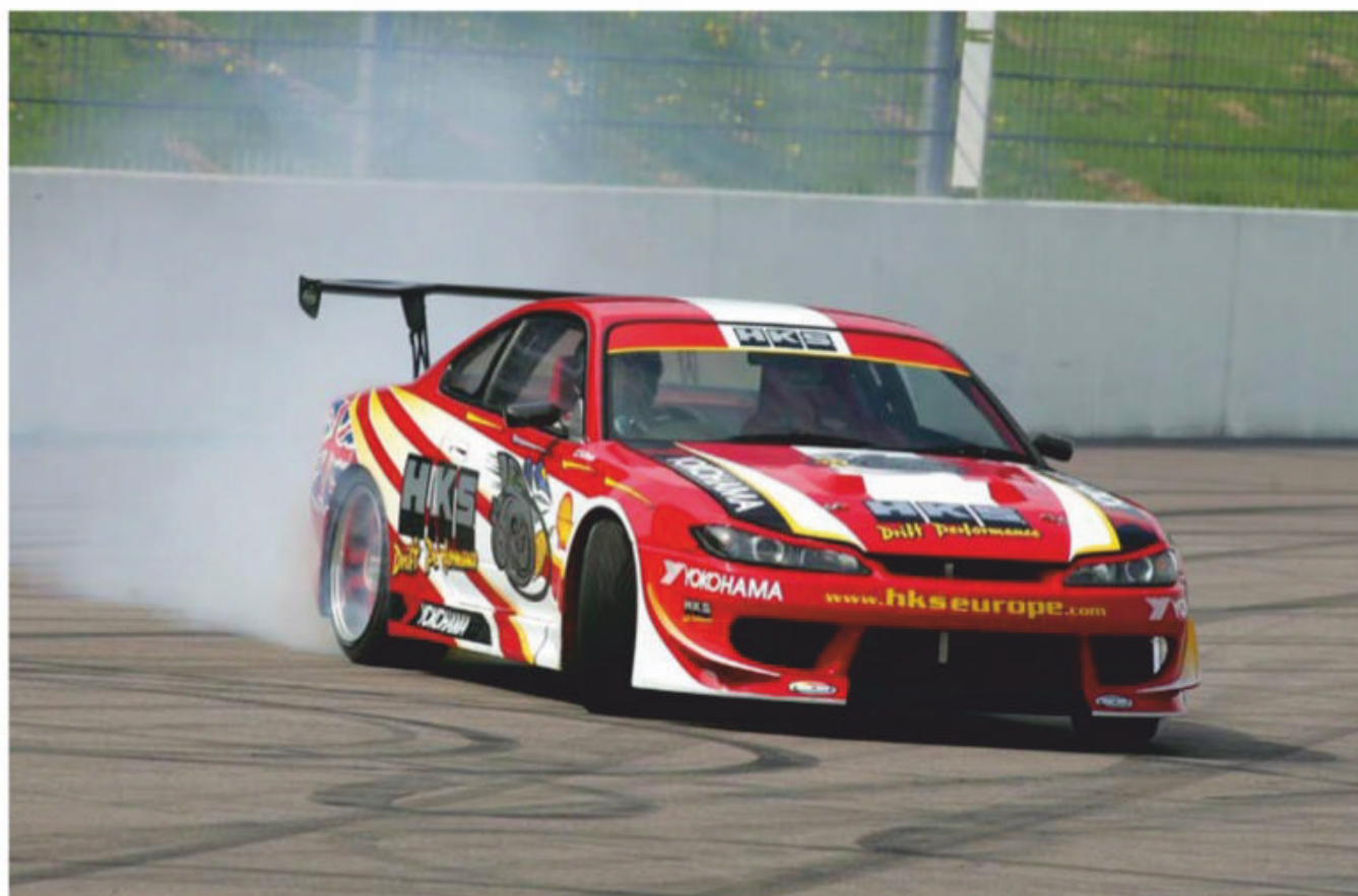
One category that makes use of locked diffs is drifting, where once the rear has broken away understeer is rarely an issue
