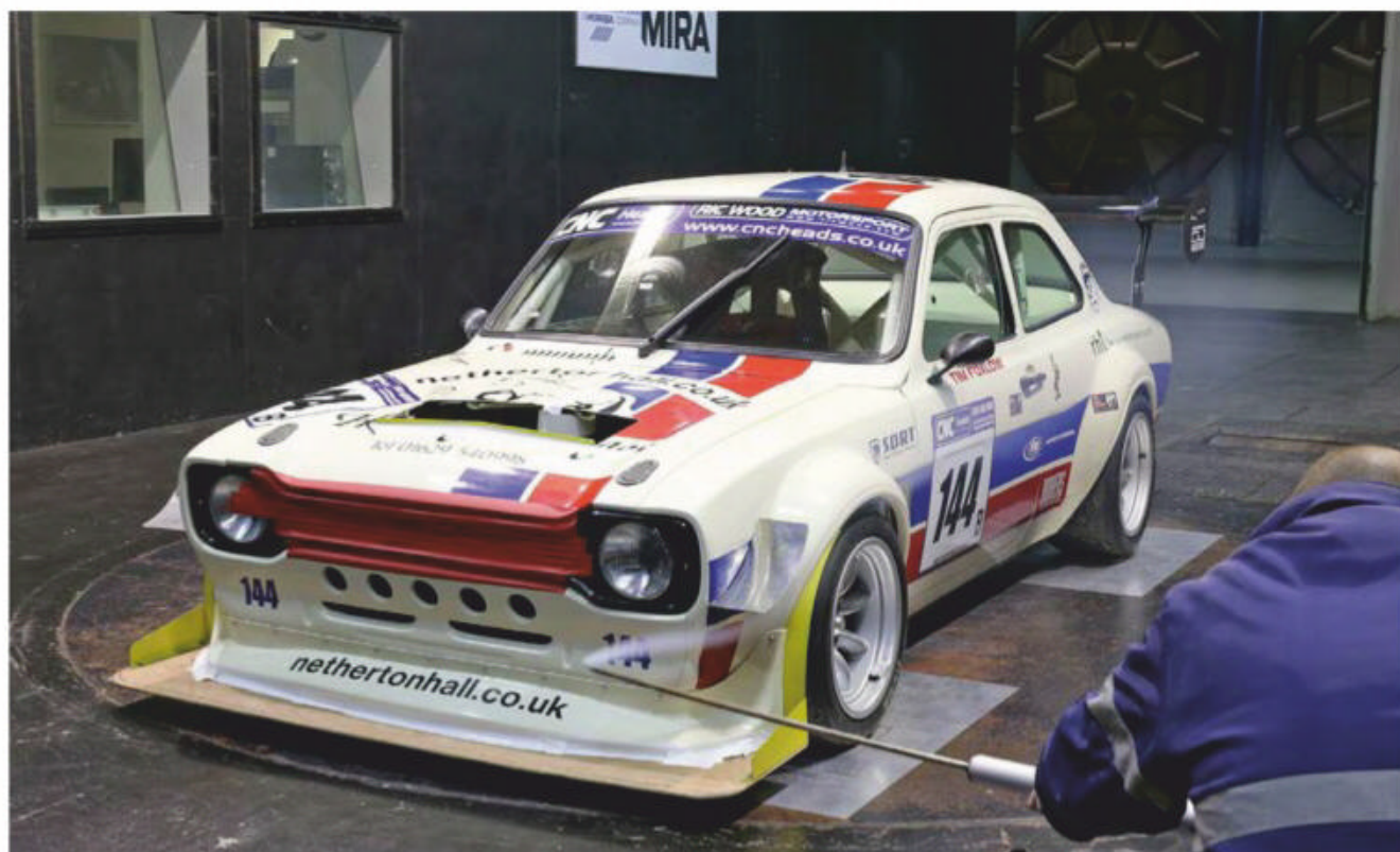
Above: The Escort RSR requires a strong front end if it is to achieve the target aero balance
