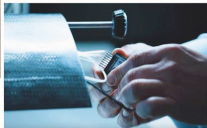
With numerous inconsistencies due to the length of tubes connecting pressure sensors, limiting the length offers a benefit
