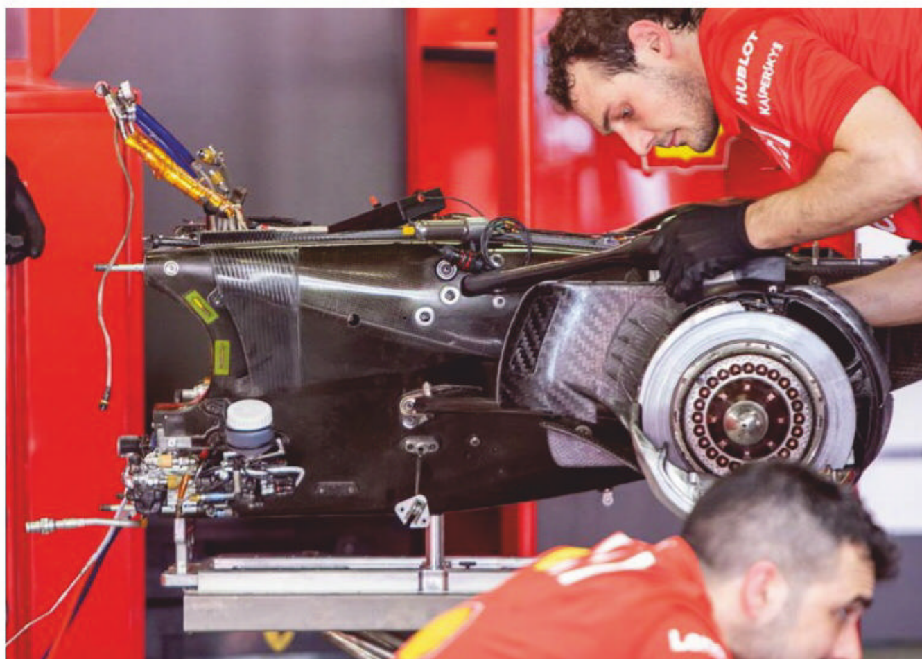
Left to their own devices, teams will use different materials for their transmissions, Ferrari choosing a composite casing
