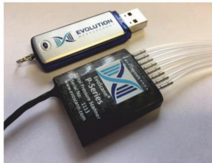
The minute size of EvoScann® scanners allows their placement in critical areas of racecars where larger scanners cannot fit
