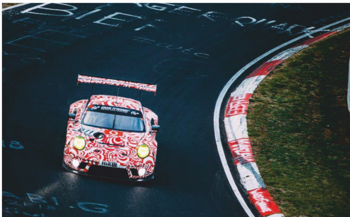
Track surface plays a part in the optimal set up, especially with high-downforce cars. A lumpy track like the Nürburgring requires a very different approach to spring-damper systems compared to a smooth circuit
