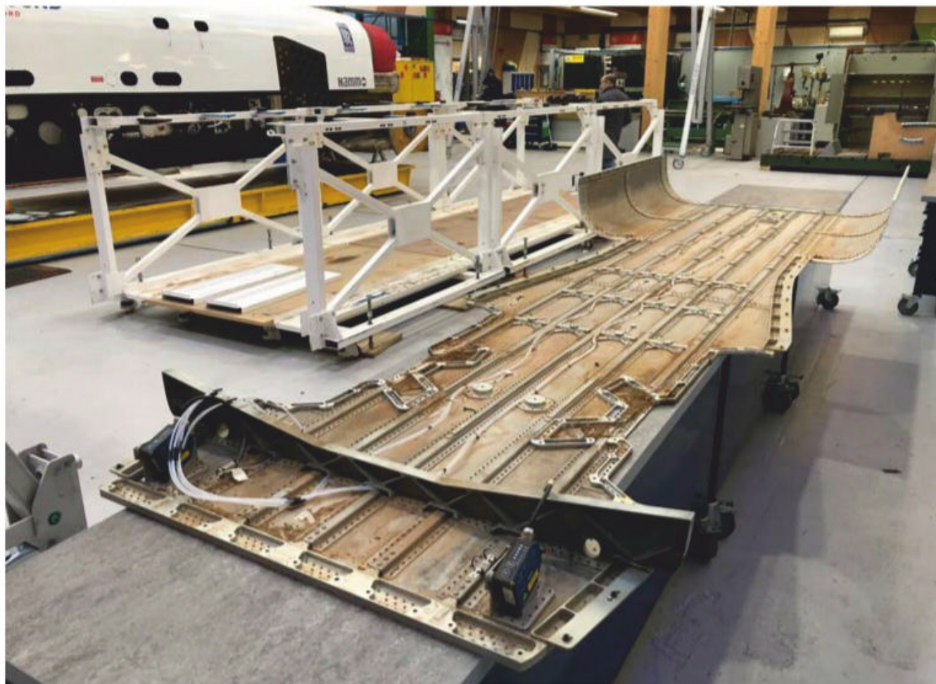
Above and below: stripped down for assessment and maintenance, Bloodhound LSR shows signs of a life well lived, the dust and debris from the Hakskeen Pan is evident everywhere you look. All things considered, it stood up very well to the task
