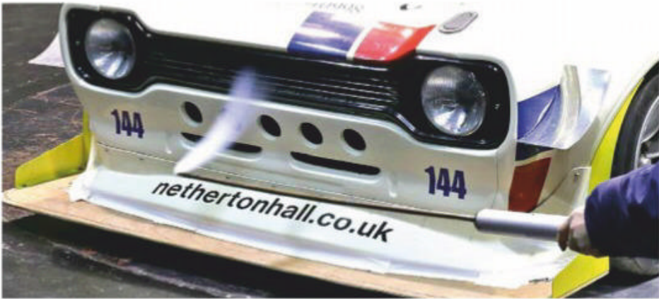
Flow into upper grille aperture inclined steeply upwards
