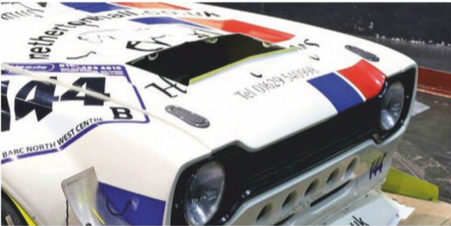
Central aperture in bonnet aided by Gurney on front edge
