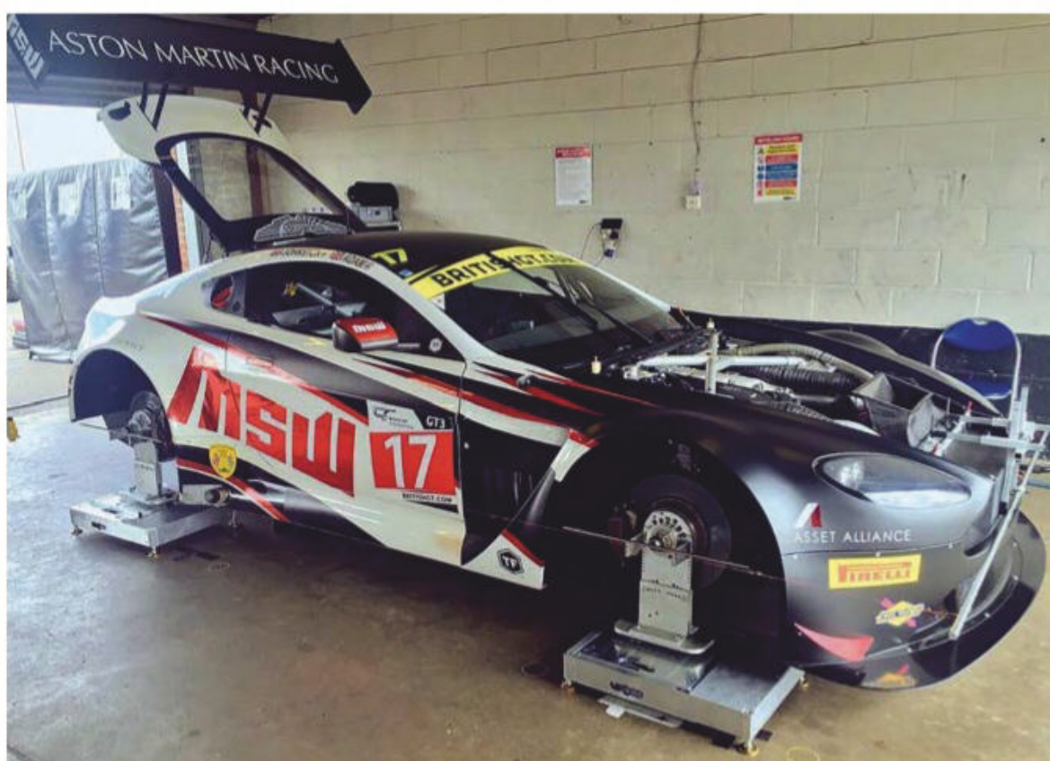
One of the first things teams do upon arrival at a circuit is establish a flat patch, a level surface from where corner weights can be measured and set up changes made to geometry and ride height
