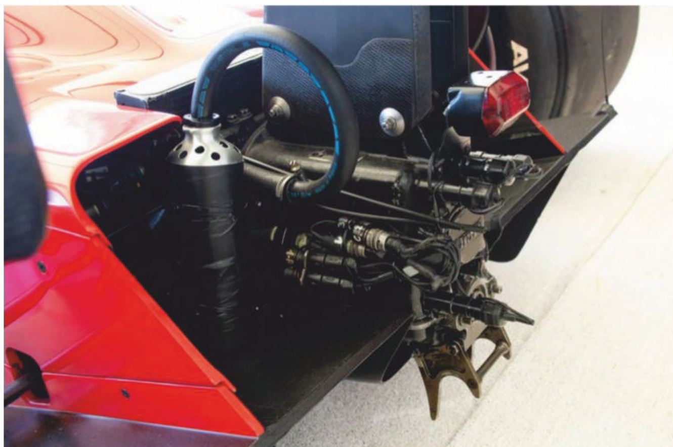
The numerous and complex hydraulic connections that actuated the revolutionary seven-speed gearbox
