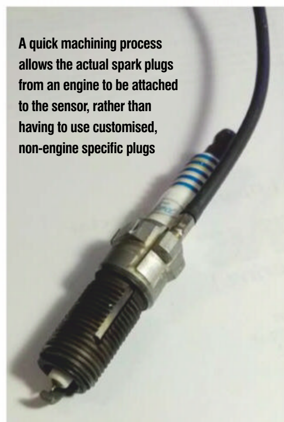
Top-end categories such as F1 most likely use piezoelectric pressure sensors, with the quartz crystal shown here in blue
