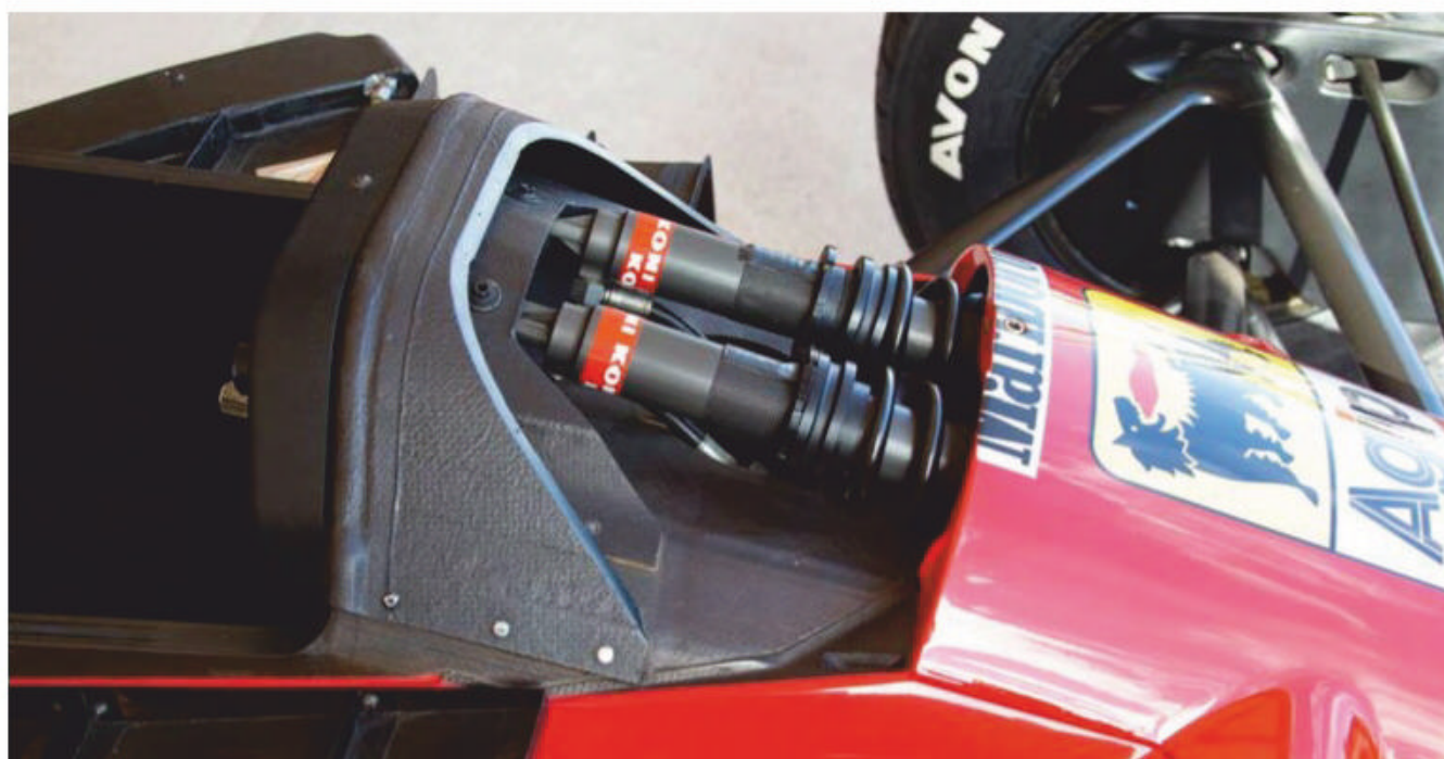
The 1988 639 which was tested and never raced still had conventional coil springs, which were replaced by vertically-mounted torsion bar set up on the 640 F1 which took part in the 1989 season with varying degrees of success
