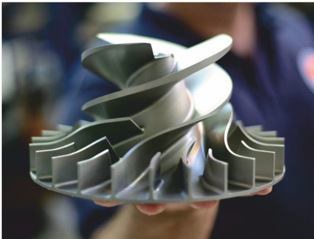
Required to deliver 800 litres of fuel at 1,000psi in just 20 seconds, the design of the pump impeller has been critical
