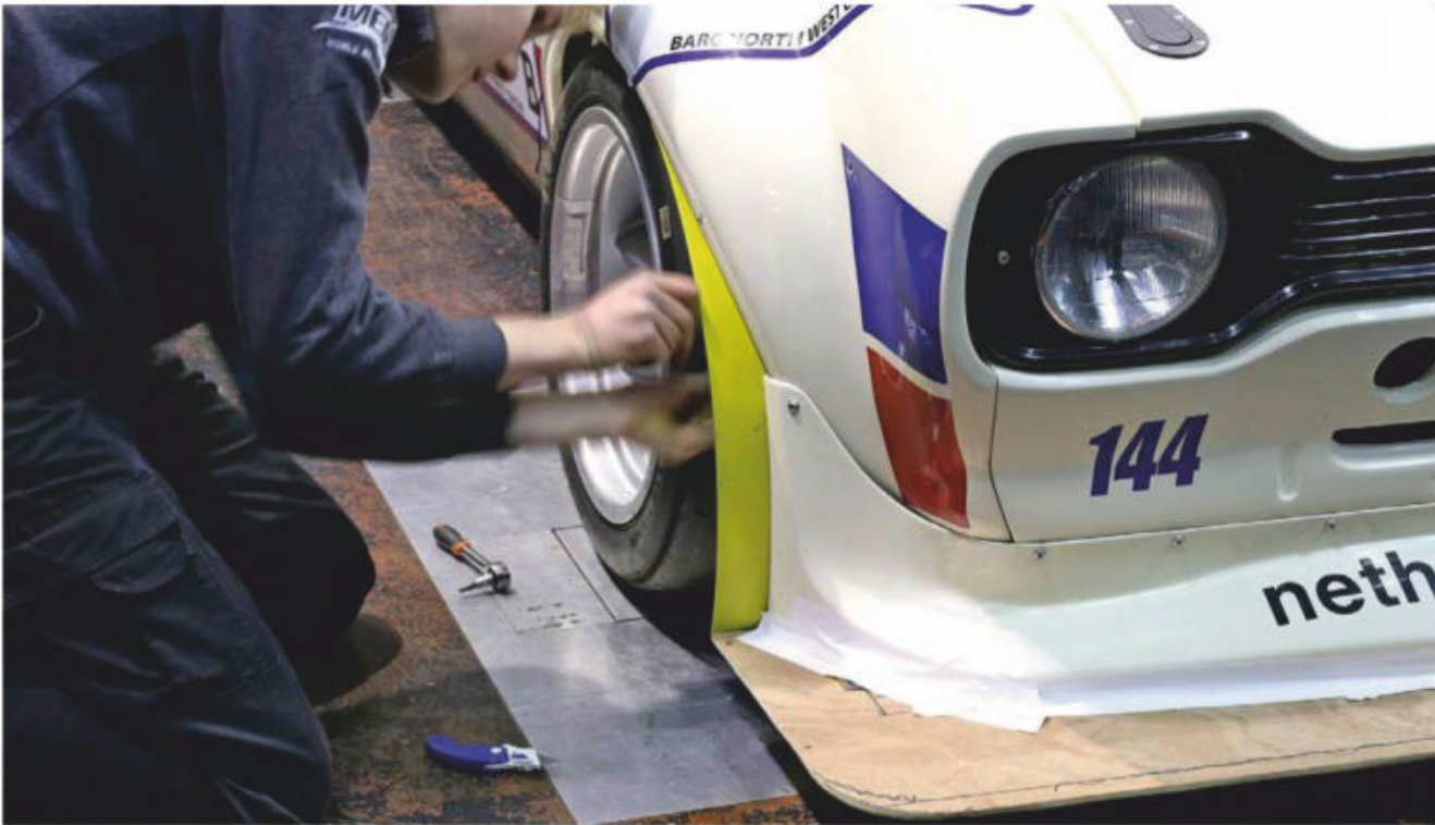
Installing wheelarch Gurneys (WAGs) for testing
