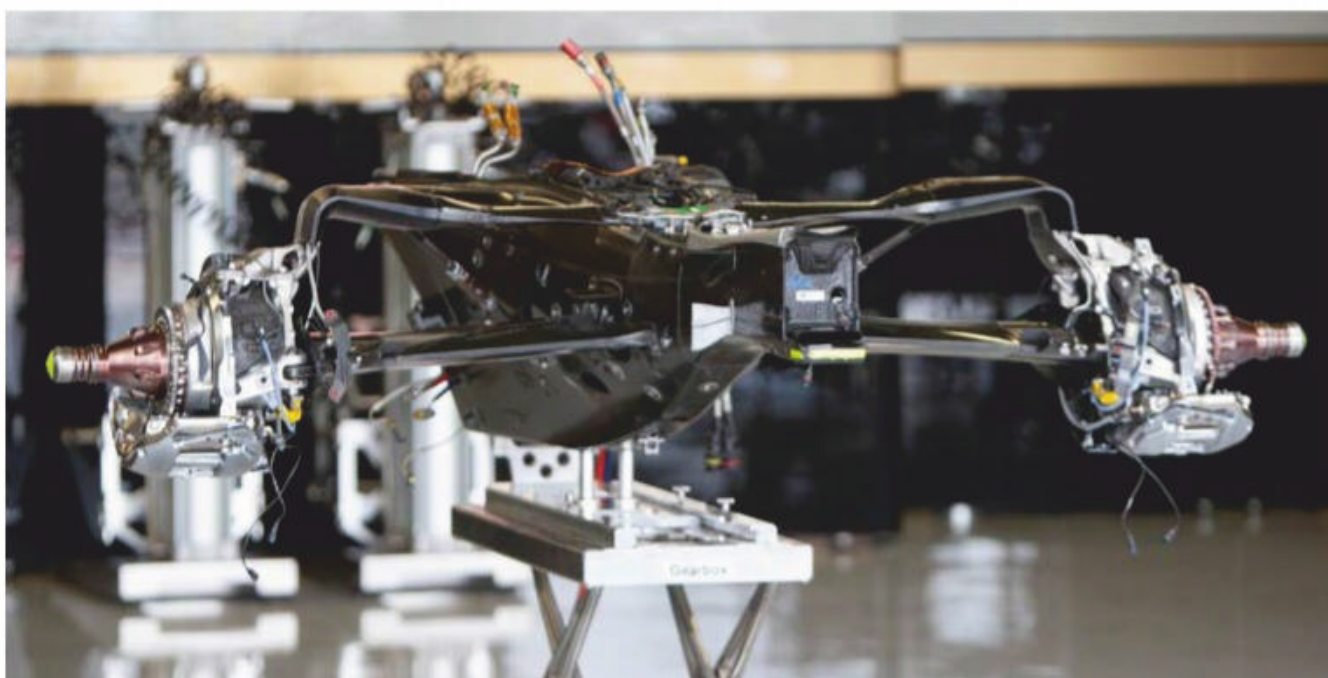
Tuning the gearbox to the harmonics of particular engines would take more than just changing the input shaft, says Ricardo
