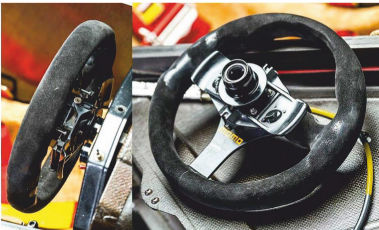
Working with Magneti Marelli, Barnard reprised Forghieri's paddle shift concept but with electro-hydraulic actuation
