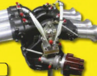
Greenwood "Spirit of 76" LeMans Corvette. Ran Kinsler crossram manifold with Lucas mechanical metering.
