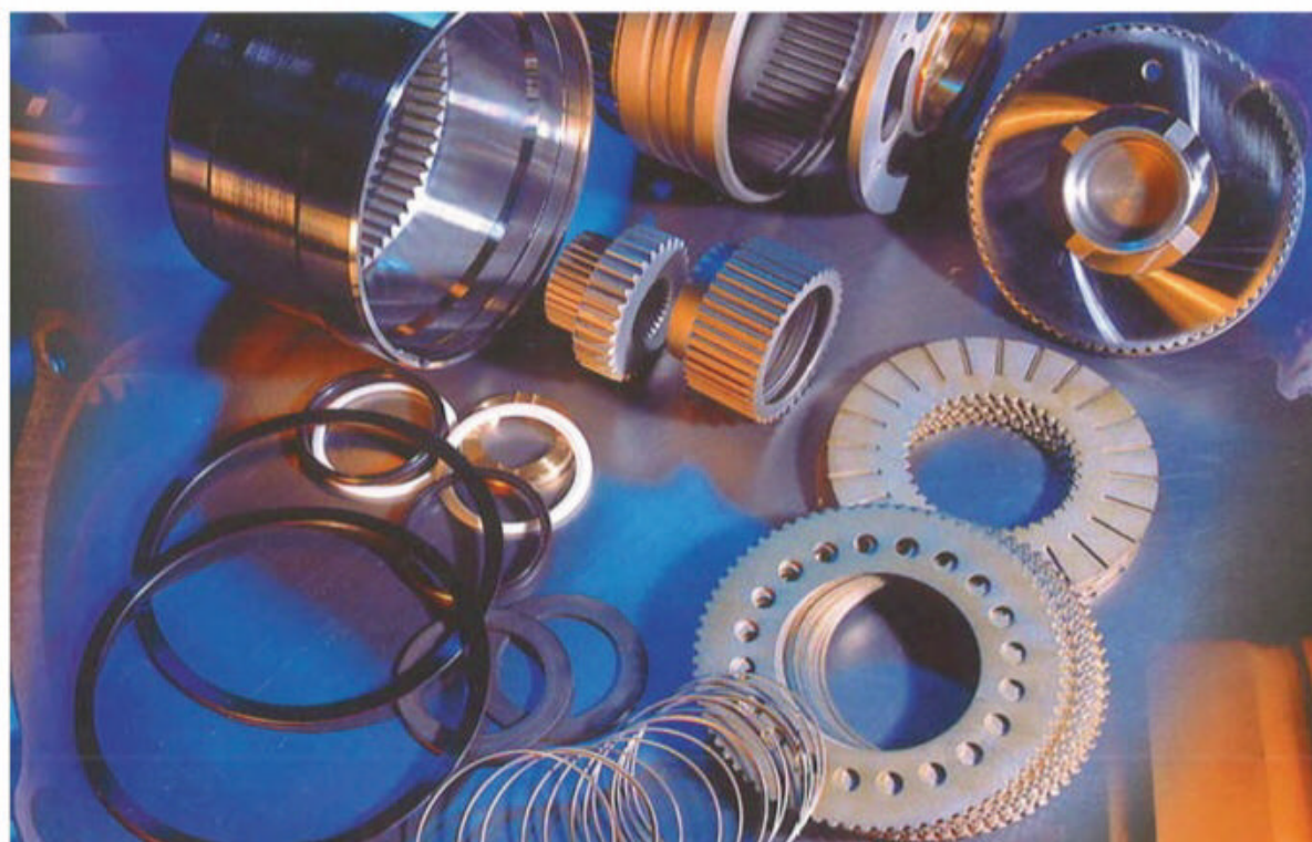
The parts that make up a viscous coupling type differential from Ricardo
