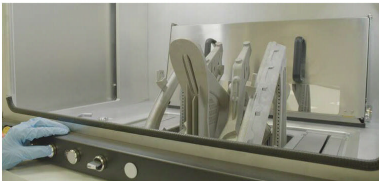
When the print job is complete, a vacuum cleaner system draws out any residual powder, which is sieved and then re-used
