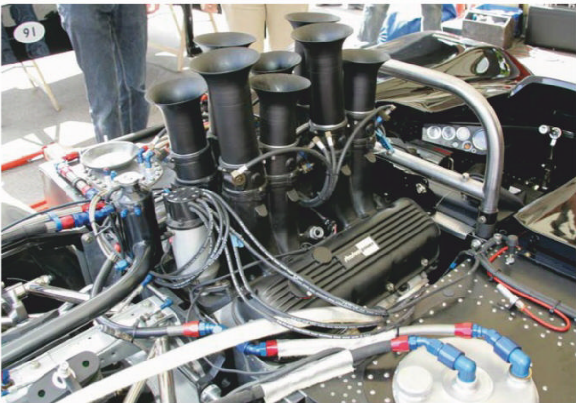
Power came from a brutal big block Chevrolet V8 with Kinsler / Hilborn constant flow fuel injection
