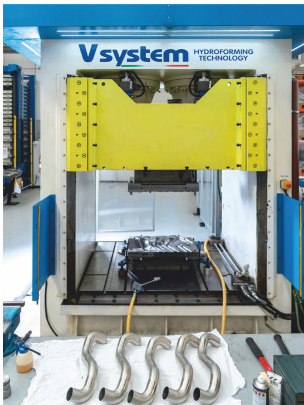
A hydroforming press equipped with a hydro tool. Examples of what can be achieved in the foreground
