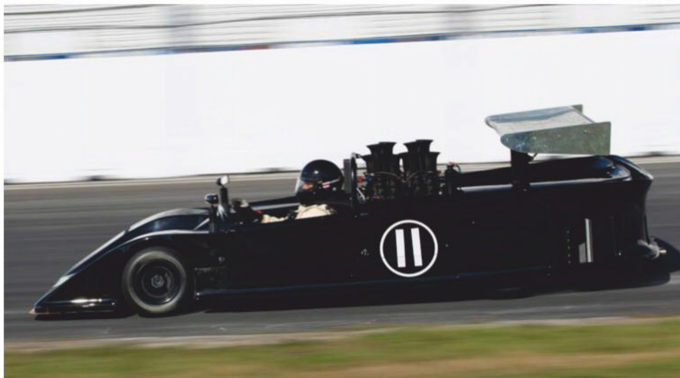
The first major compromise to the original design was the addition of a full-width rear wing as the car lacked downforce
