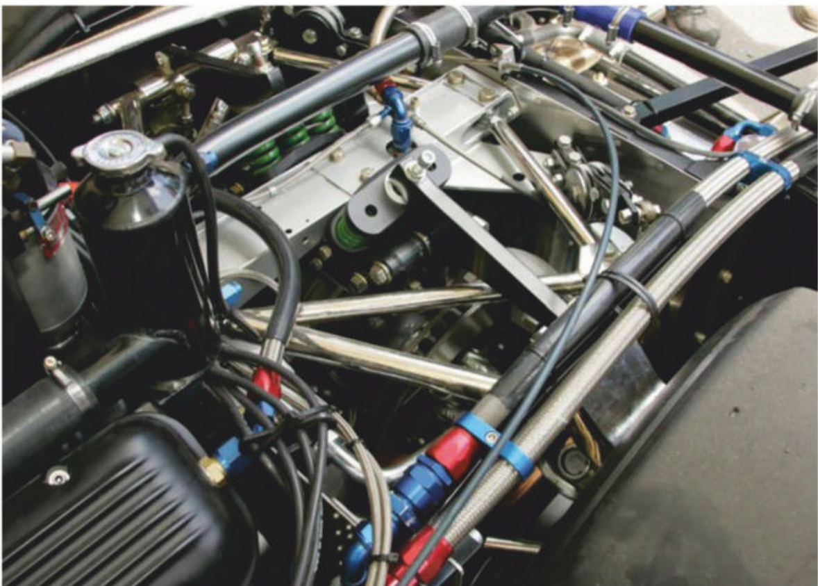
The rear suspension used three small coil springs each side, mounted inboard and with pushrod actuation
