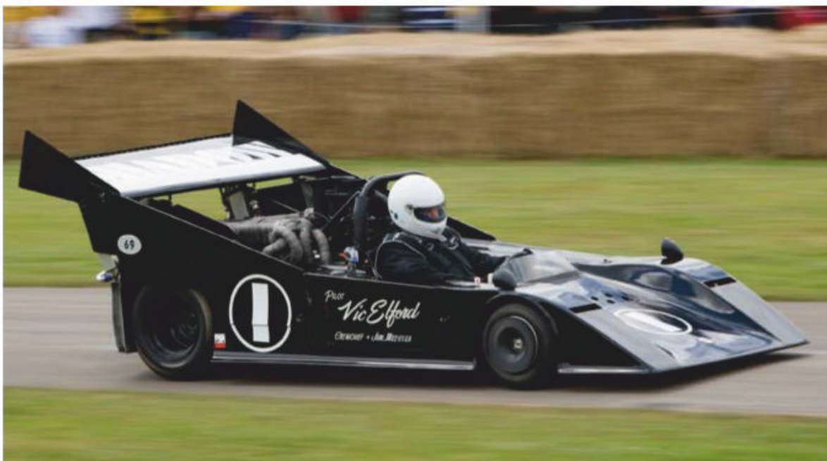
The car as raced by Vic Elford with wing-mounted radiators. It was said to be unstable on long straights
