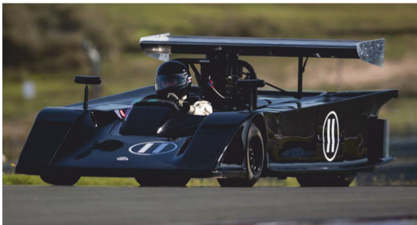
The first major compromise to the original design was the addition of a full-width rear wing as the car lacked downforce
