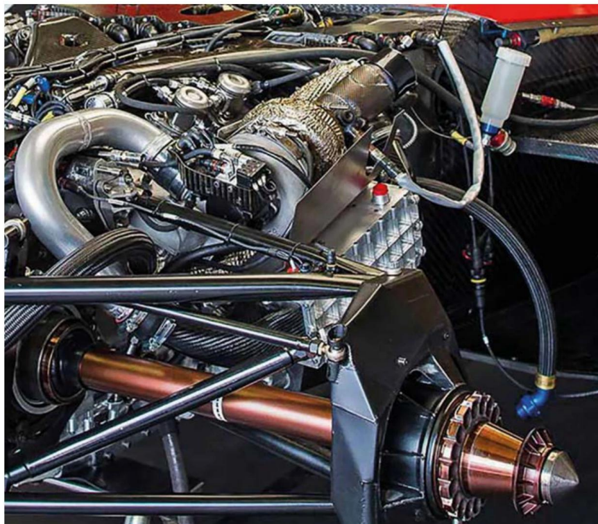
This detail of the AAR-fabricated front suspension shows the sturdy Metalore driveshaft, sized for engine power and also for harvesting duty. You can also see the oil / air turbo heat exchanger under the turbo
