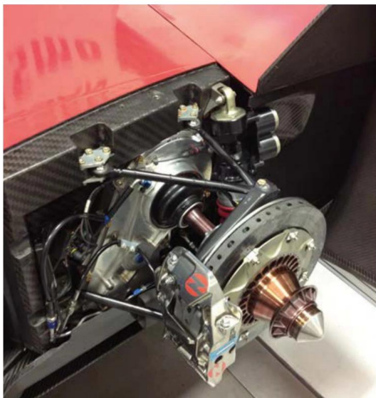
The rear suspension, due to packaging constraints caused by the through ducts, was overly complex but very fine in construction
