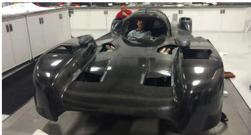
Yep, I think I can see the apex! 220 individual composite parts went into the construction of each GT-R
