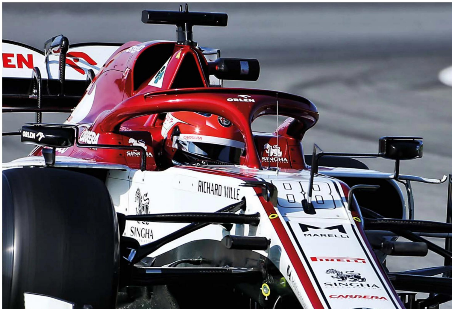
The unique two-tiered arrangement of the engine air intake has been refined to a more conventional A-shape on the C39, compared to the split oval on the C38 (right)
