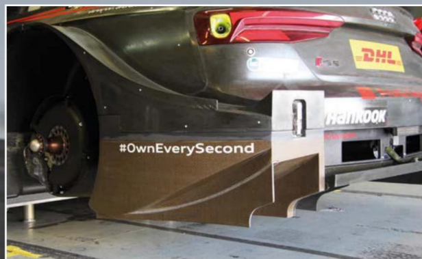
Here the DTM Bcomp natural fibre 'shoebox' being tested by Audi Sport
