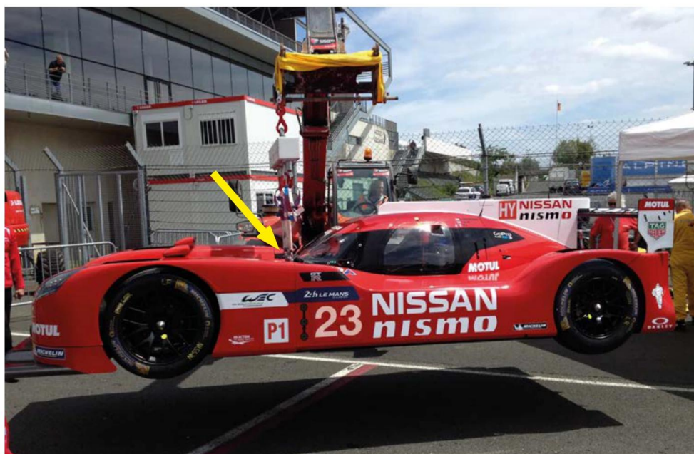
The lifting test at Le Mans that's part of the scrutineering process shows how far forward the centre of mass (indicated by the yellow arrow) was in the GT-R LM. A typical P1 car would have the lifting inserts at the rear of the cockpit
