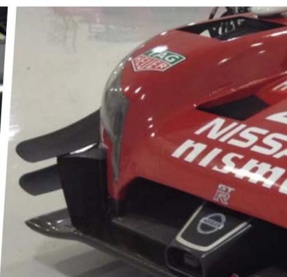
The final 'catcher's mitt' brake duct and radiator inlet splitter seen in 2015 post-Le Mans trim
