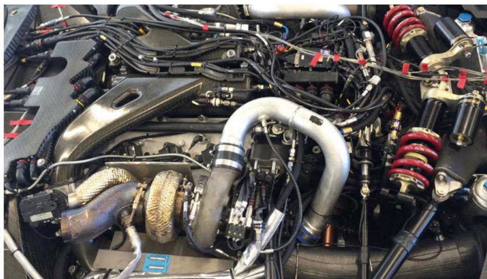
Somewhere beneath all that lot is the specially made Cosworth 3.0-litre V6 direct injection engine, which proved itself efficient and reliable, even if it was a mechanic's nightmare to access it
