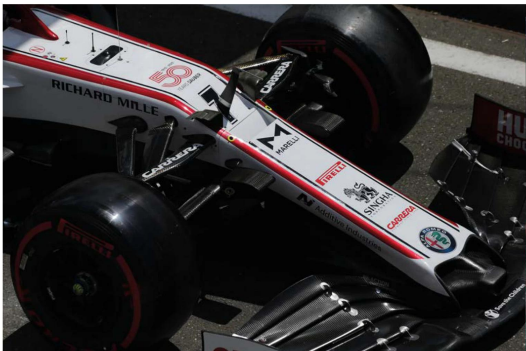
The C39's s-duct outlet is low down the nose and flat, in contrast to the higher, protruding outlet of the Red Bull RB16 (right)
