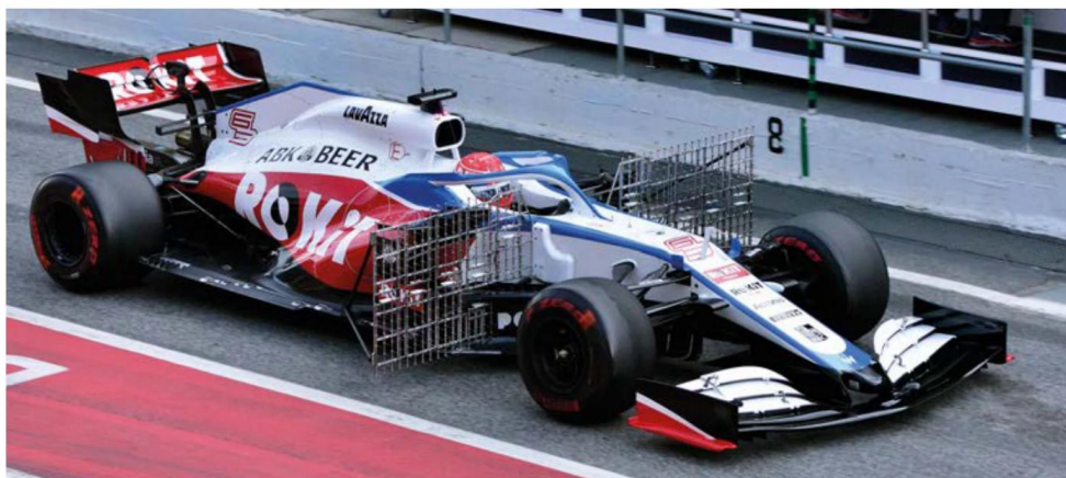
As often seen in Barcelona, all manner of measurement apparatus appear in efforts to correlate lab and CFD methods
