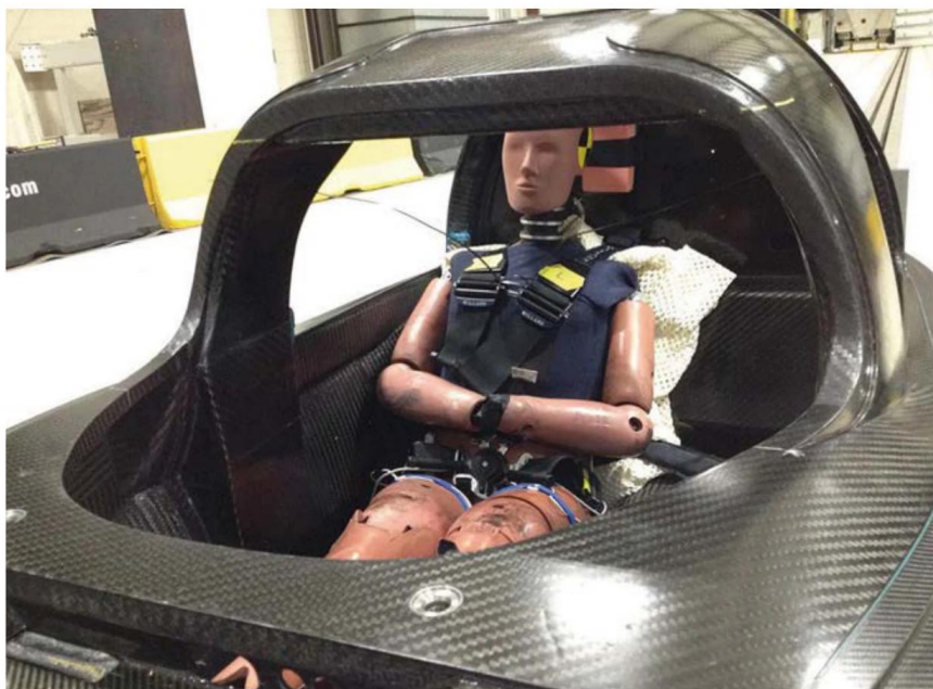
To pass revised crash tests, the right-hand door was re-made as a beefier 1kg part, and resisted the 713kg load, together with the custom latch mechanism designed by my colleague, Brian Oeters
