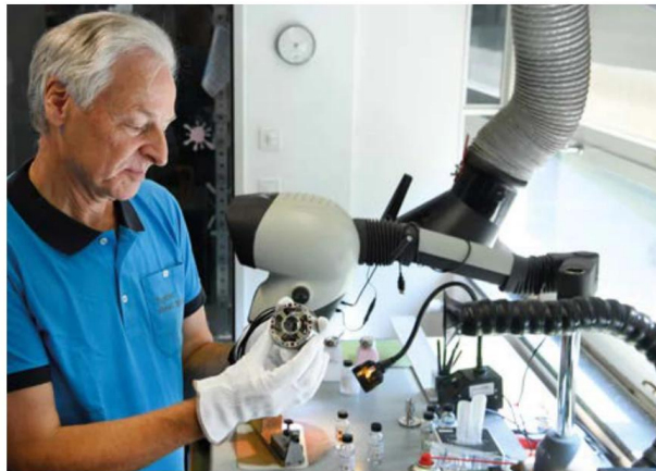
Precision counts. The strain gauges are applied in a controlled environment at exactly defined locations to provide great accuracy in measurement
