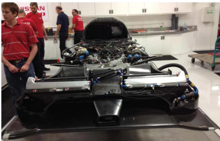
Through ducts meant the radiators had to go in front of the engine. This was a logistical nightmare as the inevitable splitter change took an hour in the race as a 1.5in quick release coupling was too big to package, so the system needed draining, re-filling, bleeding and heating
