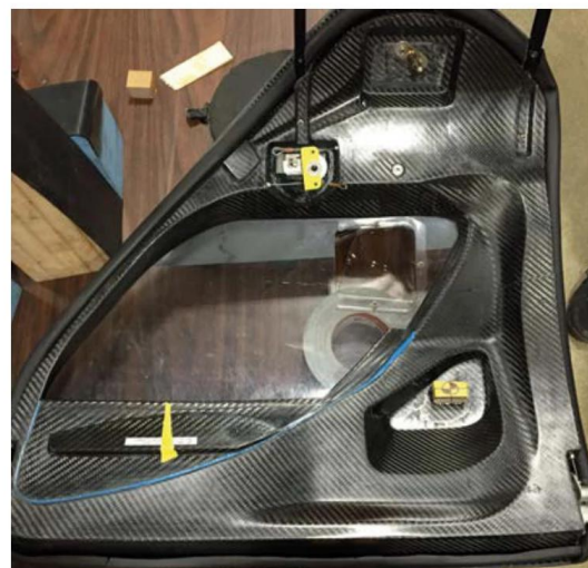
To pass revised crash tests, the right-hand door was re-made as a beefier 1kg part, and resisted the 713kg load, together with the custom latch mechanism designed by my colleague, Brian Oeters
