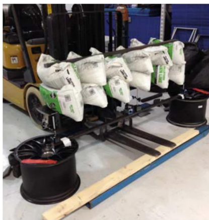
That's a rear wing under 245kg (539lb) of lime. Note the dial indicators at the wing tips
