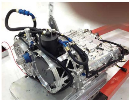
Flybrid two-flywheel ERS was a bold move and promised a potential 700bhp of accelerative power for five seconds, but its multiple wet clutch actuation proved its downfall in practice and reliability issues eventually sidelined the system completely
