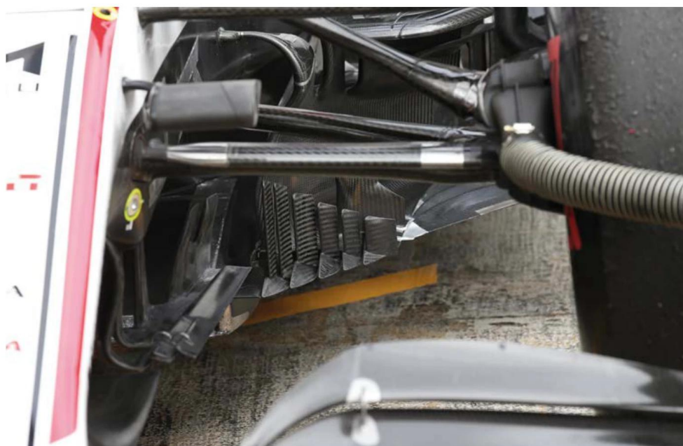
Both the front and rear suspensions have been developed to make the car easier to drive over kerbs
