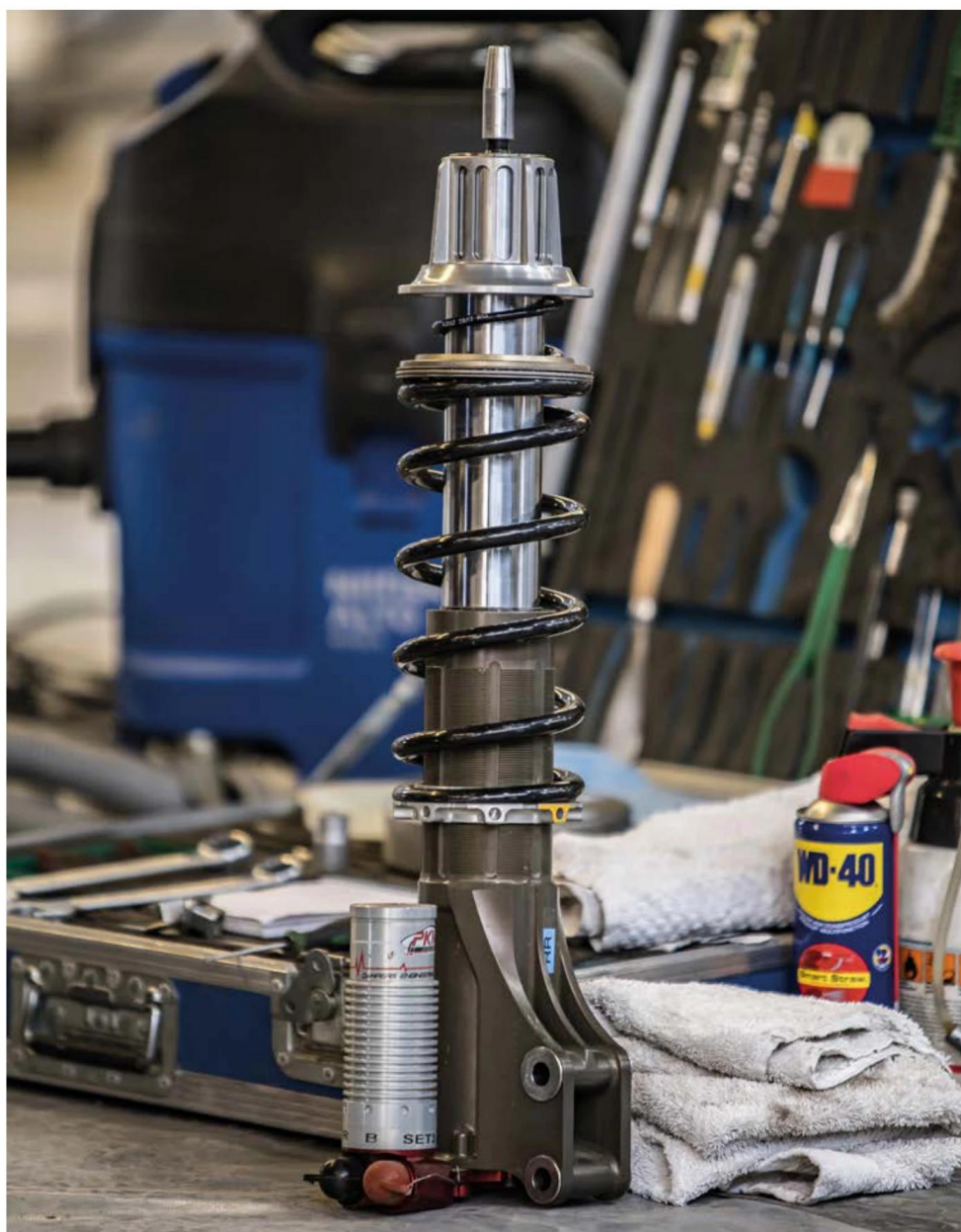
Clutch-equipped mechanical inerters enjoyed a brief period of acceptance in rallying (and Rallycross), where they were used to help control ultra high-frequency suspension and tyre movements, but were banned from the categories in 2018
