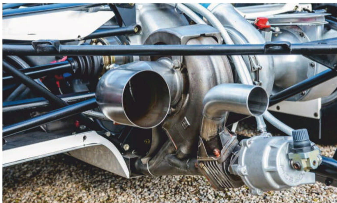
A single Garrett turbocharger was used, but it all hinged on the intake boost pressure the 935/72 engine was allowed to run
