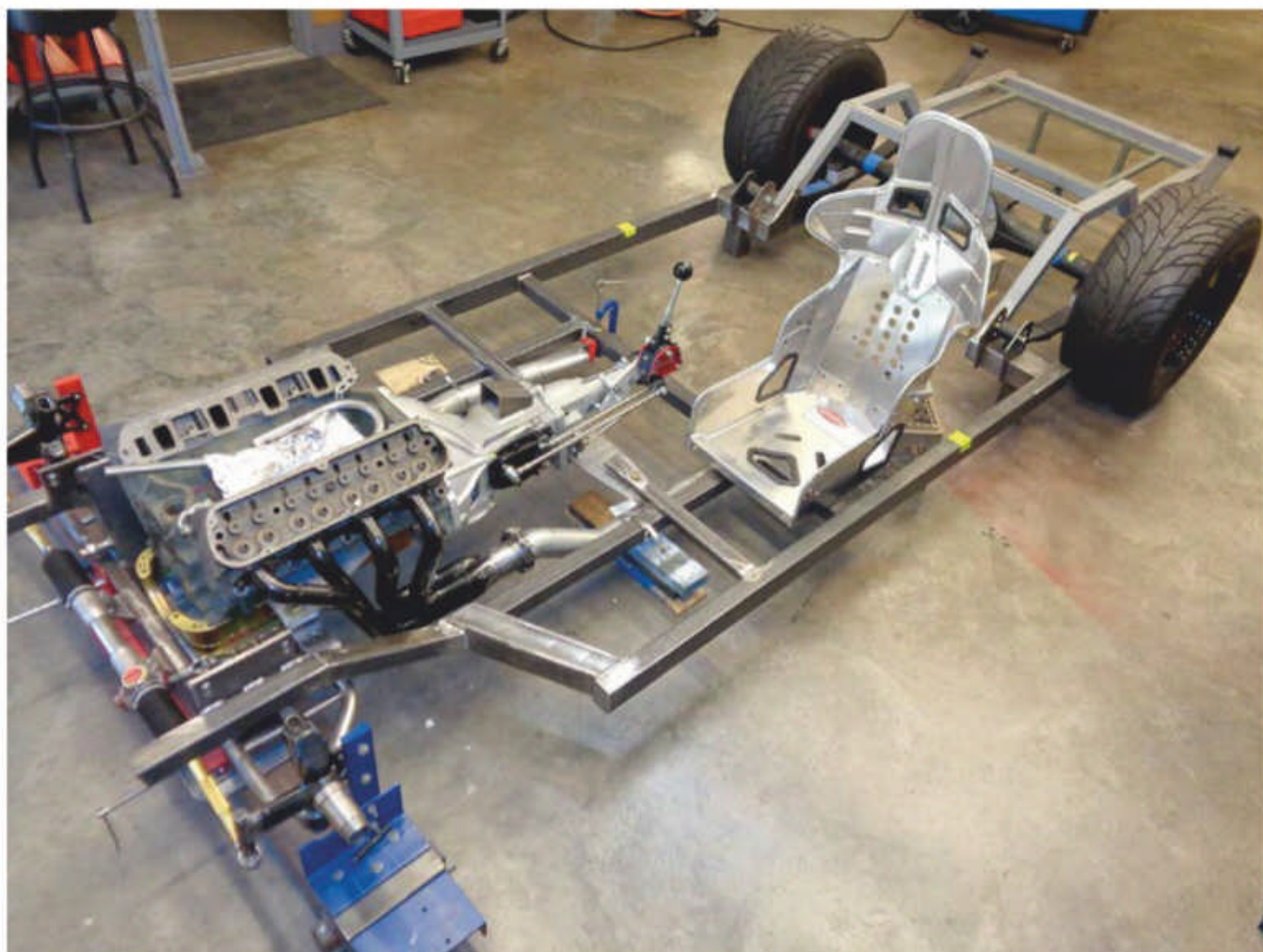
The questioner's 'somewhat vintage reproduction' road course car uses slider-mounted, Chrysler-style leaf spring packs
