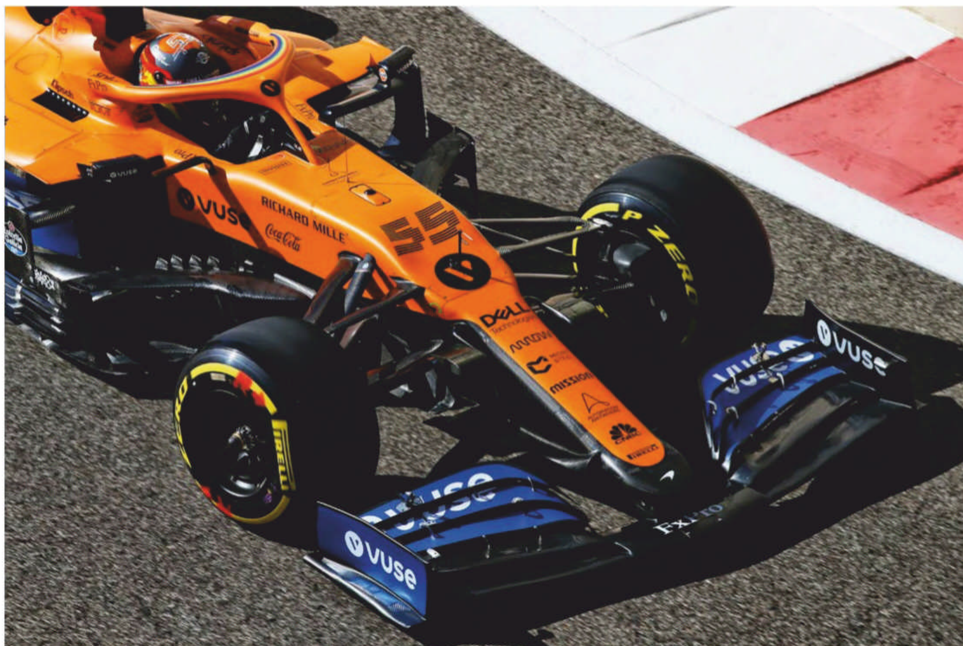
The nose and sidepod design were heavily revised throughout 2020. Here is how the MCL35 appeared with its aerodynamic upgrades at the final race of the season in Abu Dhabi
