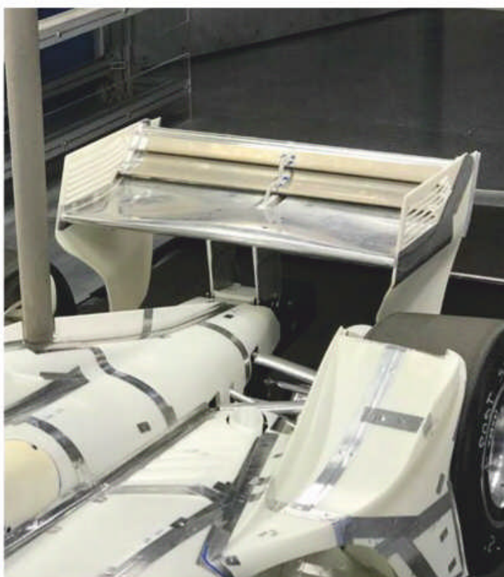
Chris Beatty's 2018 rear wing included tyre ramps and a swept-back design that improved the car's aesthetic while maintaining aero efficiency. The rear wing with almost a truly swept-back end plate was not signed off, despite looking quick enough
