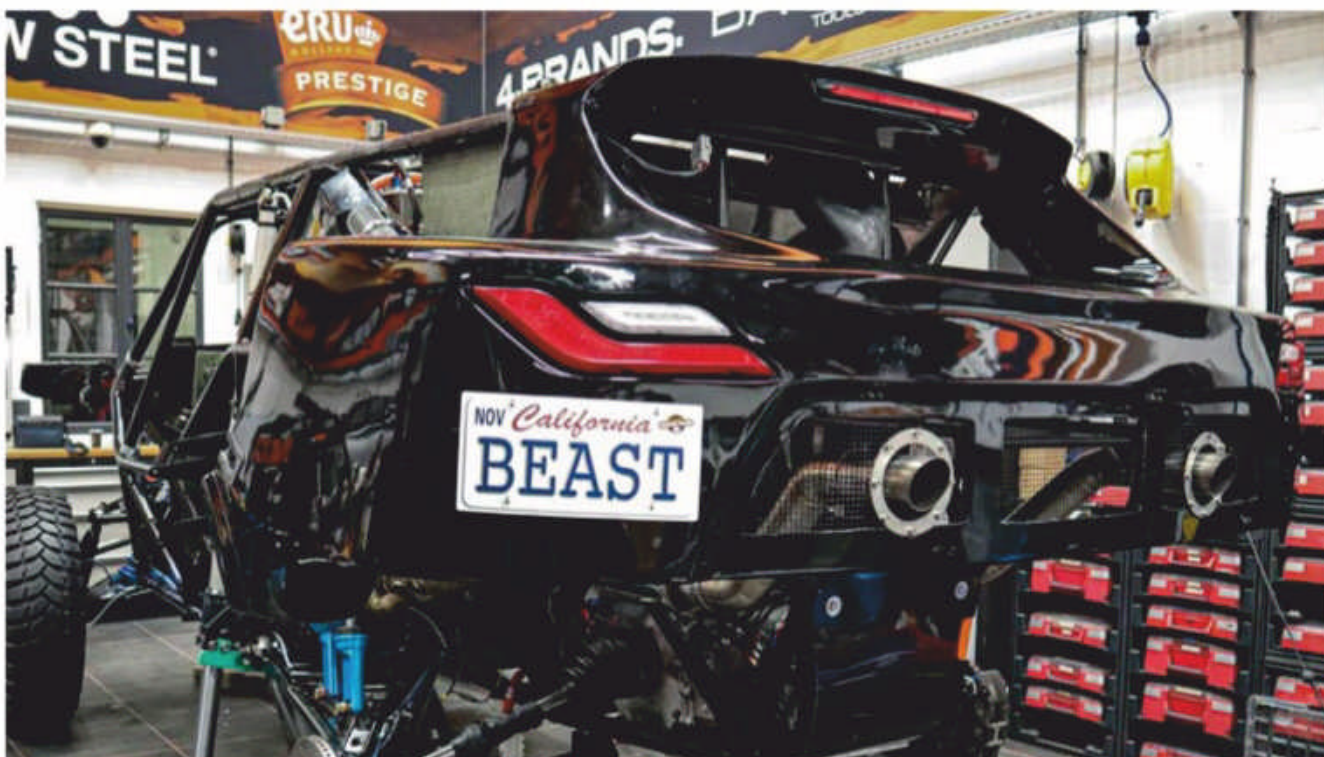
Week 11: The lightweight carbon bodywork, reduced to the thinnest skins possible by Dutch company Van Thull, goes on
