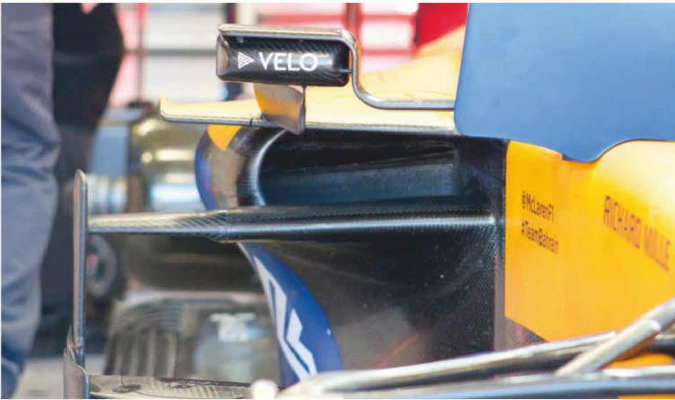
The mid-height side impact structure concept was also adopted by McLaren for its MCL35
