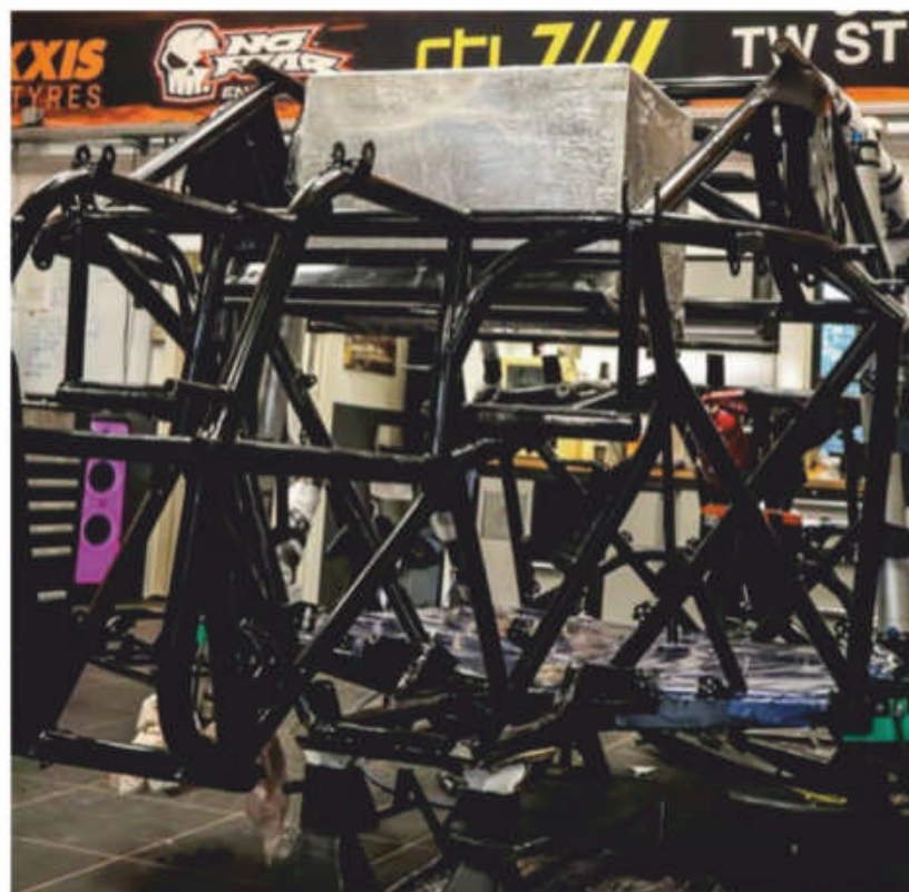
Week 1: Fuel tank and fluids are mounted high up for rollover protection
