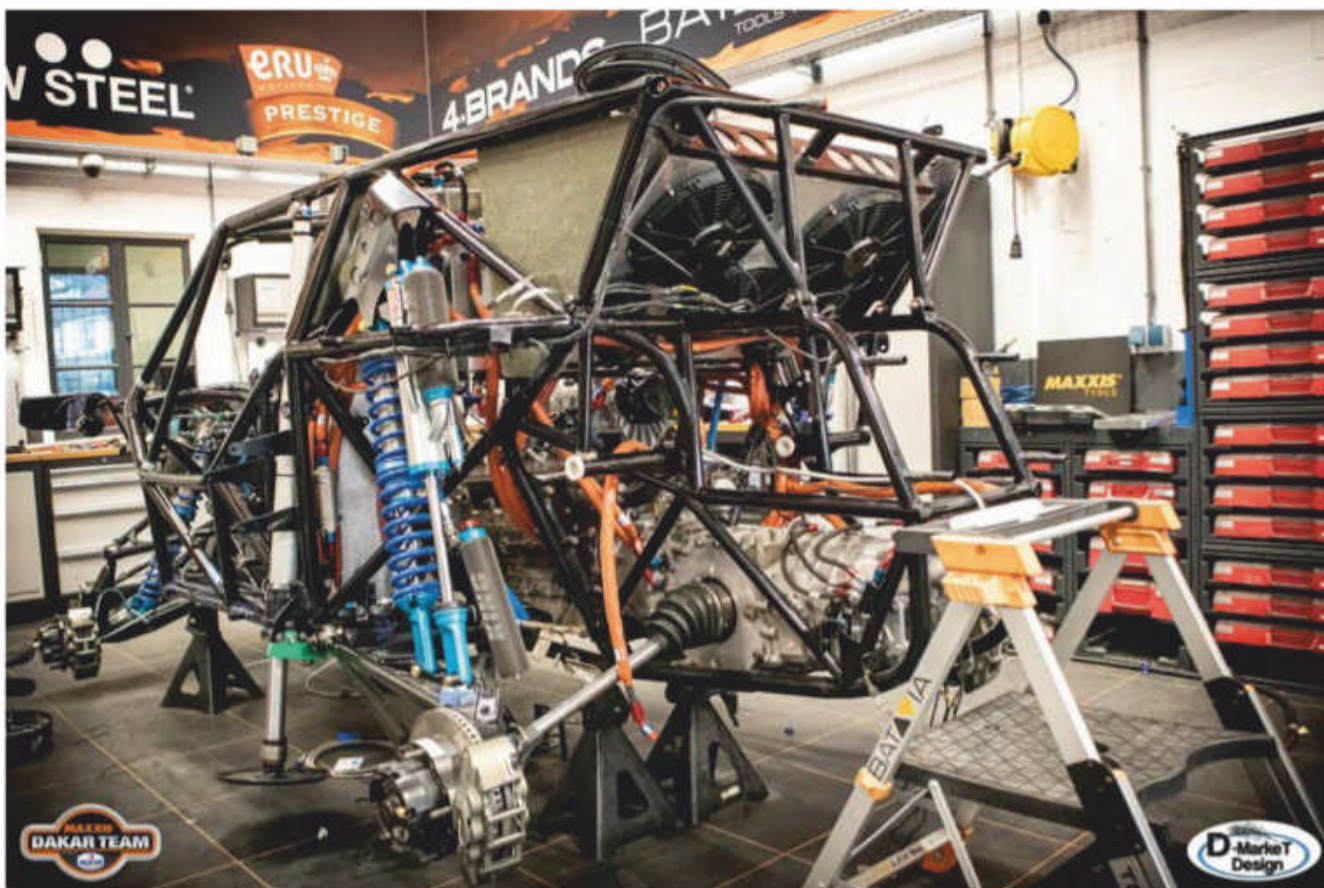
Week 10: The Beast almost complete and race ready, weighing in at 200kg less than the original base weight of the chassis
