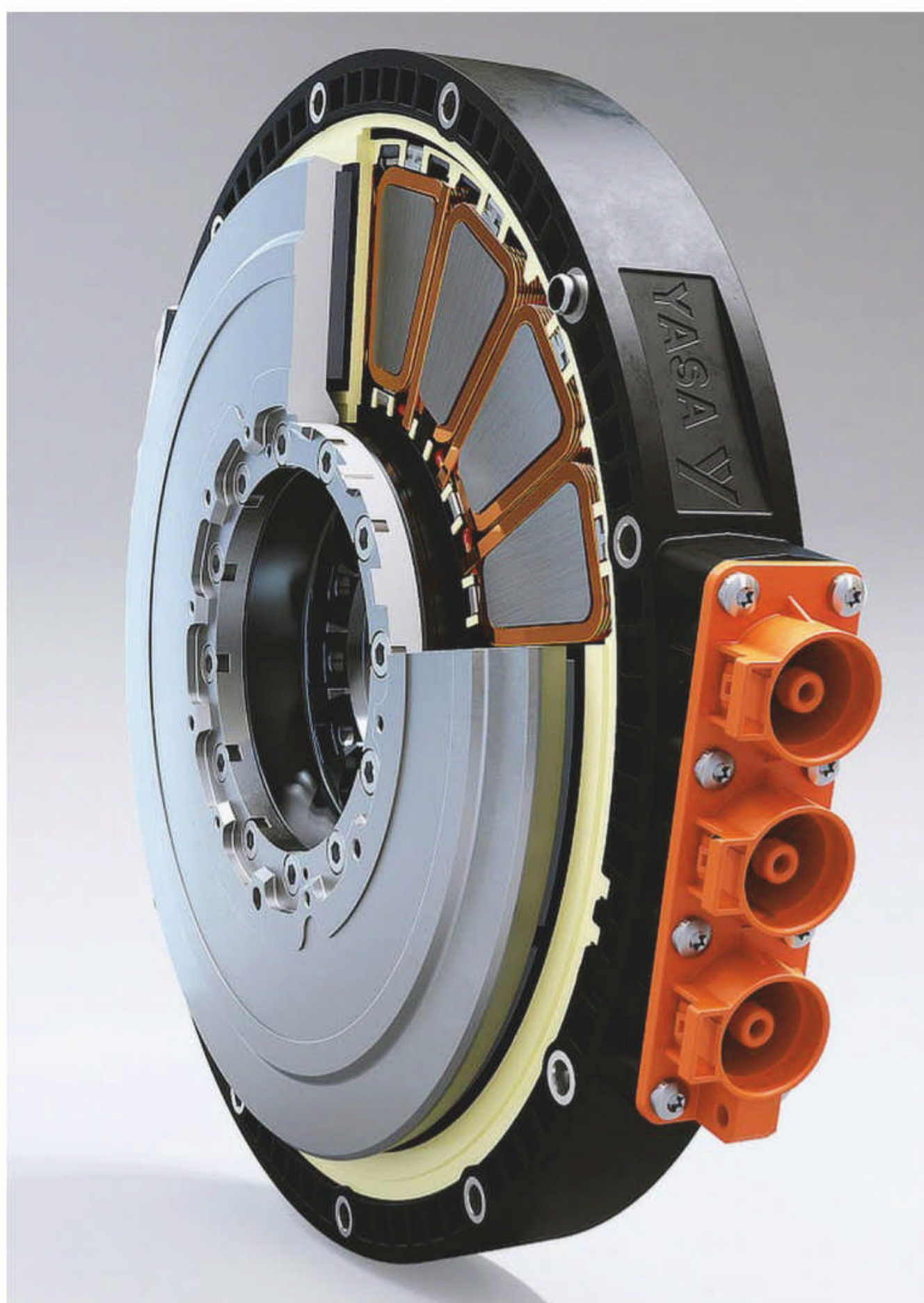
YASA (Yokeless And Segmented Armature) is a compact, lightweight, powerful type of axial flux motor with no stator yoke
