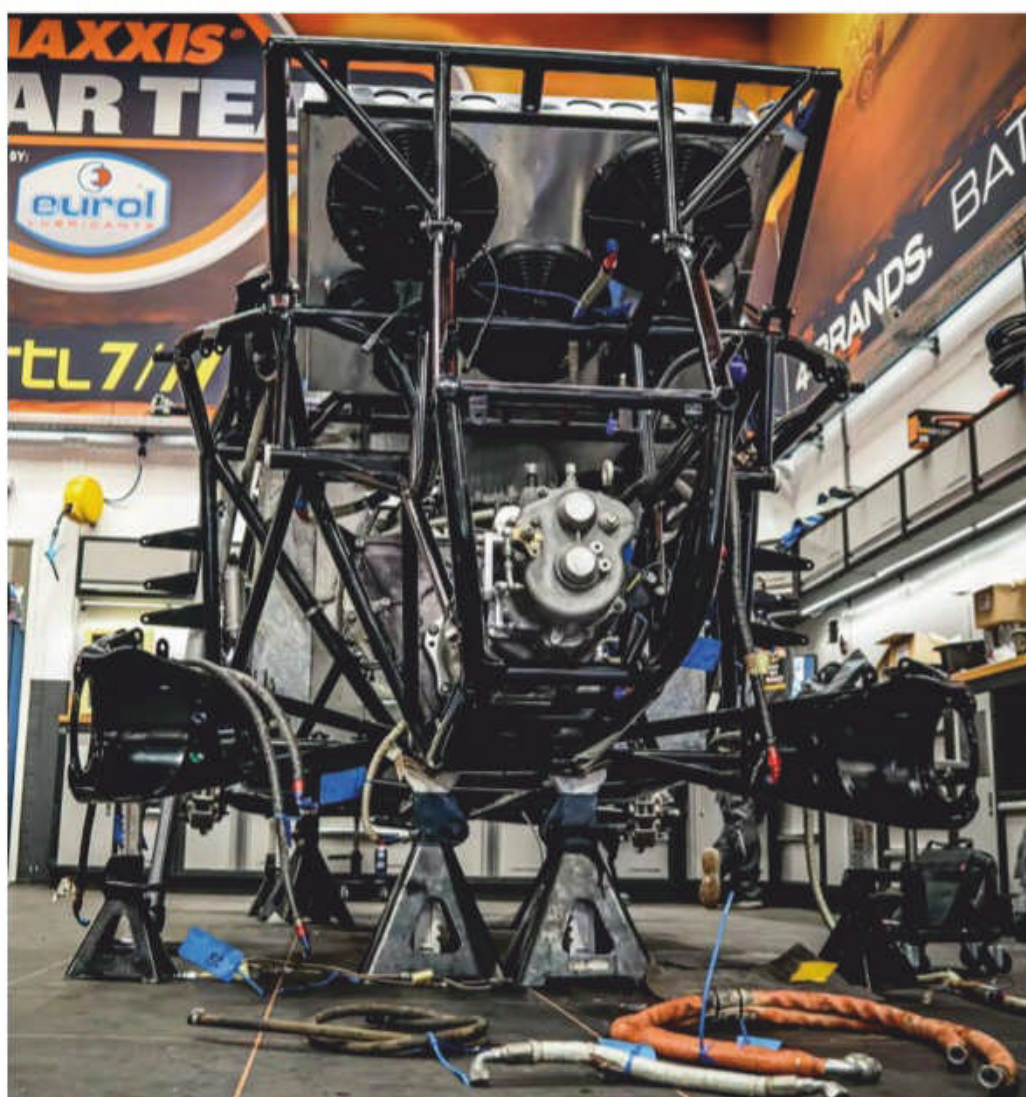
Week 6: A late decision to change the fluid lines from metal to Dyneema yielded an astonishing 18kg weight saving
