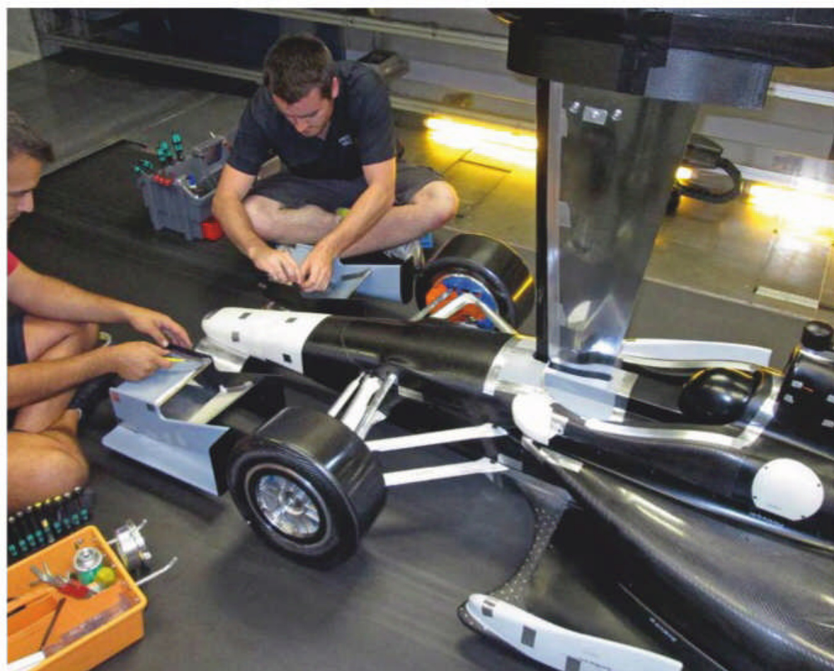
Chevrolet's AeroKit for was tested extensively at 50 per cent before being introduced for the 2016 season
