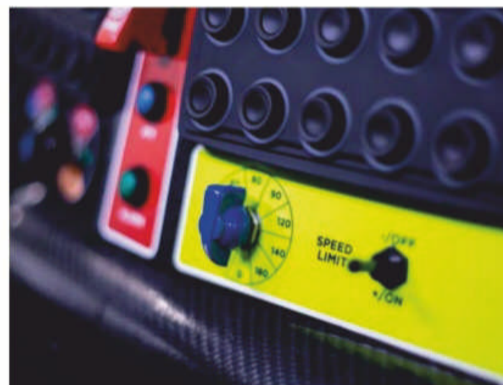
With variable, and enforced, speed limits on road sections of the course an electronically-controlled speed limiter is vital equipment
