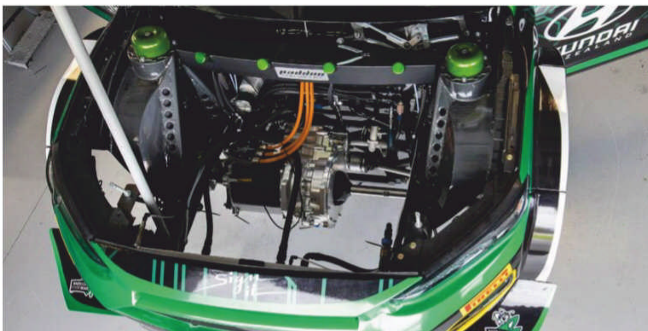
Power comes from two 200kW motors, one on each axle, both with its own transmission. This gives it significantly more available power than an ICE WRC already, but with the capacity to accept four motors for double that total power output
