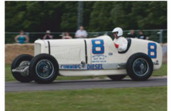
Cummins' 1931 entry used a four-cylinder motor in a Duesenberg chassis. It lacked outright pace, but was the first car ever to finish the race without refuelling
