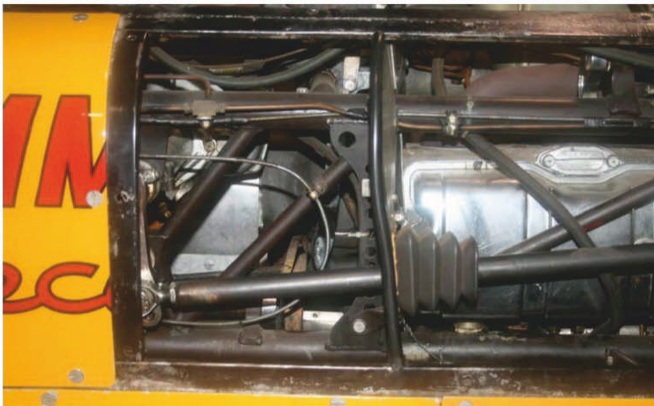
Mounting the sump, gearbox and driveshaft on the left side of the car aided weight distribution, and the driver sat lower, too
