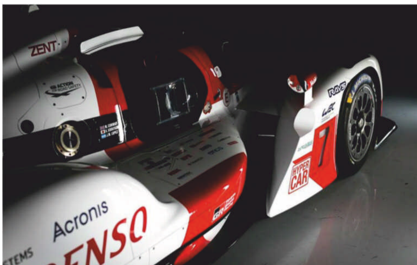
Airflow at the side of the car is directed through the radiators and into a Coke bottle effect, starting ahead of the rear wheels
