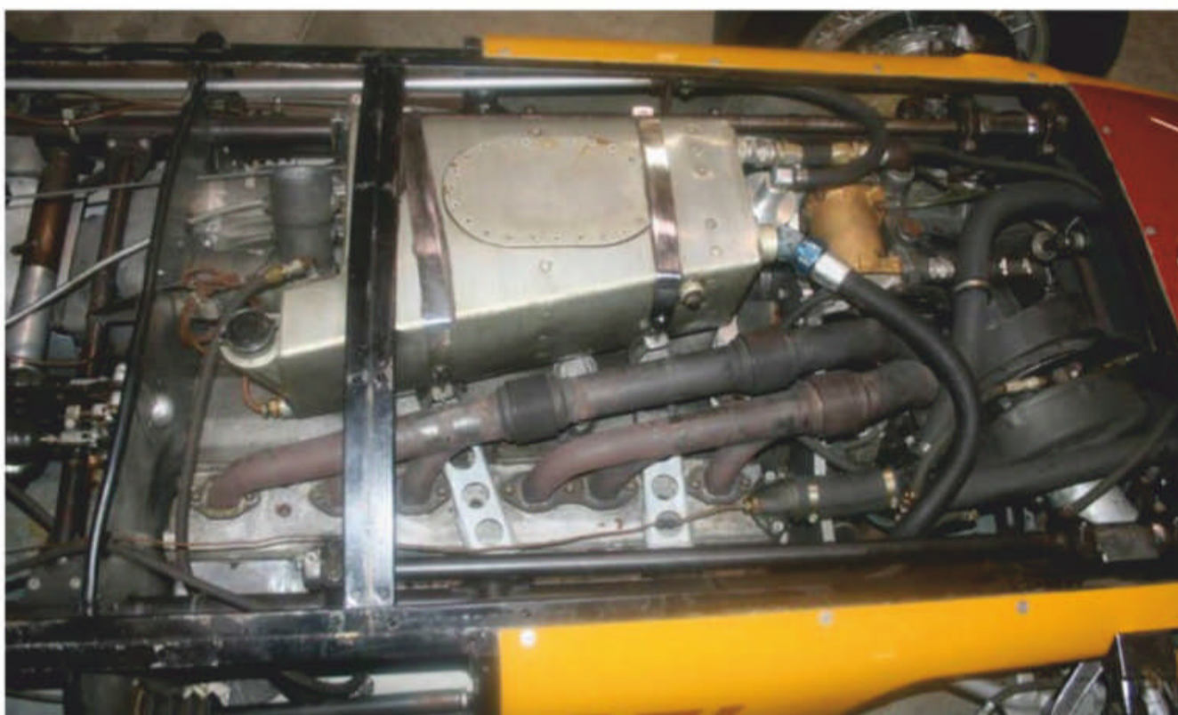
Cummins engineers experimented with alloys for weight reduction. The racing block was magnesium, the head aluminium
