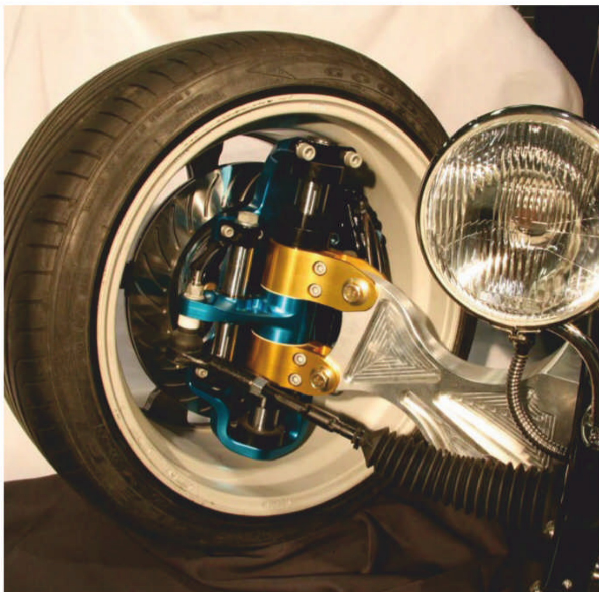
Multimatic's ingenious in-wheel sliding pillar suspension. In response to The Consultant's comment about bump steer, Larry Holt, executive VP Multimatic Special Vehicle Operations, notes: 'The observation [on bump steer] is incorrect. The tie rod end does not move with the suspension at all.'
