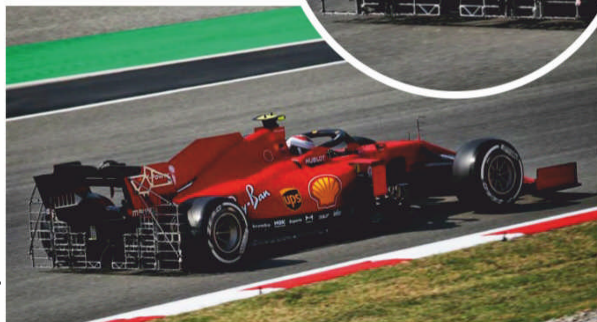
Ferrari SF1000 fitted with sensor equipment at practice day in Barcelona before the Spanish Grand Prix
