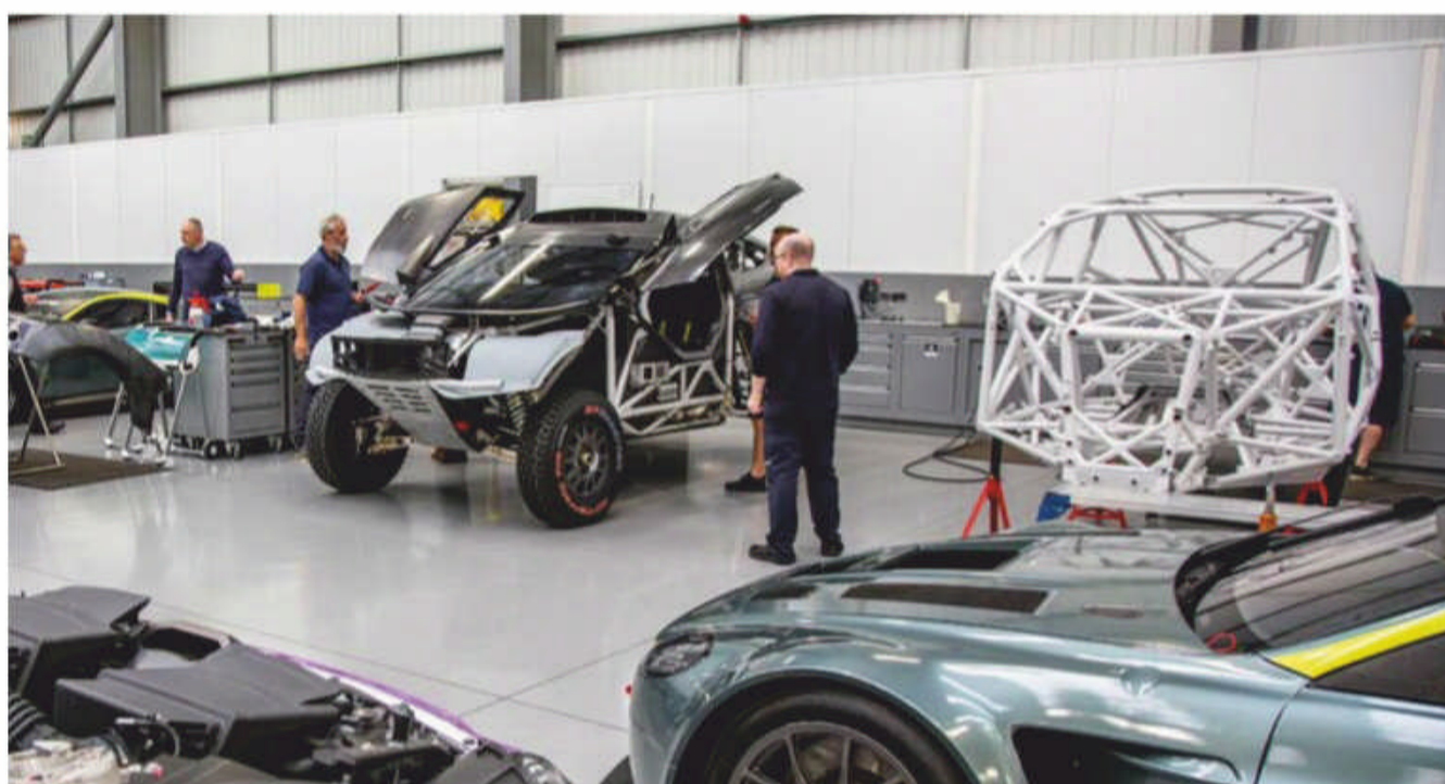
A brace of BRX Hunter T1s during assembly at Prodrive in the UK, one chassis in white and one car almost fully assembled
