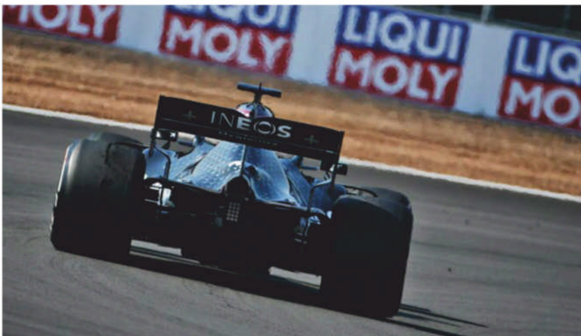
On ground effect cars, good ride height control affects both downforce and downforce distribution
