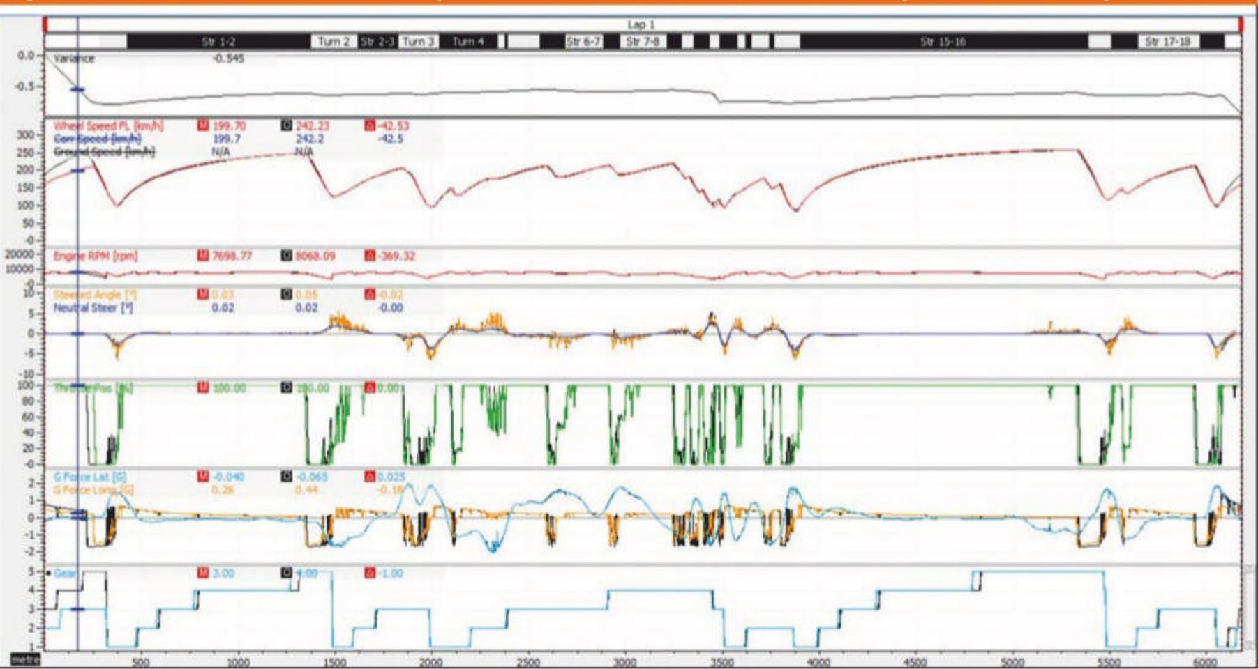
Figure 2: KERS vs non-KERS at Bathurst (non-KERS baseline is coloured, the KERS lap is shown in black)
