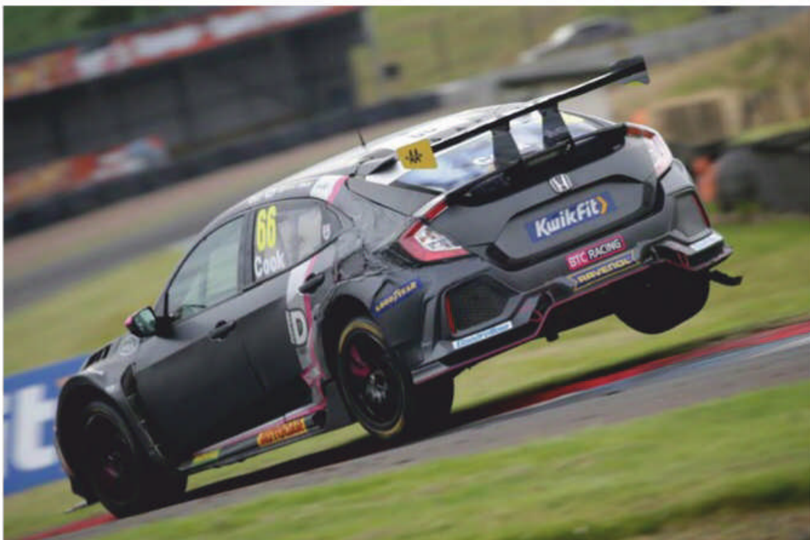
Front engine, front-wheel drive cars have a natural tendency to understeer. This can be tuned out for racing
