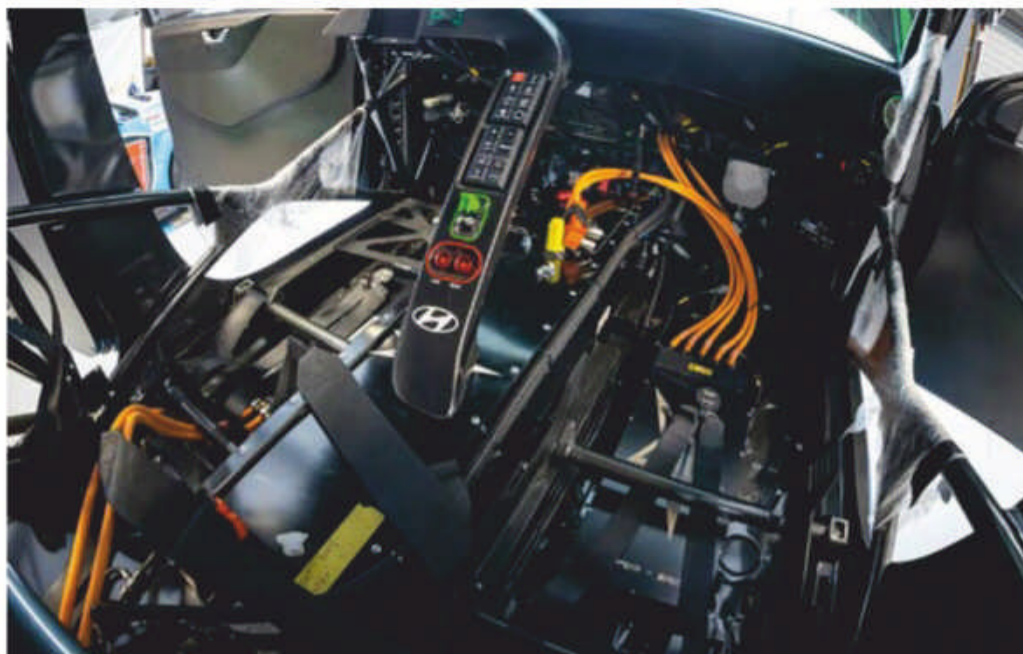
Rollcage structure is deliberately over engineered, with the safety of occupants and marshals in the event of a rollover incident in particular a paramount concern
