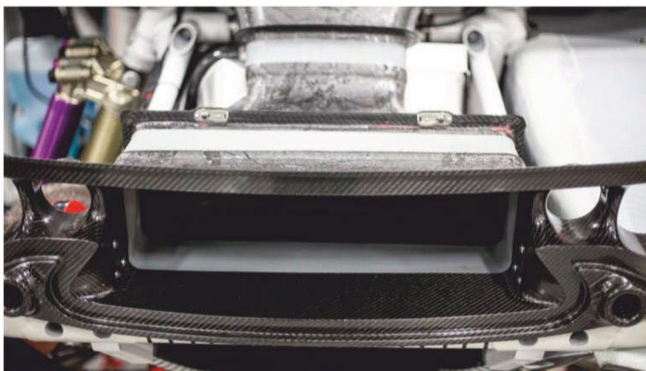
To avoid potential damage, the air intake to the engine is located within the spaceframe chassis structure
