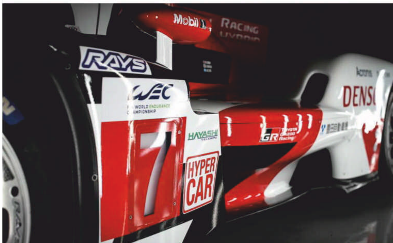
Airflow at the side of the car is directed through the radiators and into a Coke bottle effect, starting ahead of the rear wheels
