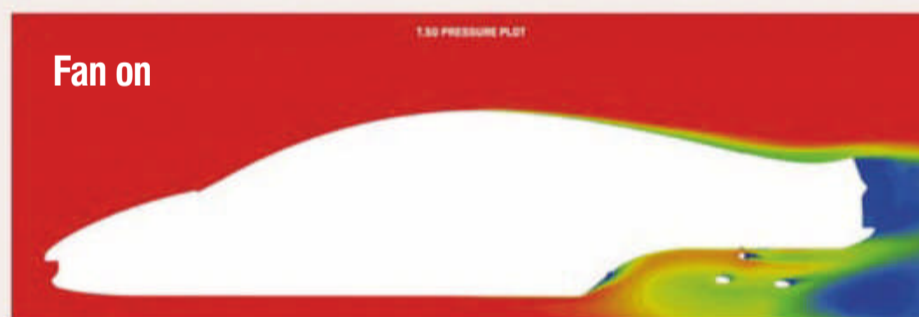
Total pressure plot of a cross section of the T.50 through the left hand diffuser tunnel at 150mph
