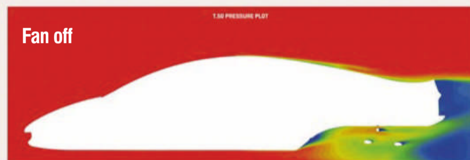
Total pressure plot of a cross section of the T.50 through the left hand diffuser tunnel at 150mph
