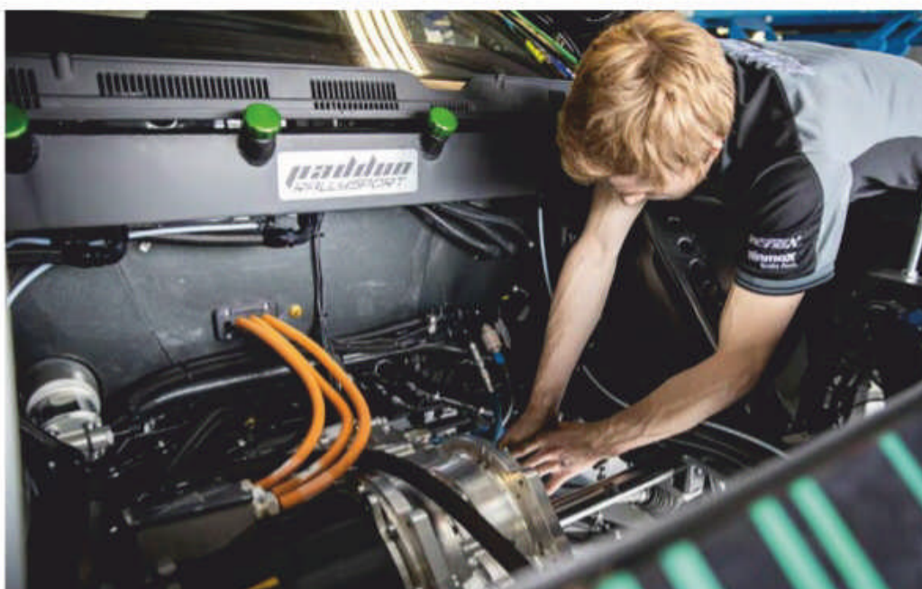
Twin two-speed transmissions rob some of the available power, but give the car greater flexibility for the changeable conditions encountered in rallying
