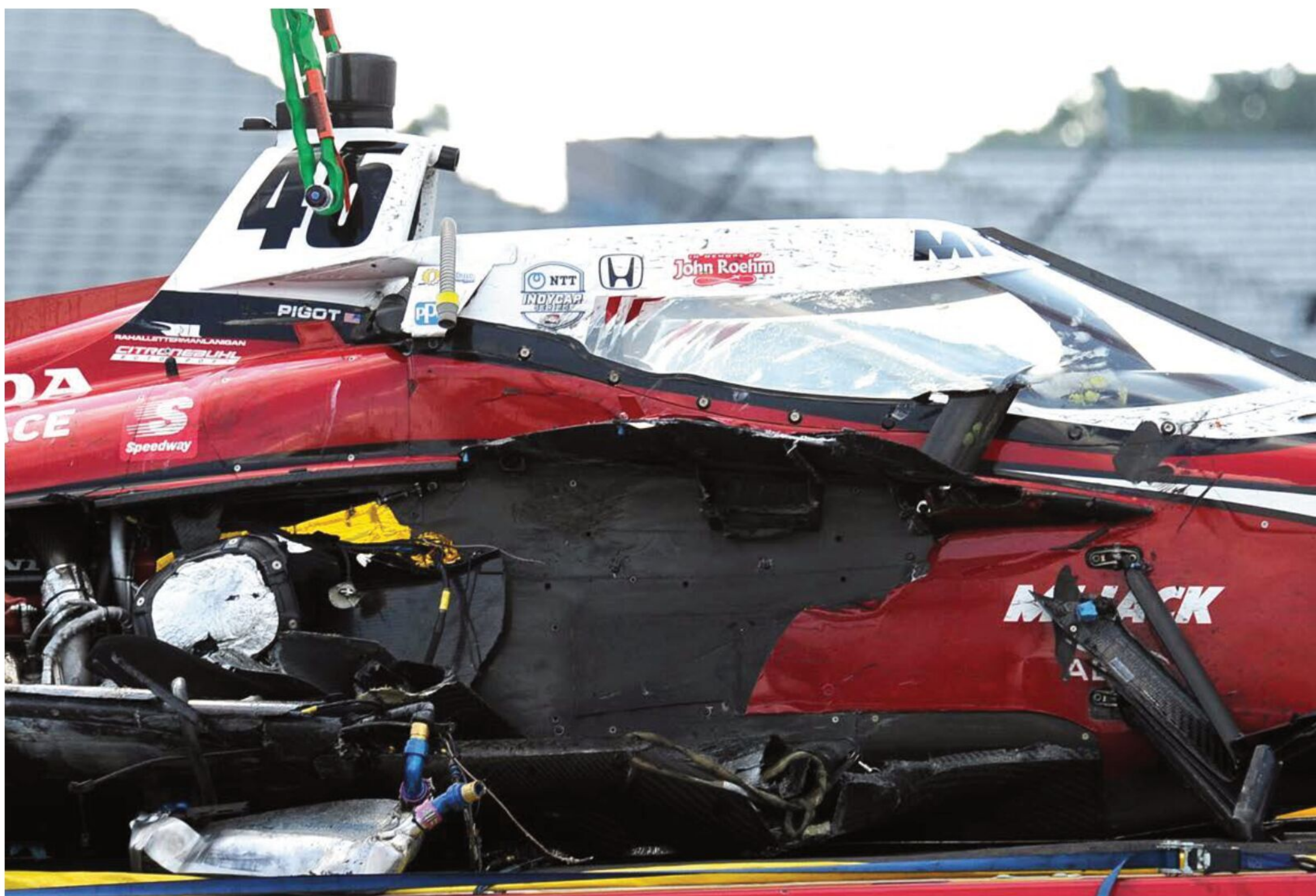
Spencer Pigot's car after crashing into the pit wall at the Indianapolis 500. The windscreen took a significant impact and damage was limited to minor cracking at an upper bolt hole
