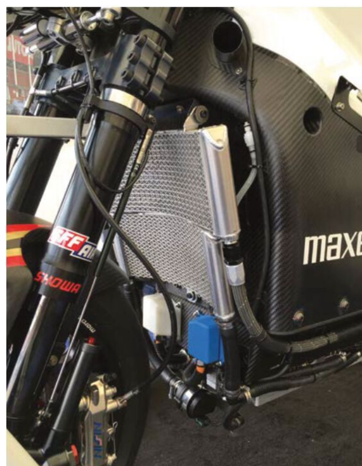
Another benefit of carbon fibre that race teams love is that one element can have multiple roles. Here, a carbon fibre motorcycle chassis doubles as a battery casing and also has cooling channels running through it. It's a complex case, but P2T carbon fibre structures could be suitable given the minimal thermal load here
