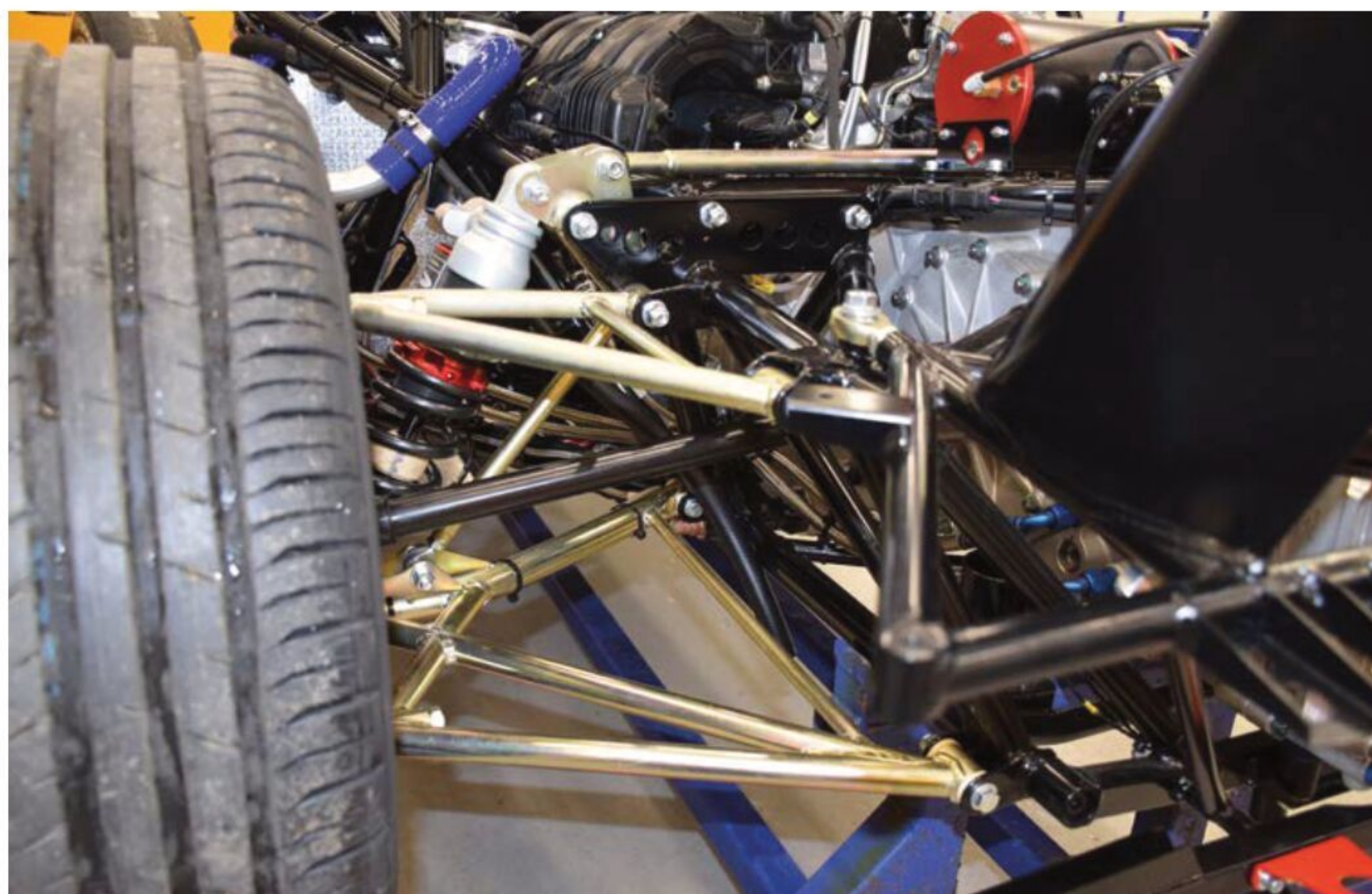
Suspension design is typical of previous Radical products, but the SR10 sees a change to a Hewland TMT200 transmission
