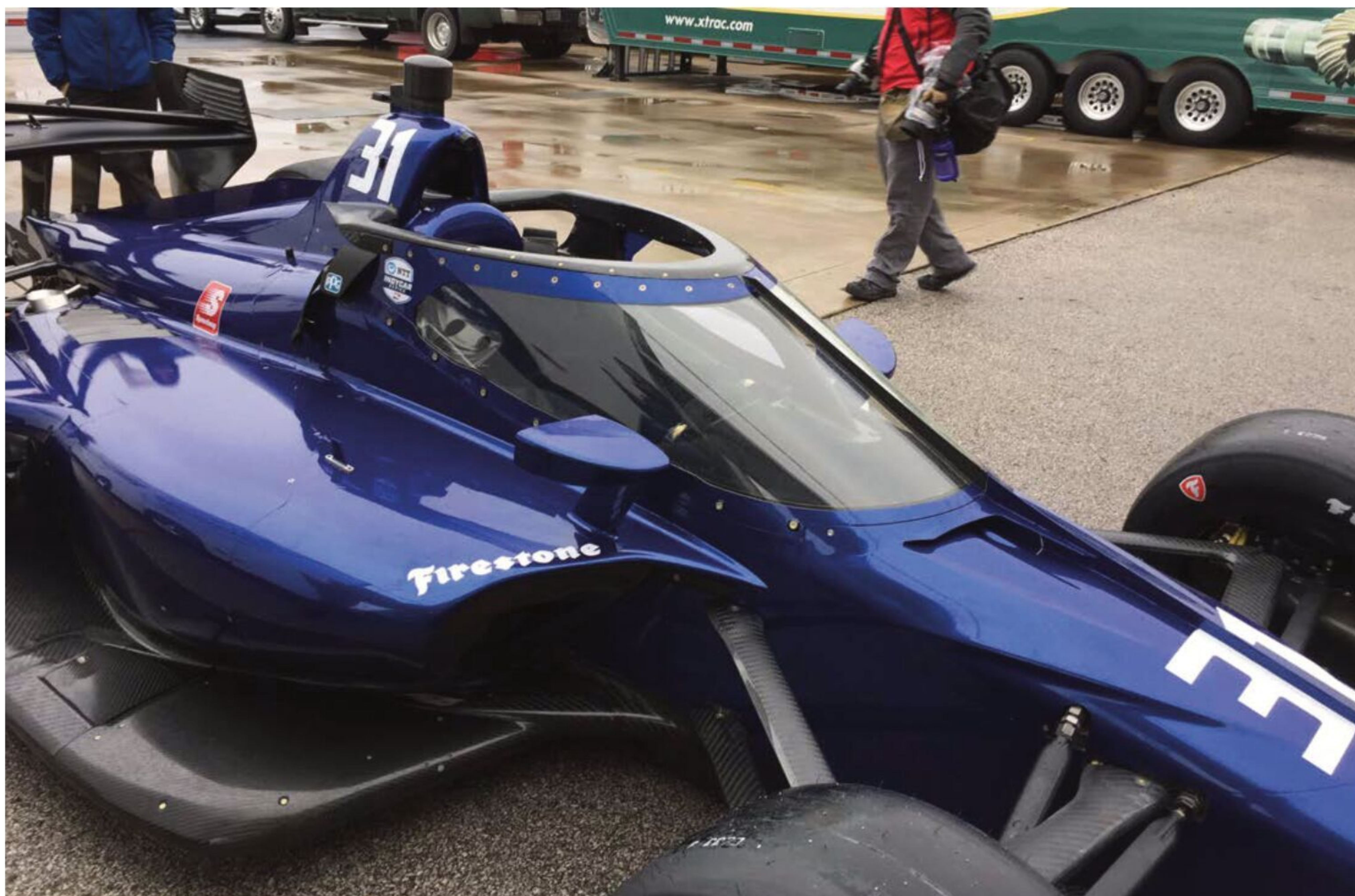
The single-piece windscreen is of triple layer construction, with two plies of polyurethane sandwiched between two layers of impact-resistant polycarbonate. Maximum weight is 18lb
