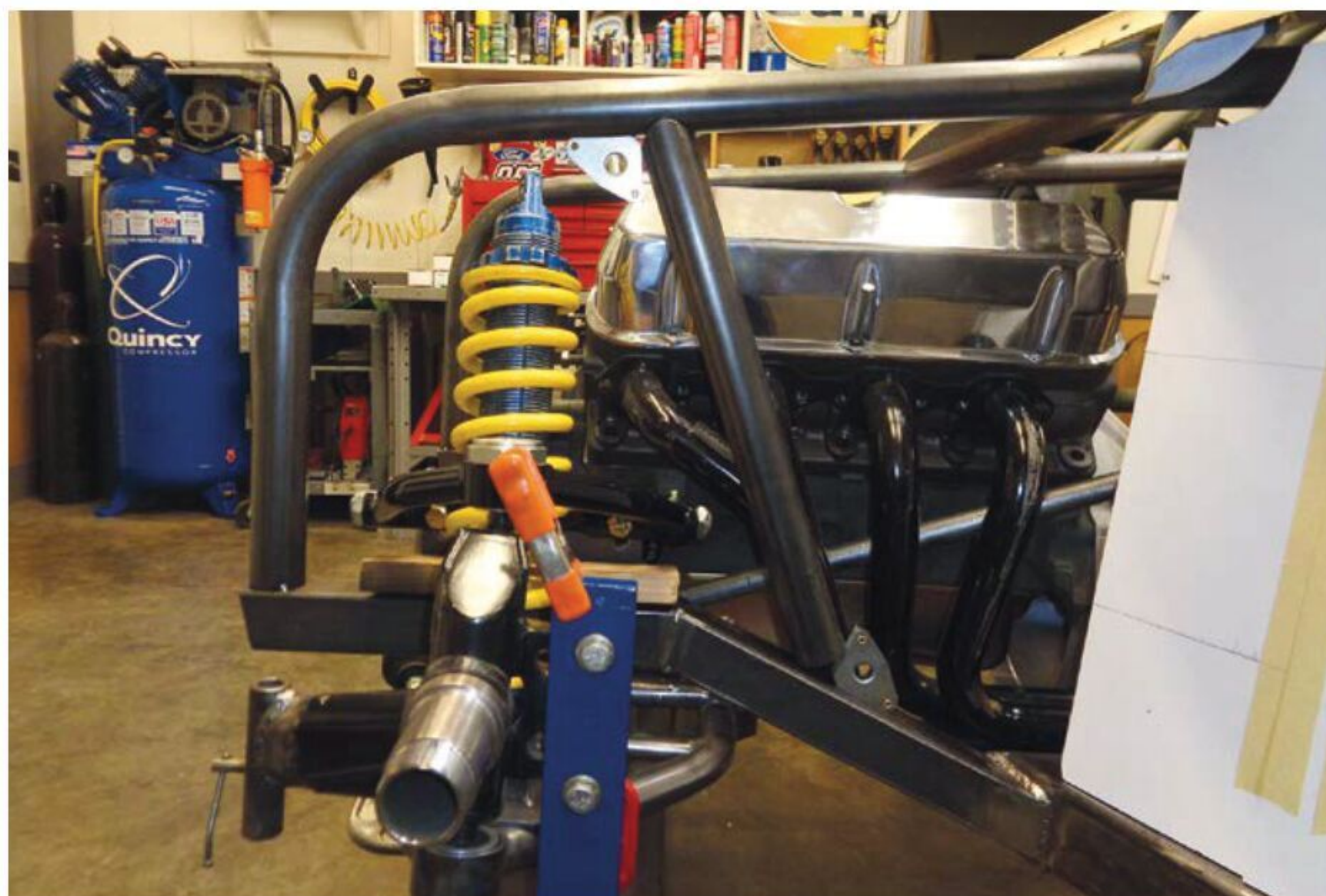
Combining a production car-style ladder frame with a tubular 'cage structure will always be a compromise
