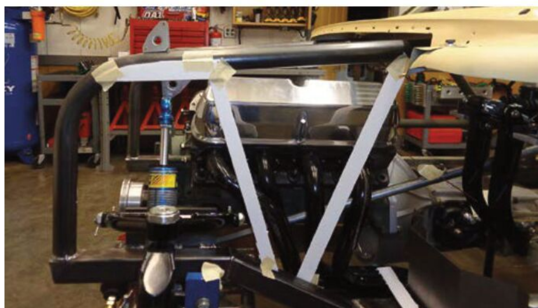
The cardboard represents the questioner's bracing concepts, none of which align with those of The Consultant, who recommends a tubular box structure and motor plate
