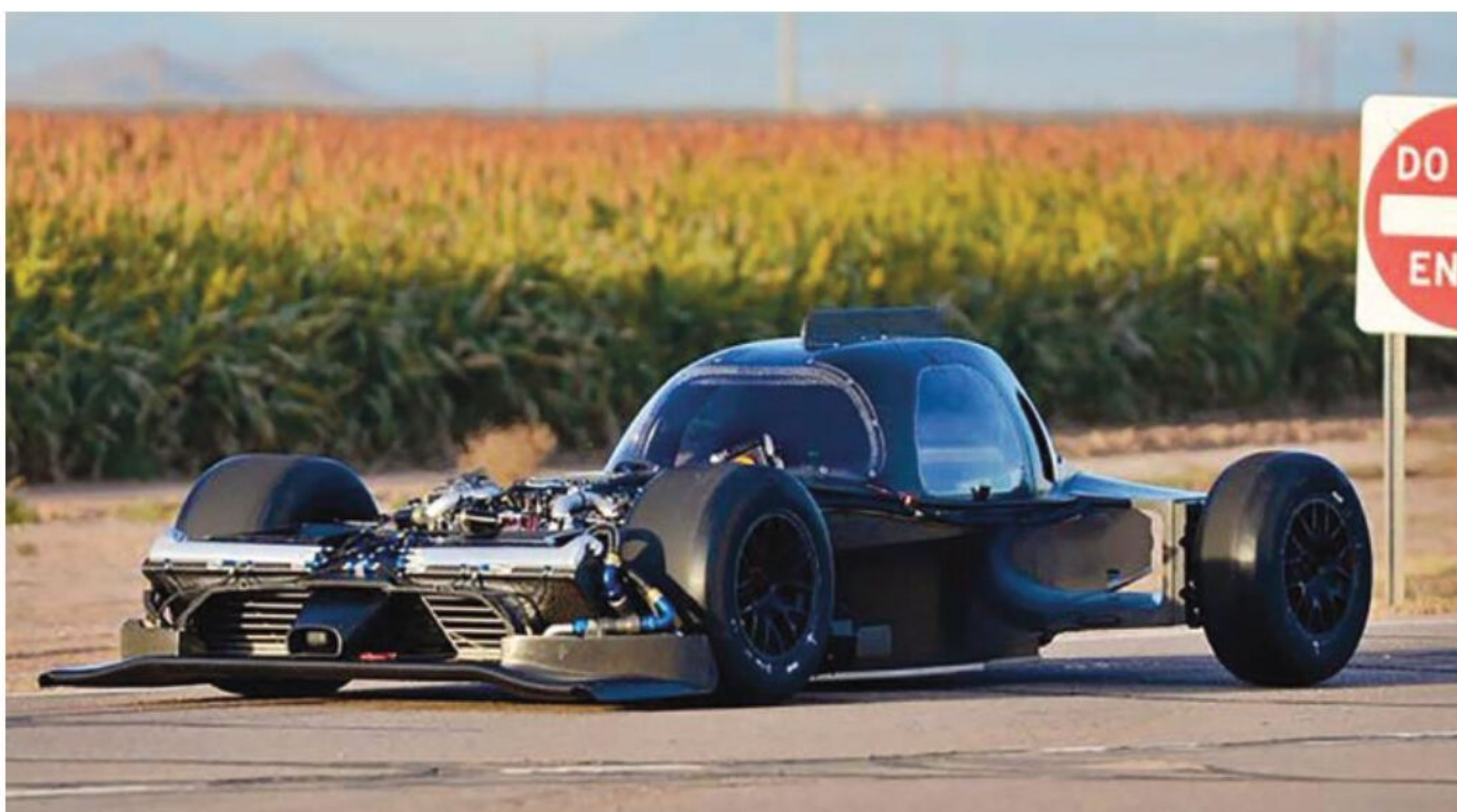
20 November 2014, first run at the Arizona Testing Centre. Without bodywork fitted, the architecture of the car was plain to see. Speeds were kept below 130mph initially for safety reasons, but a gearbox failure hampered the first test session
